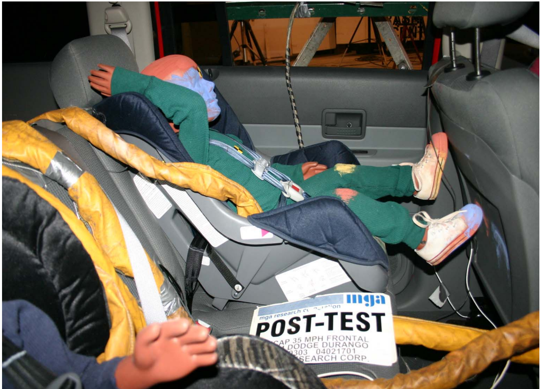
Post-Test Position 4 Right Side View
