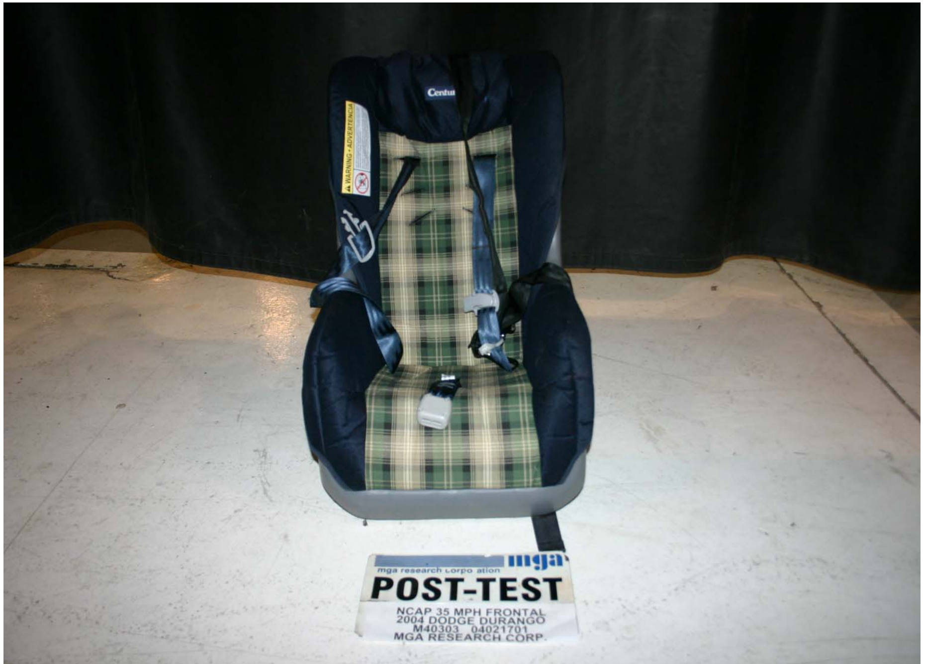
Post-Test Front View of Position 4 CRS
