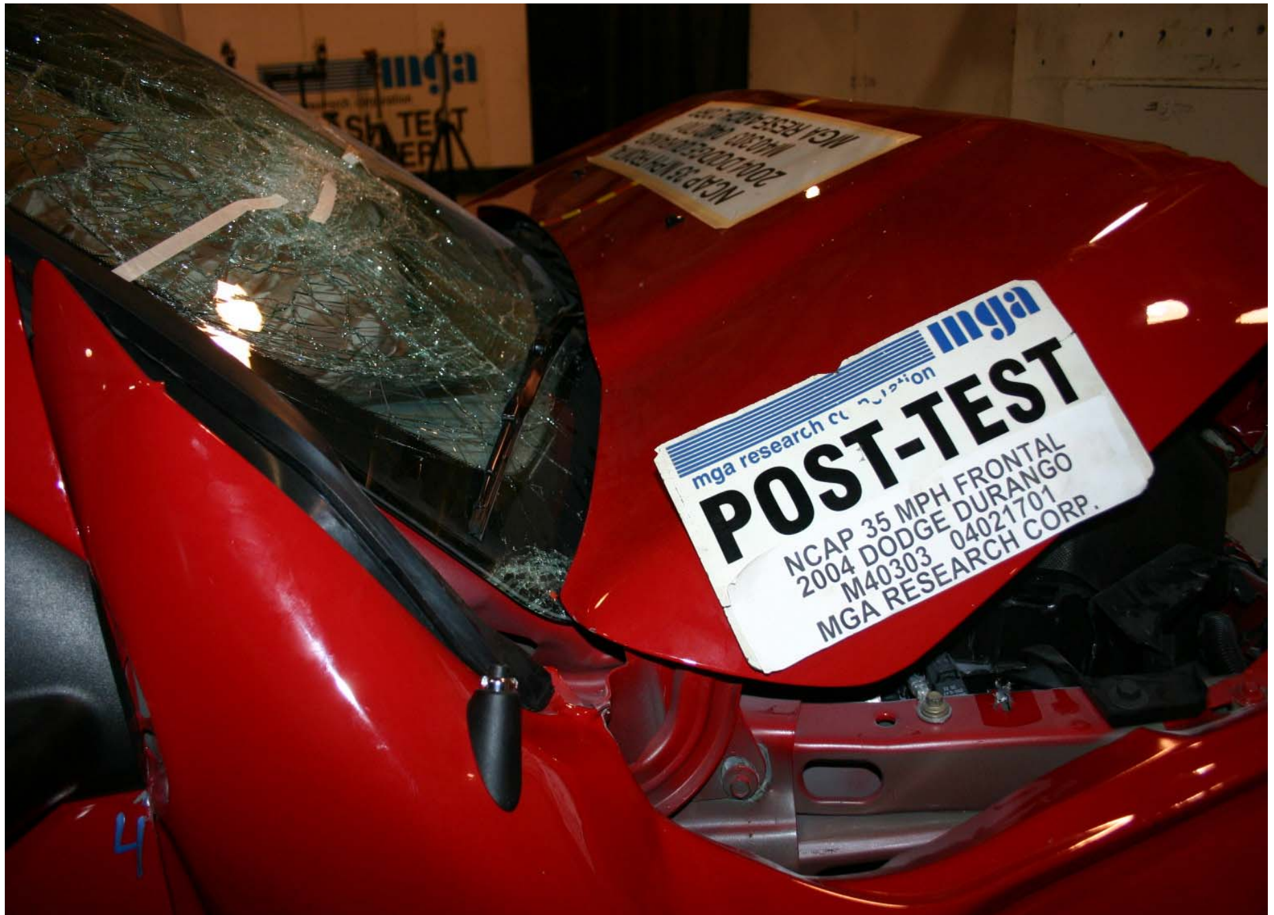
Post-Test Right Side Windshield Molding
