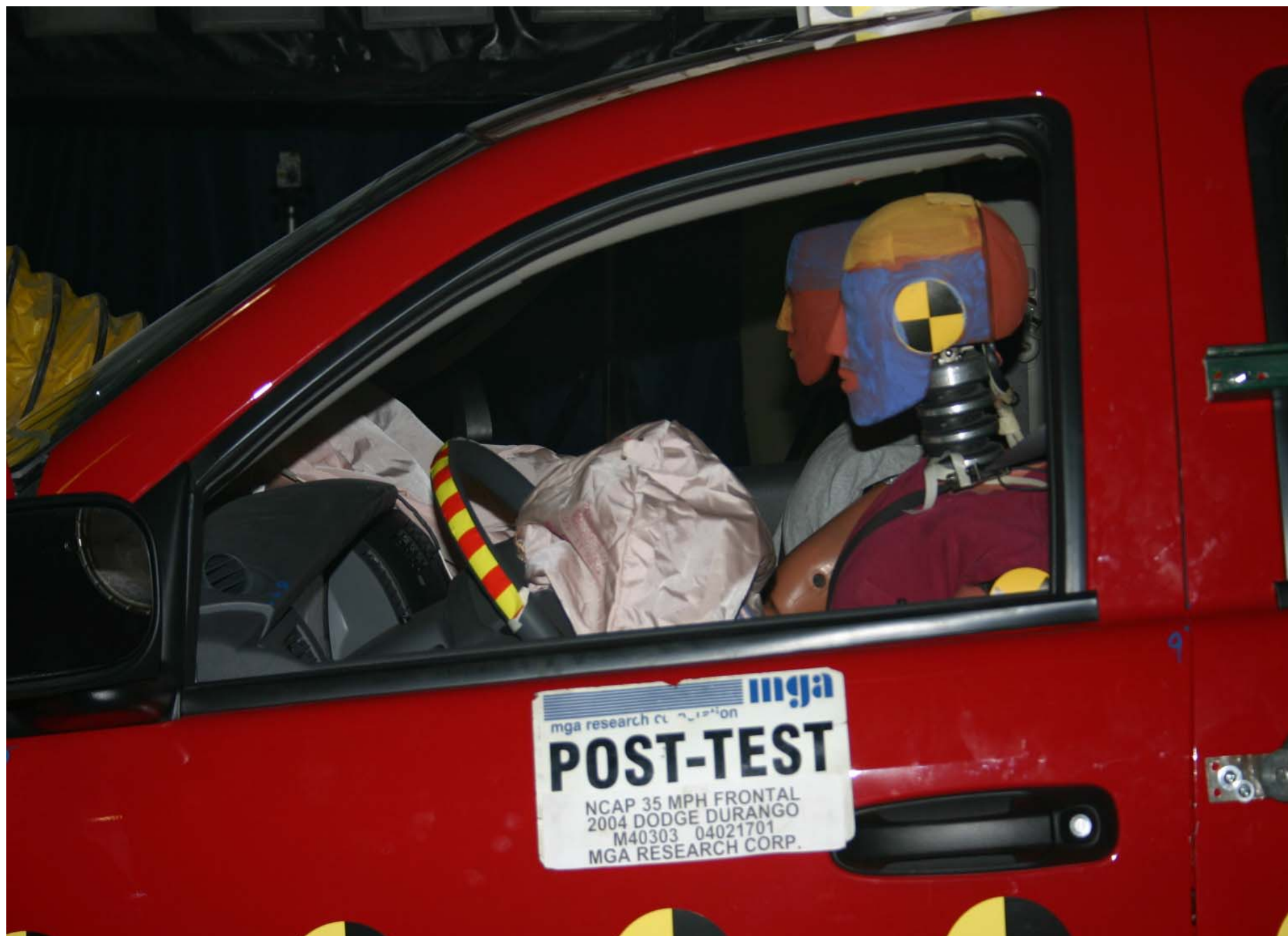
Post-Test Driver Dummy Position Left Side View
