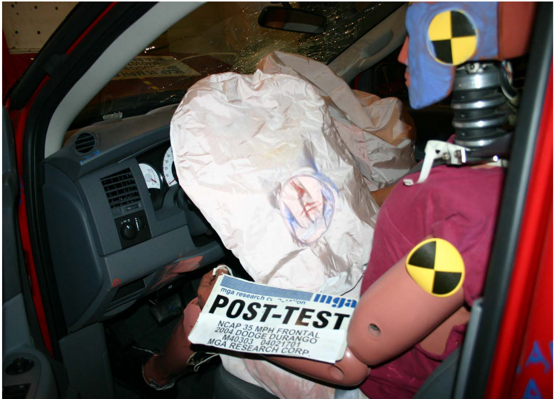
Post-Test Driver Dummy Airbag Contact
