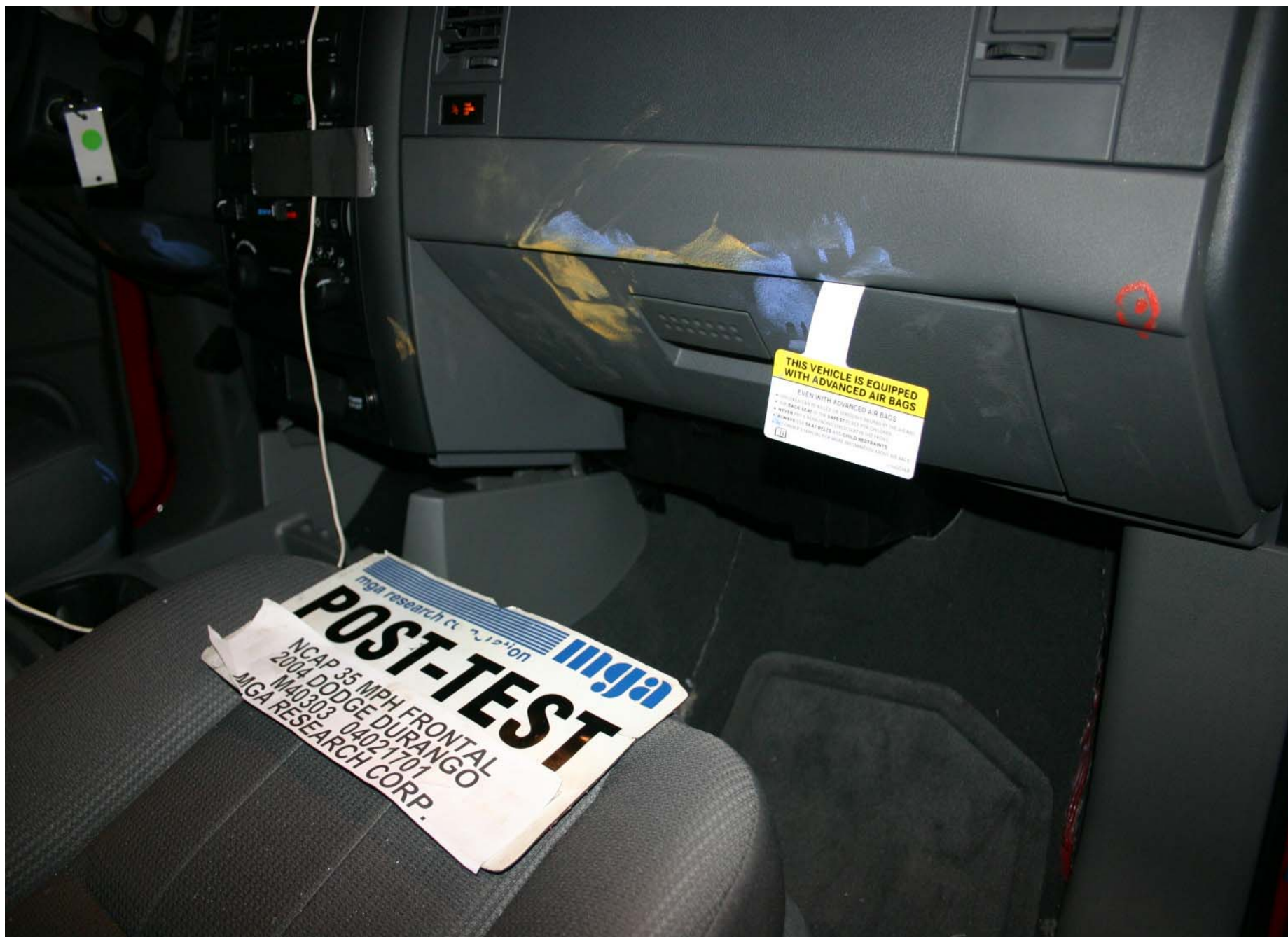
Post-Test Passenger Dummy Knee Contact
