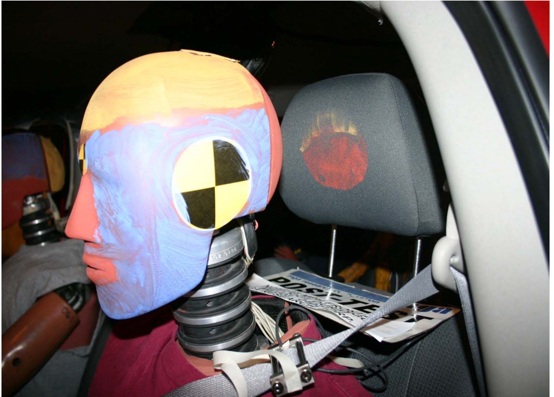
Post-Test Driver Dummy Head Contact
