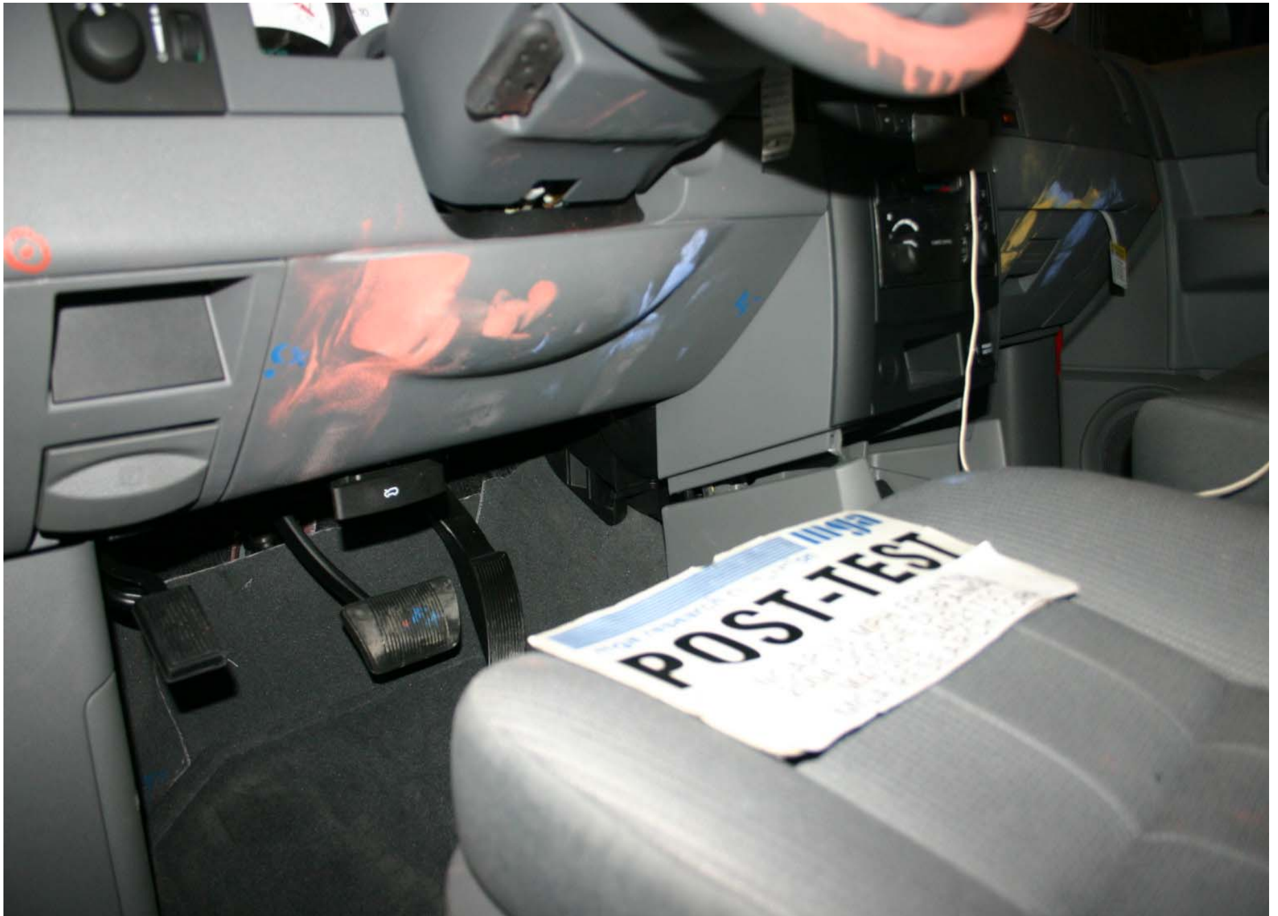
Post-Test Driver Dummy Knee Contact
