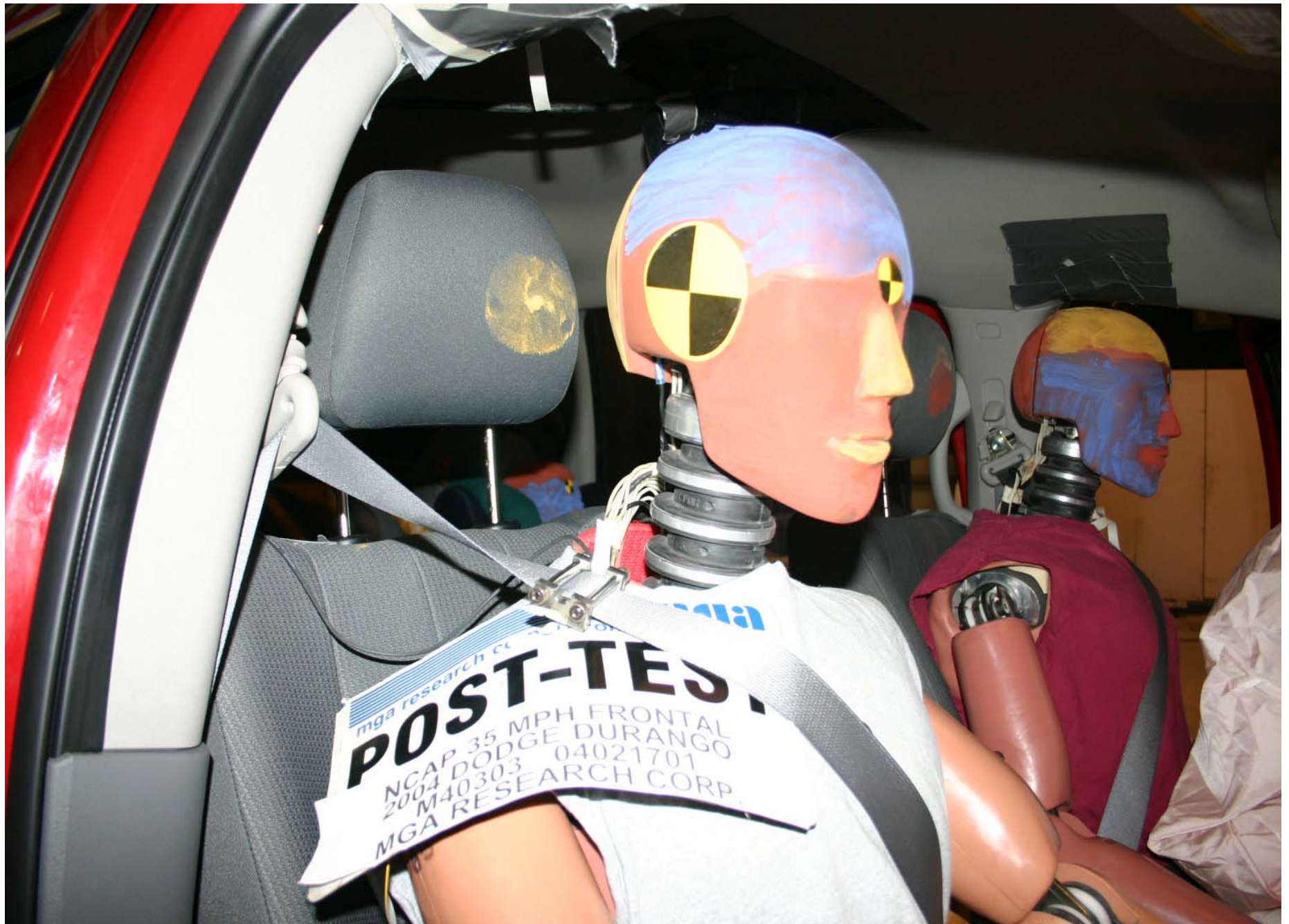
Post-Test Passenger Dummy Head Contact
