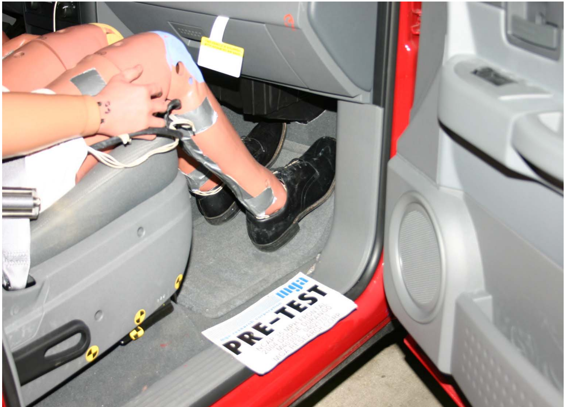
Pre-Test Passenger Dummy Feet Position
