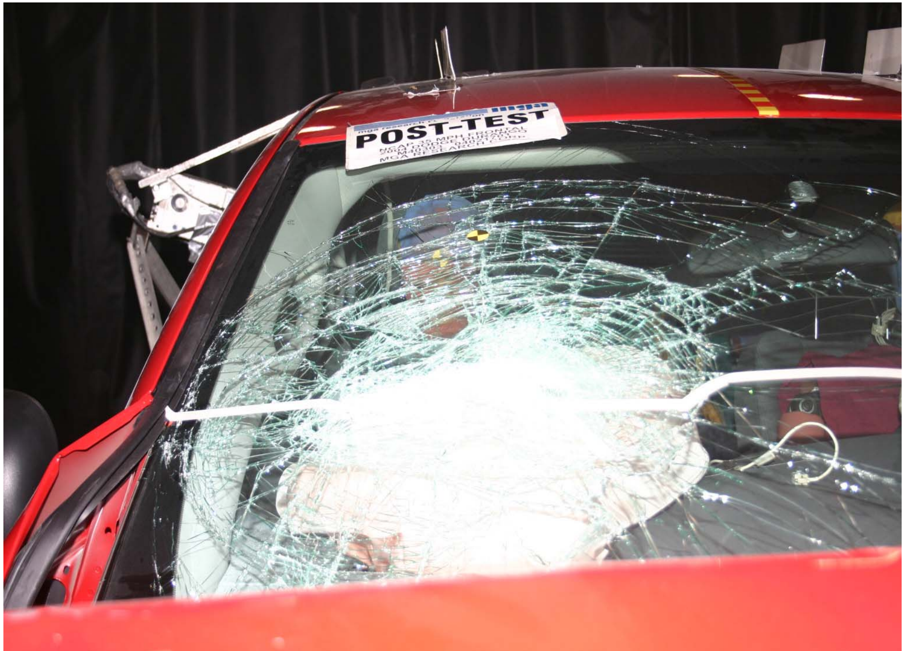
Post-Test Passenger Dummy Front View (head position)
