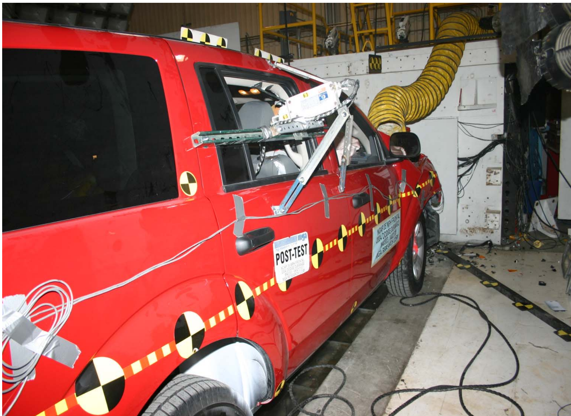
Post-Test Right Rear Three-Quarter View of Doors After Impact
