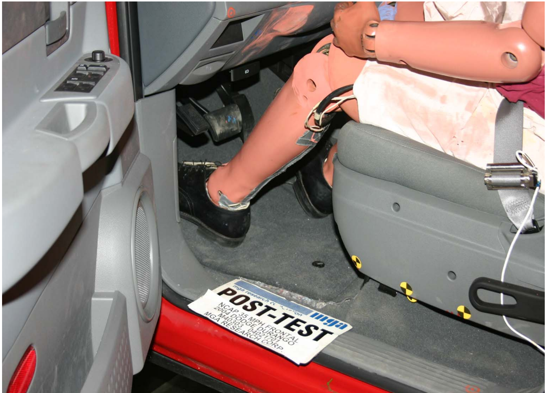
Post-Test Driver Dummy Feet Position
