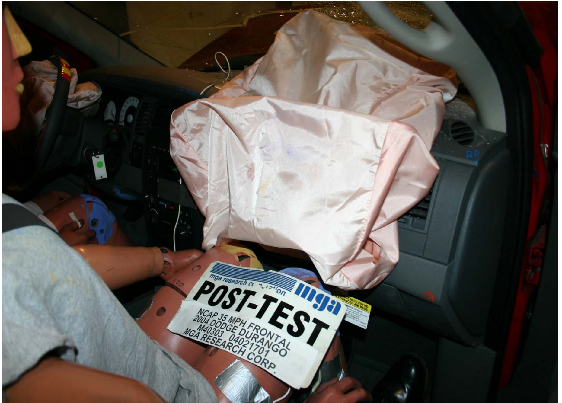
Post-Test Passenger Dummy Airbag Contact
