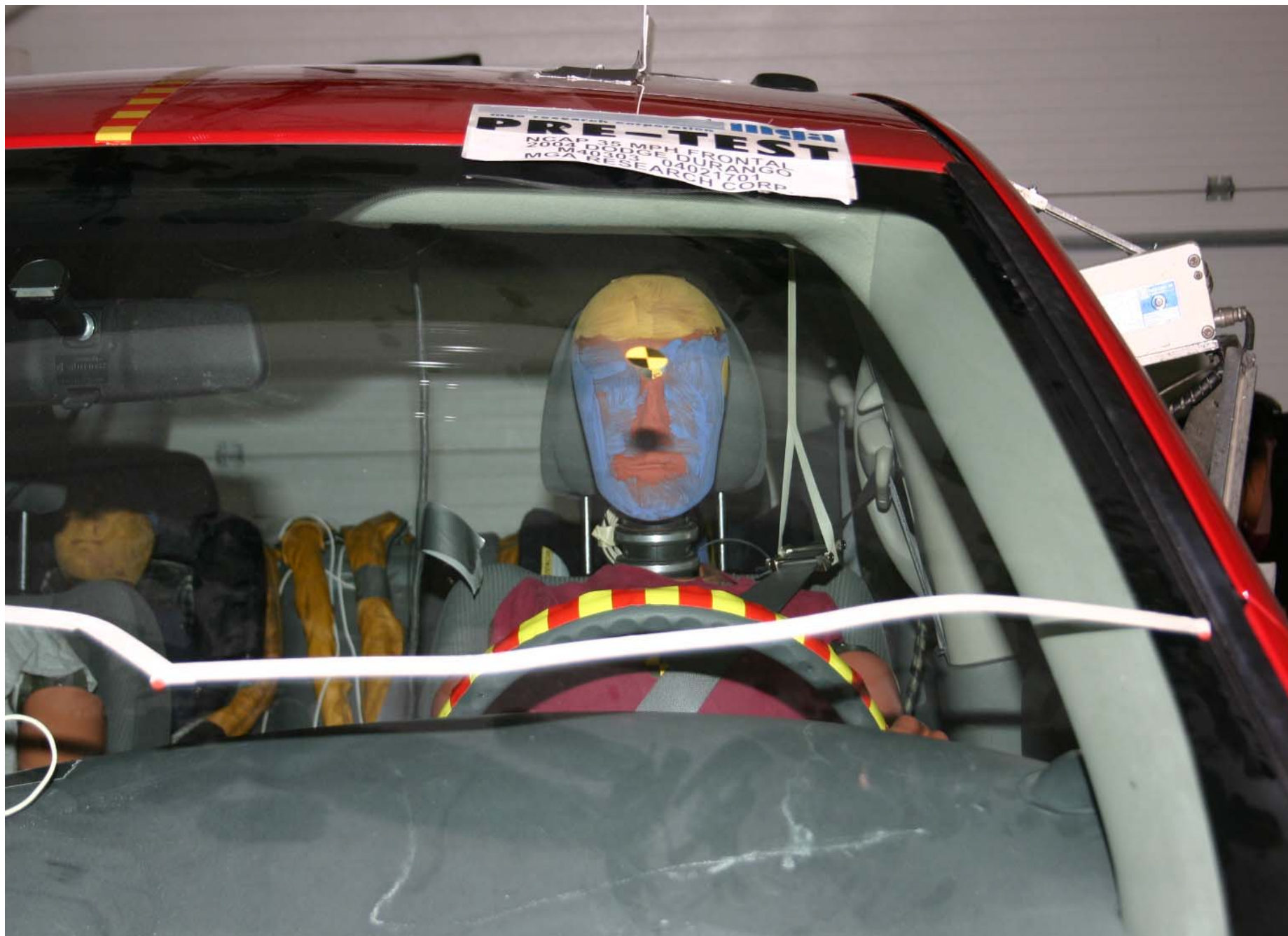
Pre-Test Driver Dummy Front View (head position)
