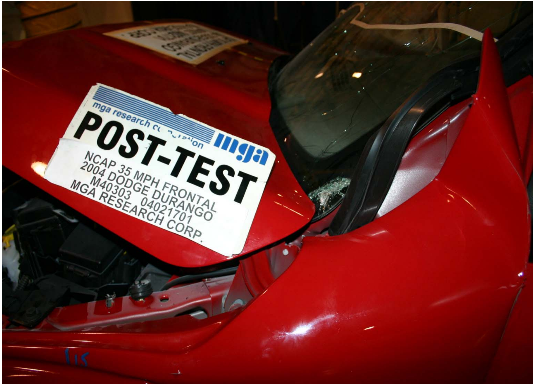
Post-Test Left Side Windshield Molding
