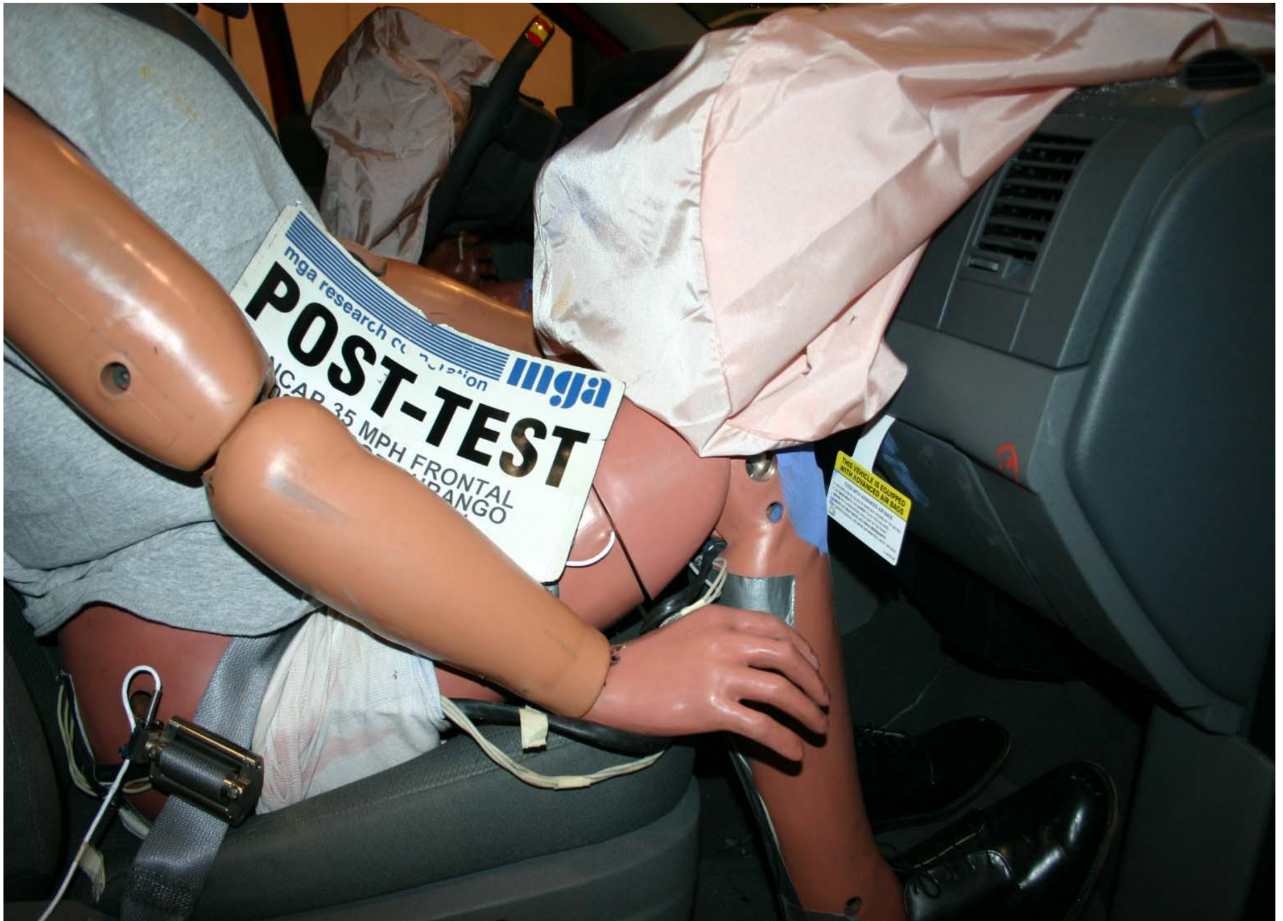
Post-Test Passenger Side Knee Bolster View
