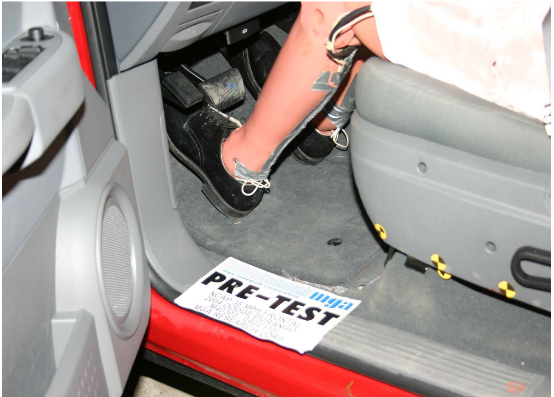
Pre-Test Driver Dummy Feet Position
