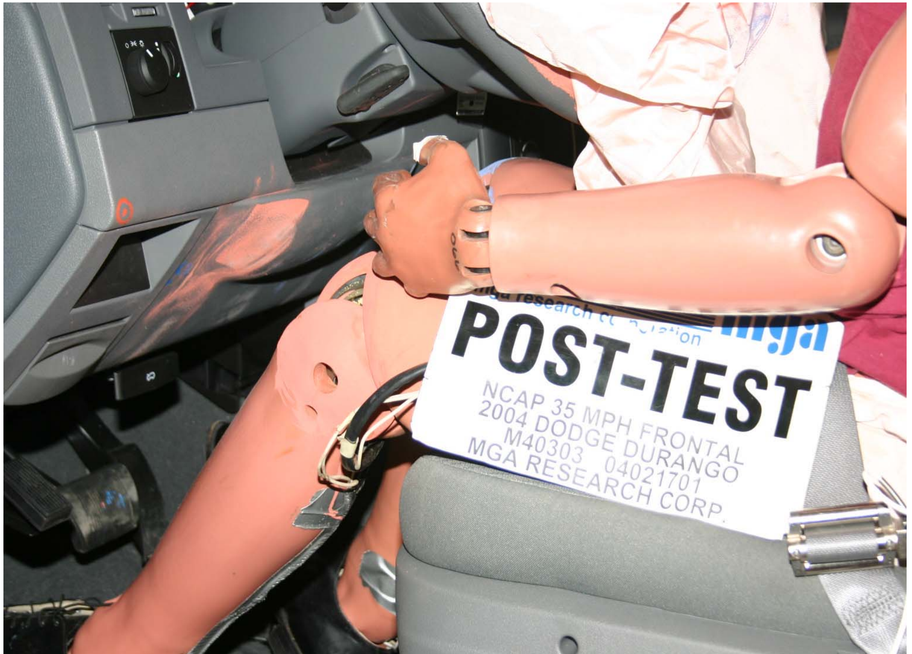
Post-Test Driver Side Knee Bolster View
