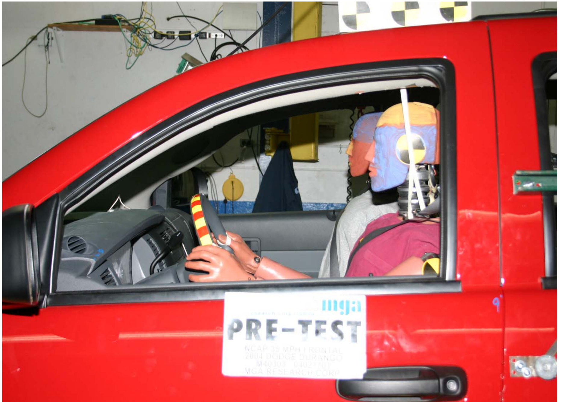
Pre-Test Driver Dummy Position Left Side View
