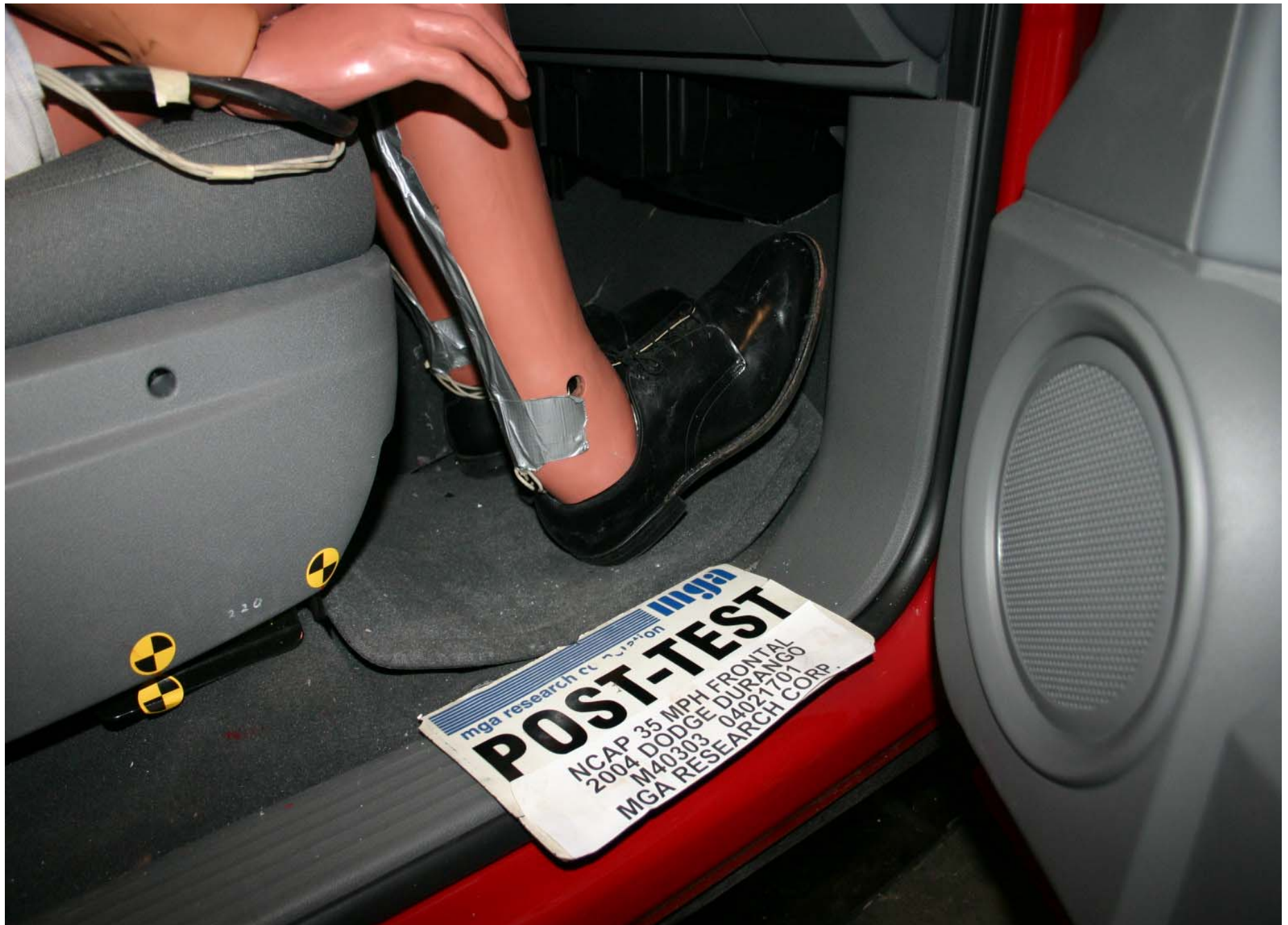
Post-Test Passenger Dummy Feet Position
