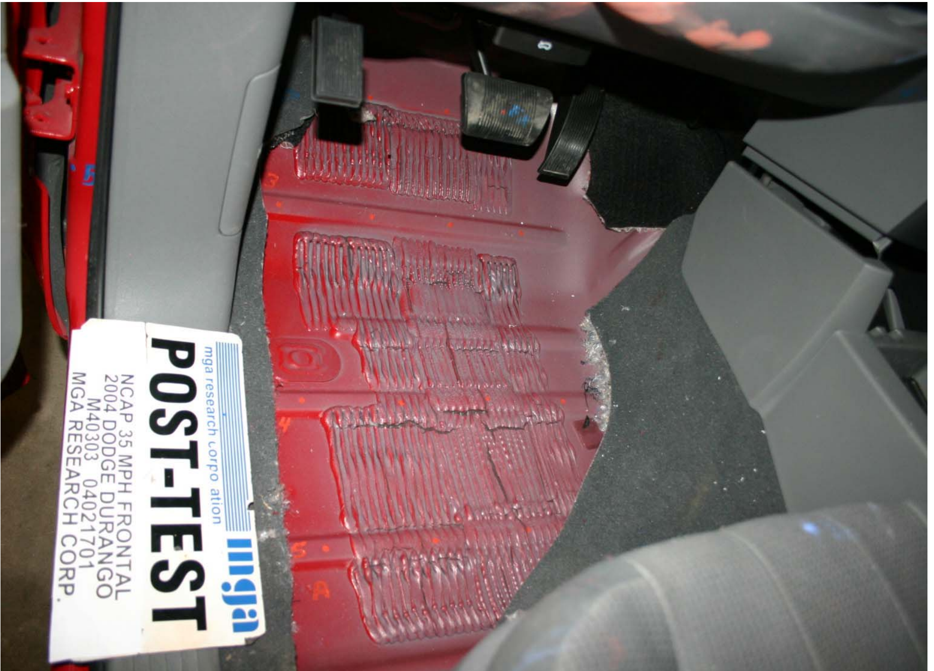
Post-Test Driver Side Floor Pan View
