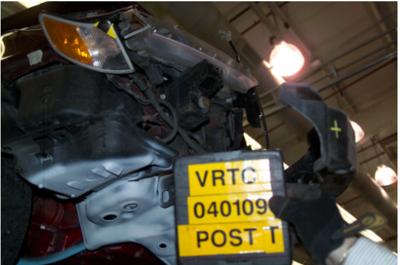
Figure A-94 Post-Test Target Vehicle Bumper Beam Separation View
