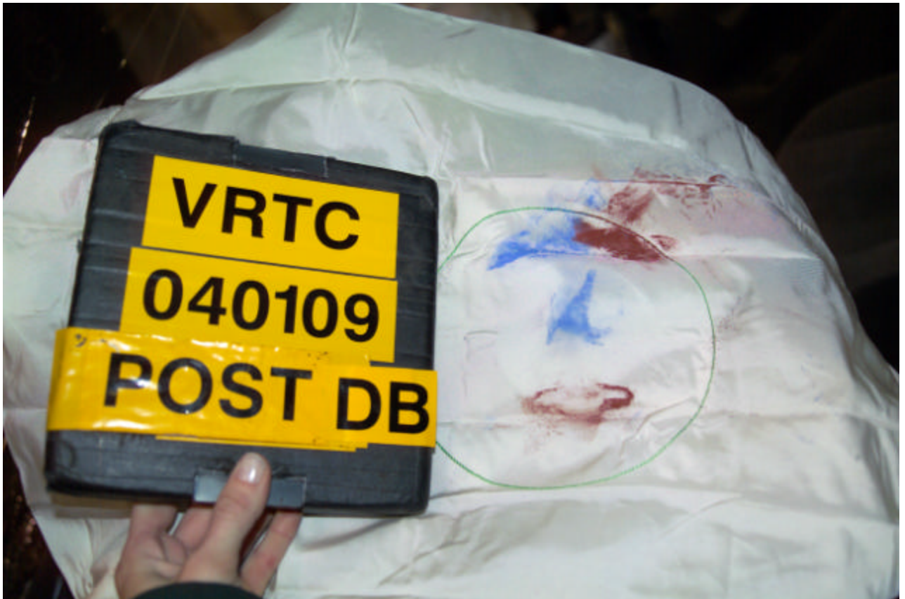
Figure A-80 Post-Test Bullet Vehicle Driver Dummy Head Contact - View 2
