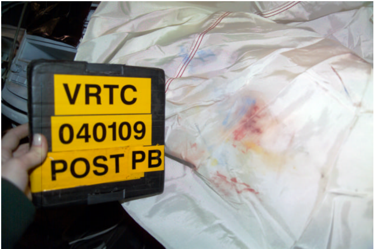
Figure A-85 Post-Test Bullet Vehicle Passenger Dummy Head Contact - View 2
