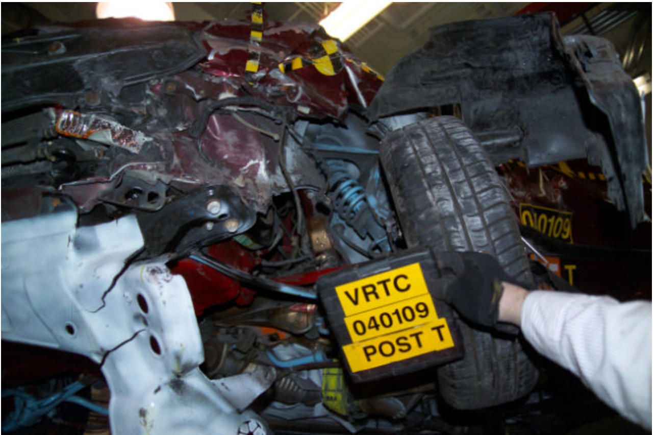
Figure A-92 Post-Test Target Vehicle Subframe Damage - View 1
