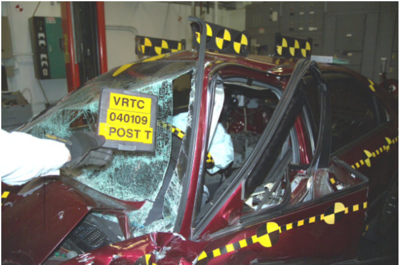
Figure A-96 Post-Test Target Vehicle A-Pillar Damage View
