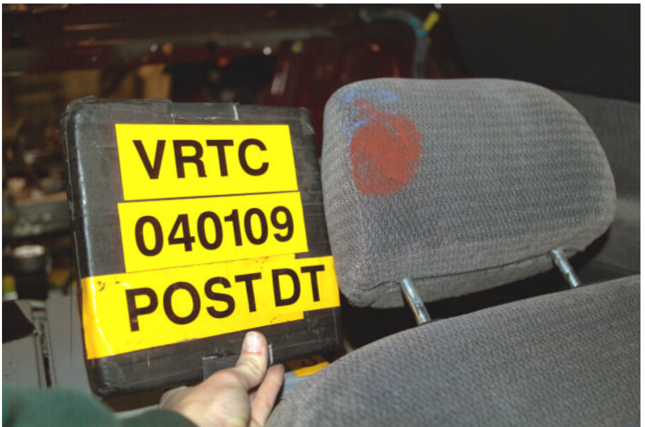
Figure A-76 Post-Test Target Vehicle Driver Dummy Head Contact - View 3
