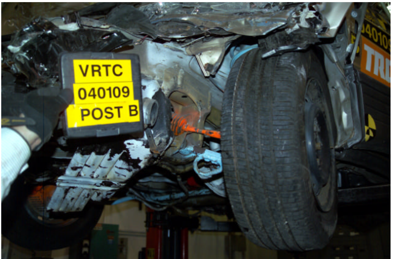
Figure A-100 Post-Test Bullet Vehicle Wheel Area Damage View
