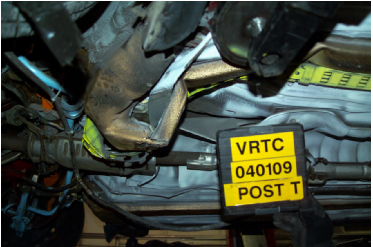
Figure A-93 Post-Test Target Vehicle Subframe Damage - View 2
