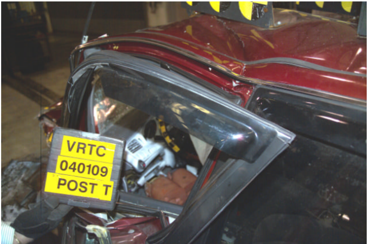
Figure A-97 Post-Test Target Vehicle Roof Damage View
