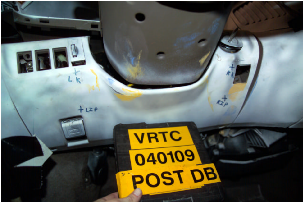
Figure A-82 Post-Test Bullet Vehicle Driver Dummy Knee Contact - View 2
