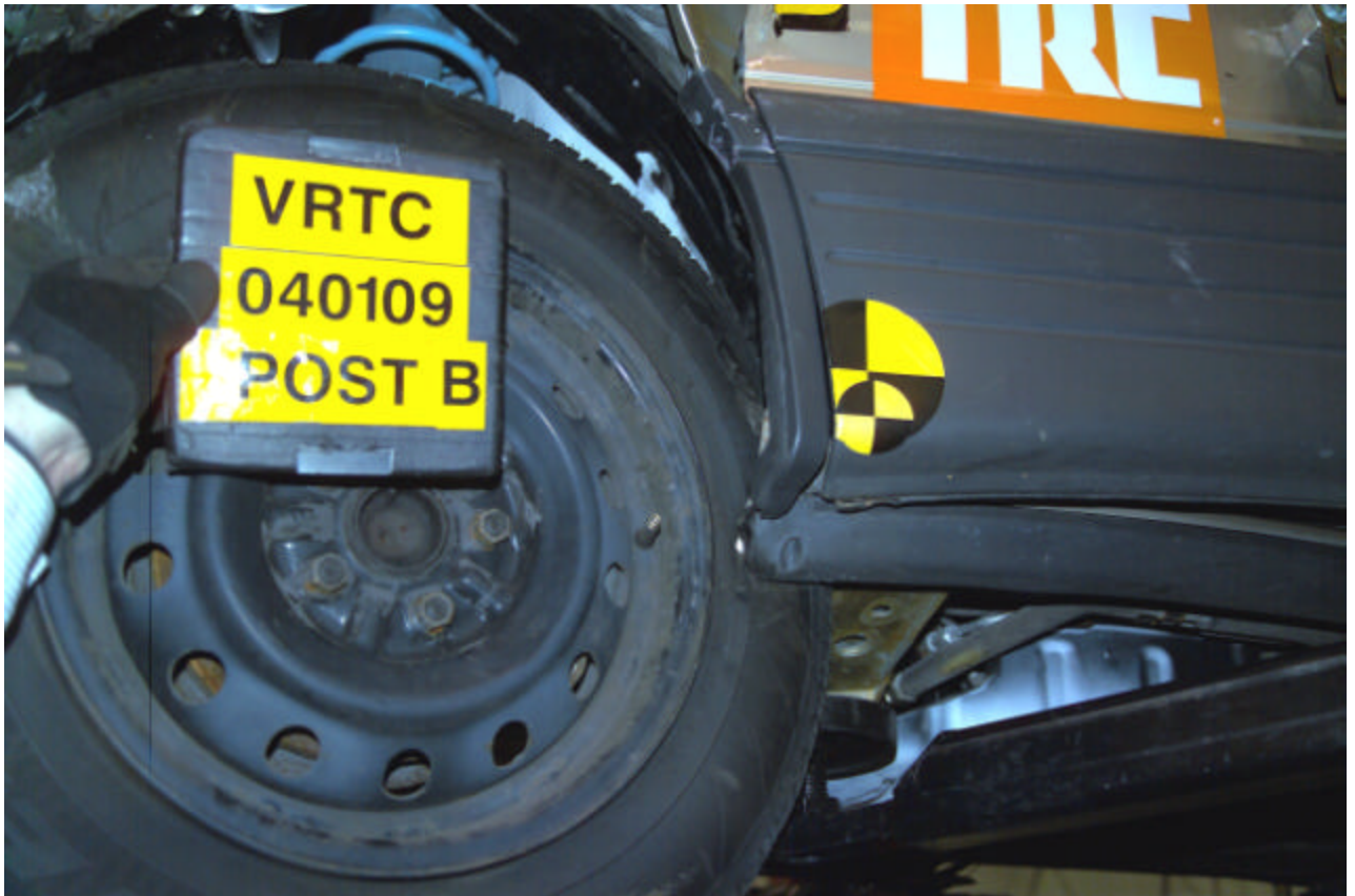
Figure A-99 Post-Test Bullet Vehicle Wheel to Rocker Contact View
