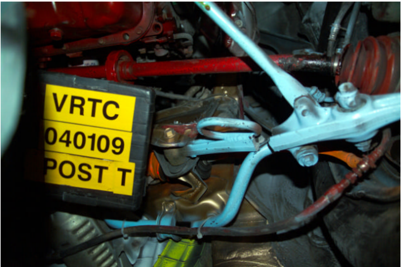
Figure A-95 Post-Test Target Vehicle Suspension Damage View
