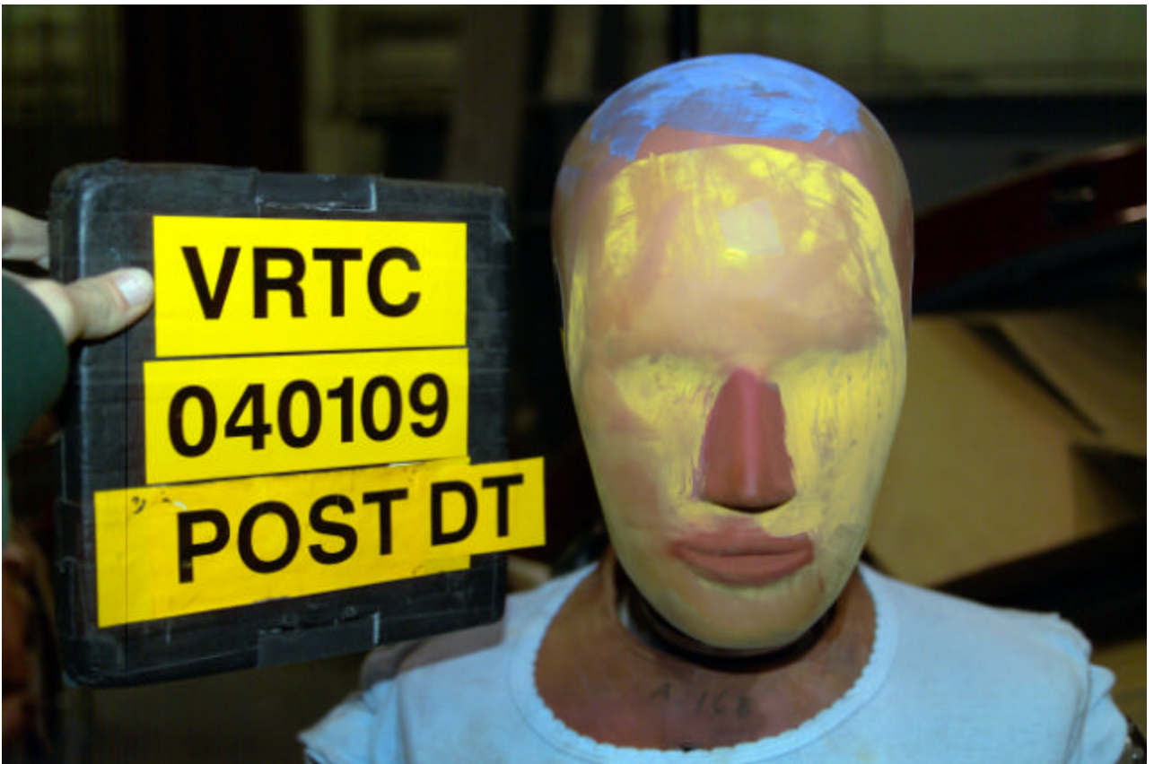
Figure A-74 Post-Test Target Vehicle Driver Dummy Head Contact - View 1
