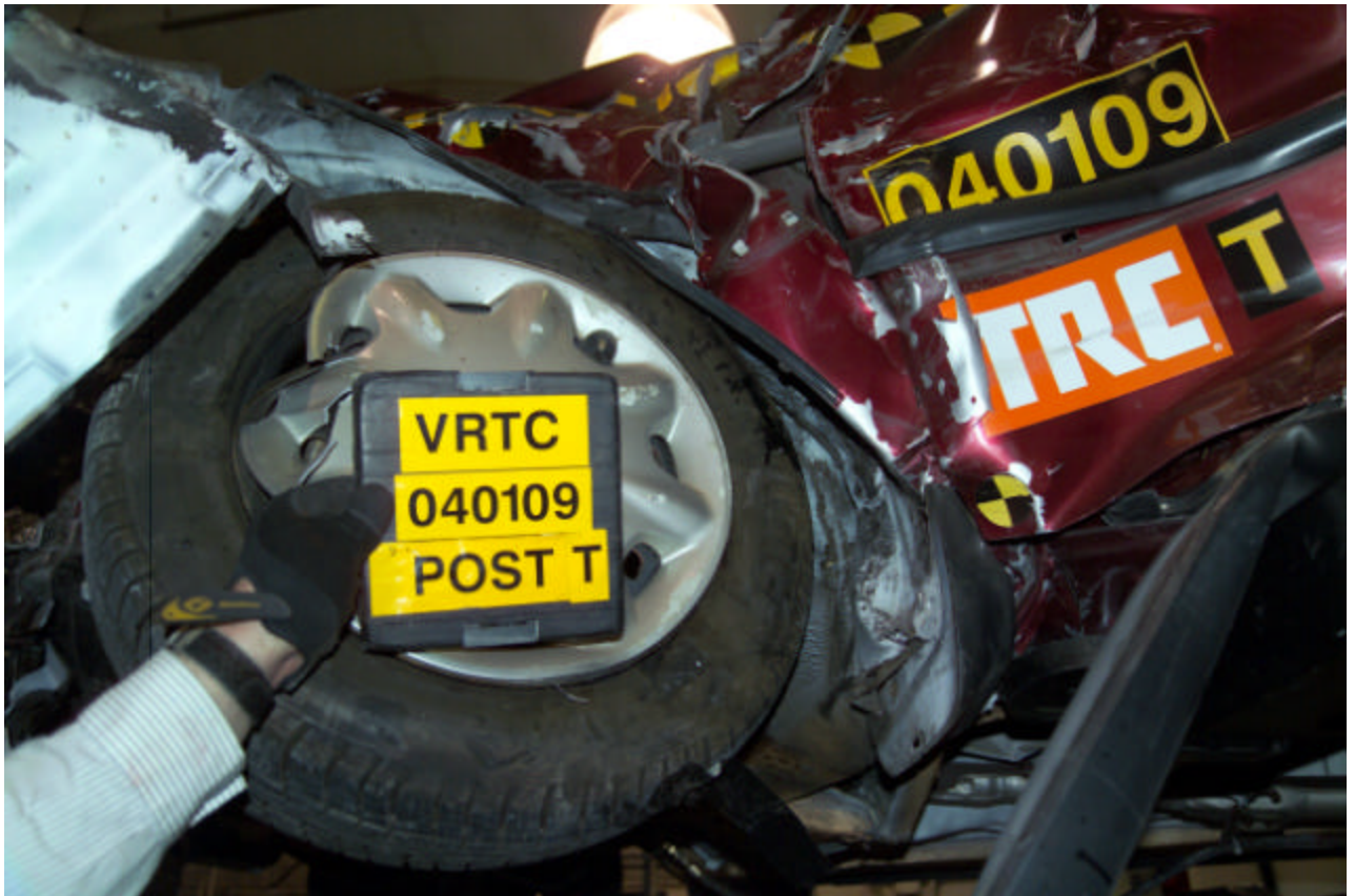
Figure A-98 Post-Test Target Vehicle Wheel to Rocker Contact View
