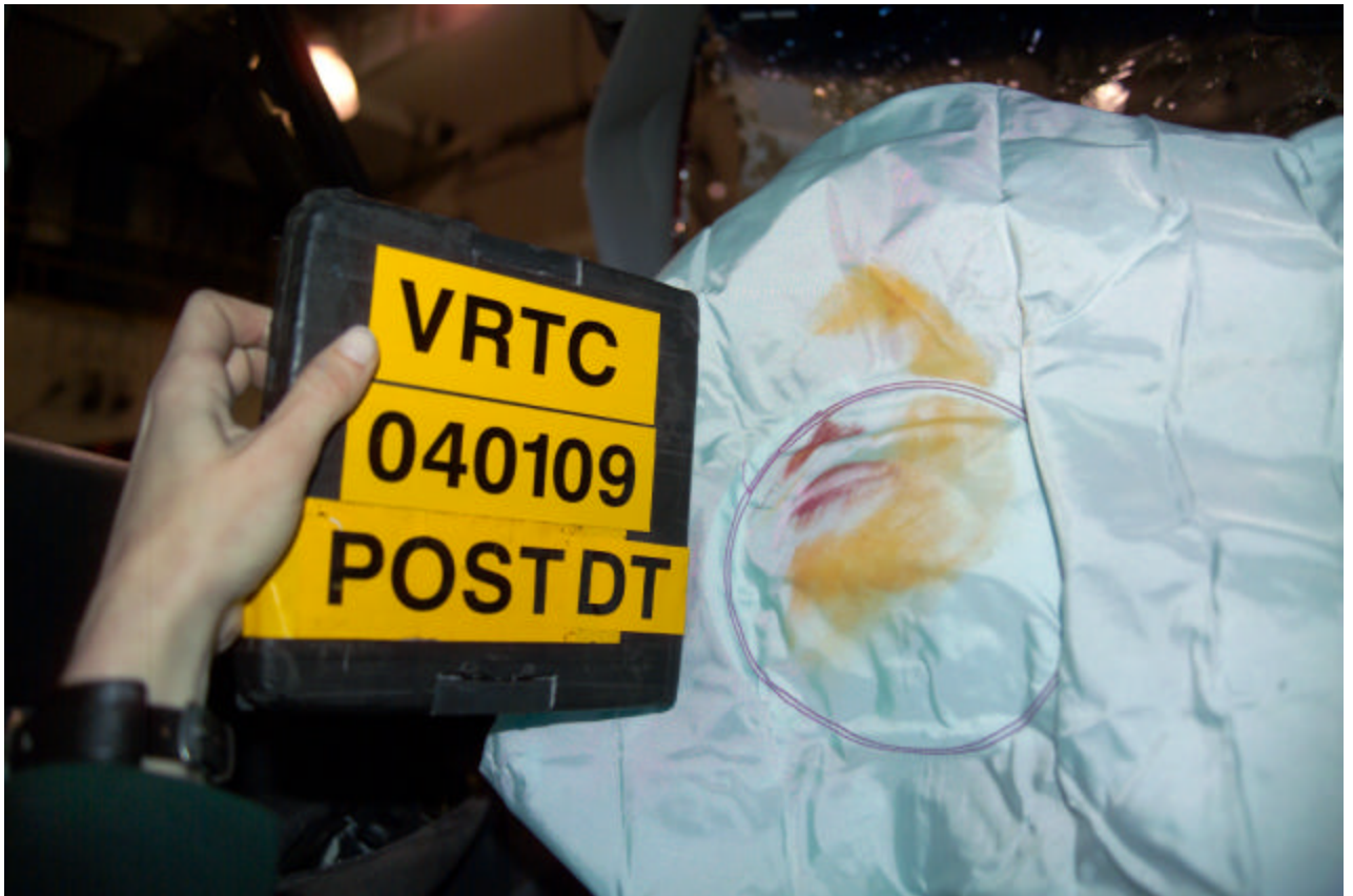
Figure A-75 Post-Test Target Vehicle Driver Dummy Head Contact - View 2
