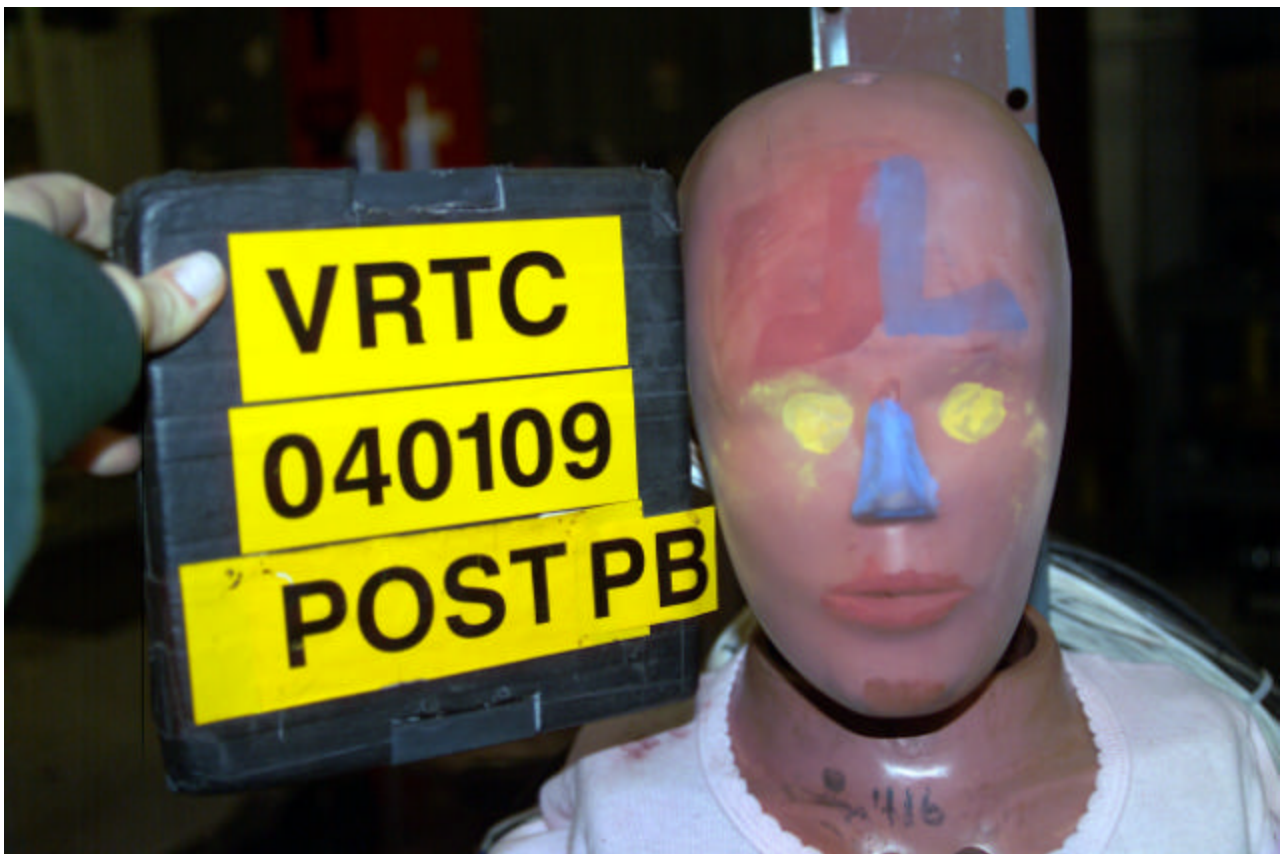
Figure A-84 Post-Test Bullet Vehicle Passenger Dummy Head Contact - View 1
