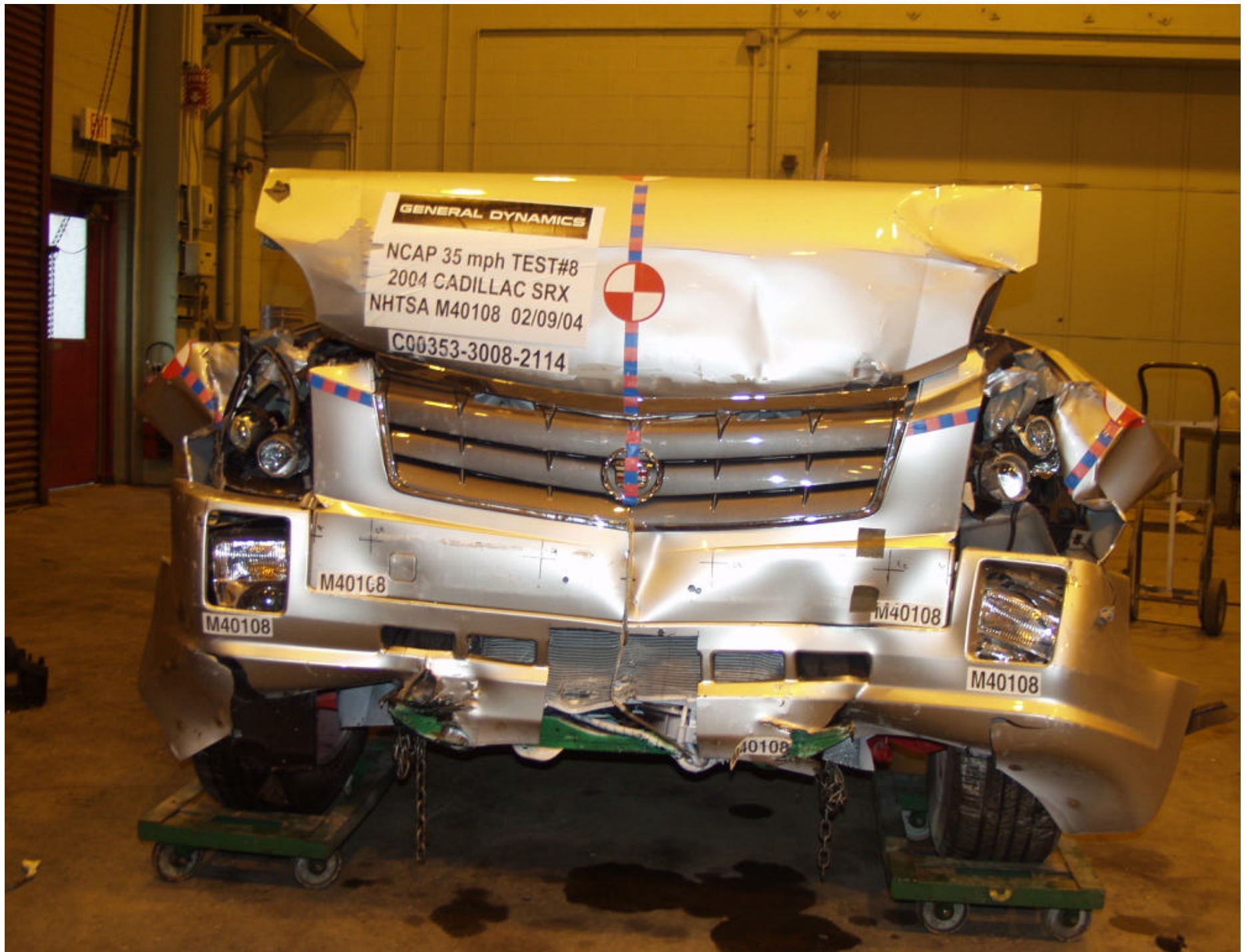
Figure A-7 POST-TEST FRONT VIEW
