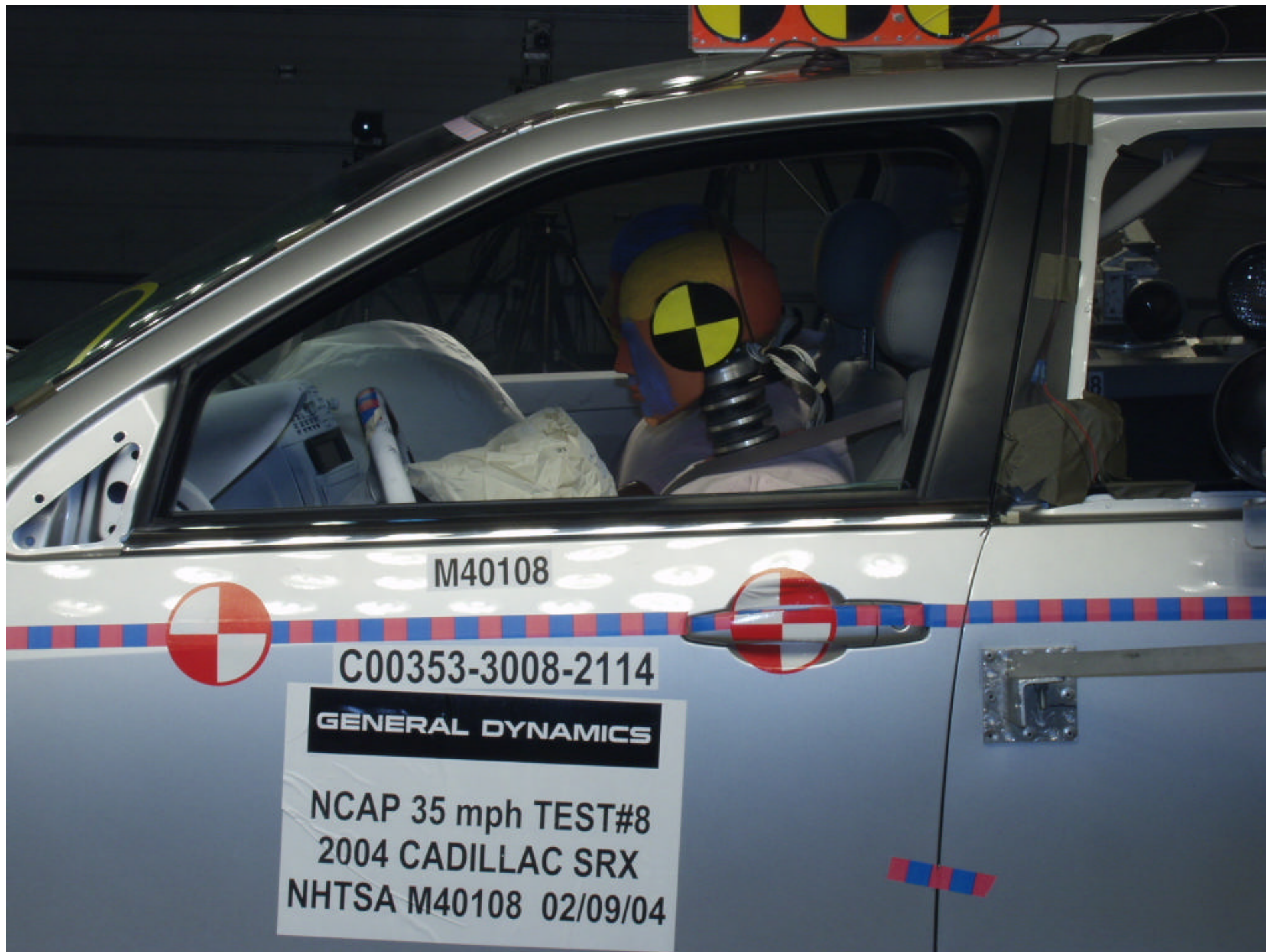
Figure A-33 POST-TEST DRIVER POSITION VIEW
