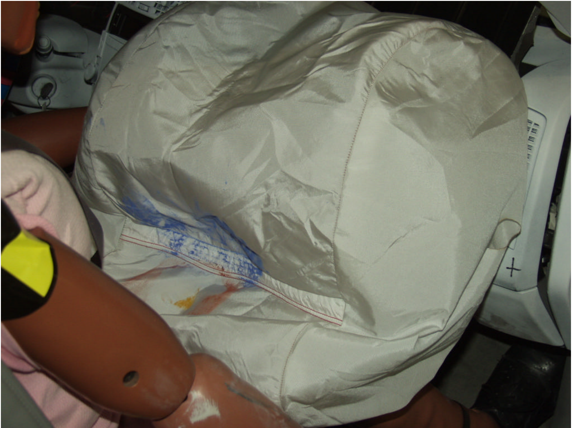
Figure A-57 POST-TEST PASSENGER CONTACT TO AIRBAG
