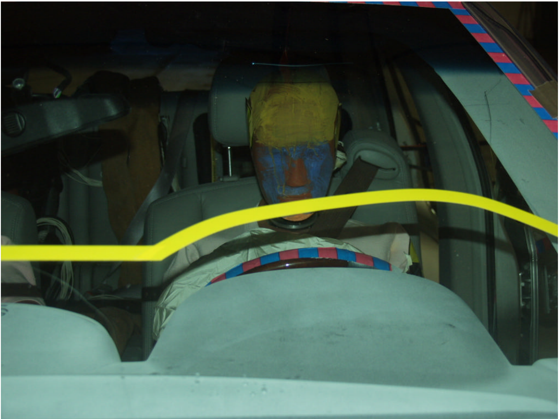
Figure A-31 POST-TEST DRIVER HEAD LOCATION
