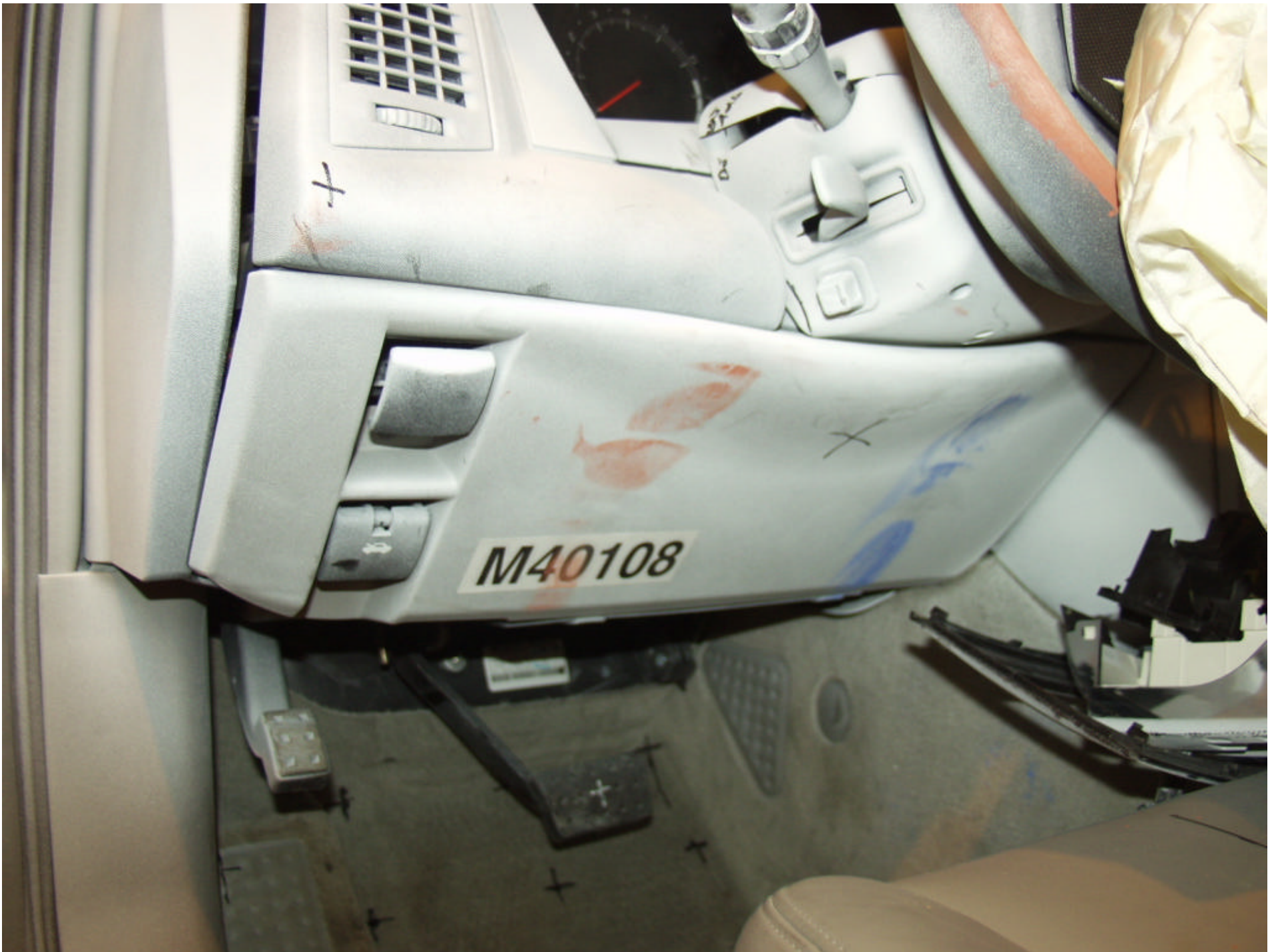
Figure A-39 POST-TEST DRIVER KNEE BOLSTER VIEW
