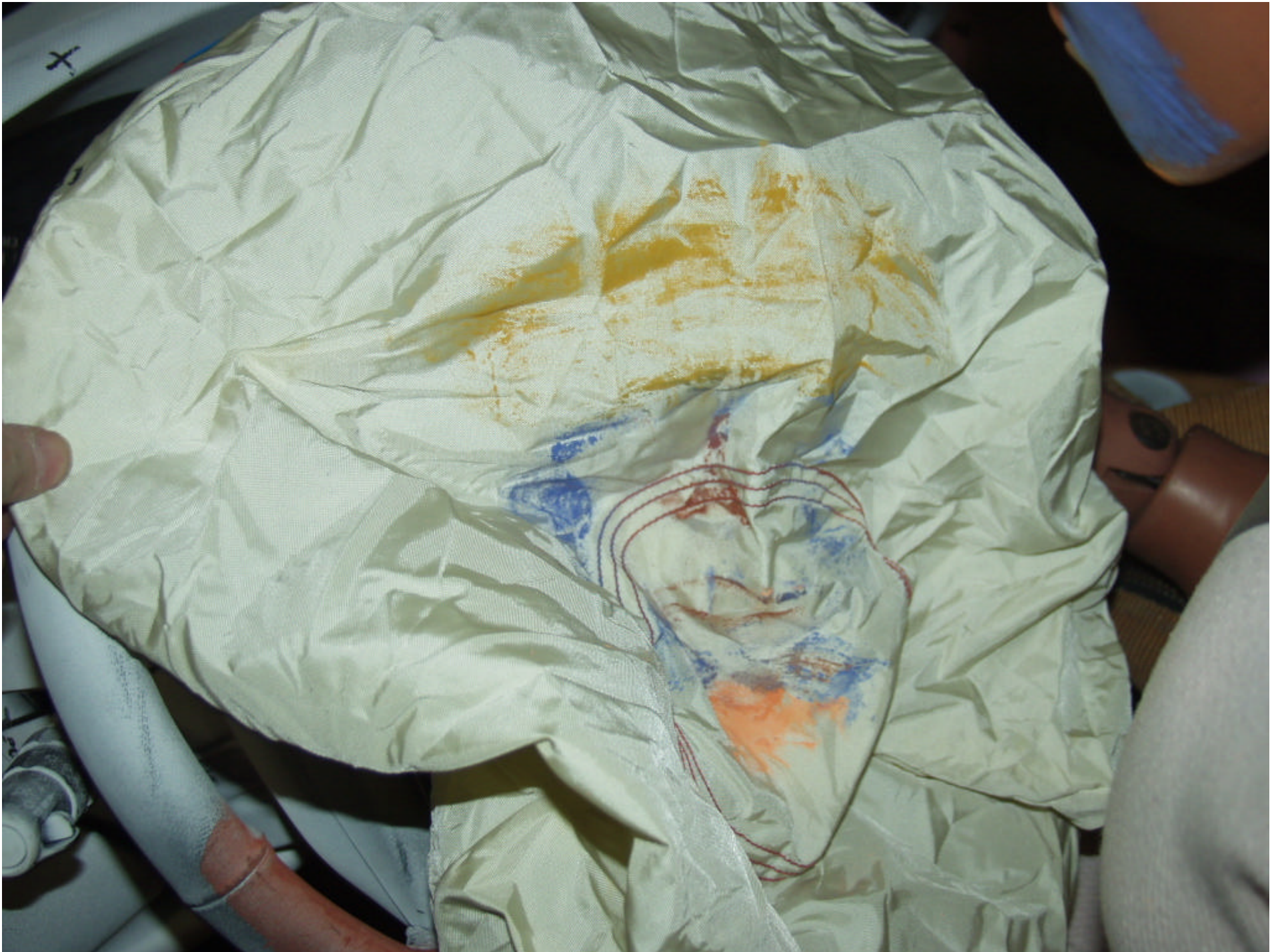
Figure A-43 POST-TEST DRIVER CONTACT TO AIRBAG
