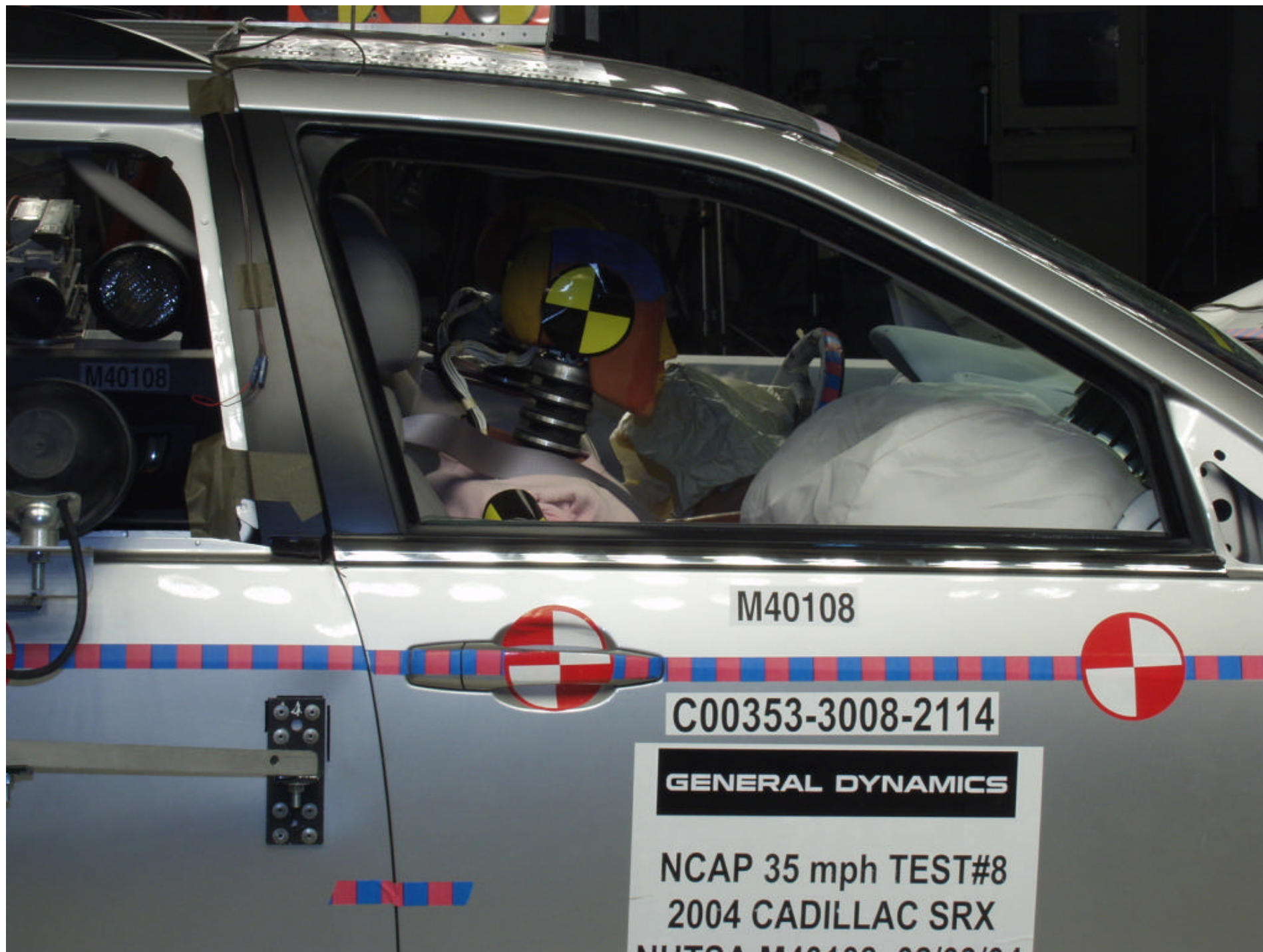
Figure A-47 POST-TEST PASSENGER POSITION VIEW
