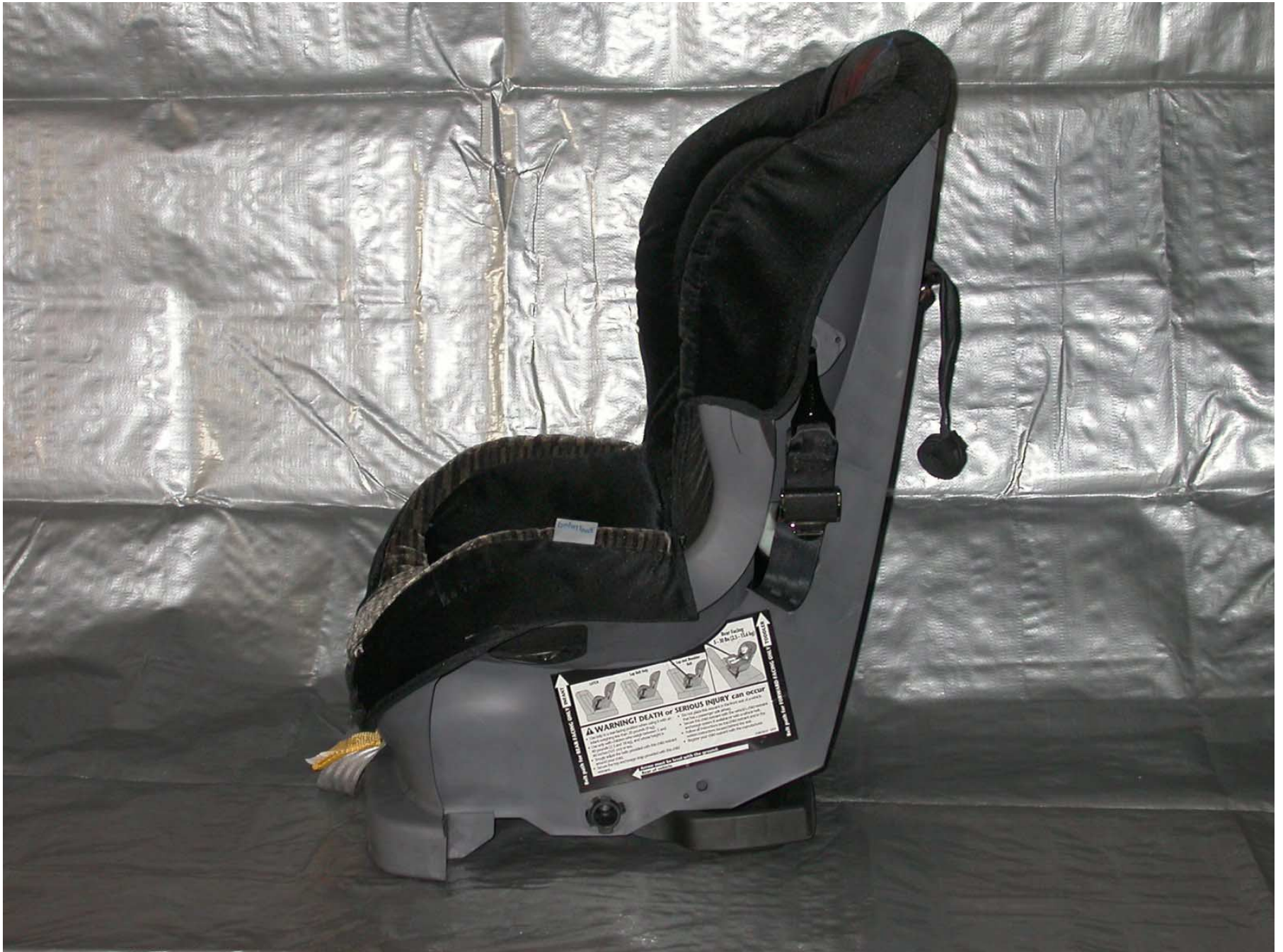
Figure F2-7: Post-Test Left Side View of Position 3 CRS (With Smoke Damage)
