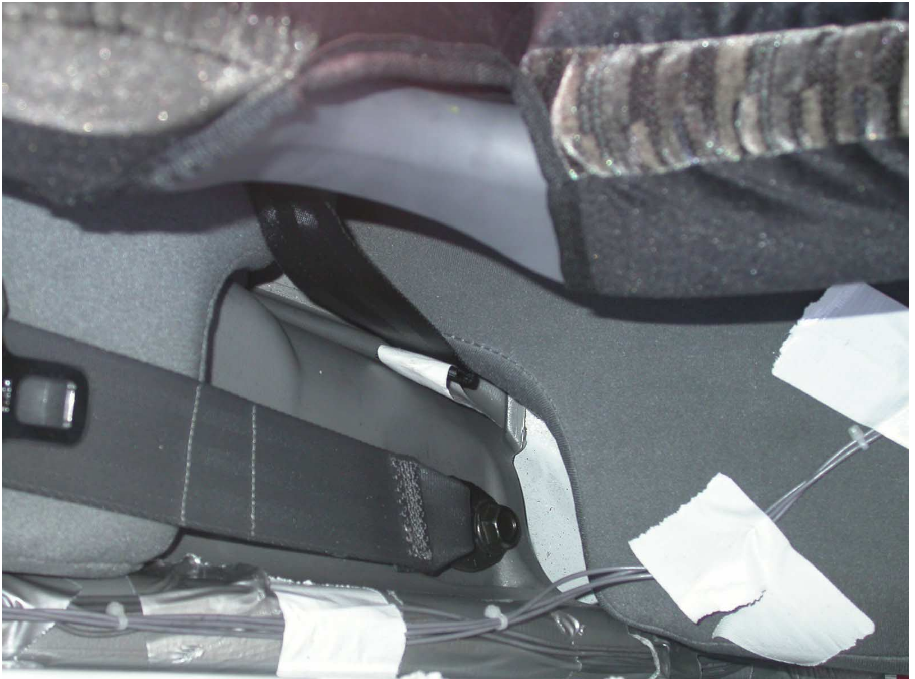
Figure F2-17: Post-Test Rear Seat Cushion Movement (Right Side View)
