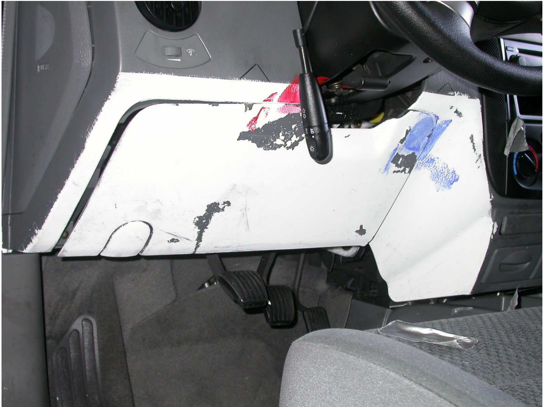
Figure A-39: Post-Test Driver Side Knee Bolster
