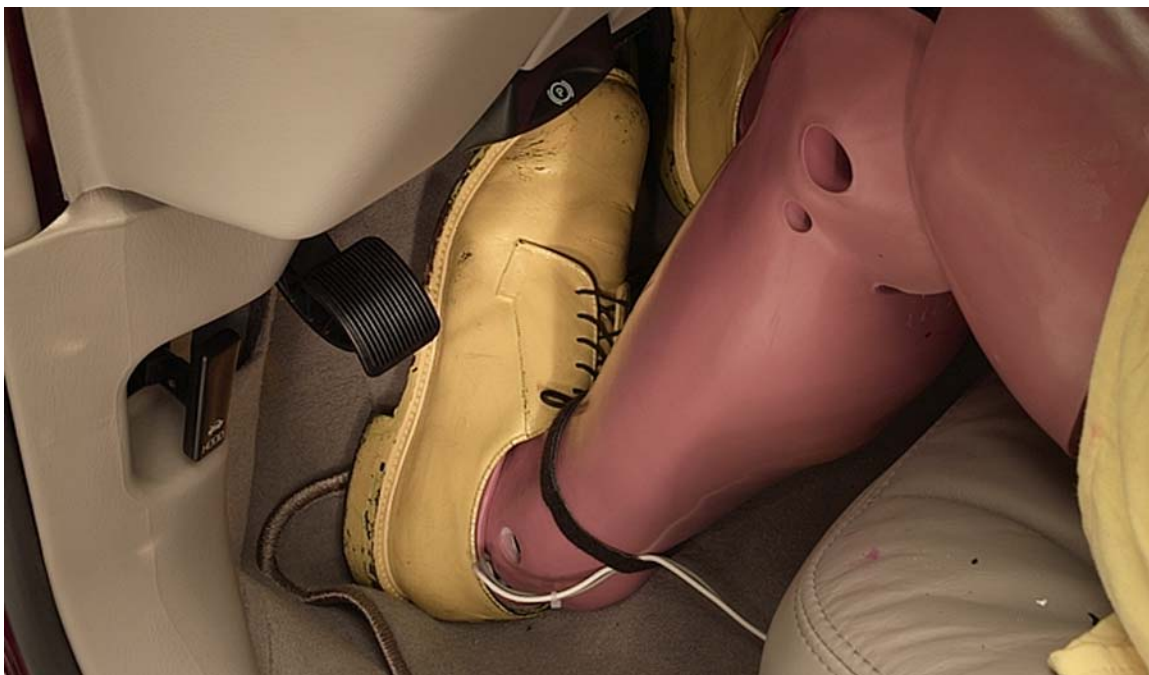
Figure 6 Dummy Feet Positions, Postcrash — 2003 Lincoln Town Car
