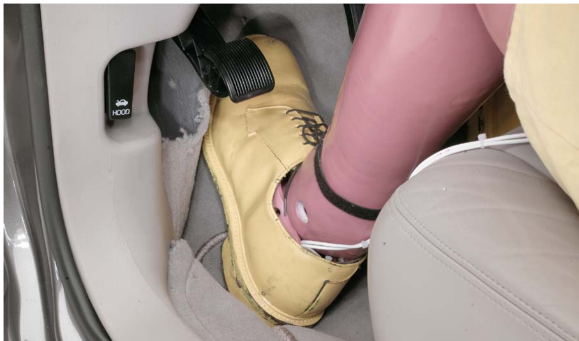
Figure 6 Dummy Feet Positions, Postcrash — 2003 Lincoln Town Car
