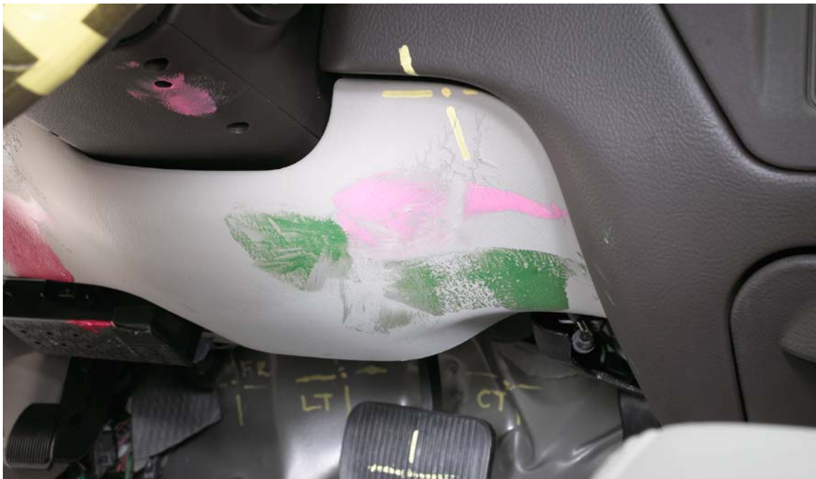
Figure 5 Dummy Right Knee/Shin Contacts, Postcrash — 2003 Lincoln Town Car
