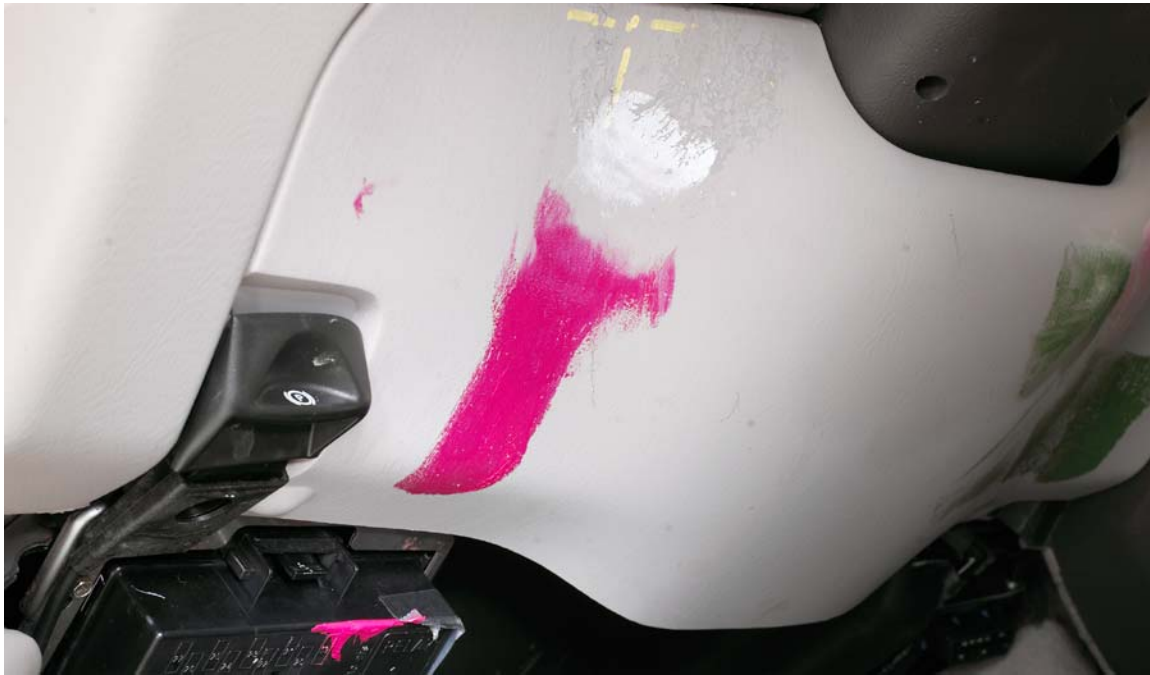
Figure 4 Dummy Left Knee/Shin Contacts, Postcrash — 2003 Lincoln Town Car
