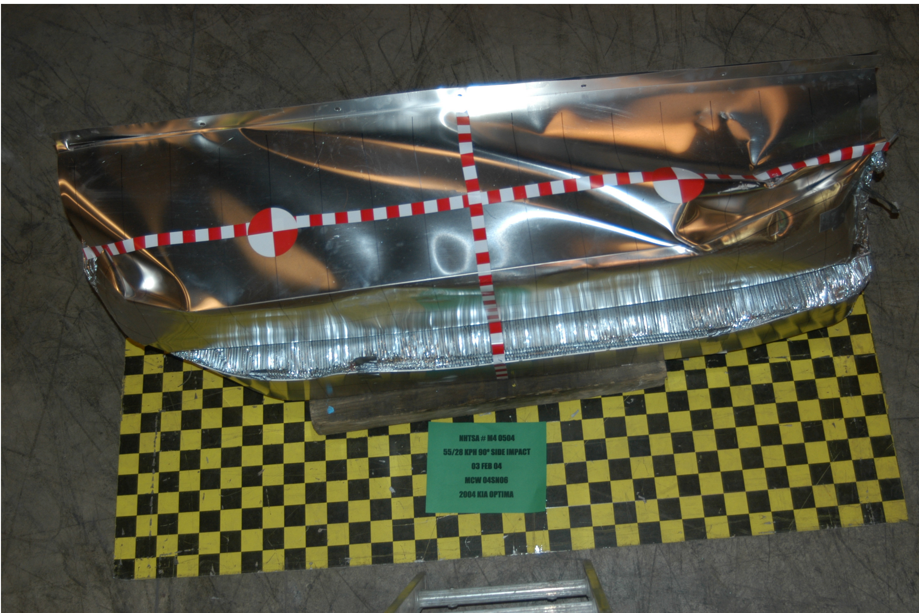
Figure A-54: POST-TEST ALUMINUM BARRIER TOP
