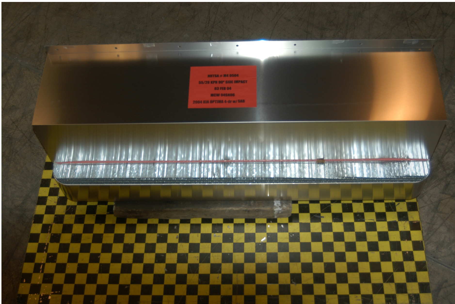
Figure A-53: PRE-TEST ALUMINUM BARRIER TOP
