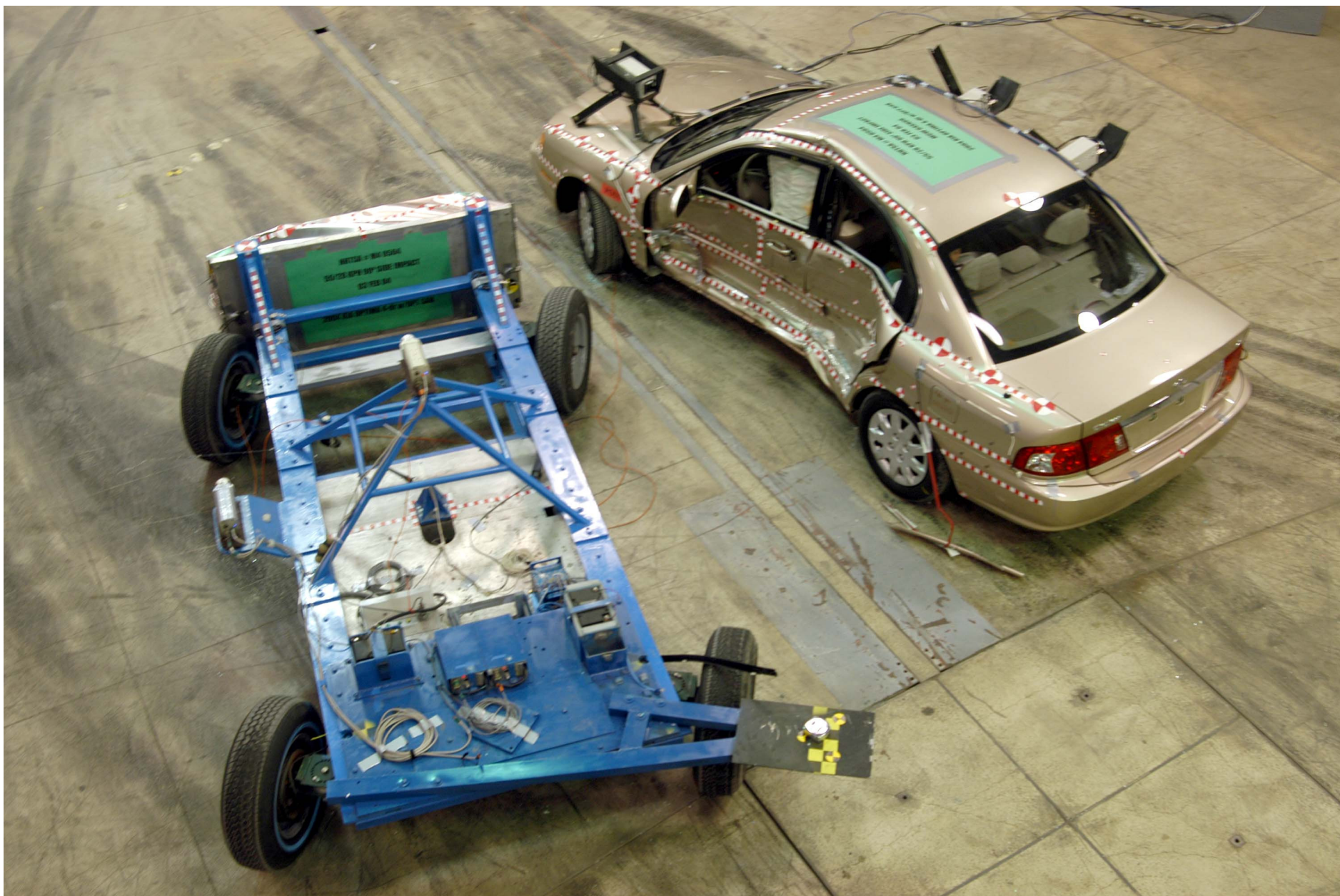
Figure A-36: POST-TEST OVERHEAD VIEW OF MDB
