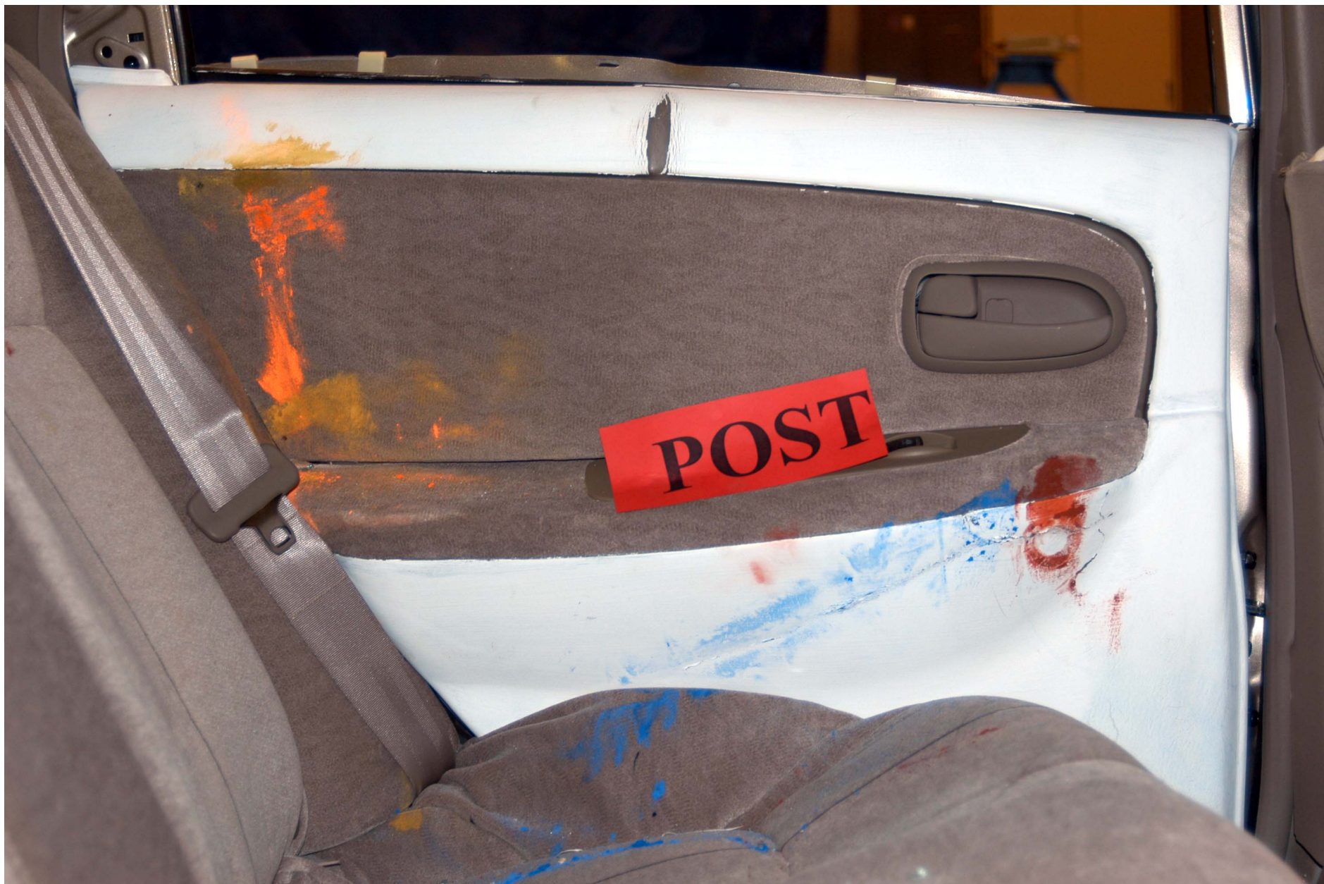
Figure A-29: POST-TEST INTERIOR OF REAR DOOR SHOWING SID H3 IMPACT LOCATIONS
