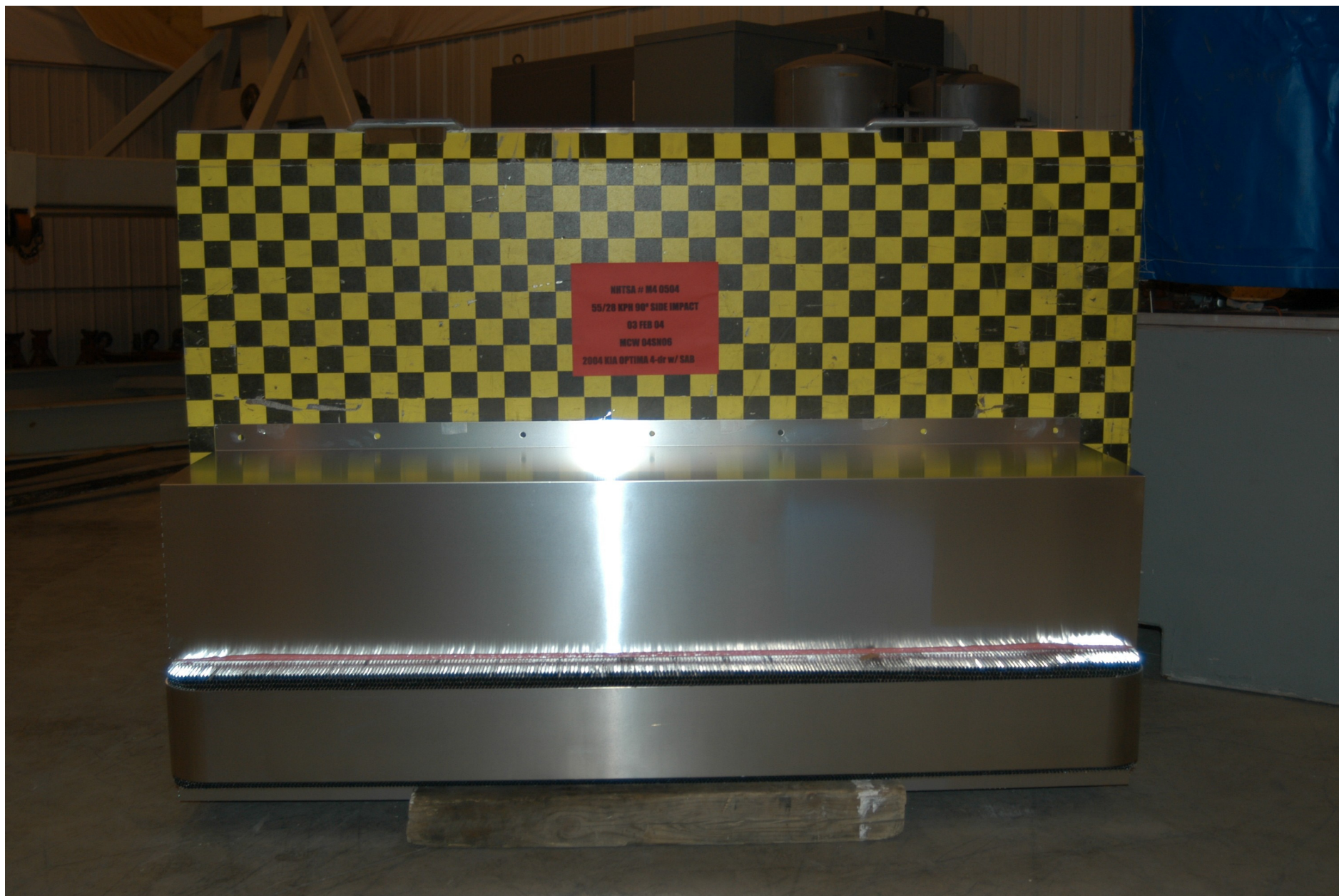
Figure A-47: PRE-TEST ALUMINUM BARRIER FRONT
