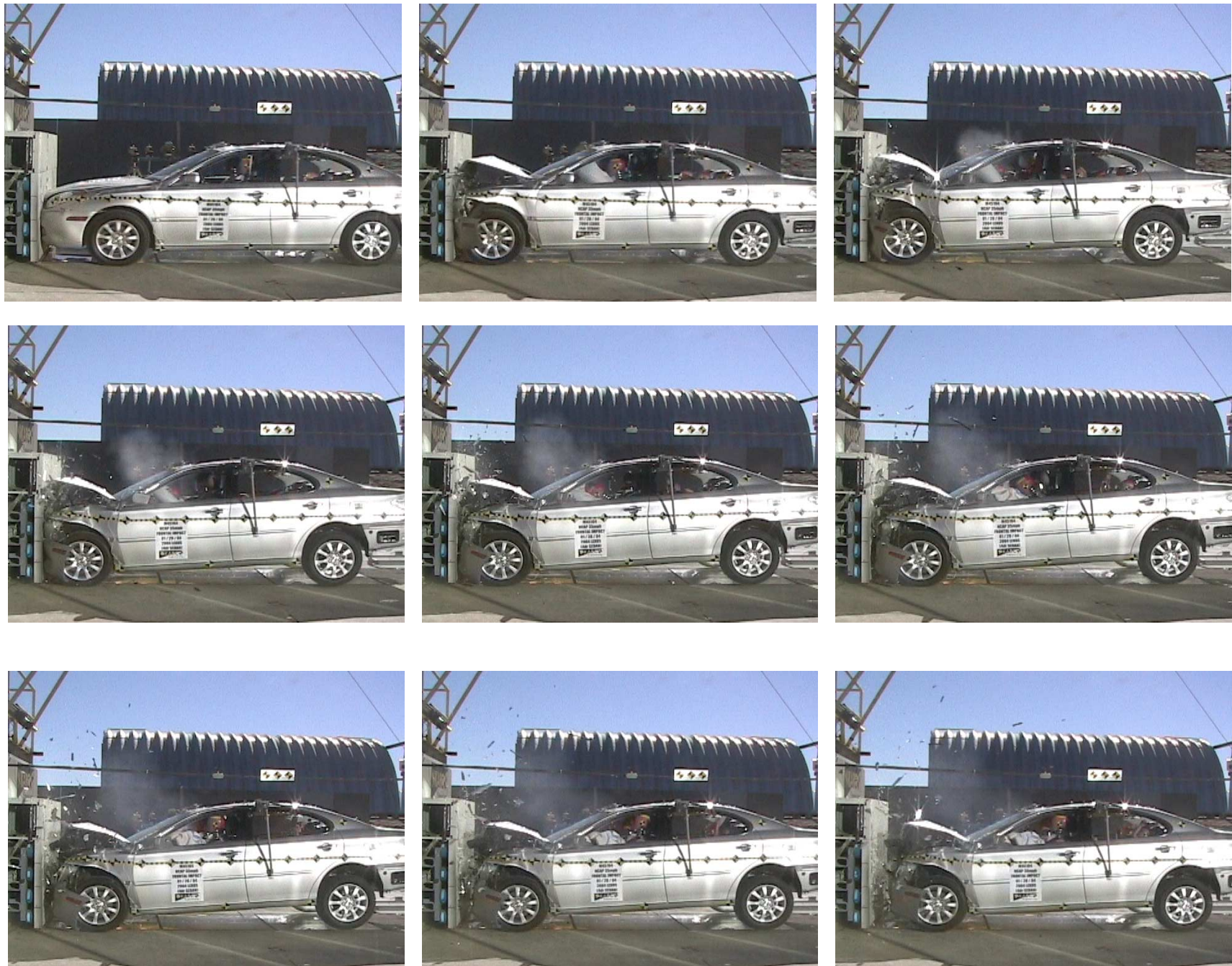
Figure A-62: Action Sequence During Impact (~33 msec. Between photos)
