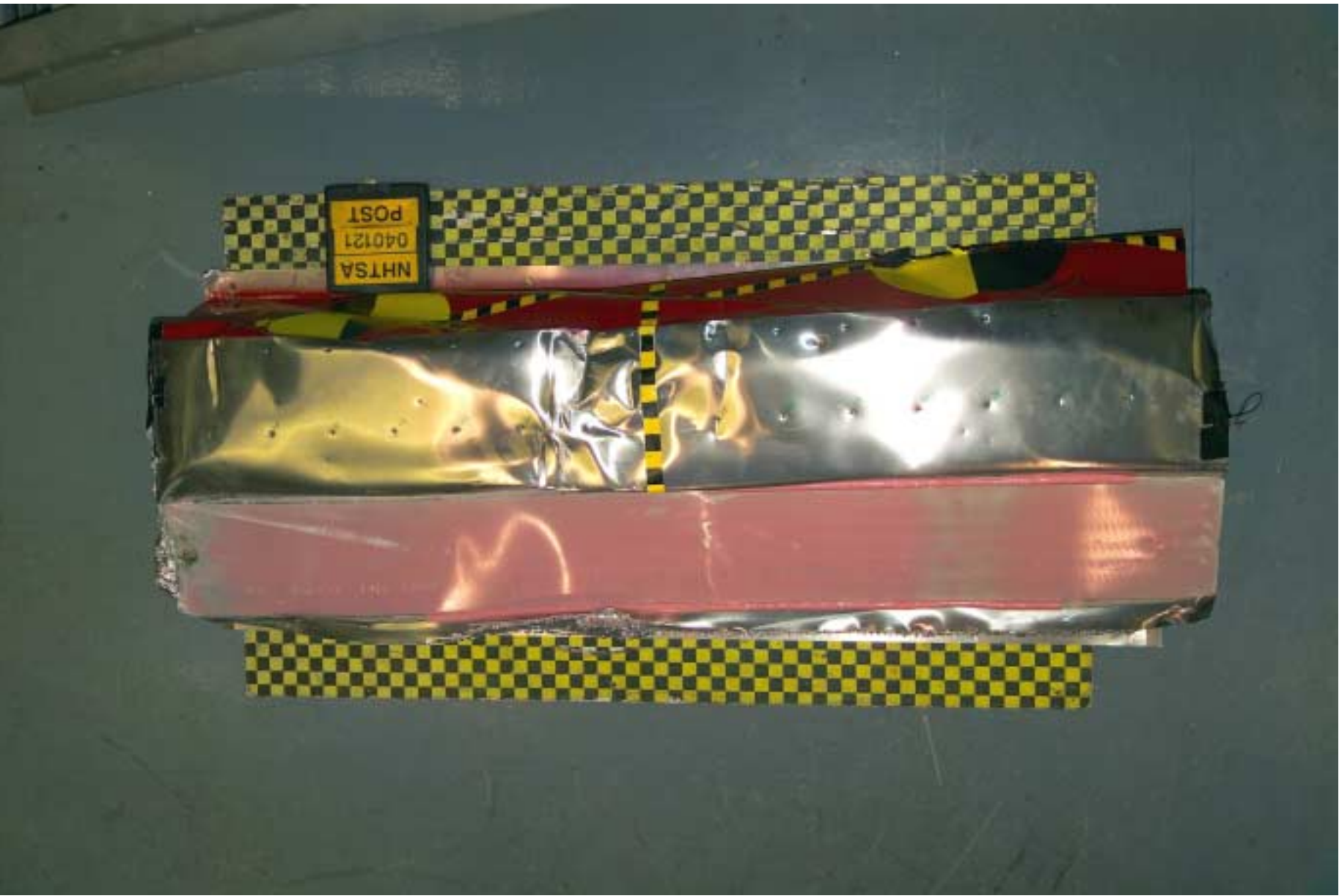
Figure A-9 Post-Test Frontal View of Impactor Face
