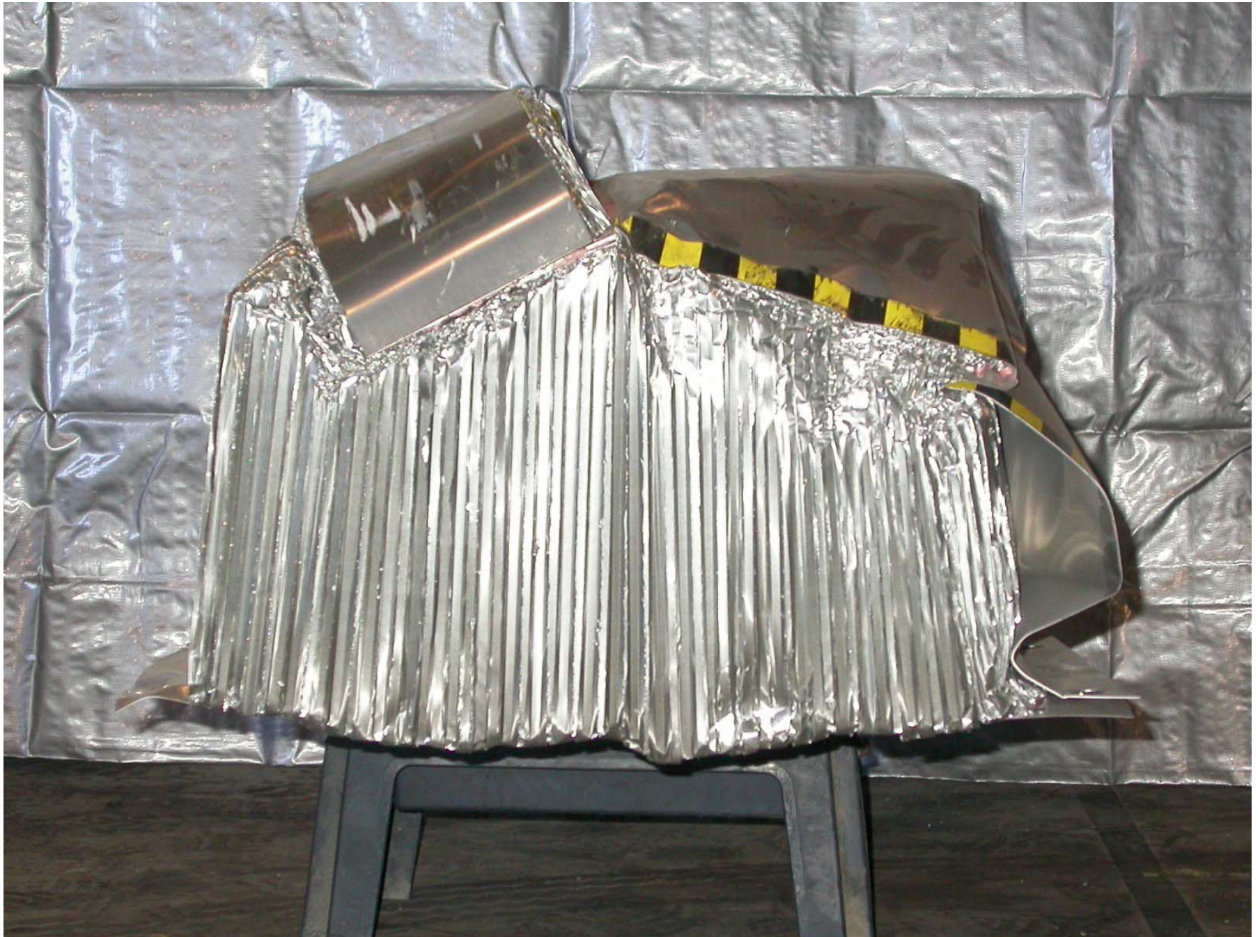
Figure A-60: Left Side View of Deformable Barrier, Post-Test
