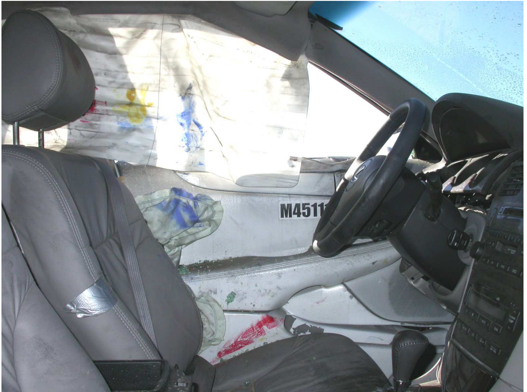
Figure A-43: Driver Dummy Contact Points Inside View, Post-Test (Vehicle Moved)
