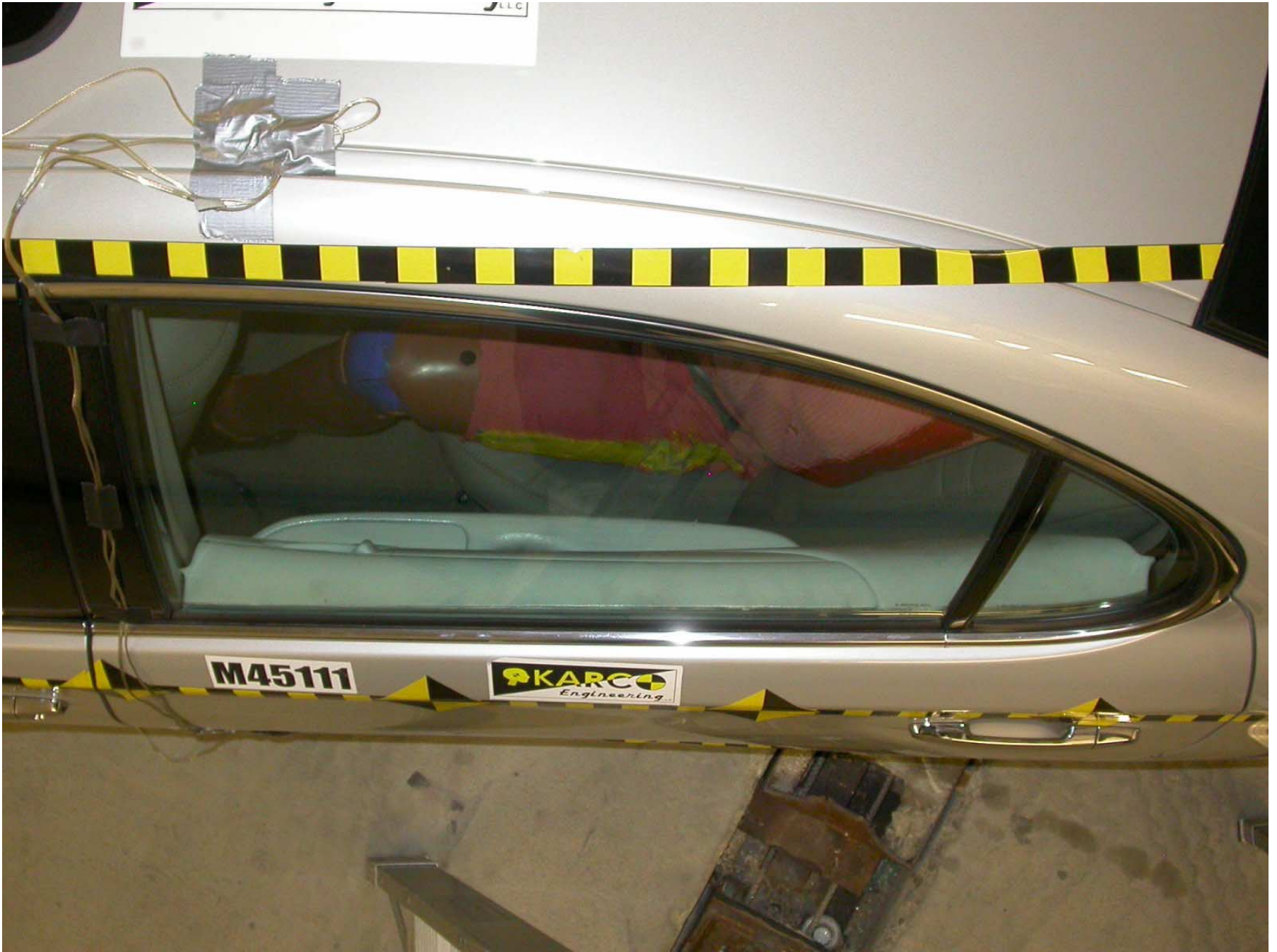
Figure A-47: Passenger Dummy Clearance, Pre-Test
