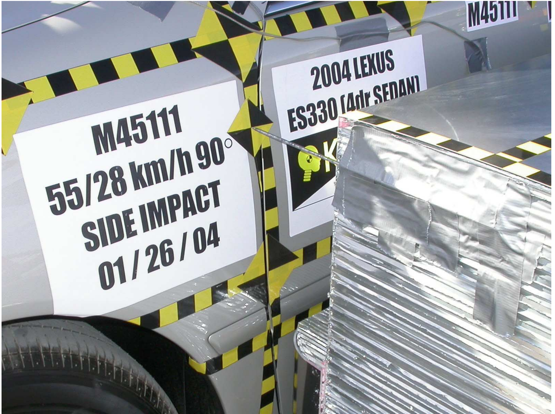
Figure A-25: Impact Point Target Set-up, Pre-Test
