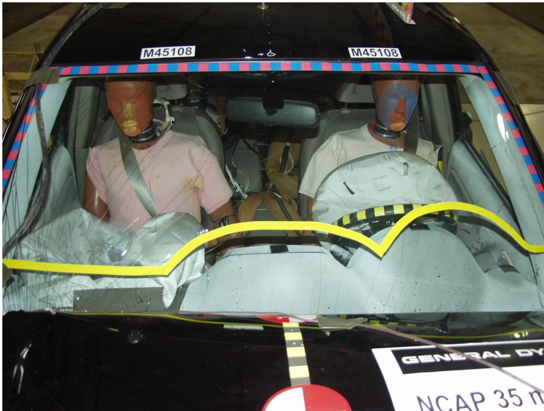
Figure A-19 POST-TEST WINDSHIELDVIEW
