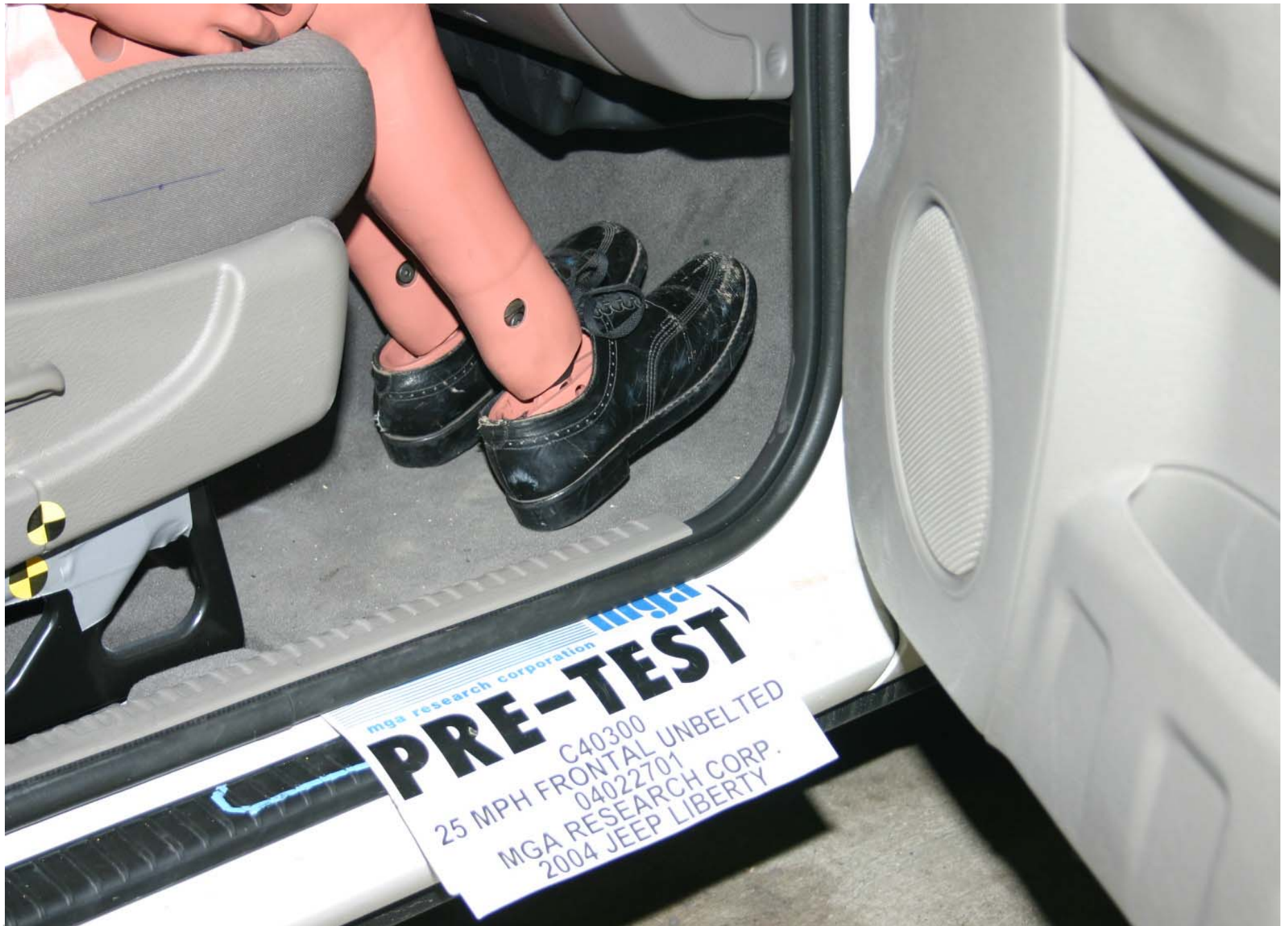
Pre-Test Passenger Dummy Feet Position
