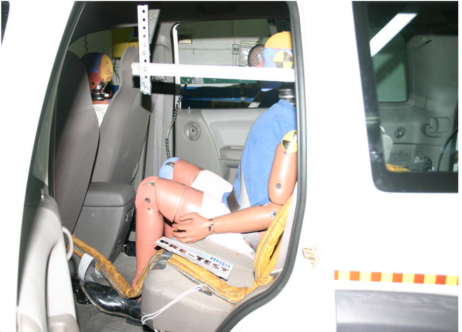
Pre-Test Rear Pass. Dummy Position Left Side View (Door Open)
