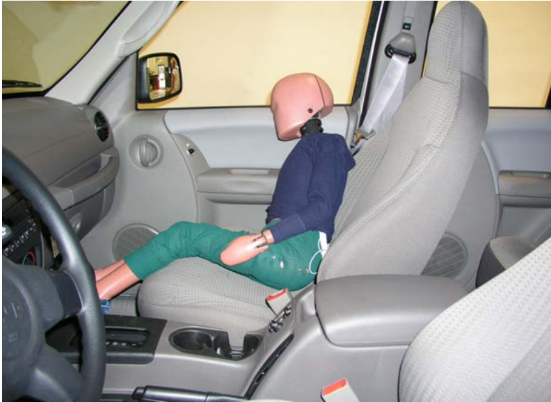
6-Year-Old Unbelted, Forward Seat Track, Position 4, Side View
