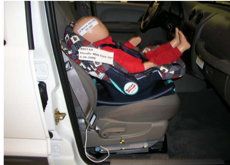
Britax Handle With Care Fwd Facing Unbelted, Middle Seat Track, Handle Down
