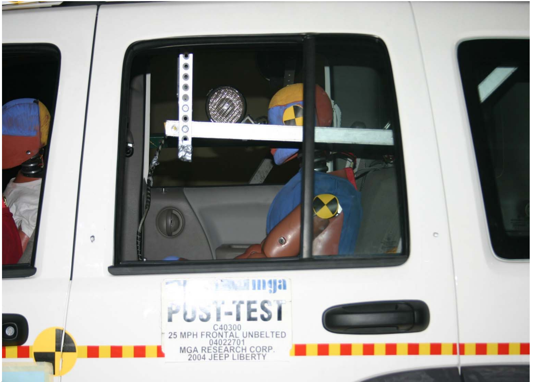
Post-Test Rear Passenger Dummy Position Left Side View
