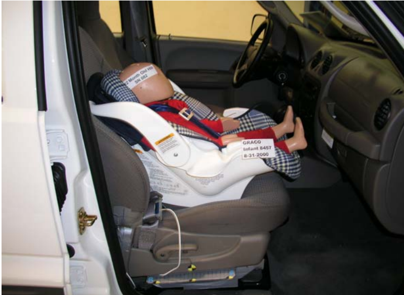
Graco Infant W/O Base Fwd Facing Unbelted, Middle Seat Track, Handle Down
