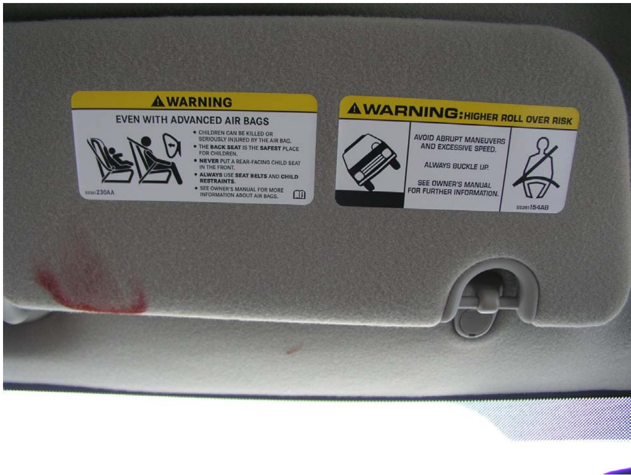
2004 Jeep Liberty MPV S.4.5.1 Air Bag Labeling Failure (Data Sheet 5 – 3.6.3)
