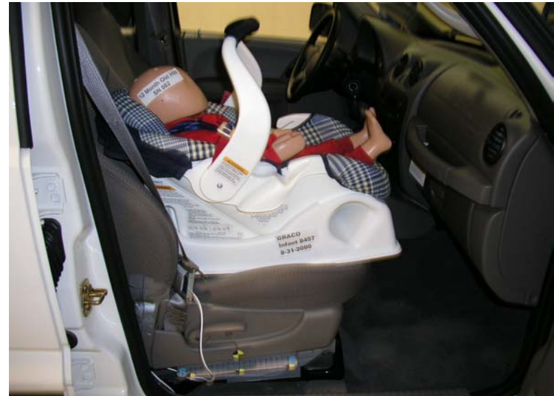
Graco Infant W/ Base Fwd Facing Unbelted, Middle Seat Track, Handle Up
