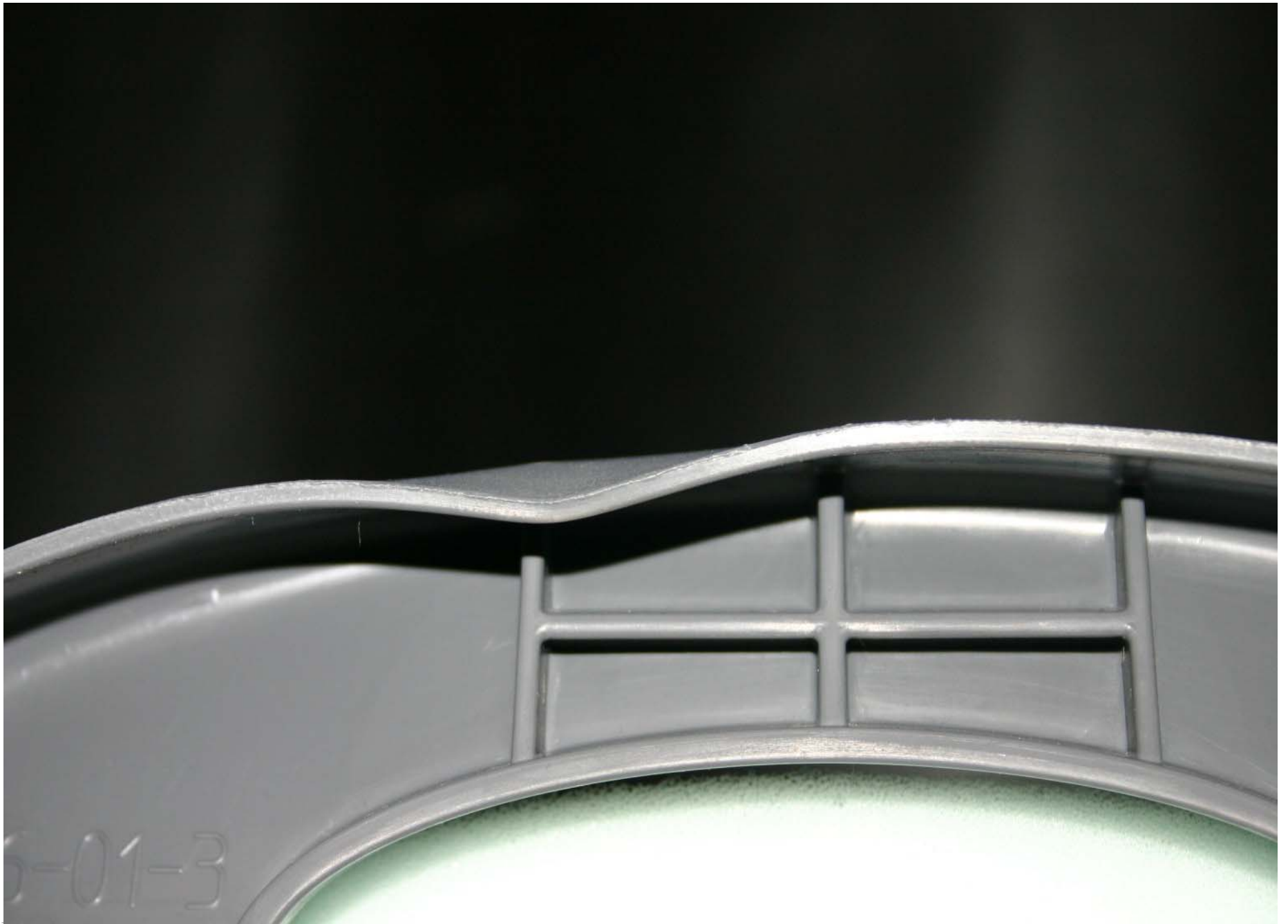
Post-Test Dent in Position 3 CRS
