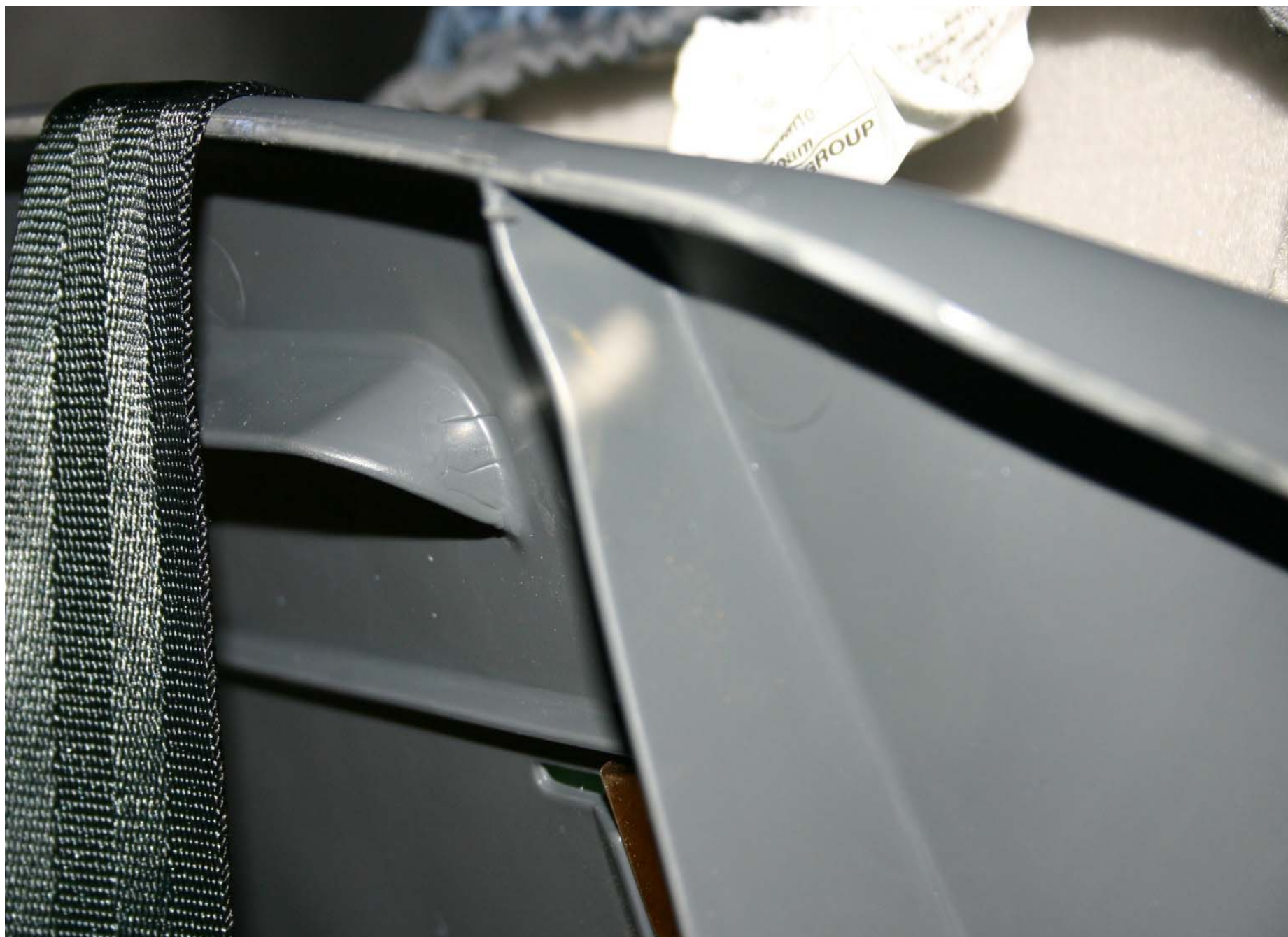
Post-Test Stress Mark/Dent in Position 4 CRS
