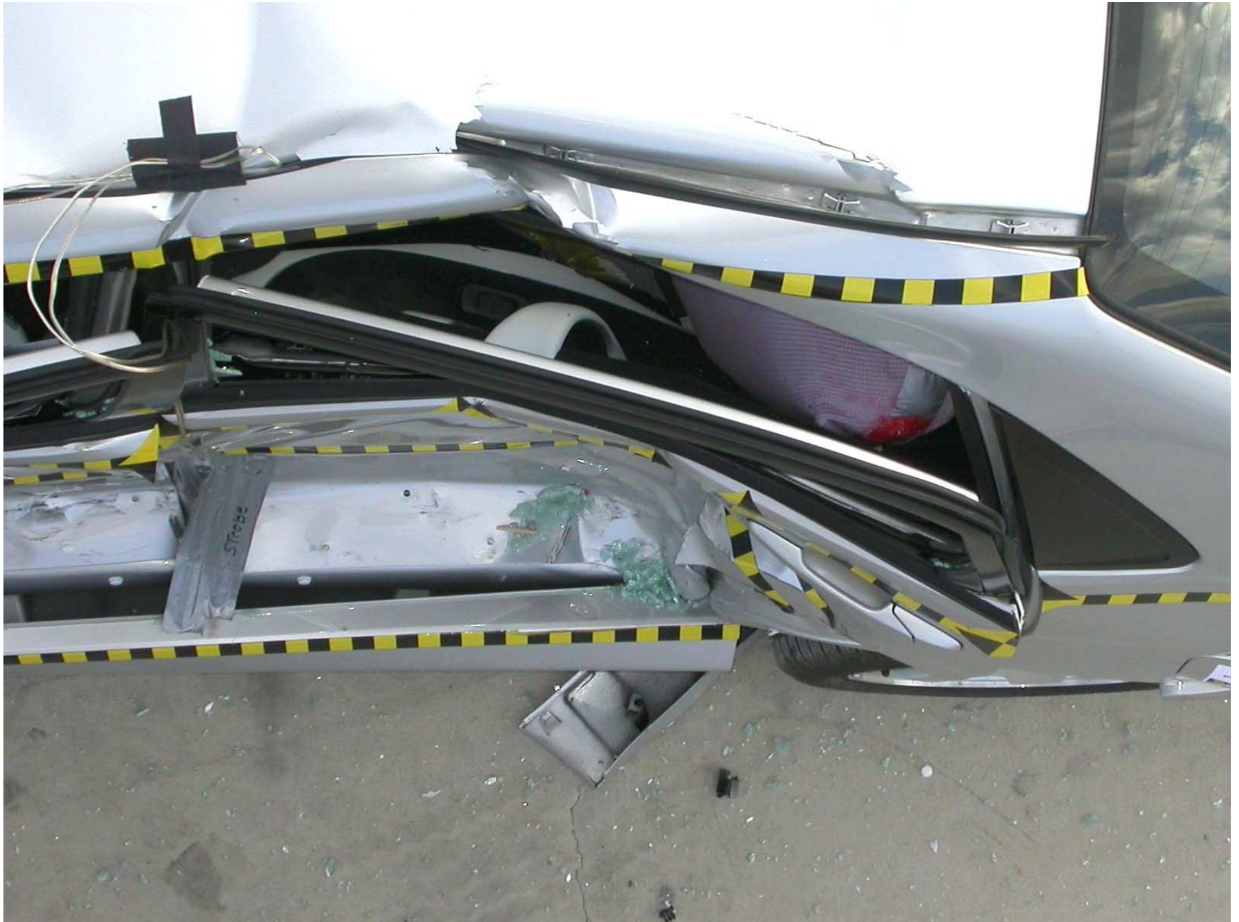
Figure A-48: Passenger Dummy Clearance, Post-Test
