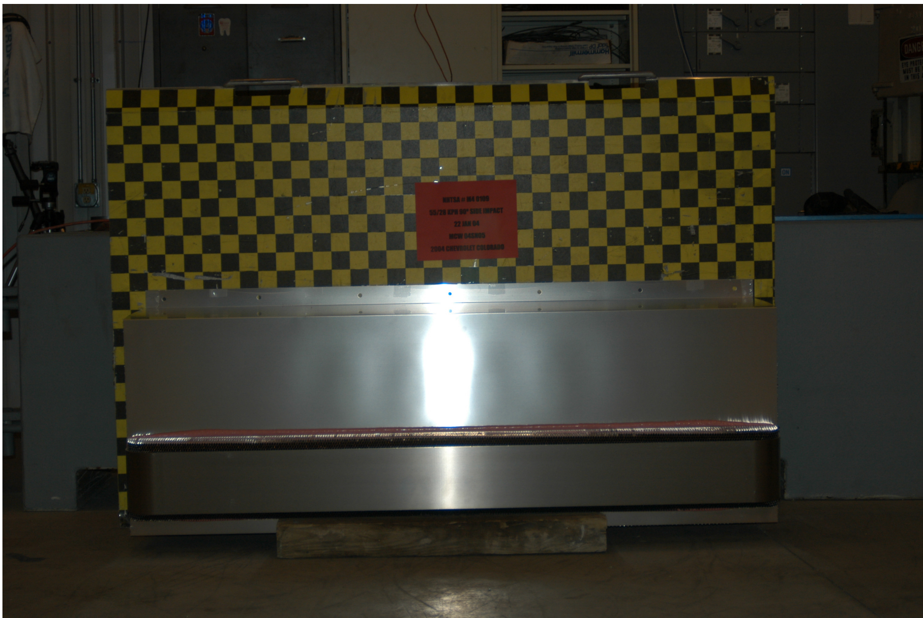
Figure A-47: PRE-TEST ALUMINUM BARRIER FRONT
