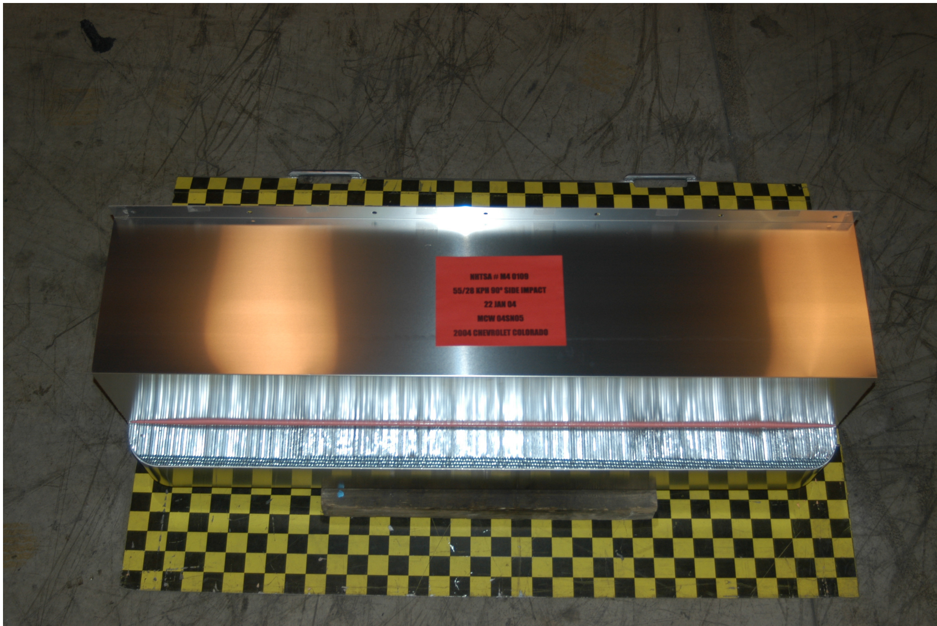
Figure A-53: PRE-TEST ALUMINUM BARRIER TOP
