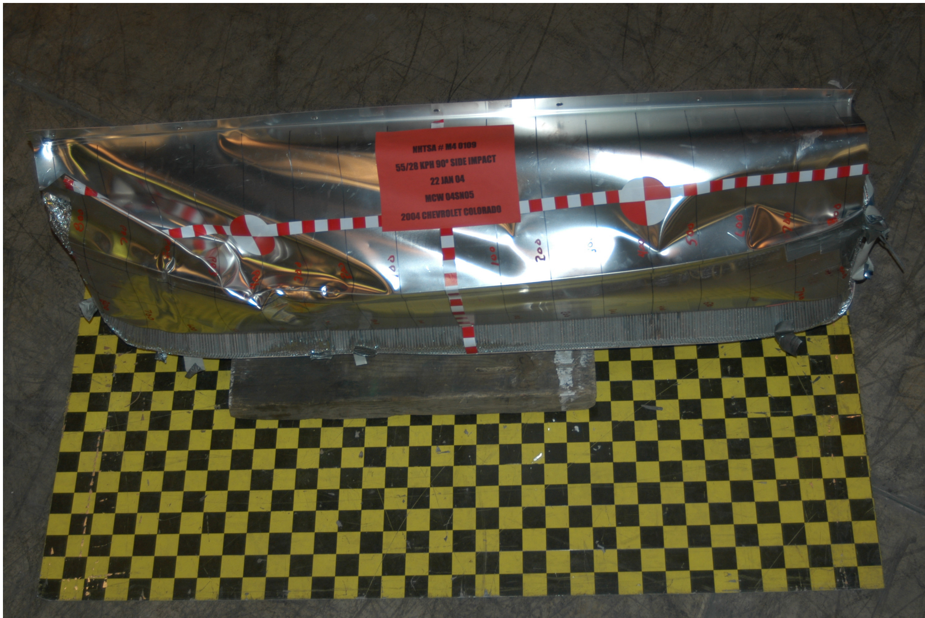
Figure A-54: POST-TEST ALUMINUM BARRIER TOP
