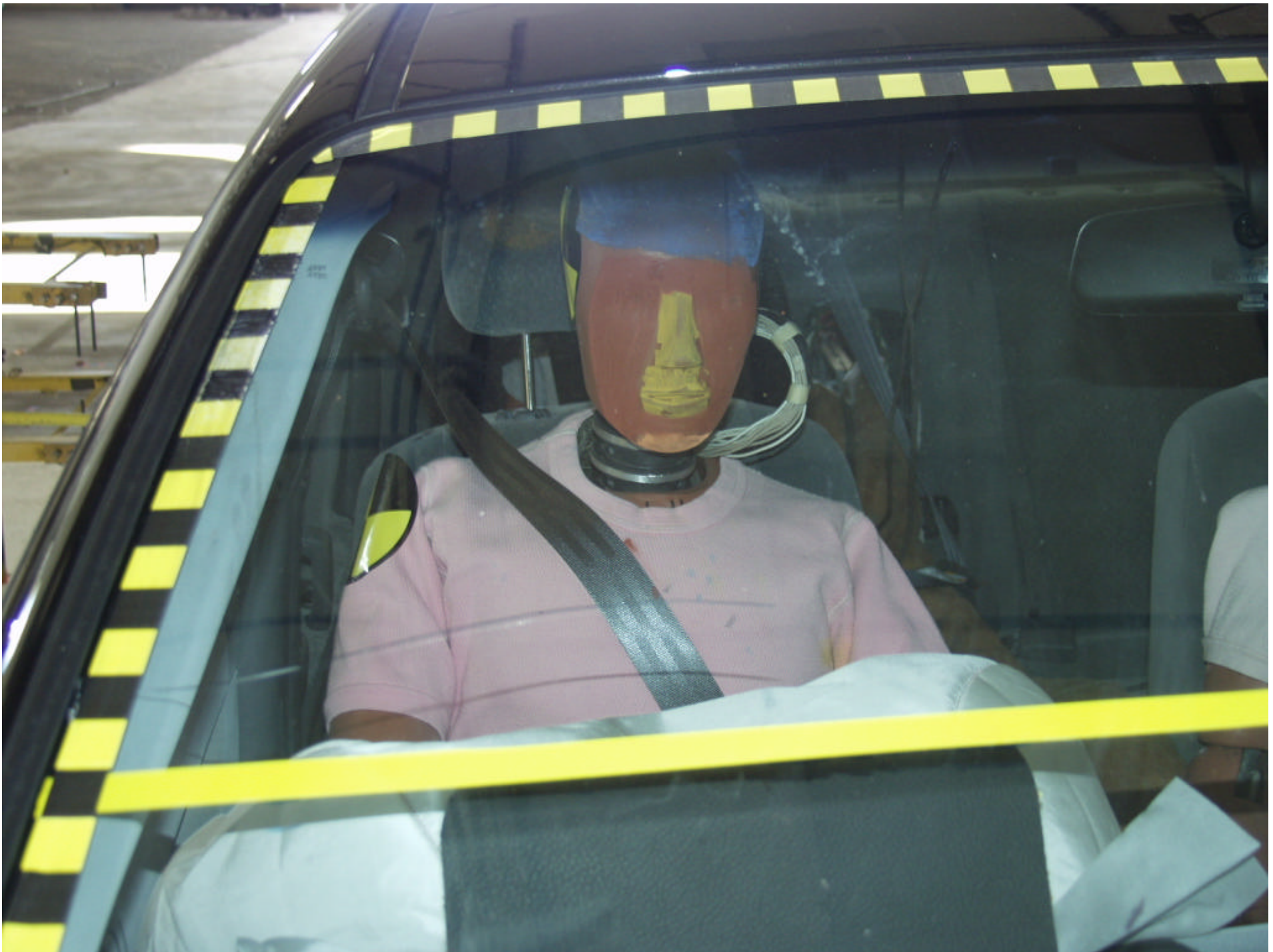
Figure A-45 POST-TEST PASSENGER HEAD LOCATION
