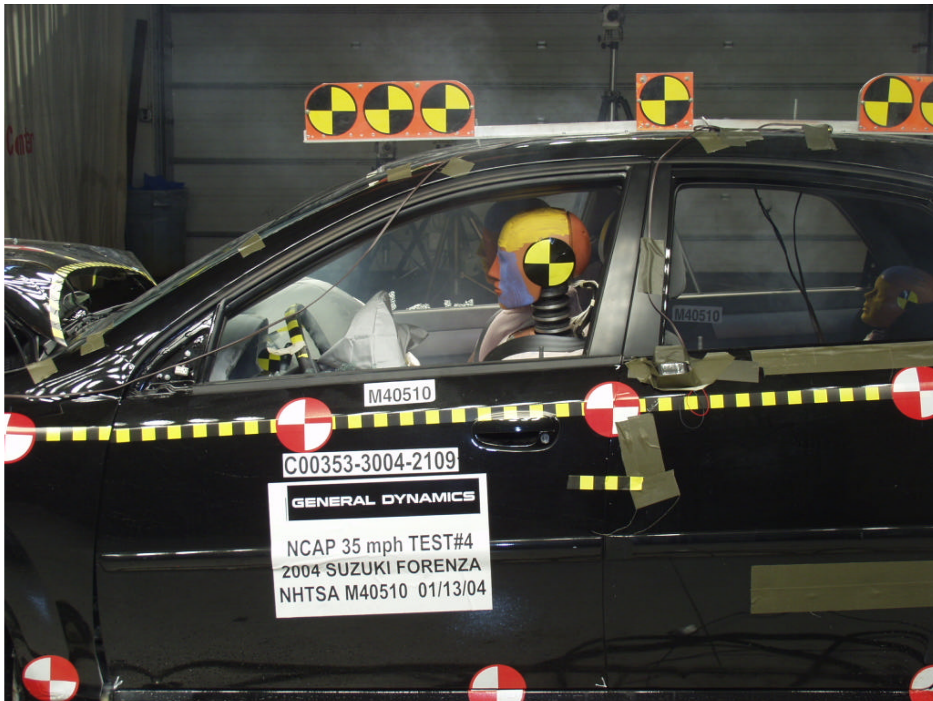
Figure A-33 POST-TEST DRIVER POSITION VIEW
