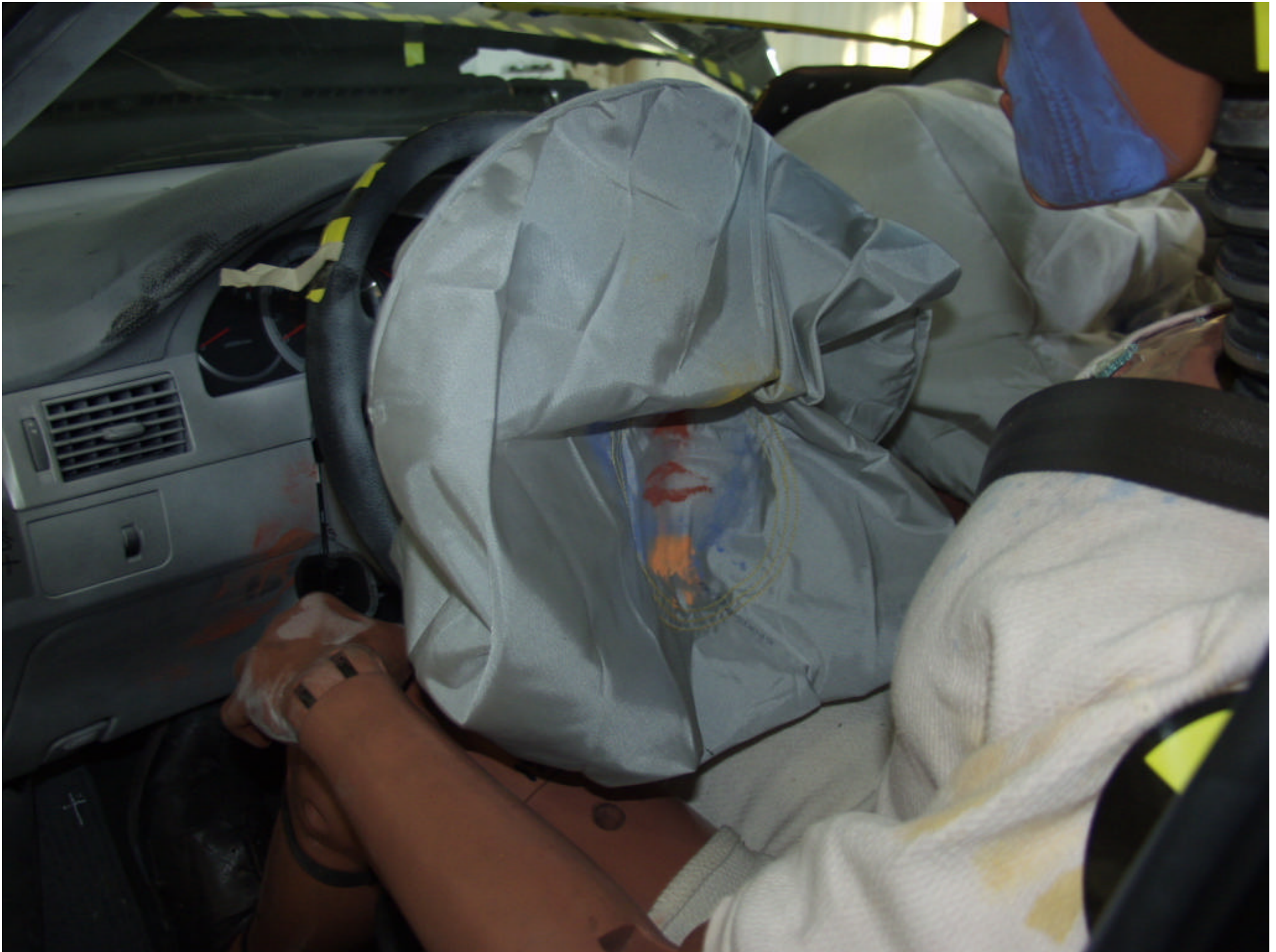
Figure A-43 POST-TEST DRIVER CONTACT TO AIRBAG
