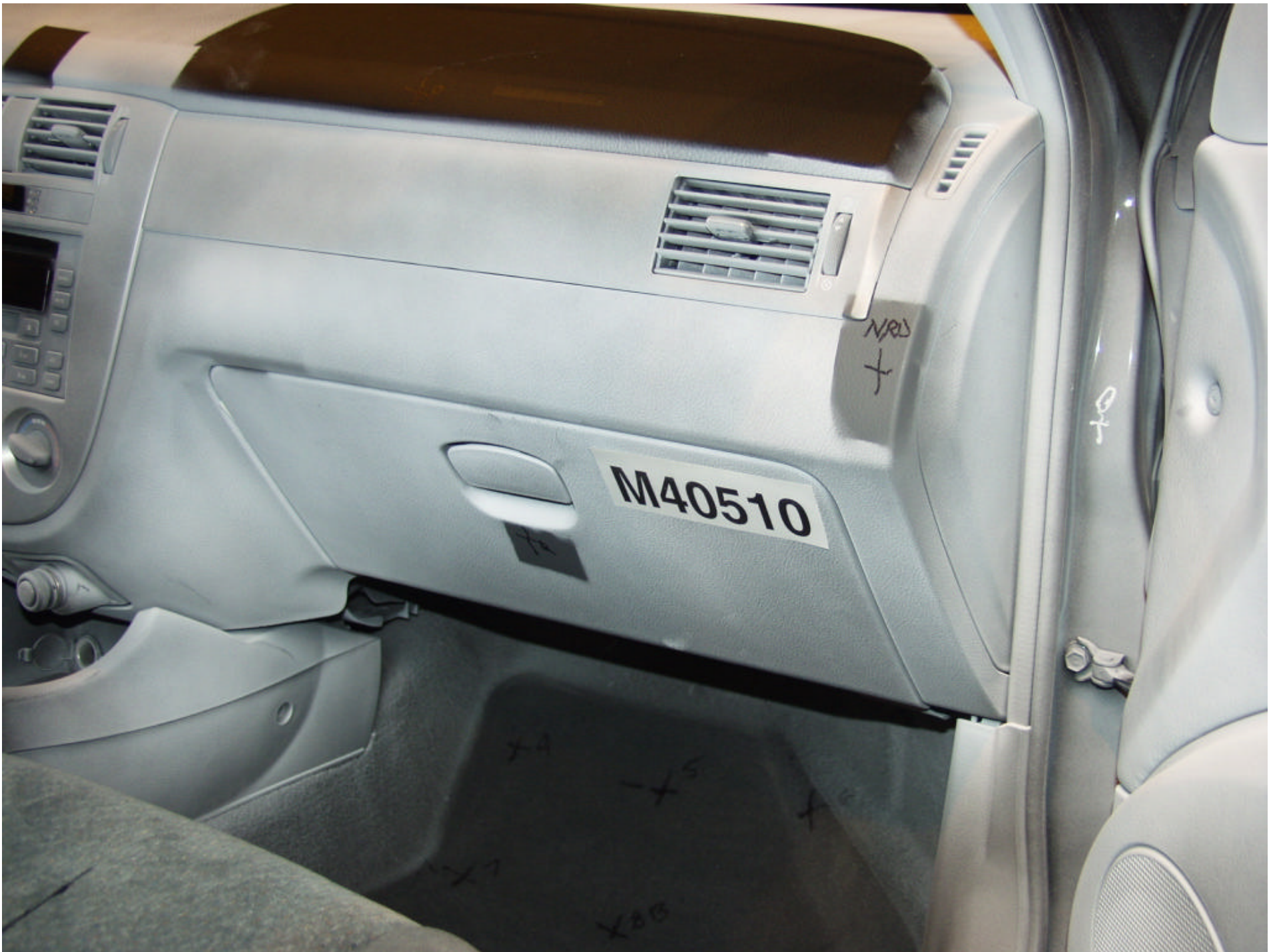
Figure A-52 PRE-TEST PASSENGER KNEE BOLSTER VIEW
