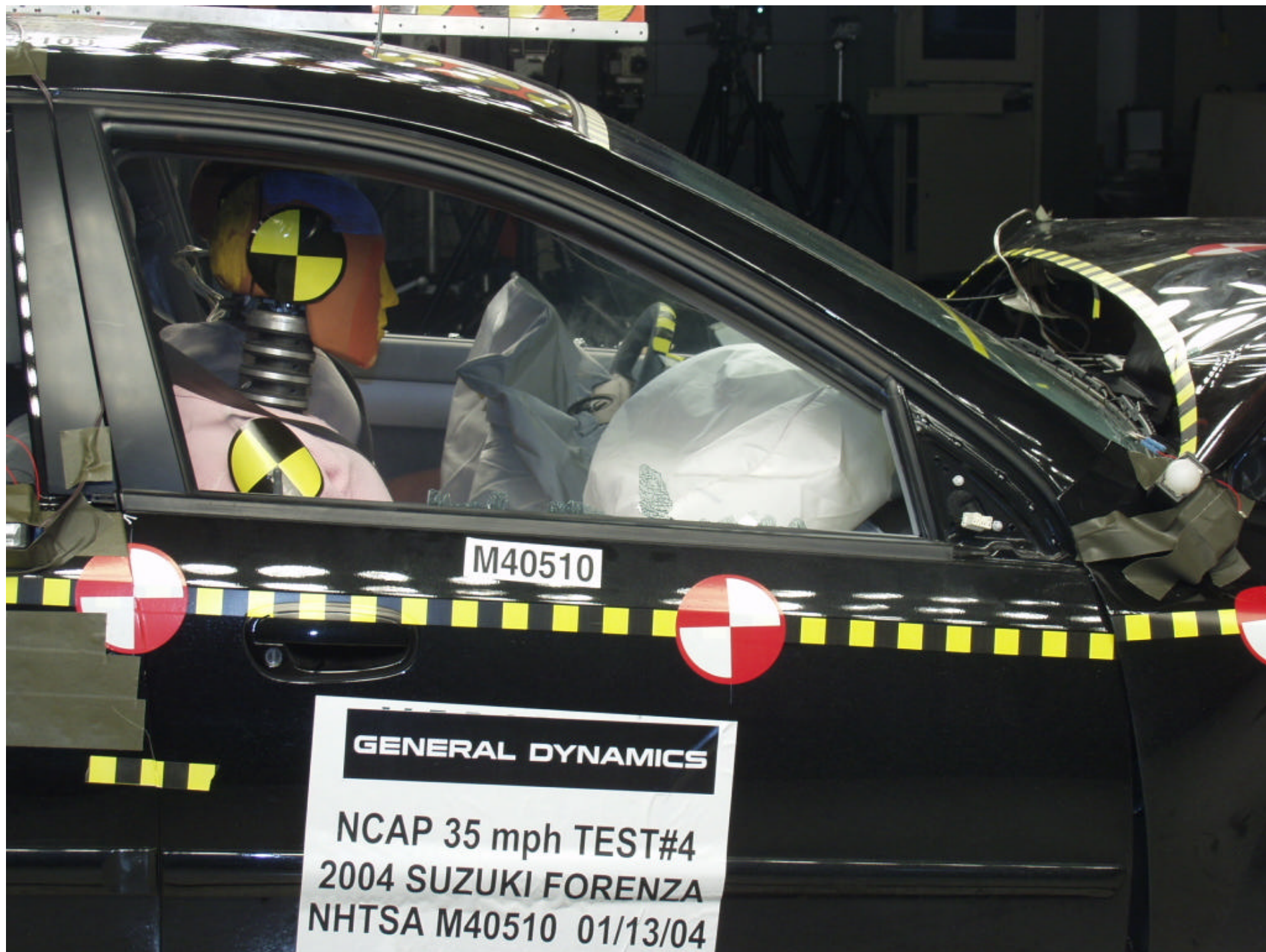
Figure A-47 POST-TEST PASSENGER POSITION VIEW
