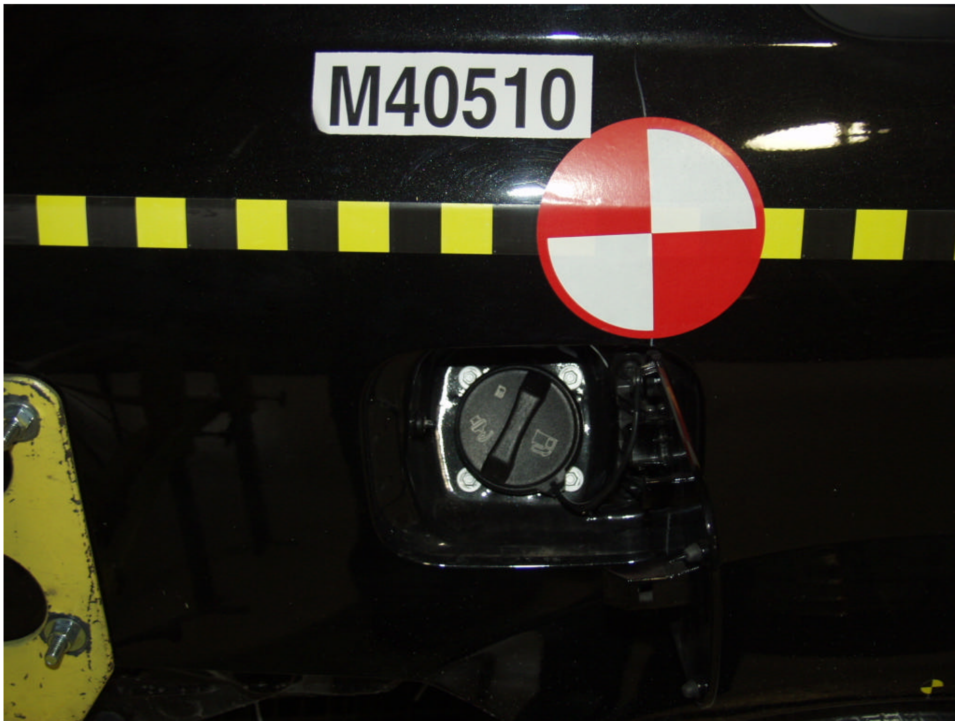
Figure A-22 PRE-TEST FUEL CAP VIEW
