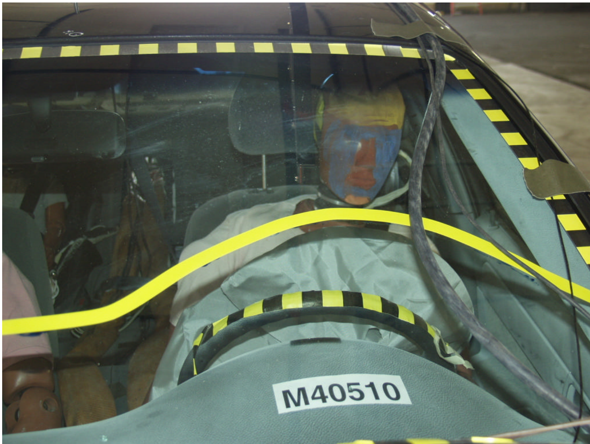
Figure A-31 POST-TEST DRIVER HEAD LOCATION
