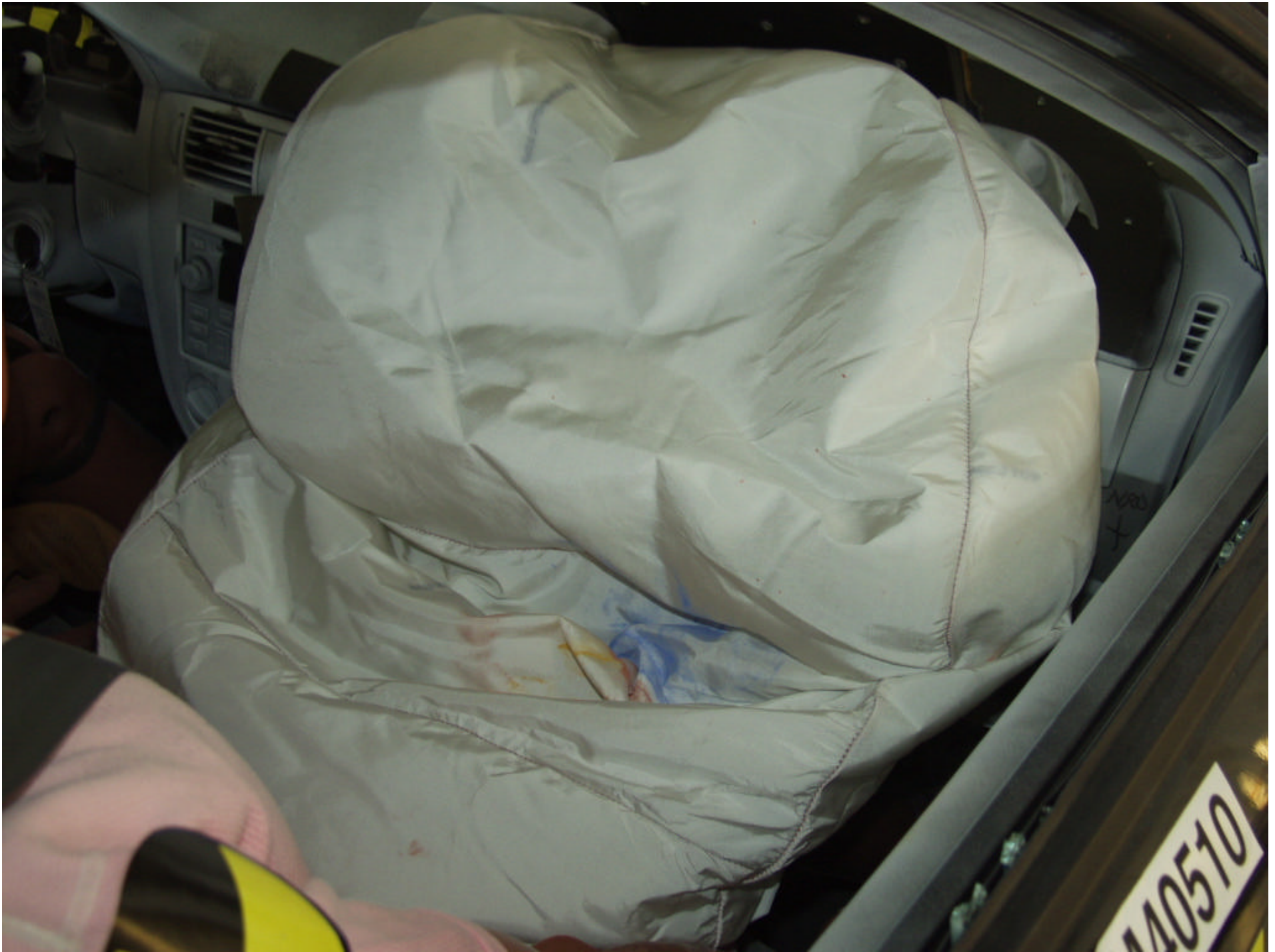
Figure A-57 POST-TEST PASSENGER CONTACT TO AIRBAG
