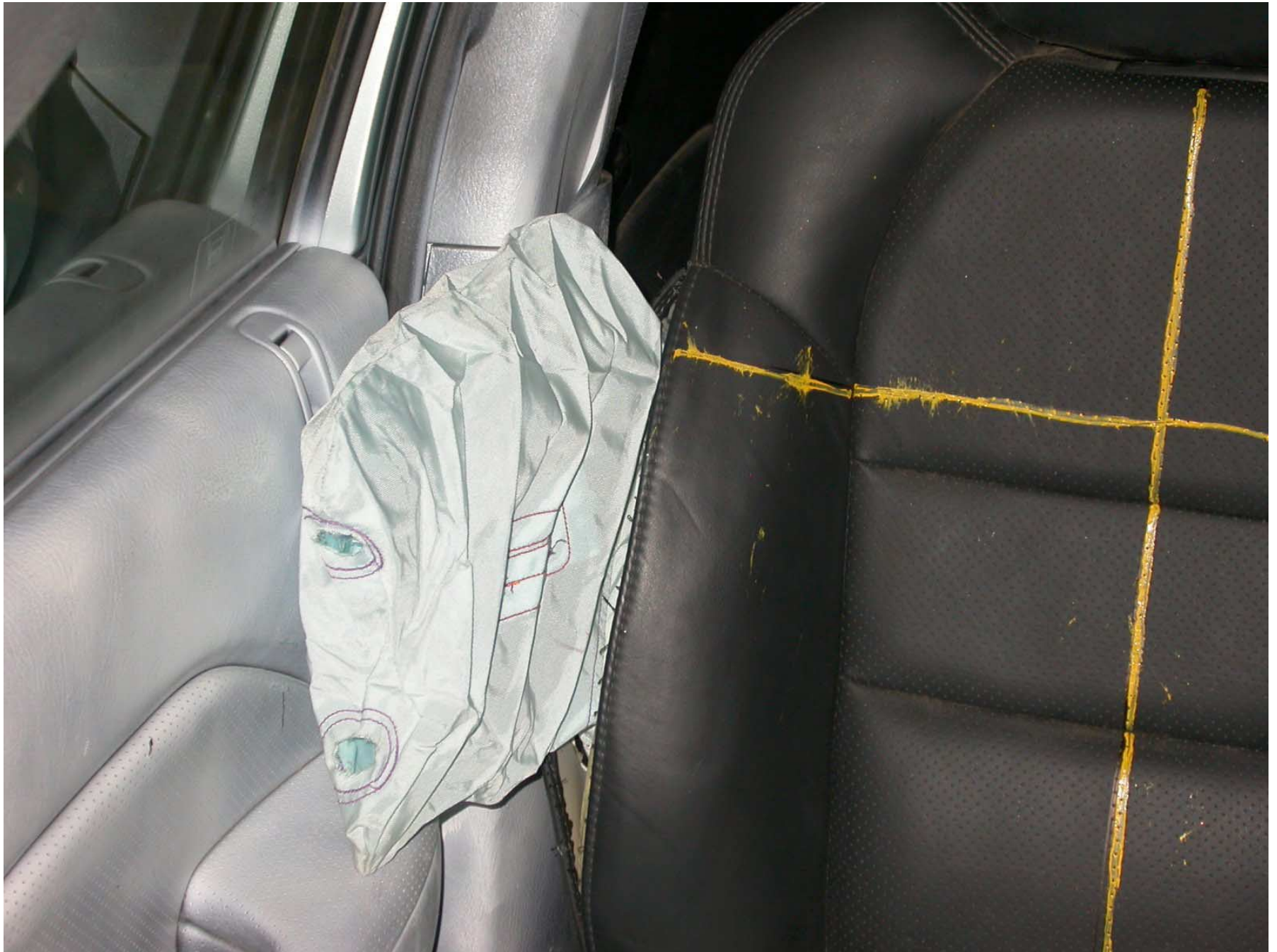
Figure A-11: Post-Test Airbag, \frac{3}{4} Front View
