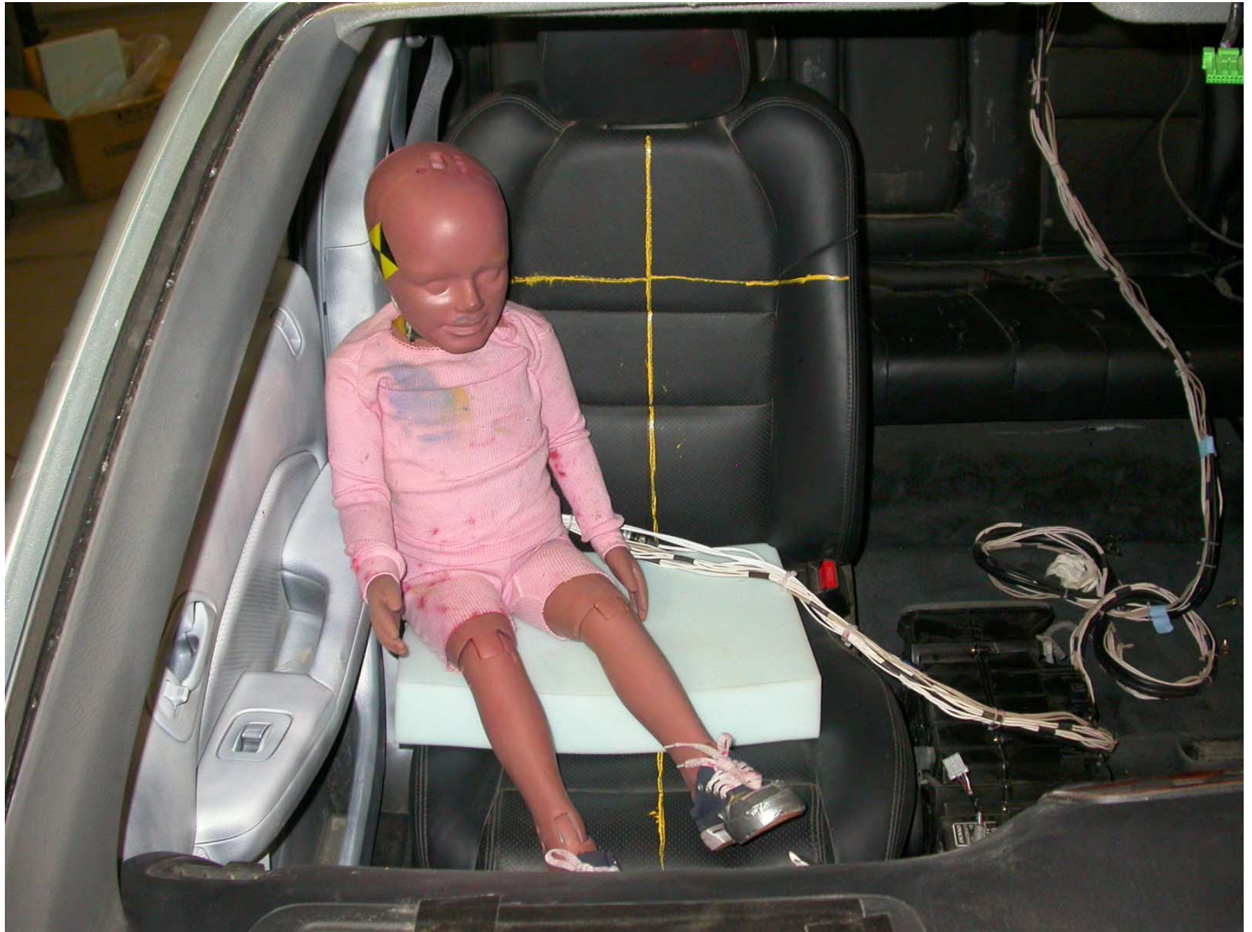
Figure A-6: Pre-Test Dummy Position, Full Front View
