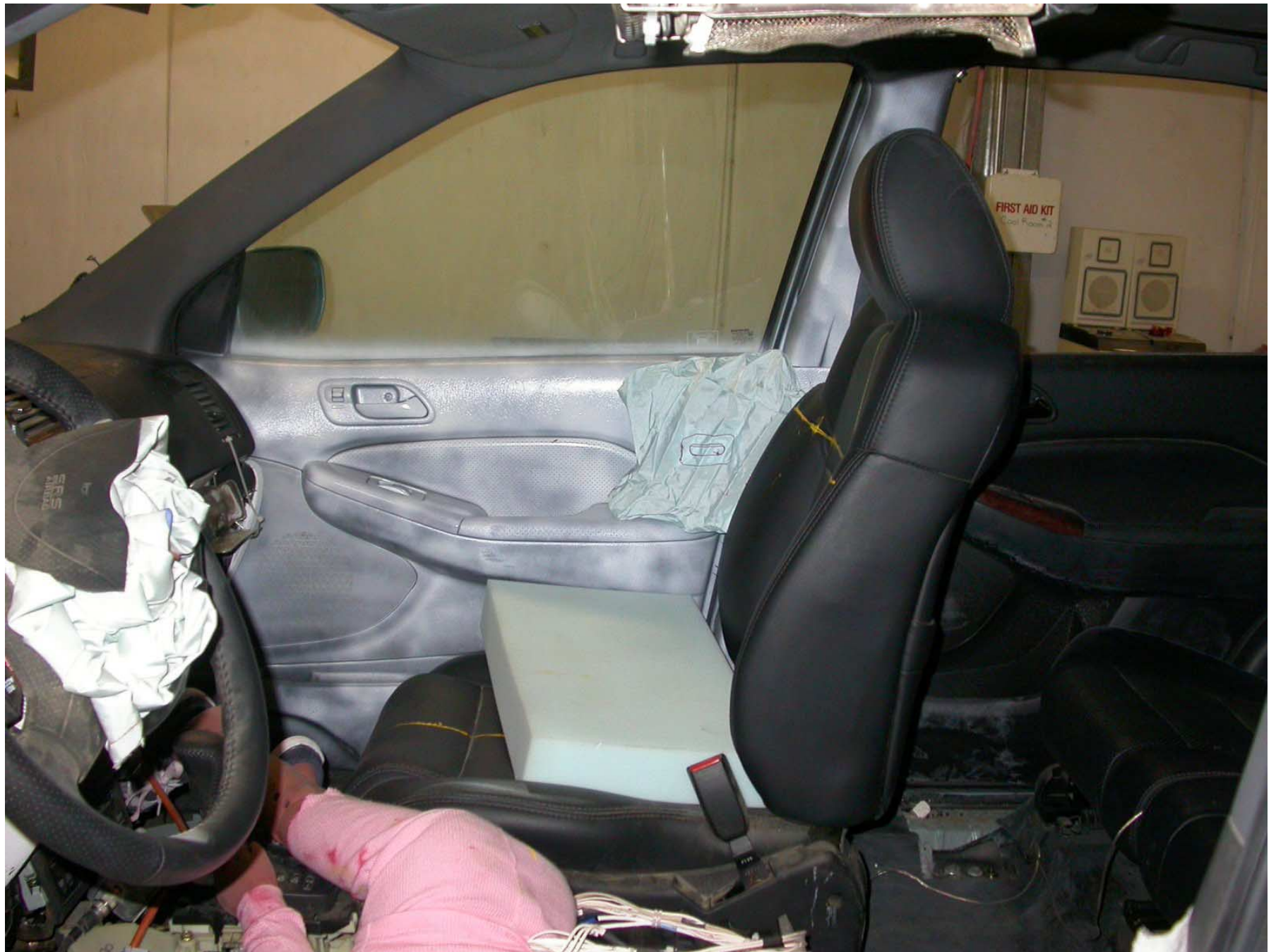
Figure A-9: Post-Test Dummy Position & Airbag, Left Side View
