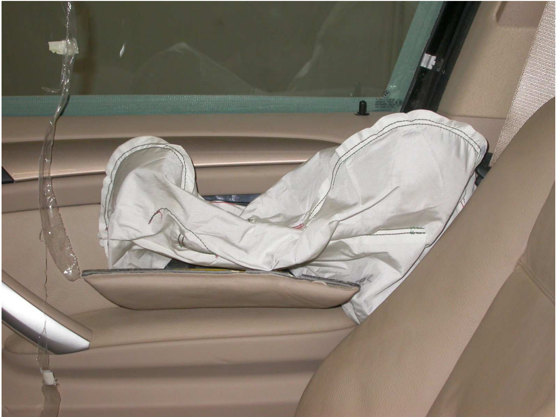
Figure A-11: Post-Test Door-Mounted Airbag, Left View
