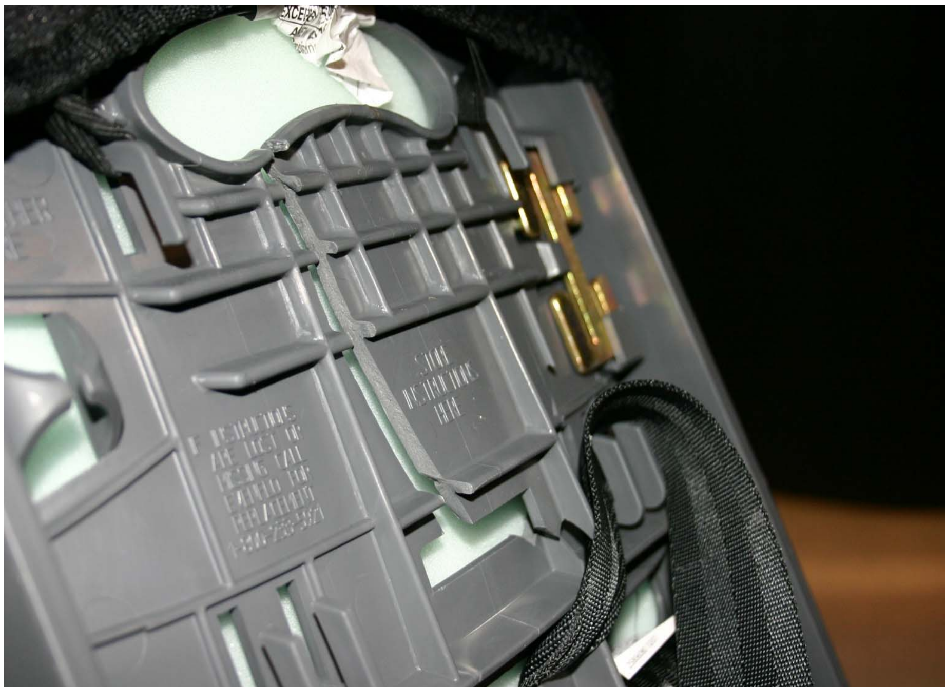
Post-Test Position 3 (Evenflo Child Seat) Left View of Cracks
