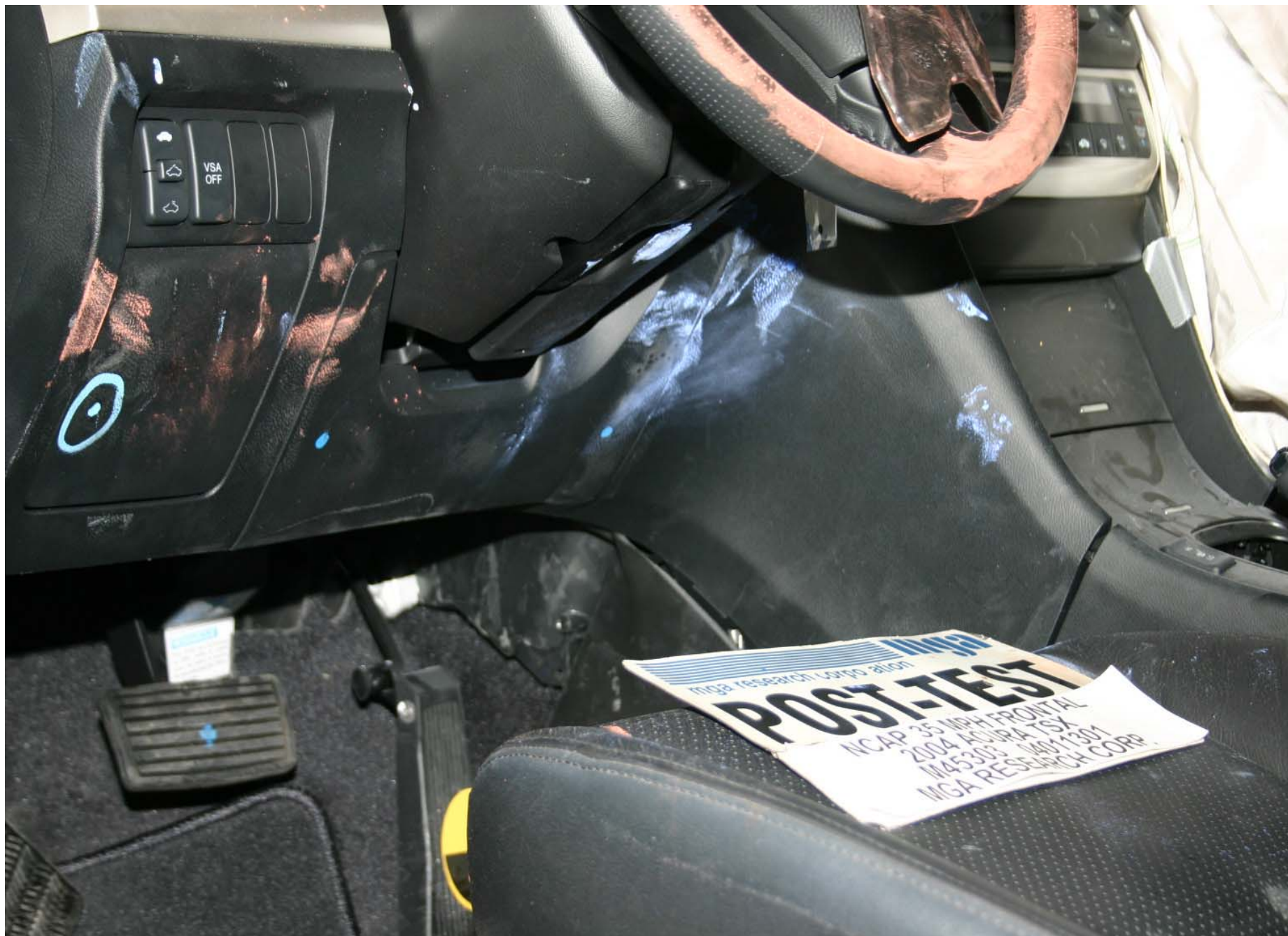
Post-Test Driver Dummy Knee Contact
