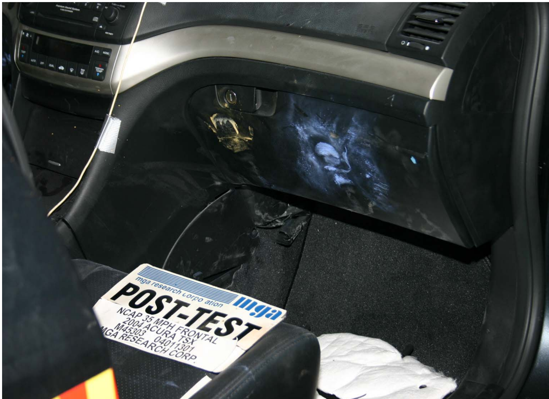
Post-Test Passenger Dummy Knee Contact
