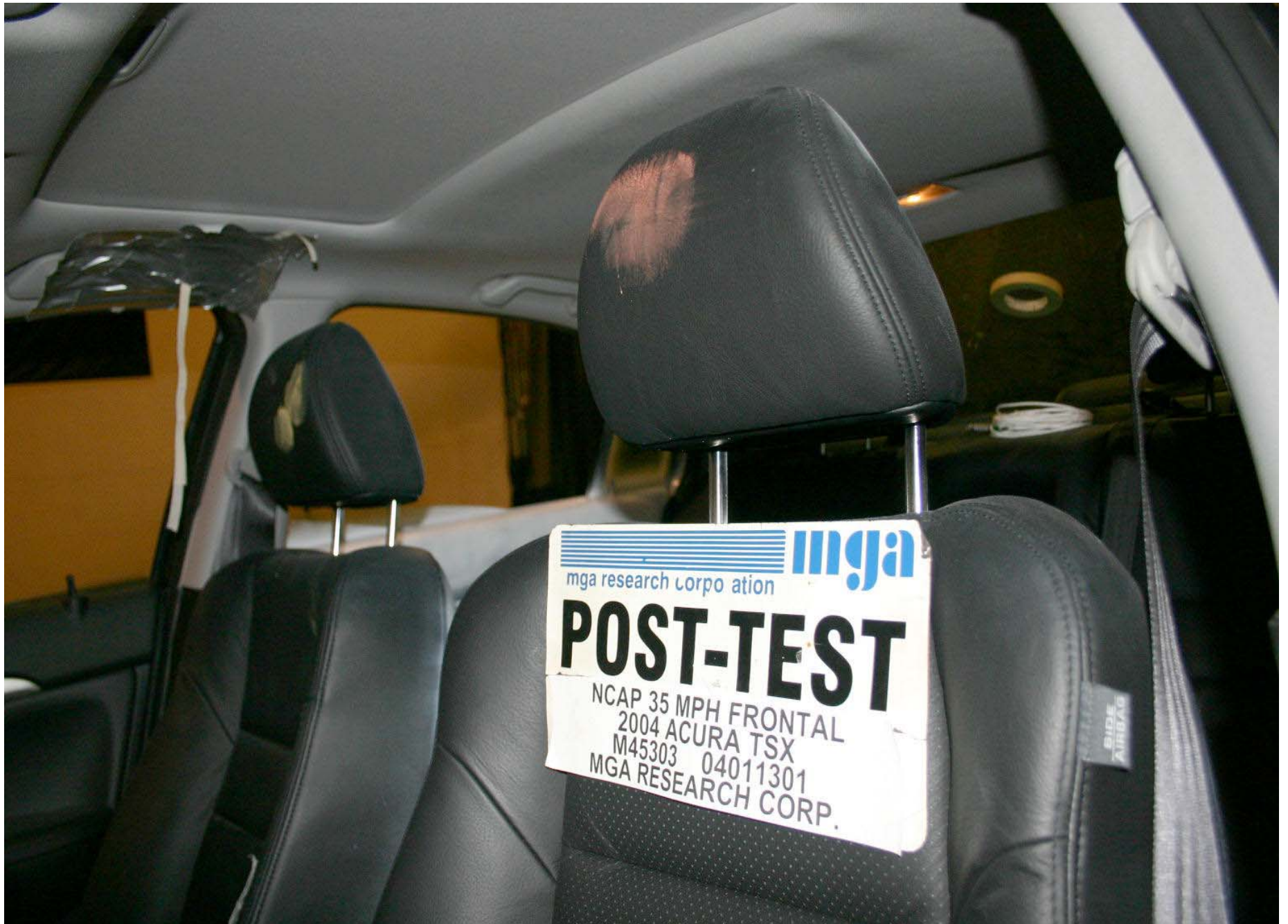
Post-Test Driver Dummy Head Contact
