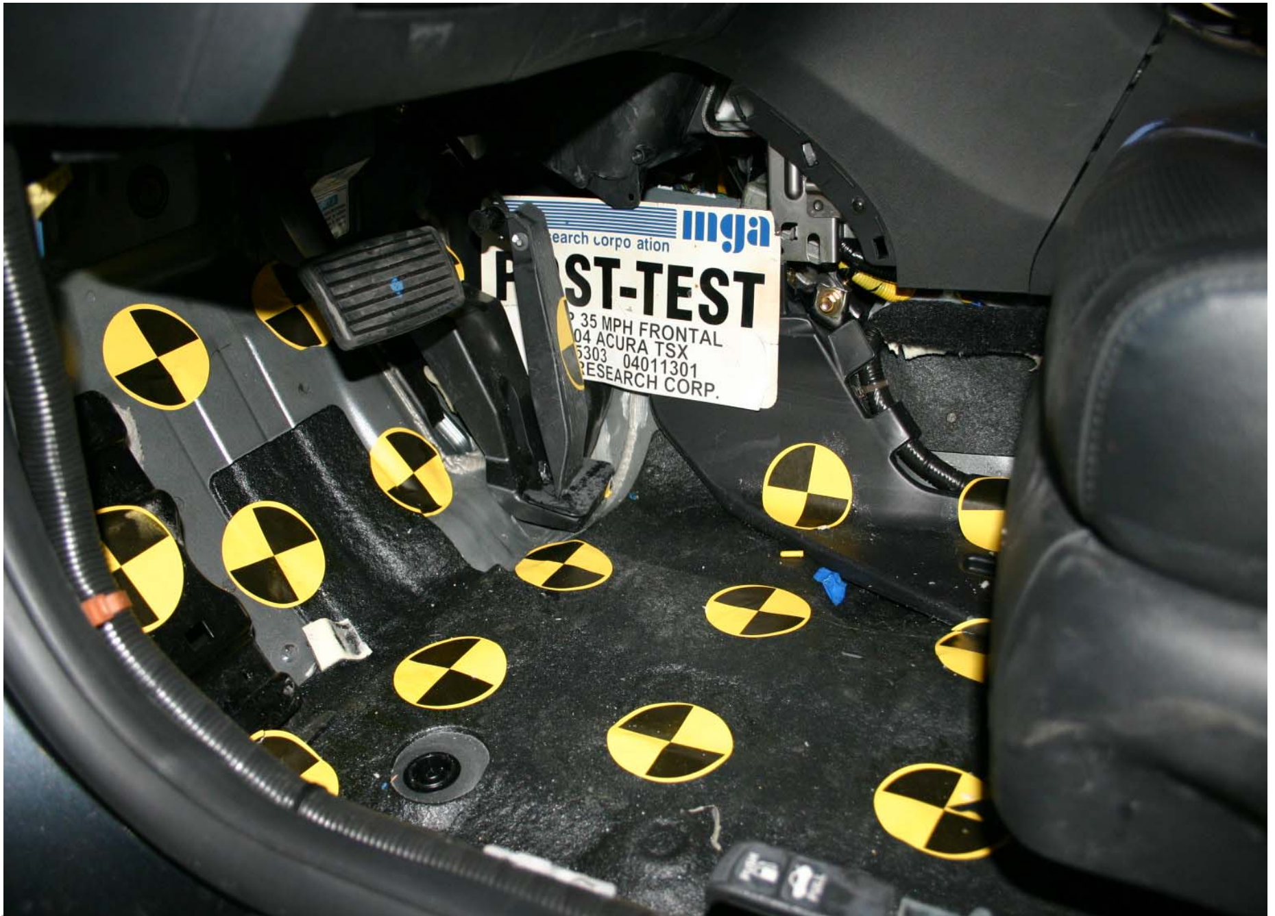
Post-Test Driver Side Floor Pan View
