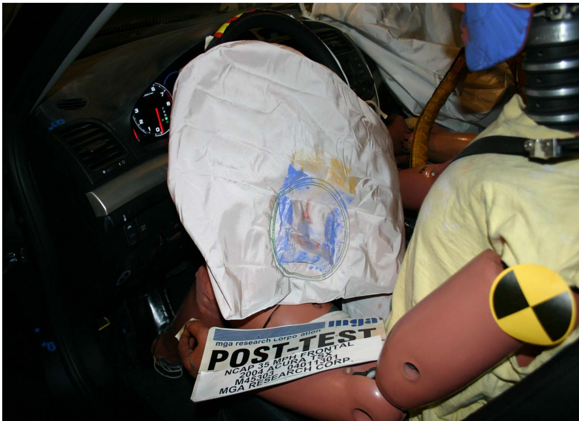
Post-Test Driver Dummy Airbag Contact
