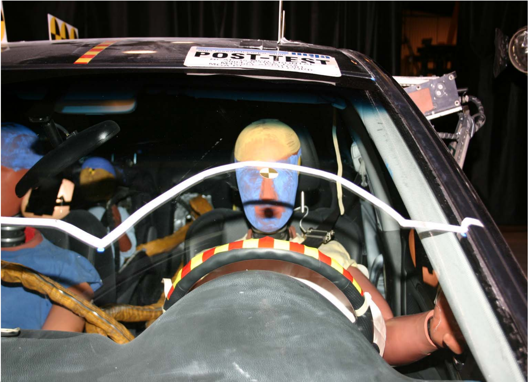
Post-Test Driver Dummy Front View (head position)
