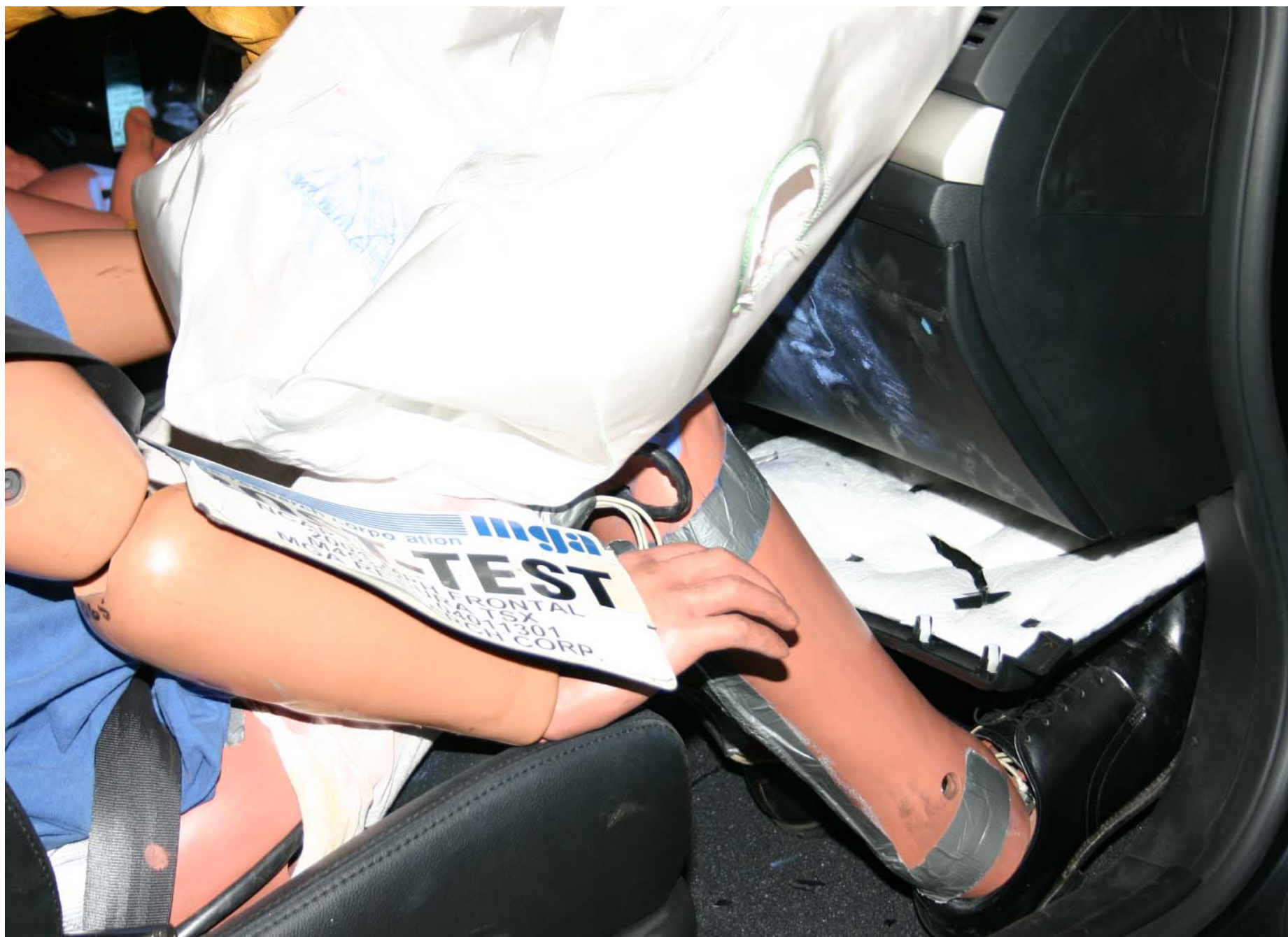
Post-Test Passenger Knee Bolster View
