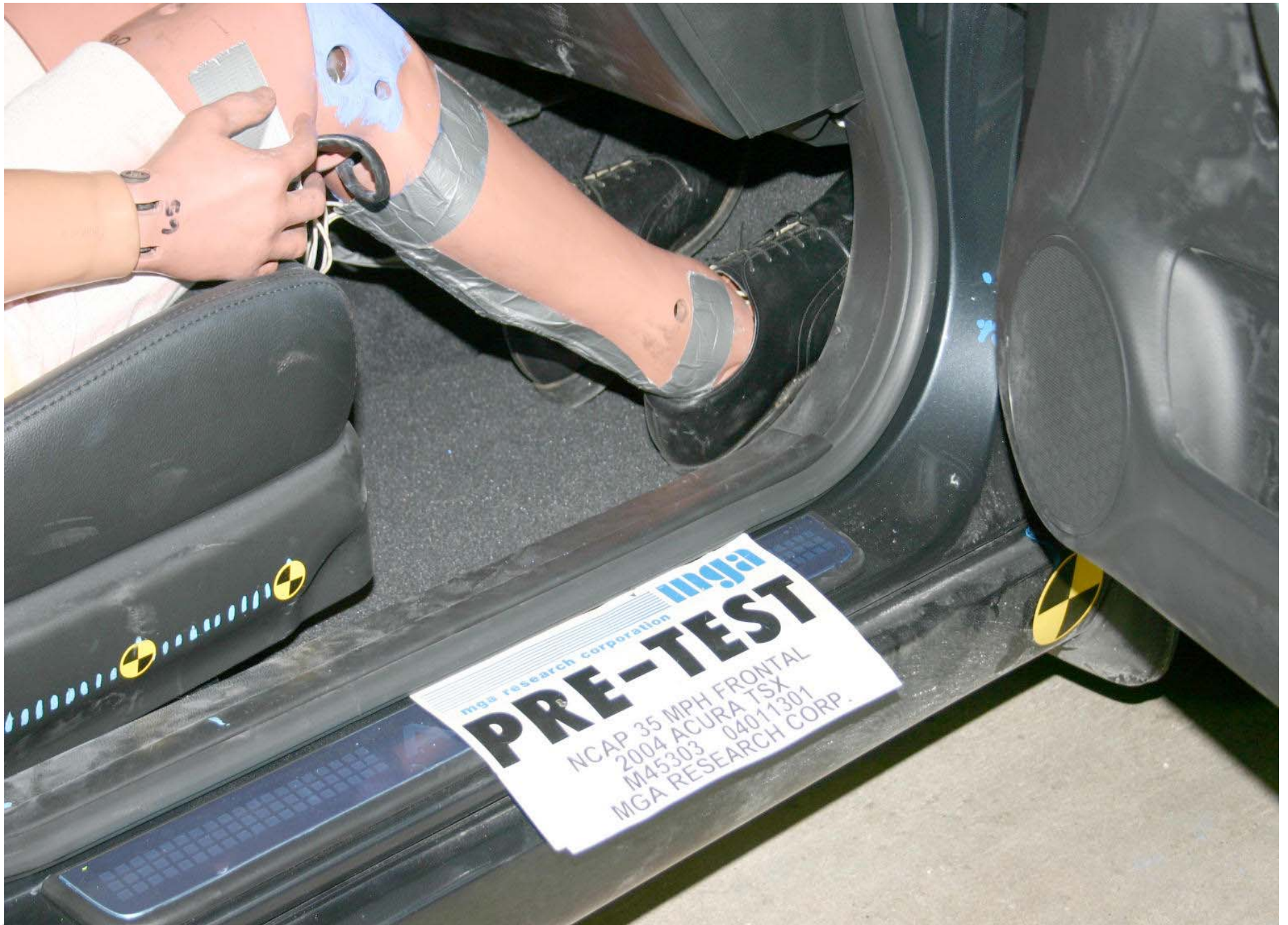
Pre-Test Passenger Dummy Feet Position
