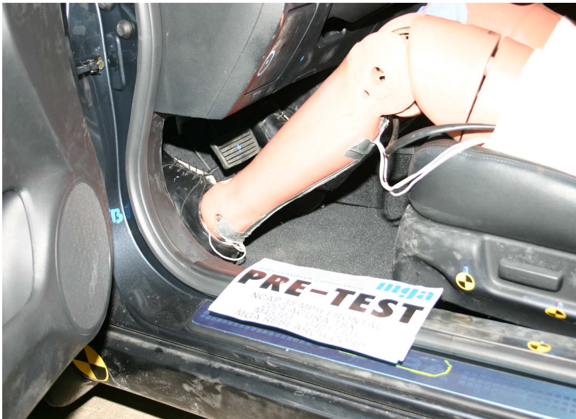
Pre-Test Driver Dummy Feet Position
