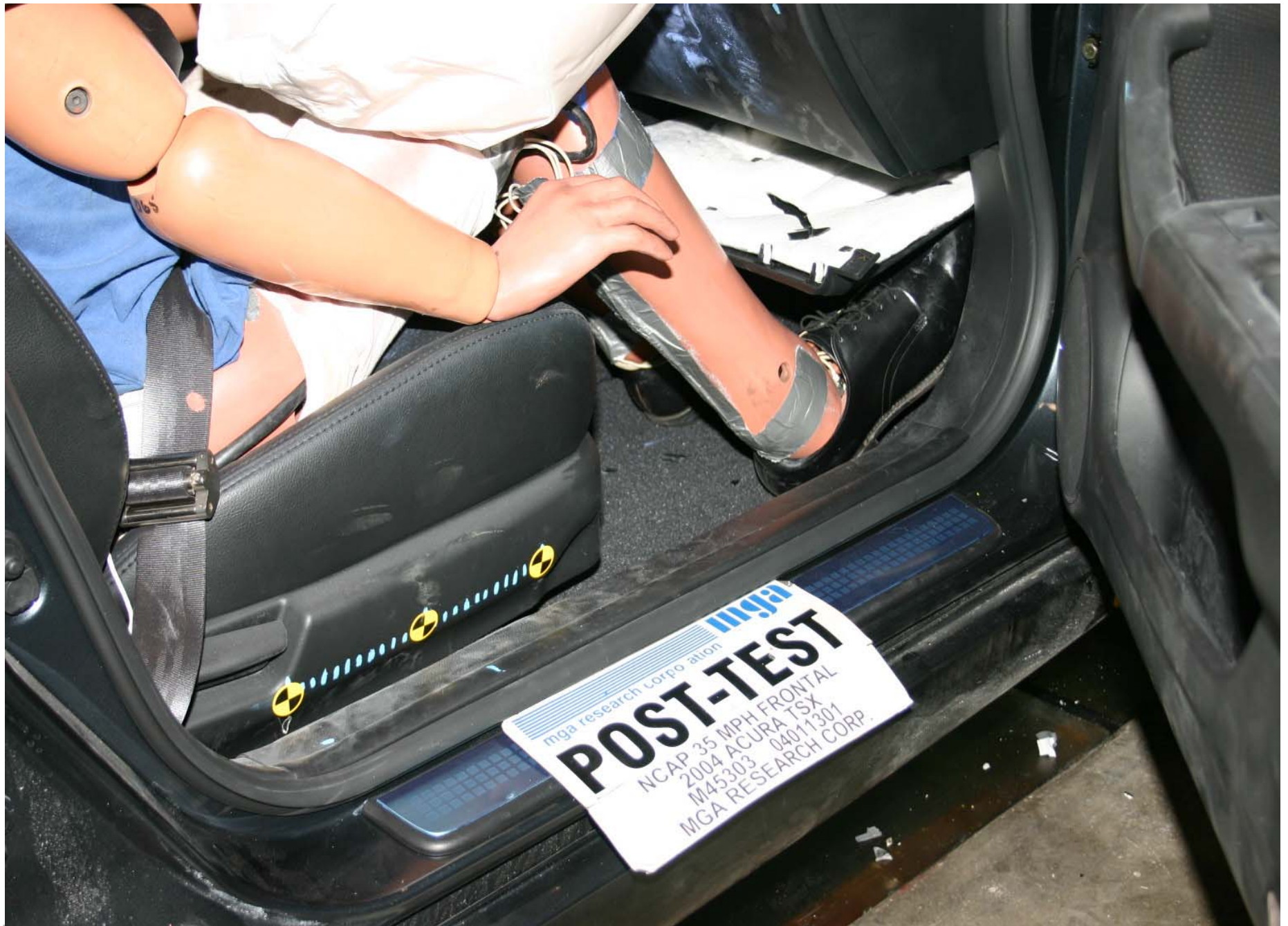
Post-Test Passenger Dummy Feet Position
