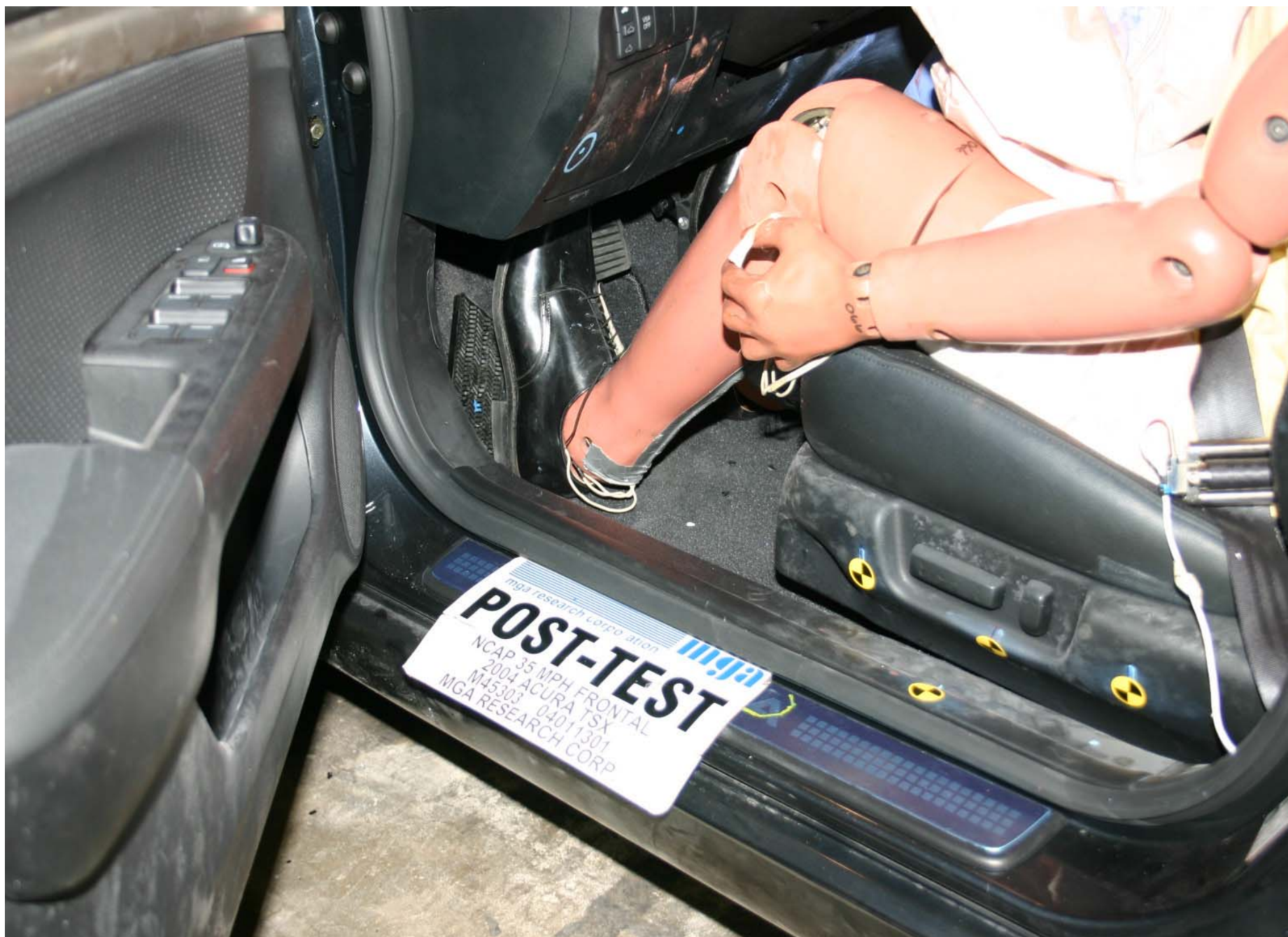
Post-Test Driver Dummy Feet Position
