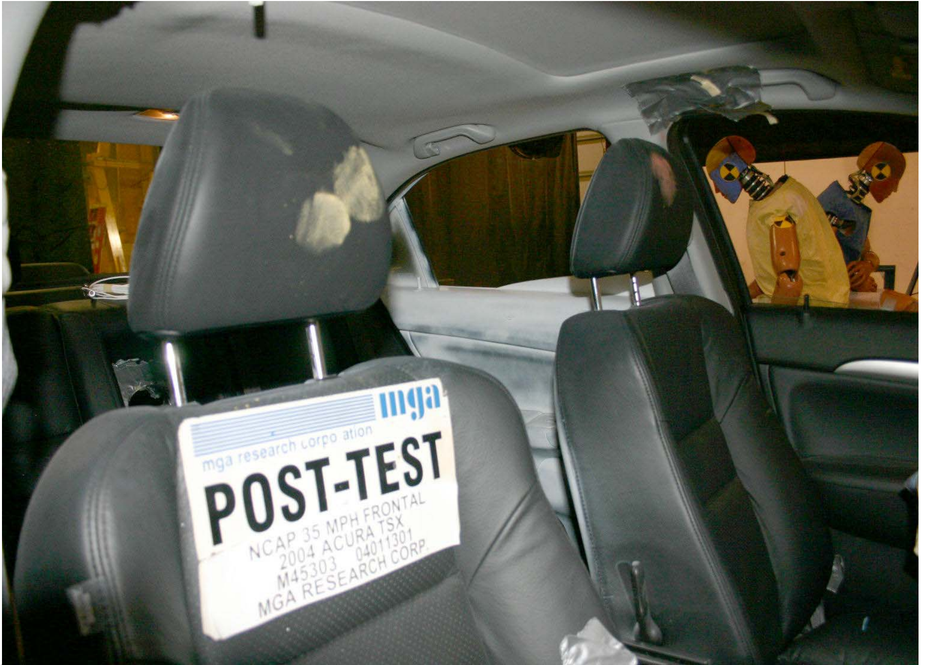
Post-Test Passenger Dummy Head Contact
