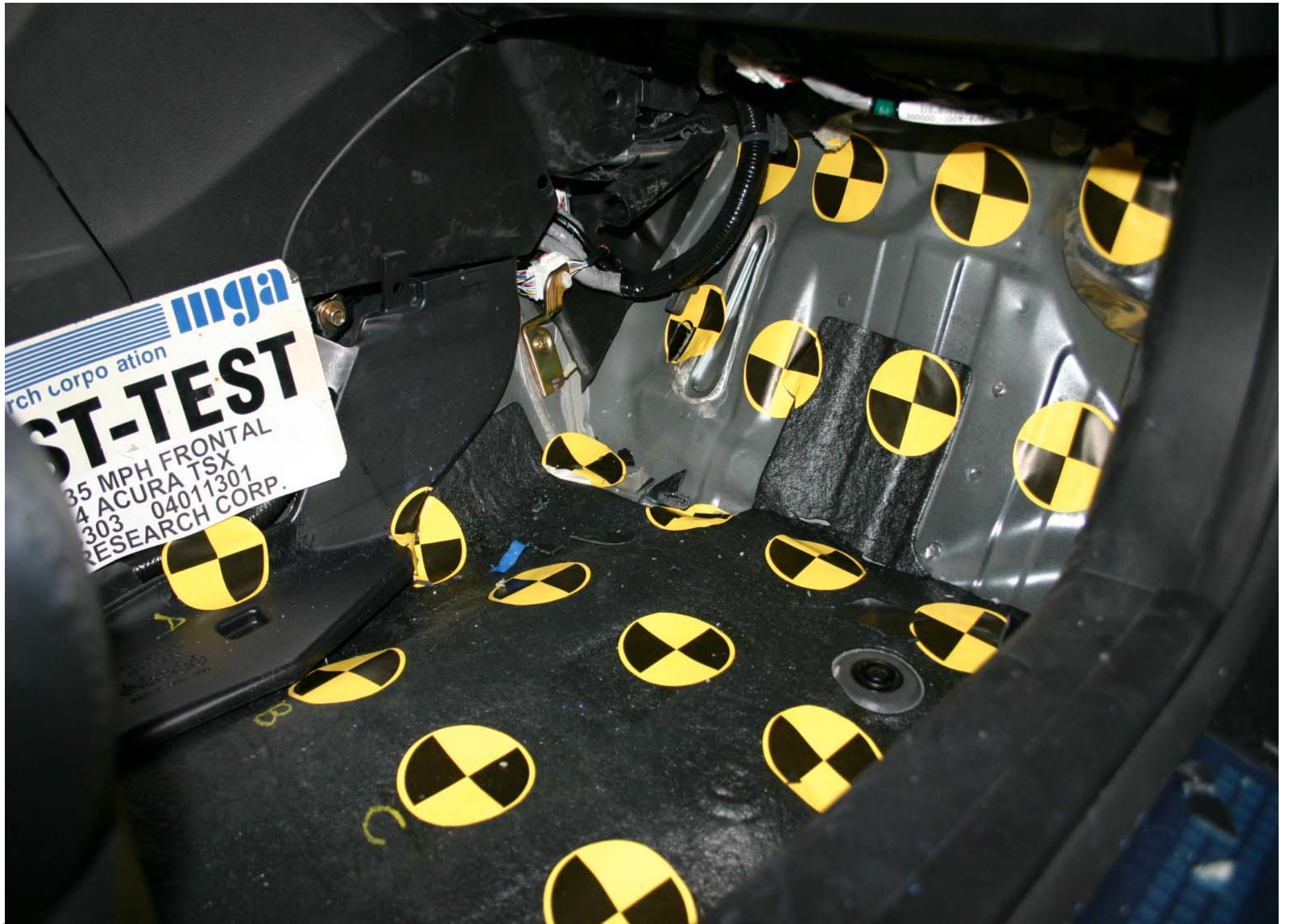
Post-Test Passenger Side Floor Pan View
