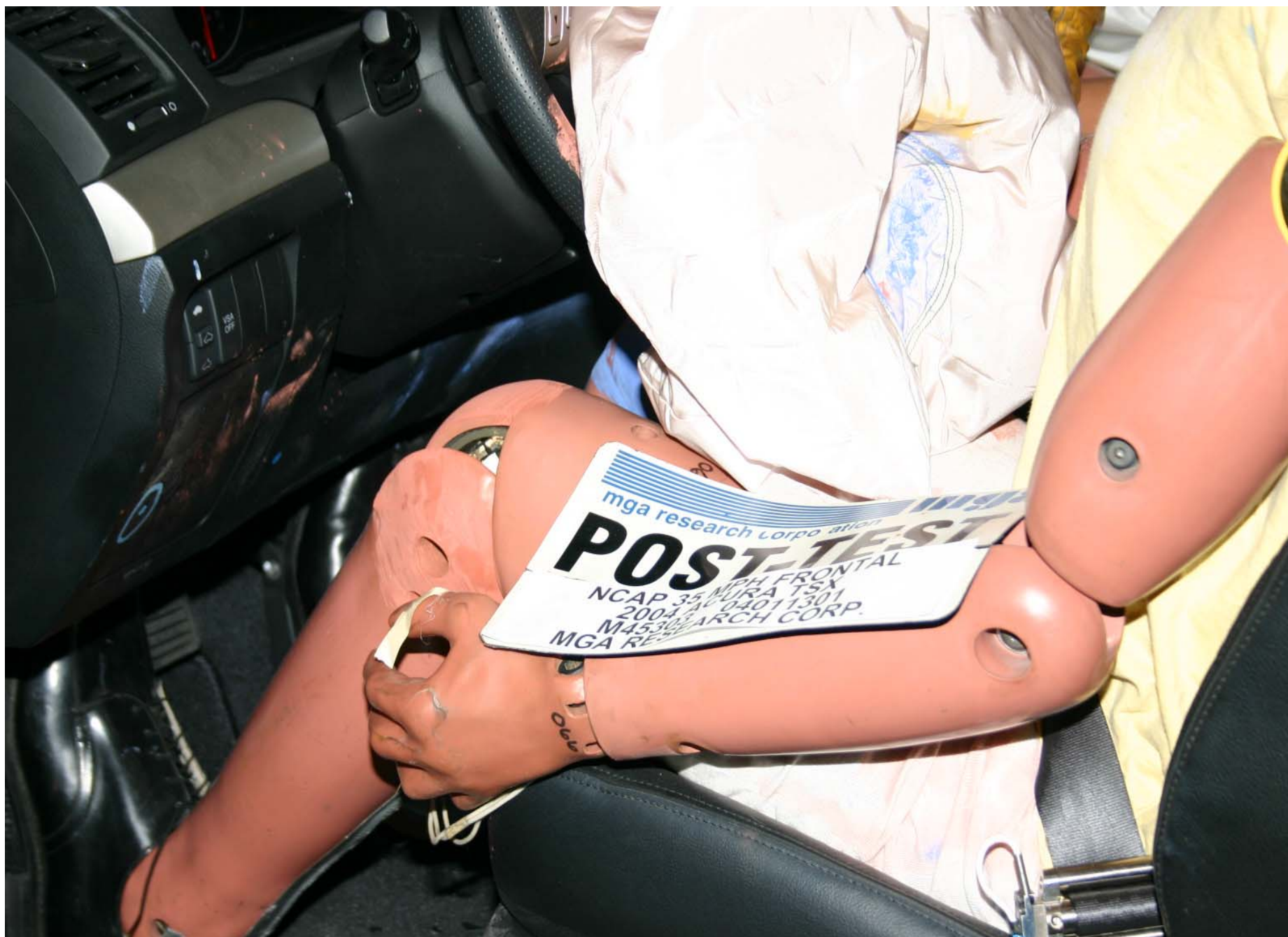
Post-Test Driver Side Knee Bolster View
