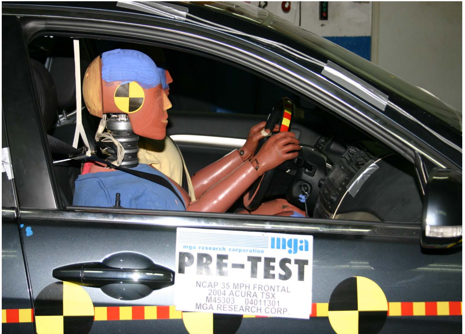
Pre-Test Passenger Dummy Position Right Side View
