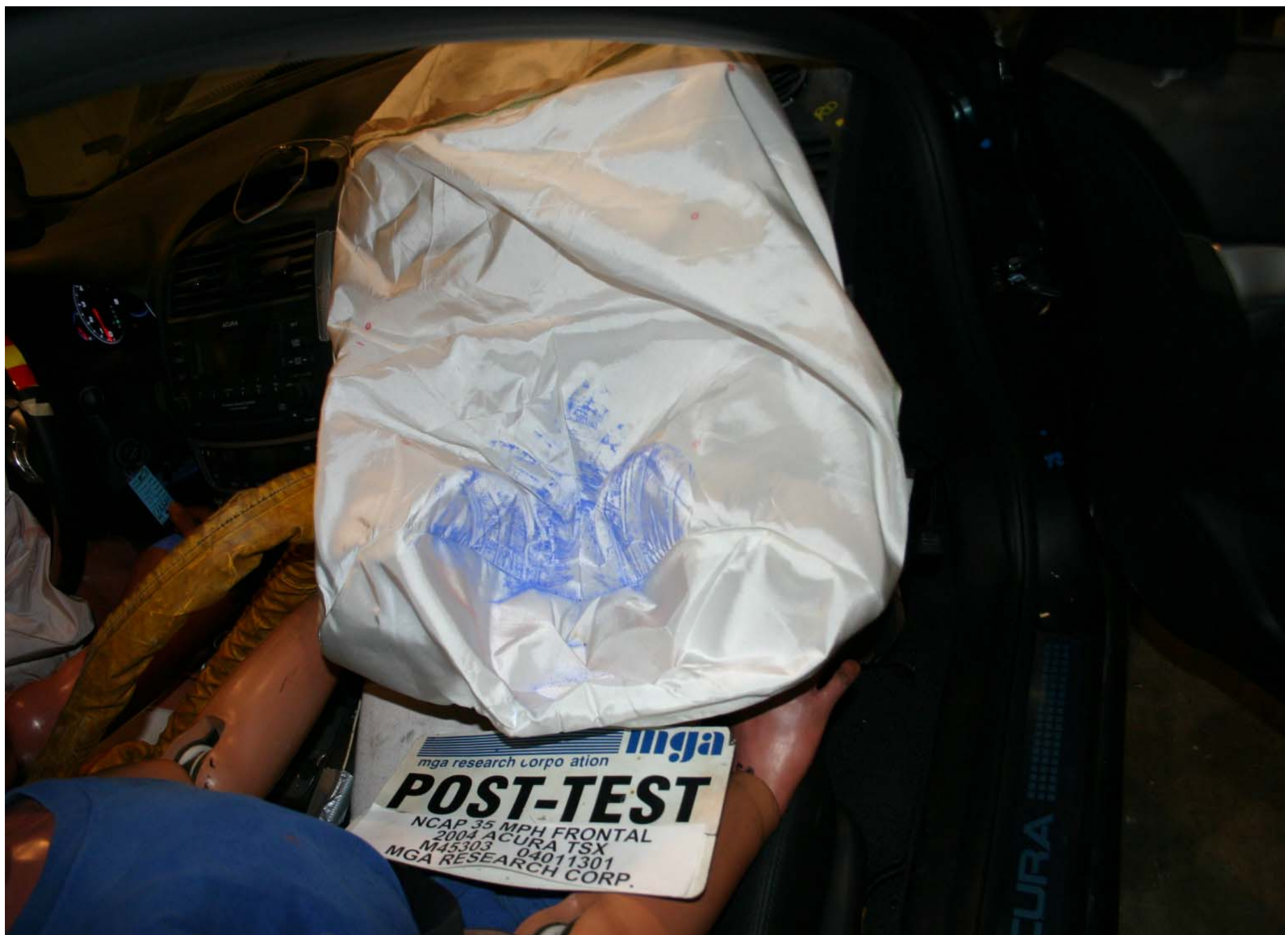
Post-Test Passenger Dummy Airbag Contact
