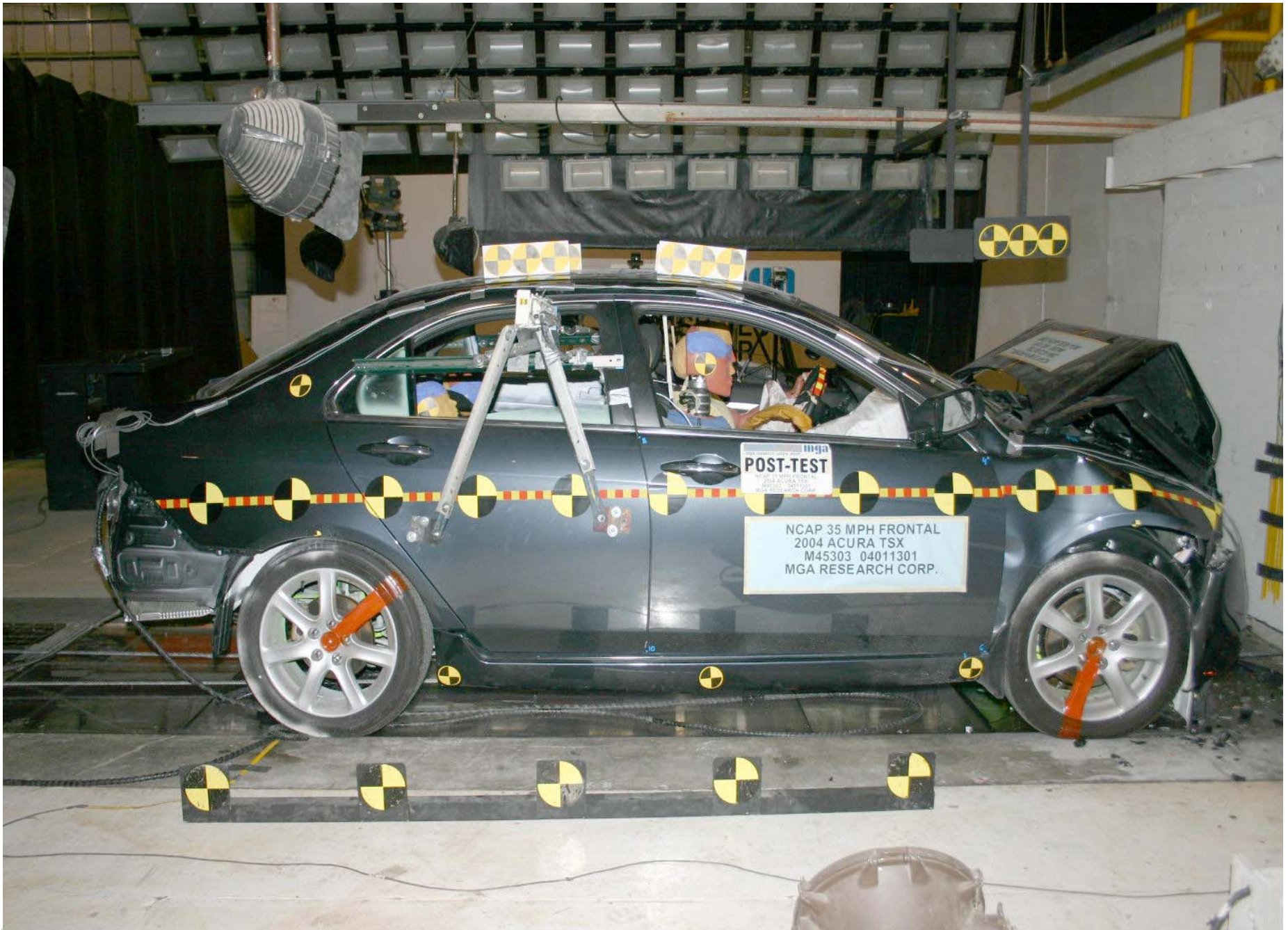
Post-Test Right Side View of Test Vehicle
