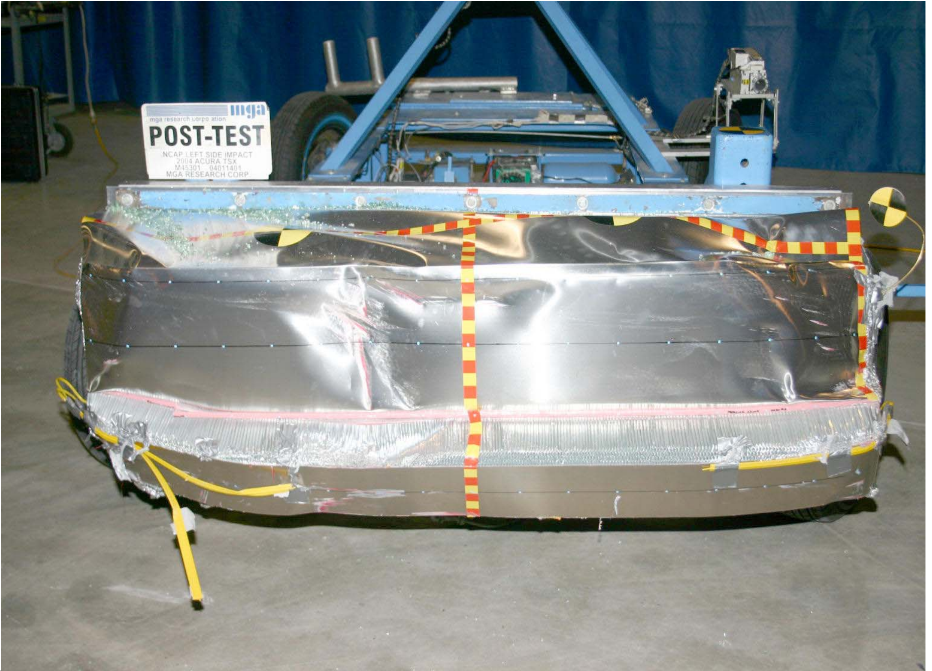
Post-Test MDB Front View
