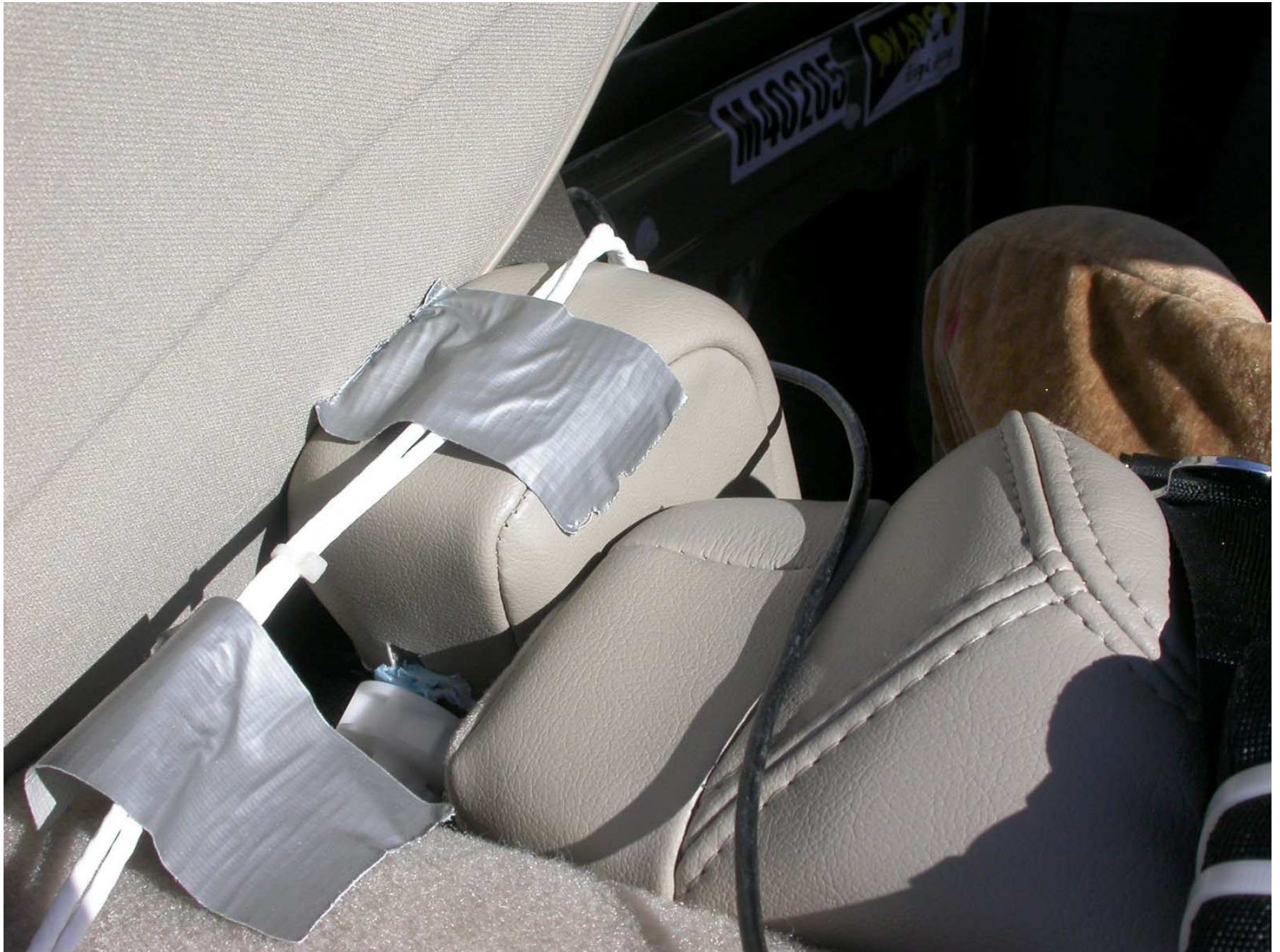
Figure F2-34: Post-Test Position 4 Seat Trim Separation
