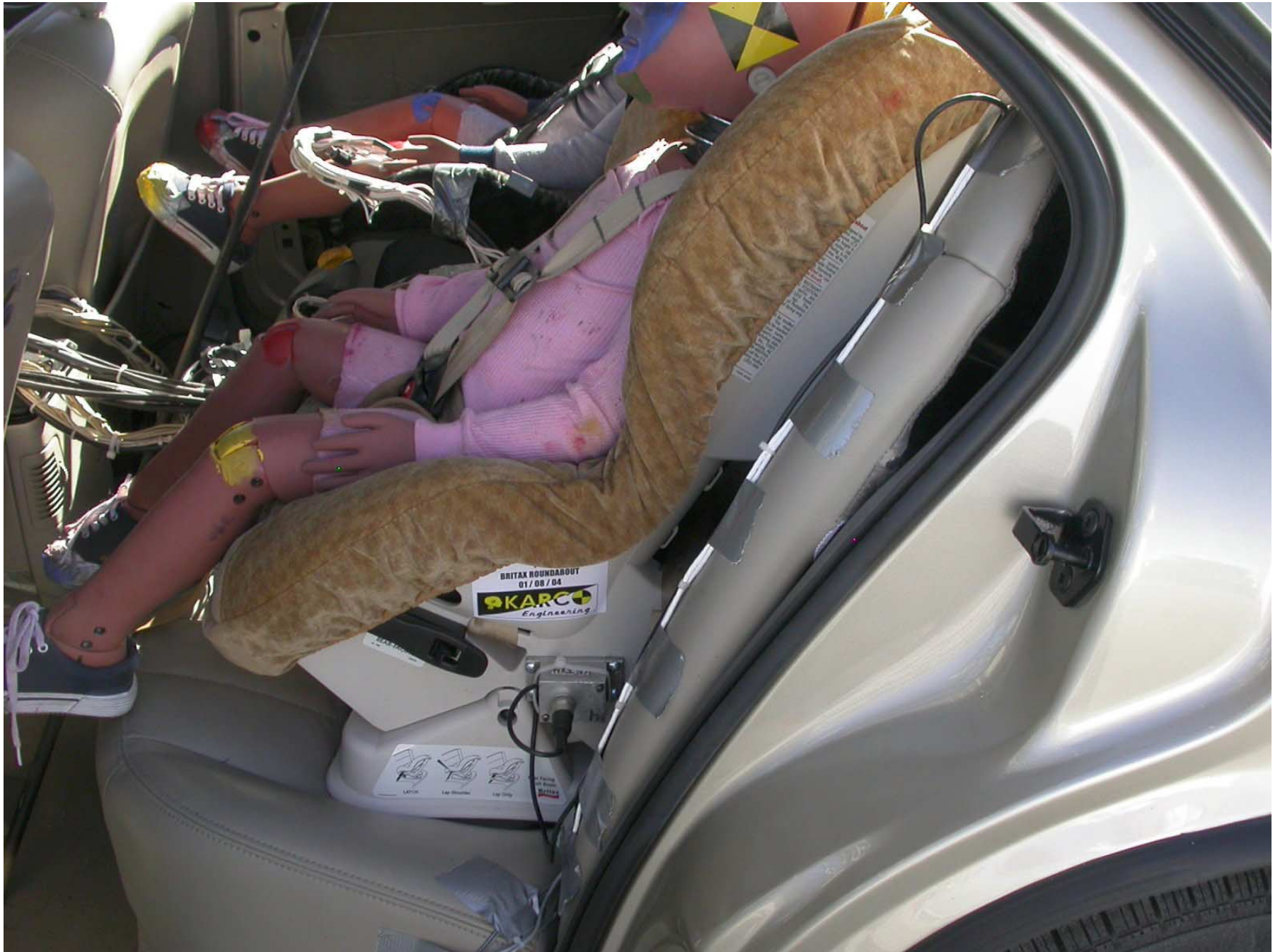
Figure F2-33: Post-Test Position 4 Seat Trim Separation
