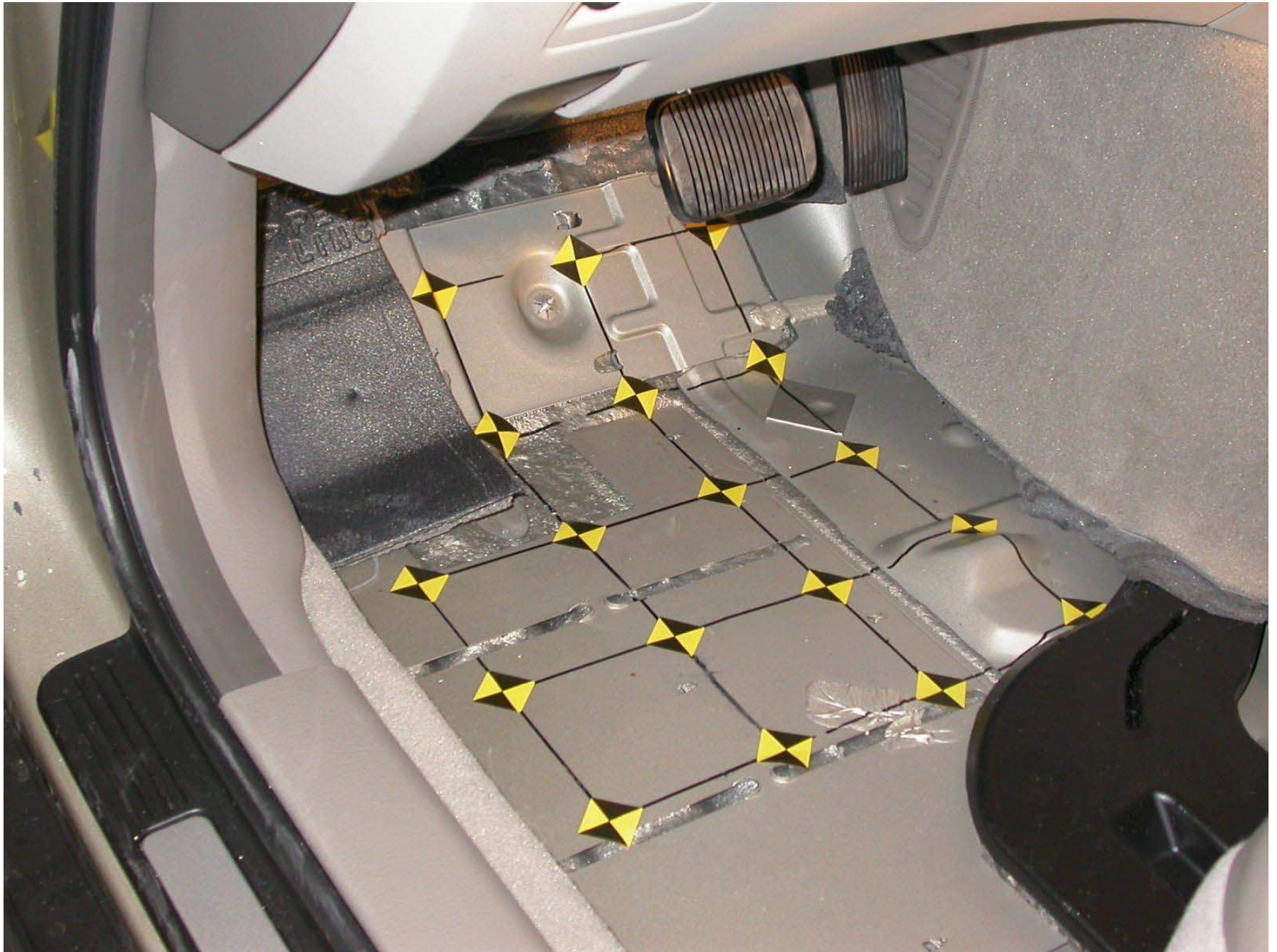
Figure A-40: Pre-Test Driver Side Floor Pan
