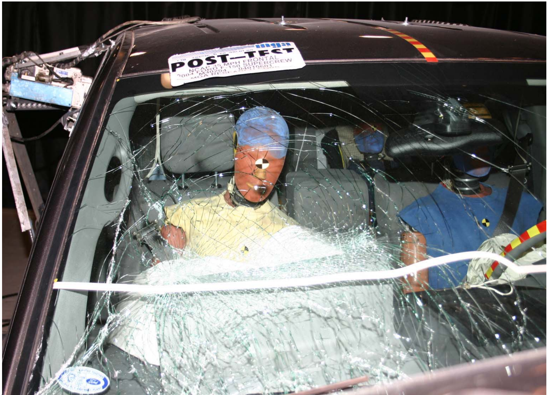
Post-Test Passenger Dummy Front View (head position)
