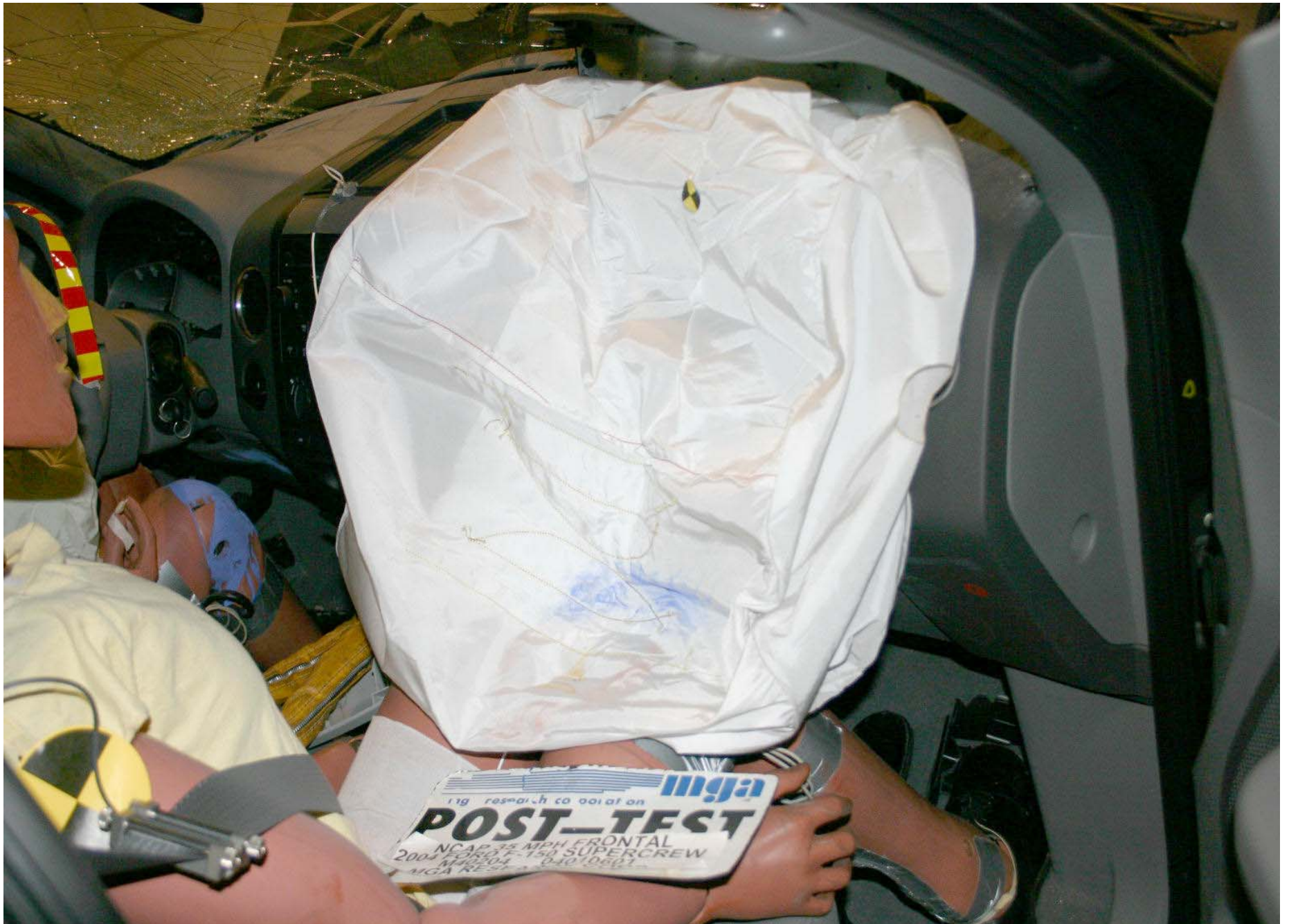
Post-Test Passenger Dummy Airbag Contact
