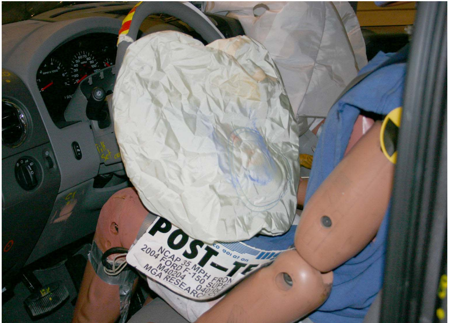
Post-Test Driver Dummy Airbag Contact
