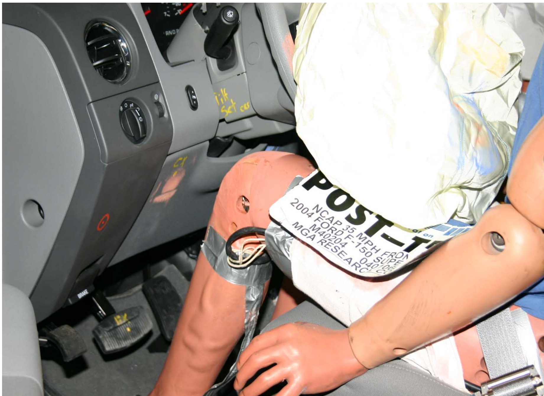
Post-Test Driver Side Knee Bolster View
