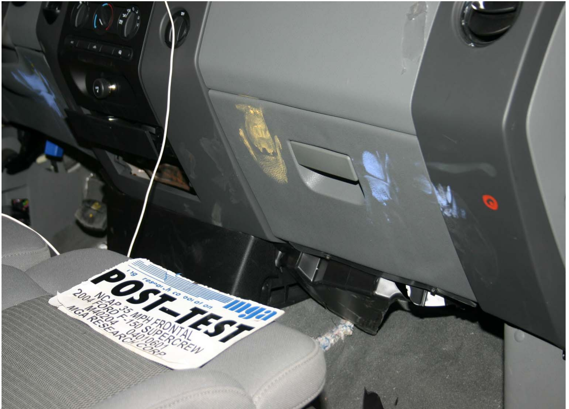
Post-Test Passenger Dummy Knee Contact
