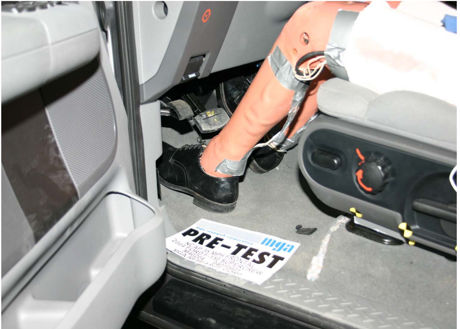
Pre-Test Driver Dummy Feet Position
