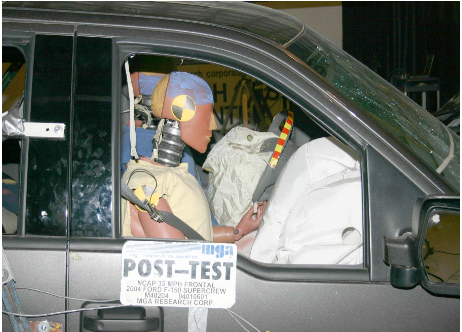
Post-Test Passenger Dummy Position Right Side View
