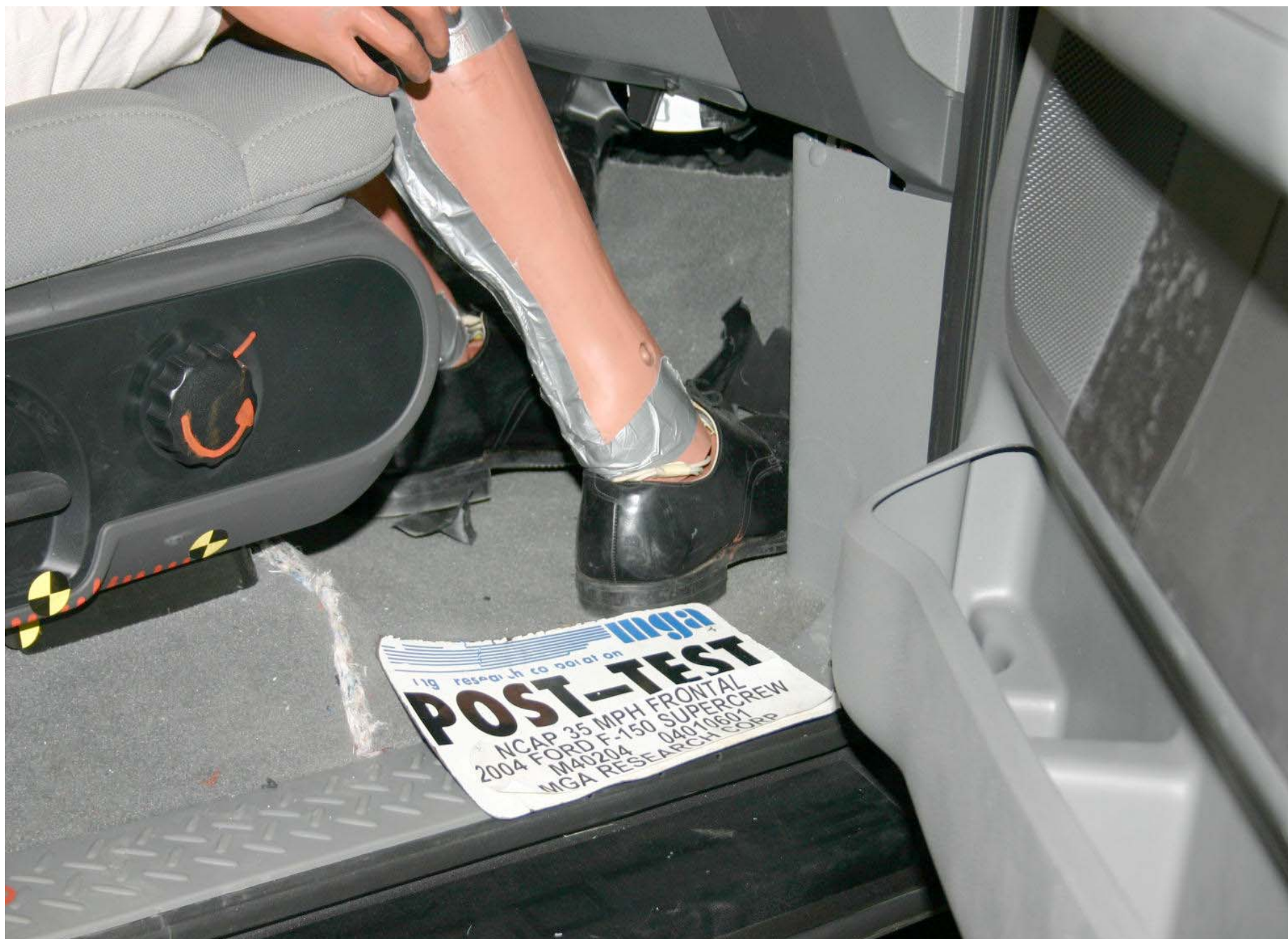
Post-Test Passenger Dummy Feet Position
