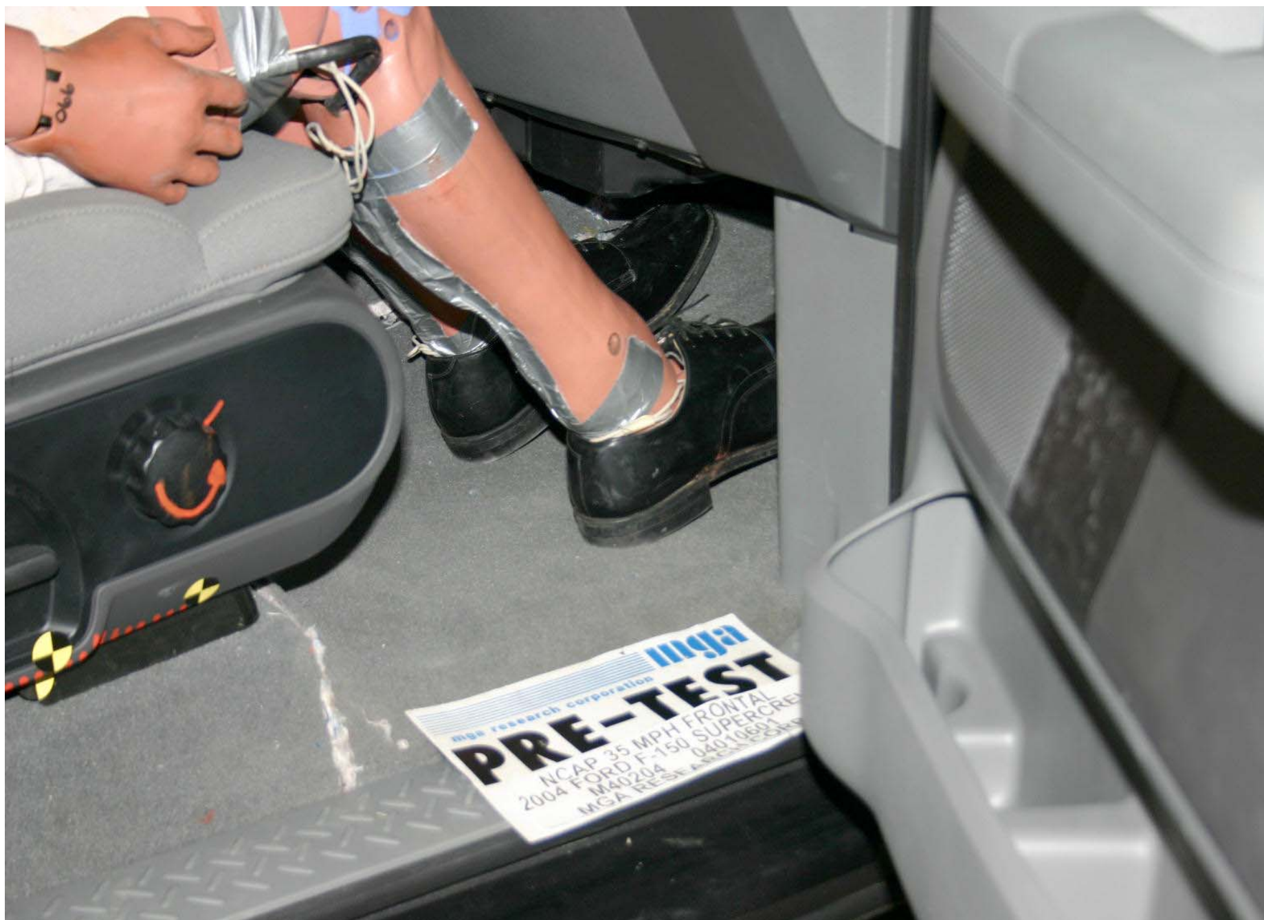
Pre-Test Passenger Dummy Feet Position
