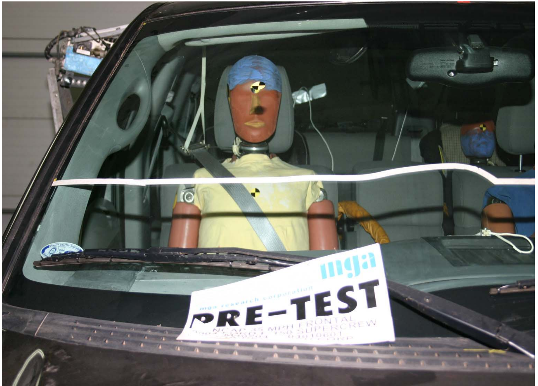
Pre-Test Passenger Dummy Front View (head position)
