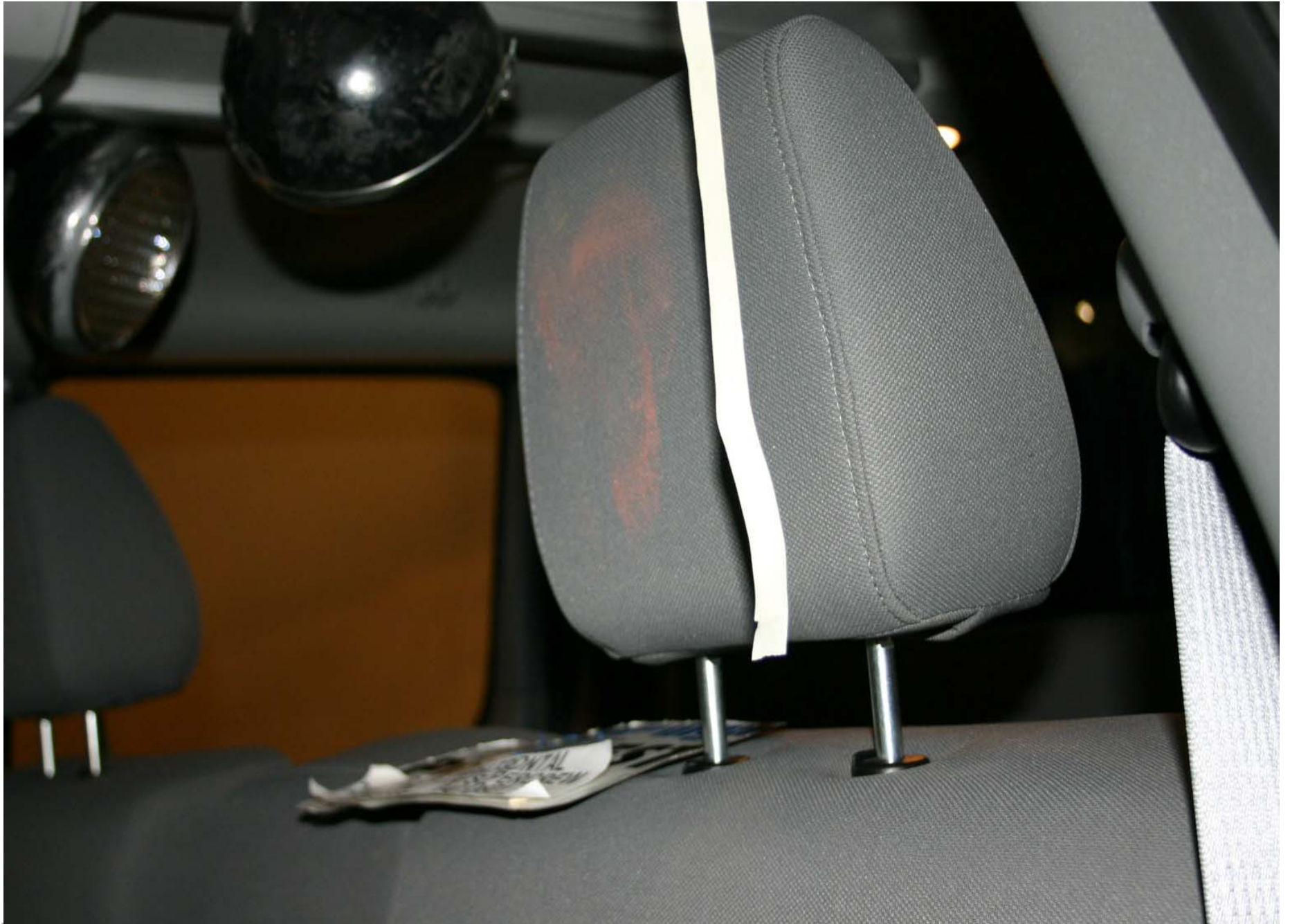
Post-Test Driver Dummy Head Contact
