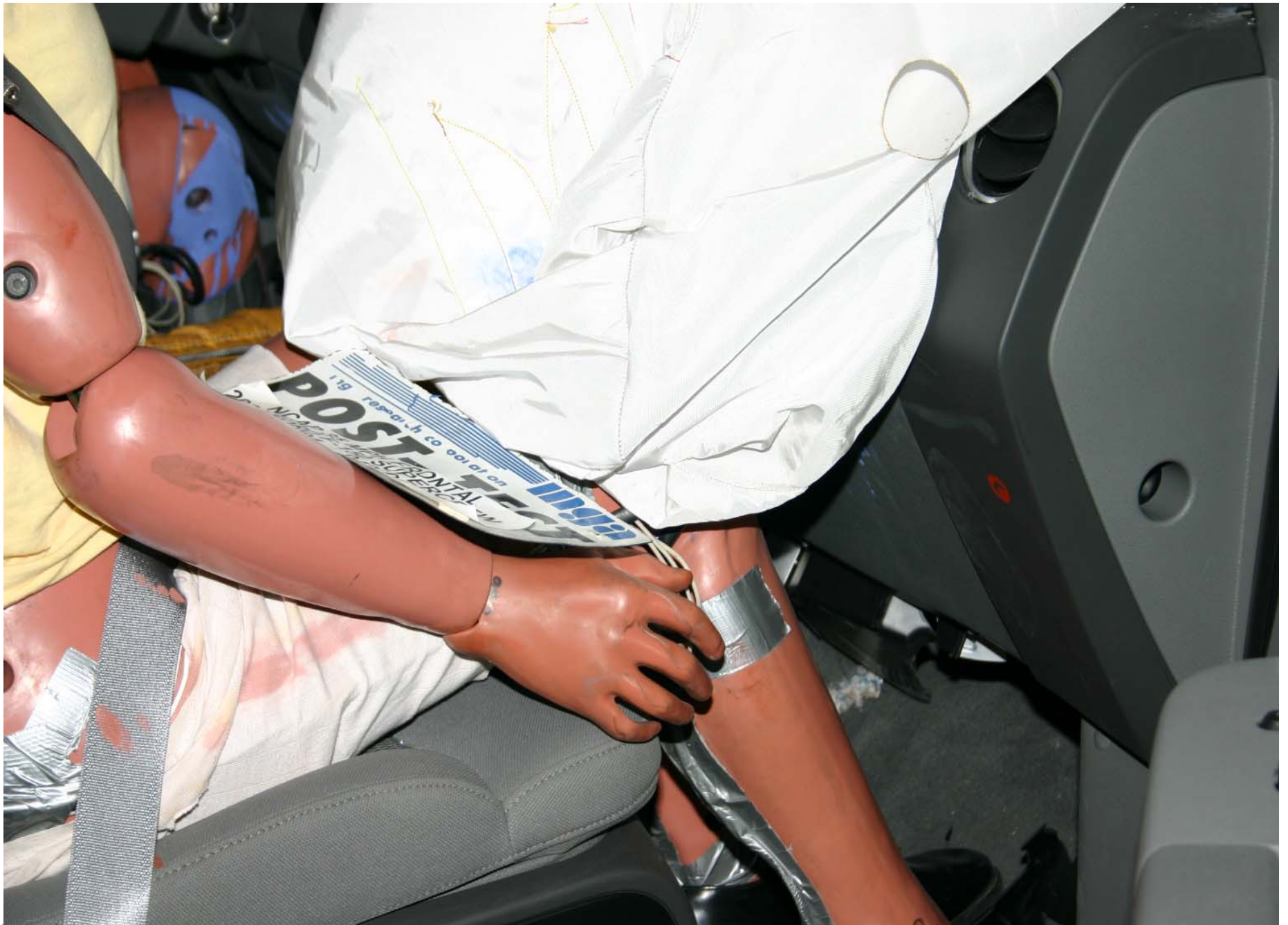
Post-Test Passenger Side Knee Bolster View
