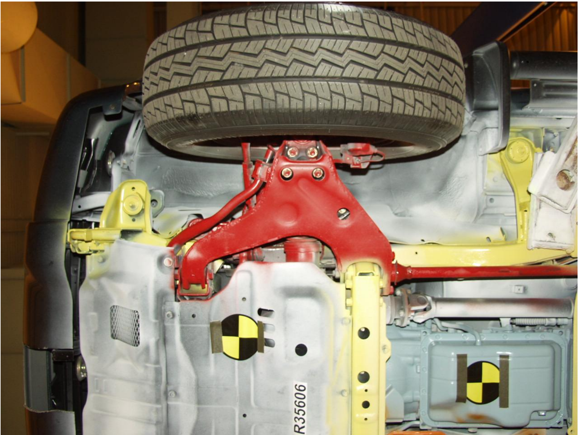
Figure A-66 PRE-TEST FRONT SUBFRAME VIEW
