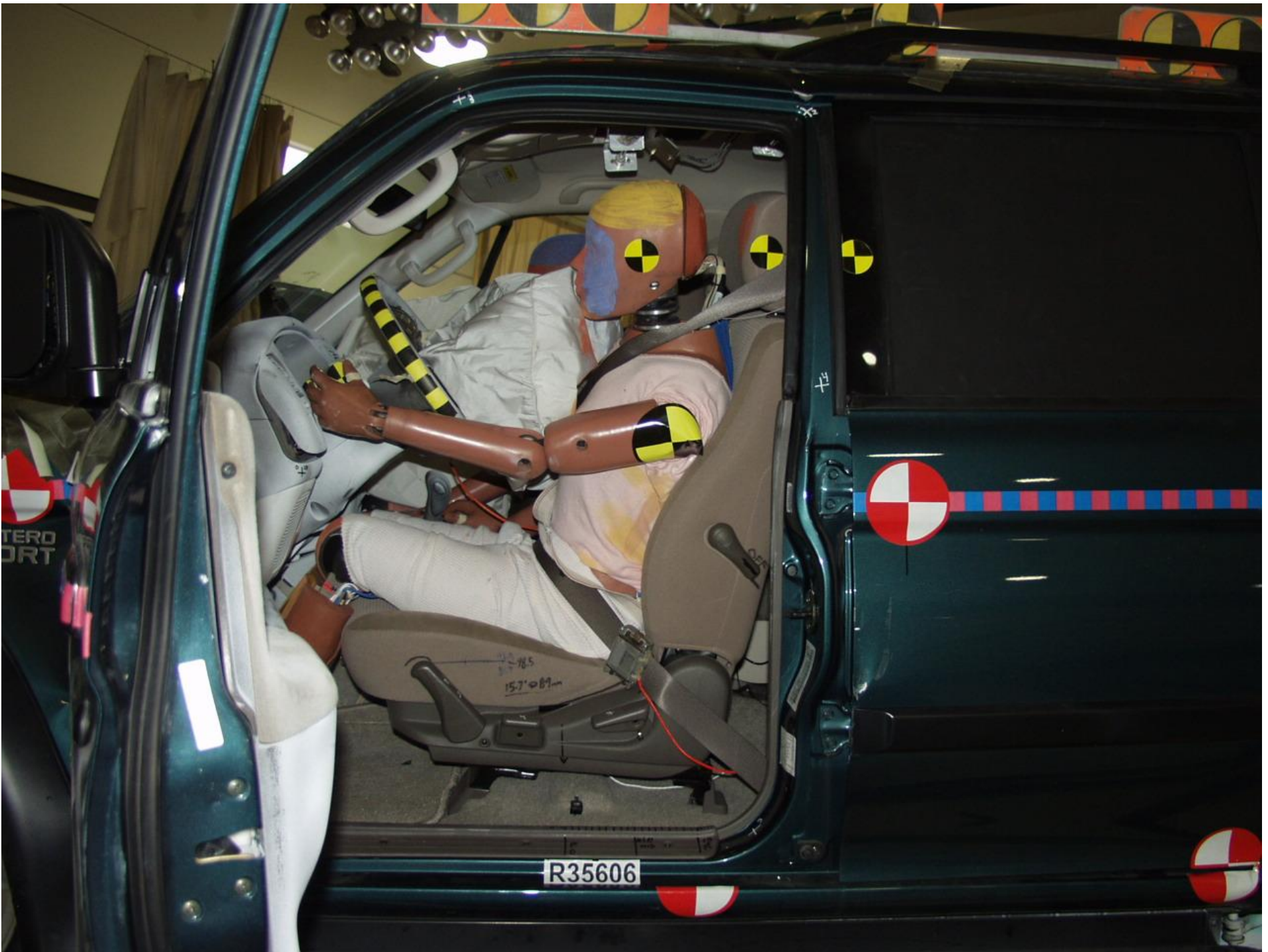
Figure A-22 POST-TEST DRIVER POSITION VIEW
