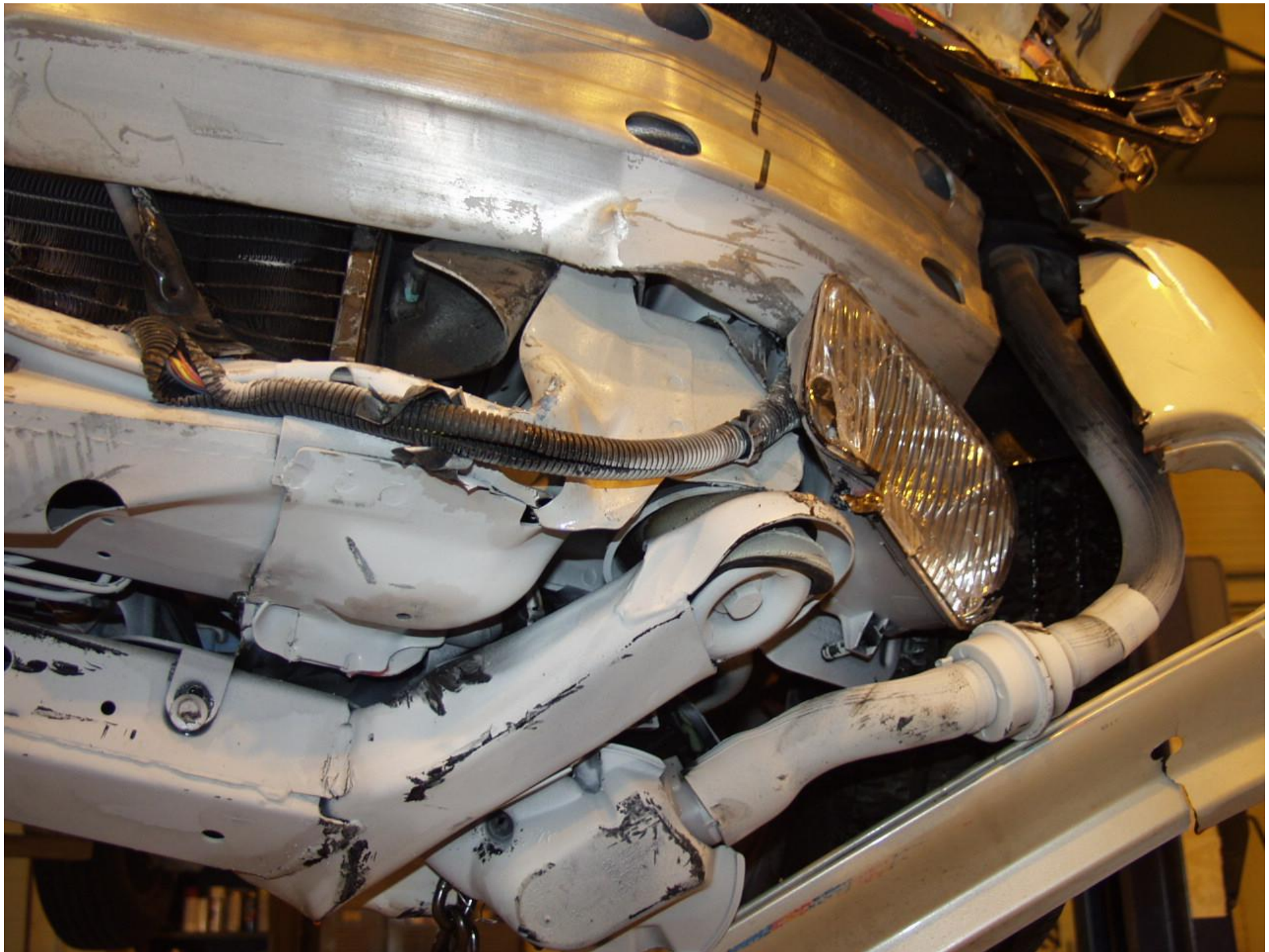
Figure A-73 POST-TEST BUMPER TO RAIL ATTACHMENT
