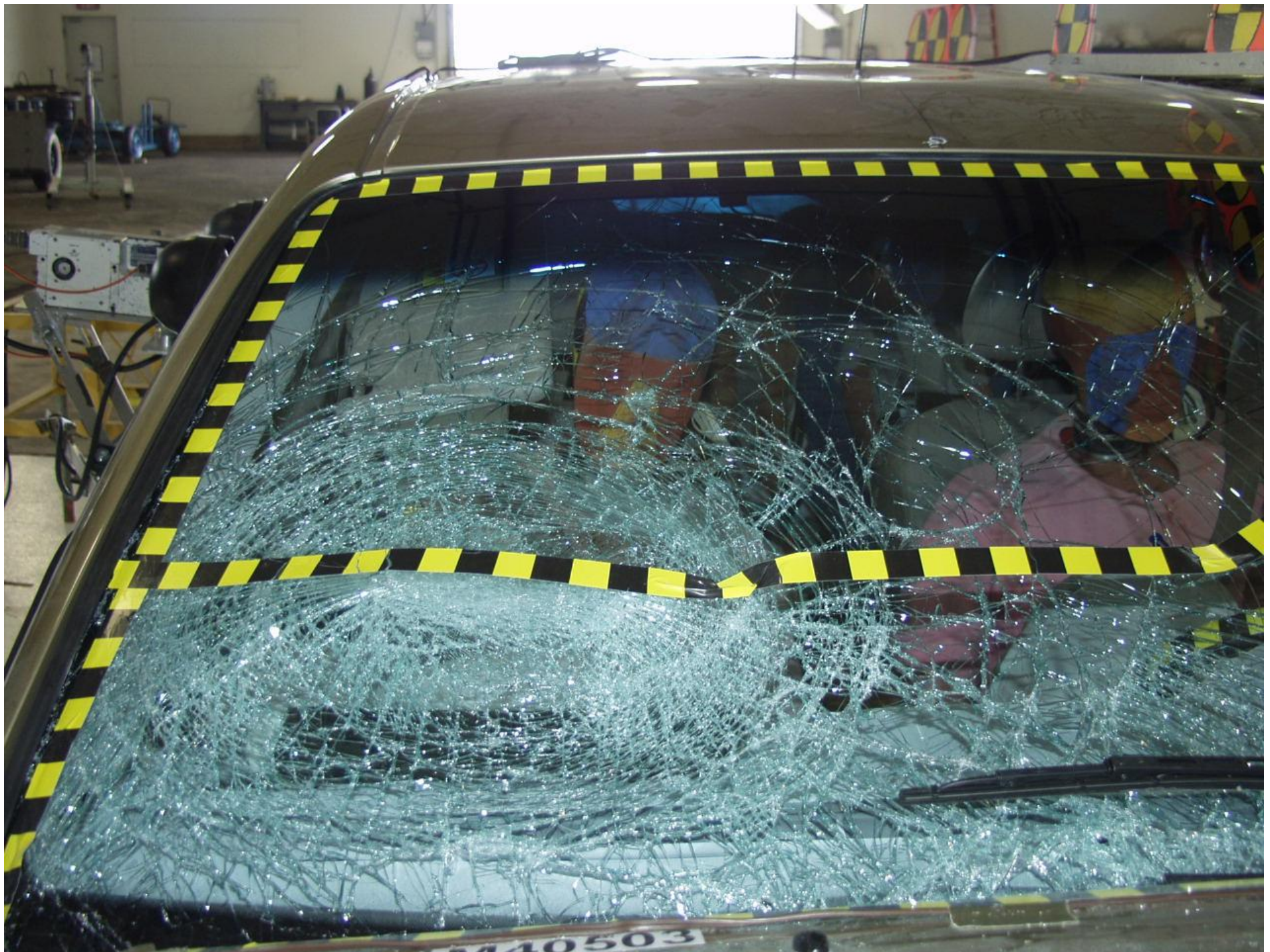
Figure A-45 POST-TEST PASSENGER HEAD LOCATION
