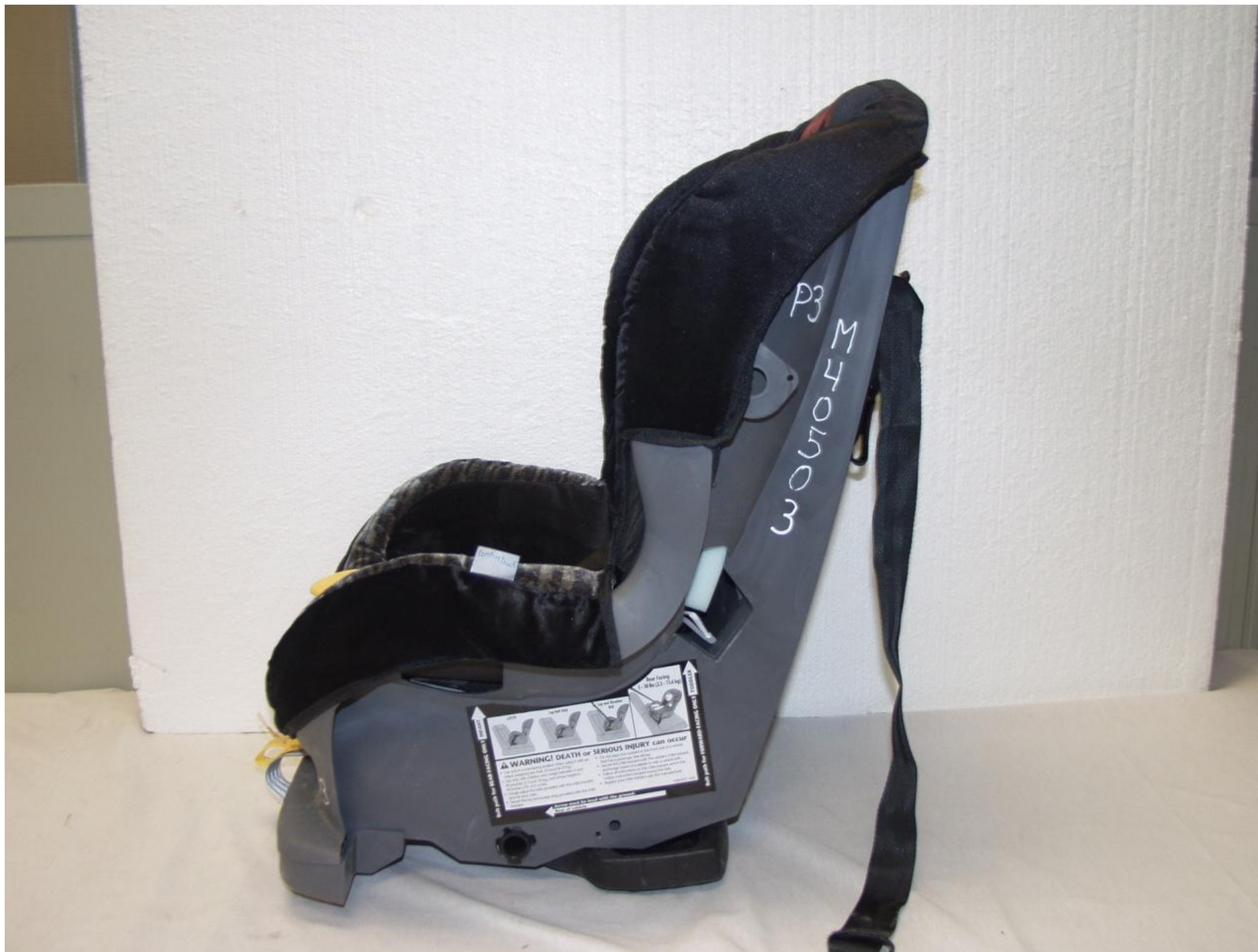
Figure 3-7 POST-TEST LEFT SIDE VIEW OF POSITION 3 CRS
