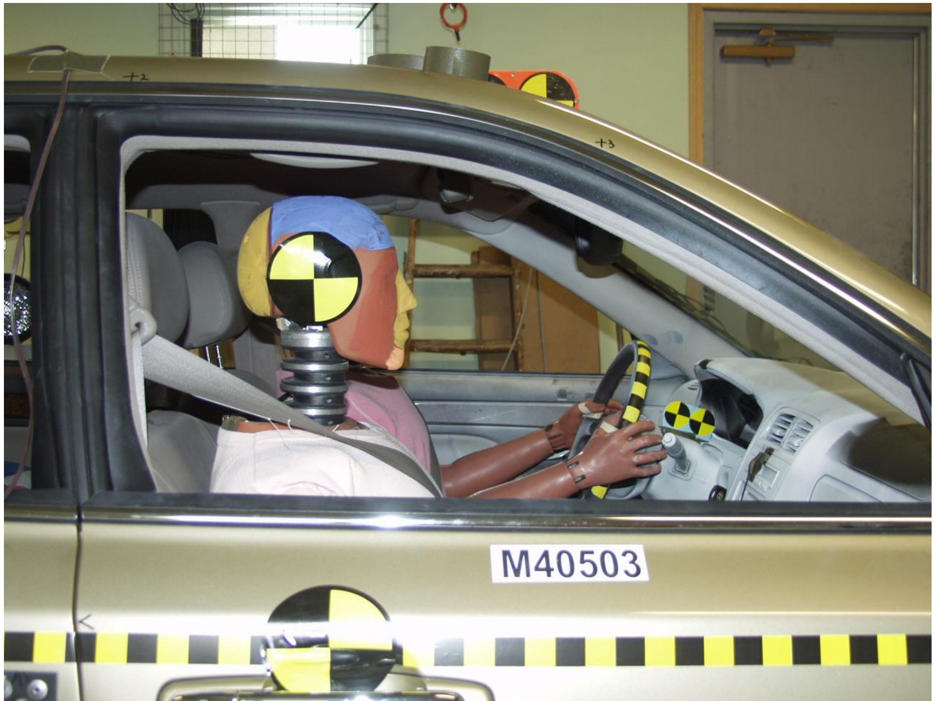
Figure A-46 PRE-TEST PASSENGER POSITION VIEW
