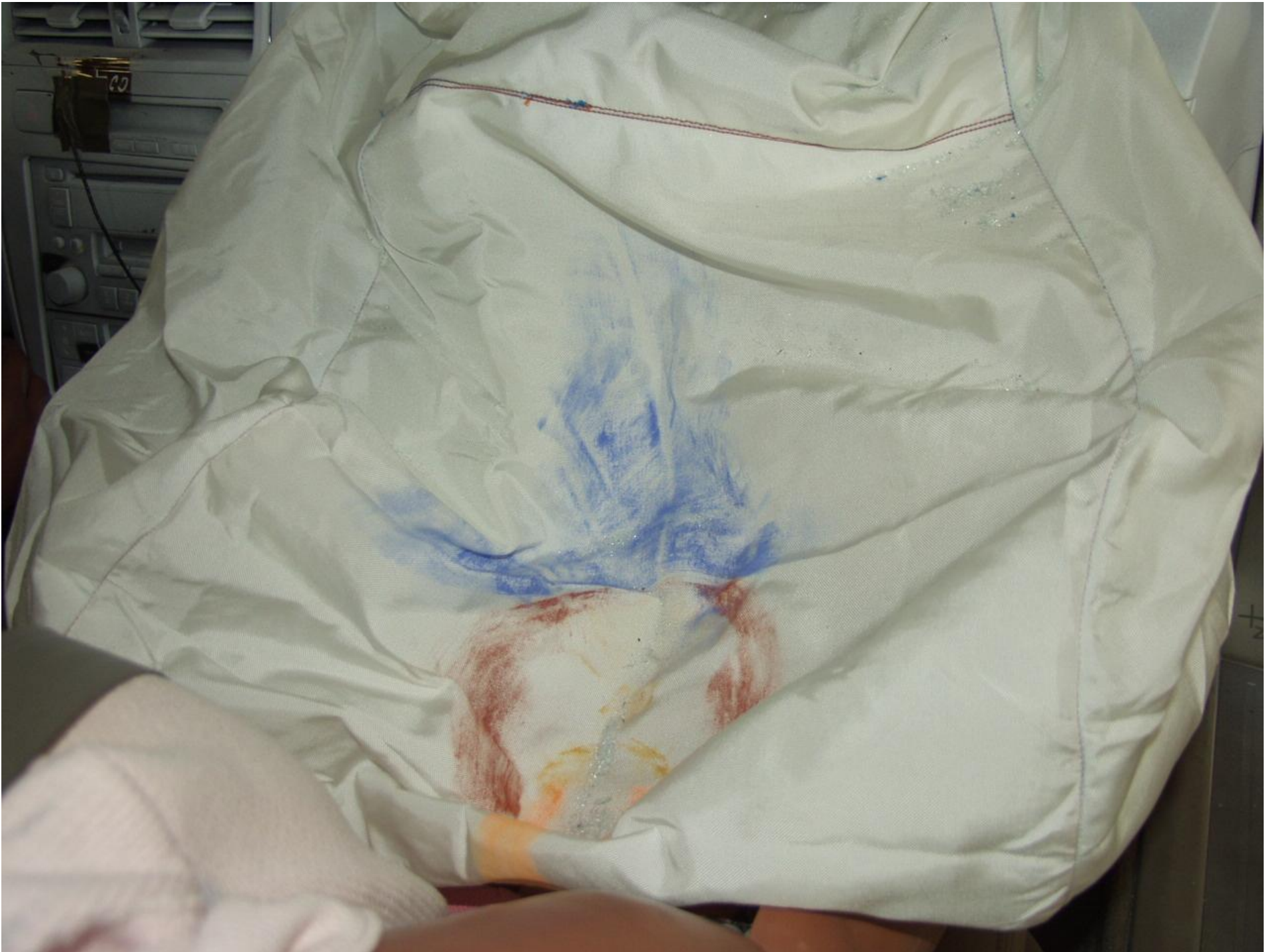
Figure A-57 POST-TEST PASSENGER CONTACT TO AIRBAG
