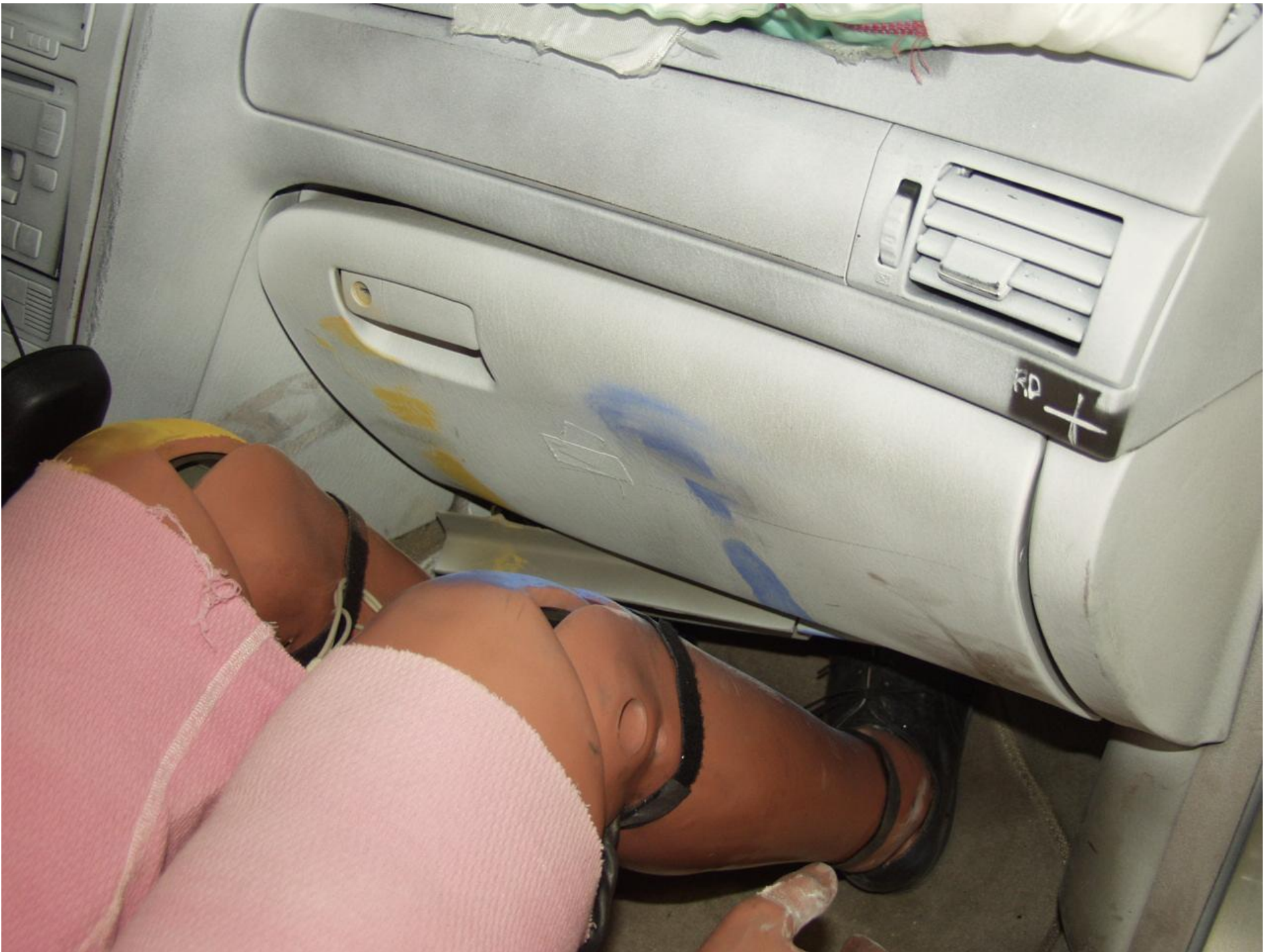
Figure A-53 POST-TEST PASSENGER KNEE BOLSTER VIEW
