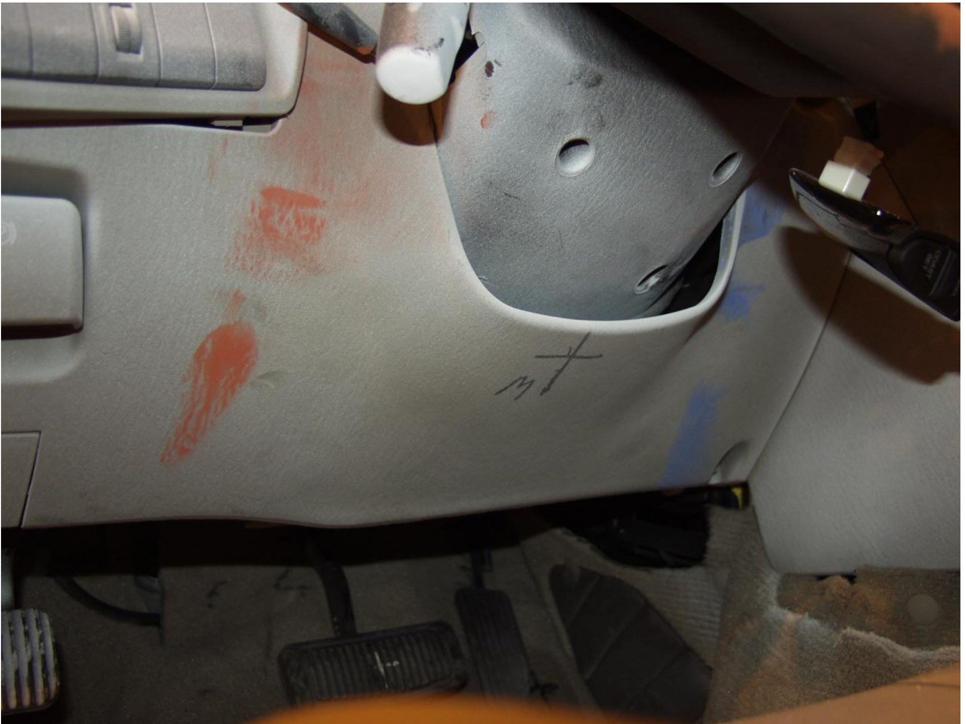
Figure A-39 POST-TEST DRIVER KNEE BOLSTER VIEW
