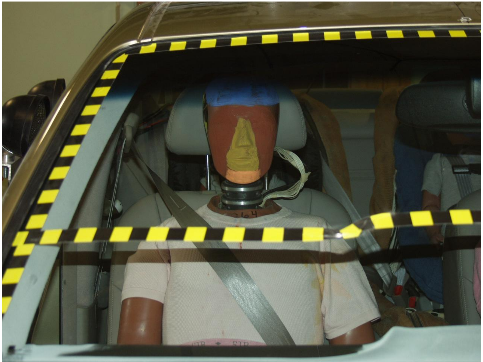
Figure A-44 PRE-TEST PASSENGER HEAD LOCATION
