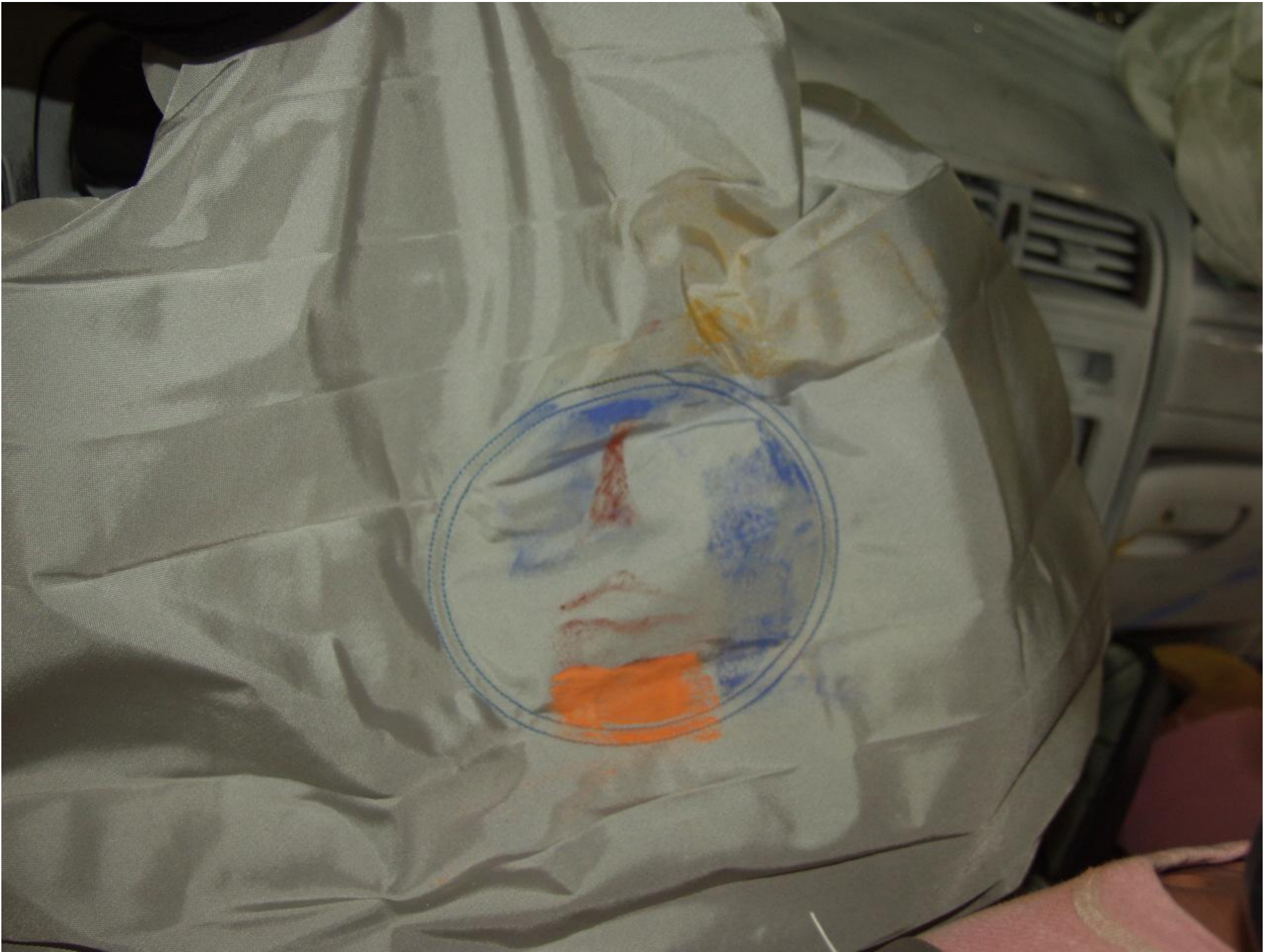
Figure A-43 POST-TEST DRIVER CONTACT TO AIRBAG
