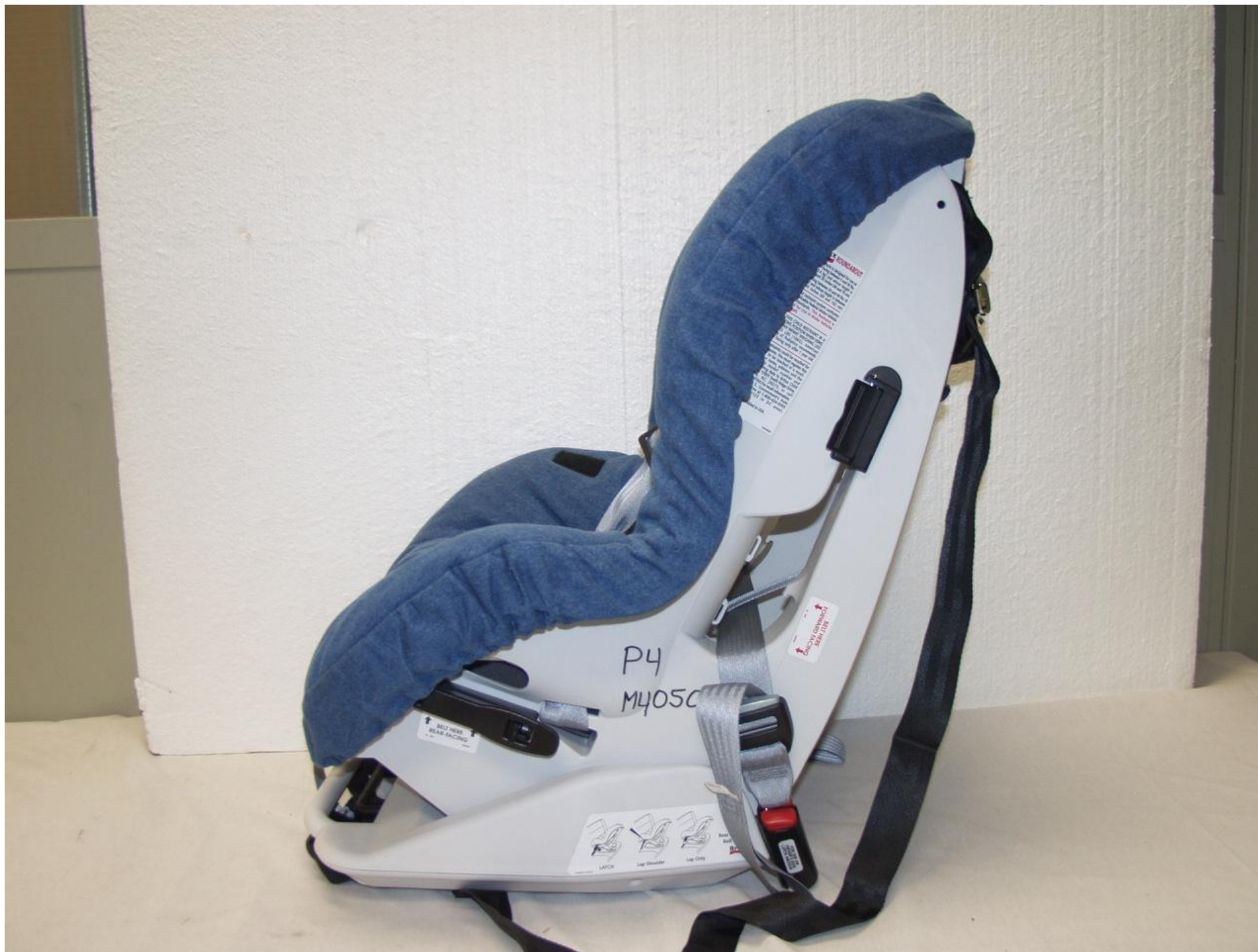
Figure 3-16 POST-TEST LEFT SIDE VIEW OF POSITION 4 CRS
