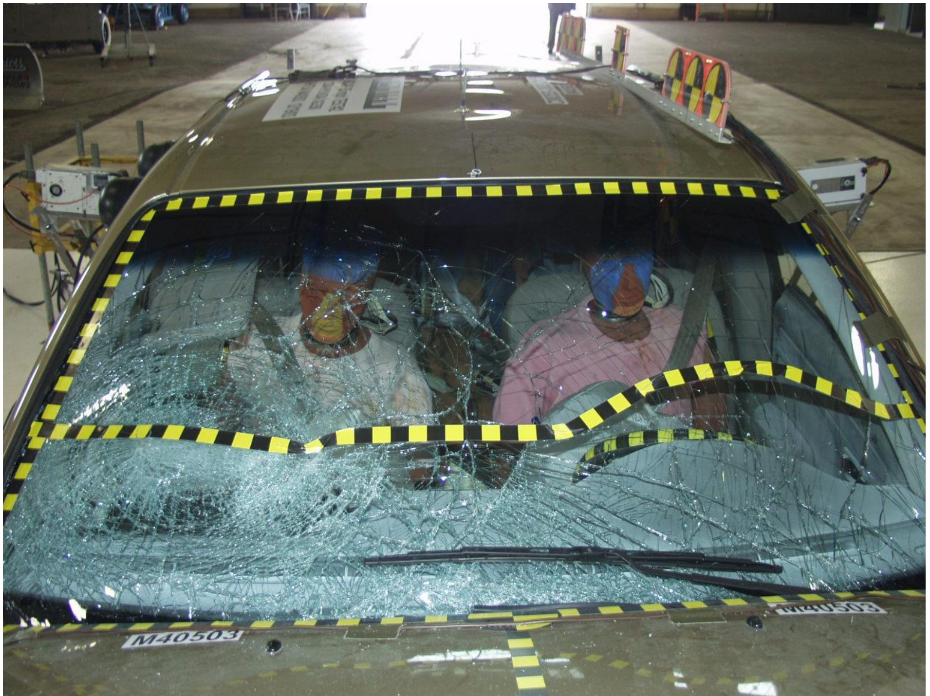
Figure A-19 POST-TEST WINDSHIELDVIEW
