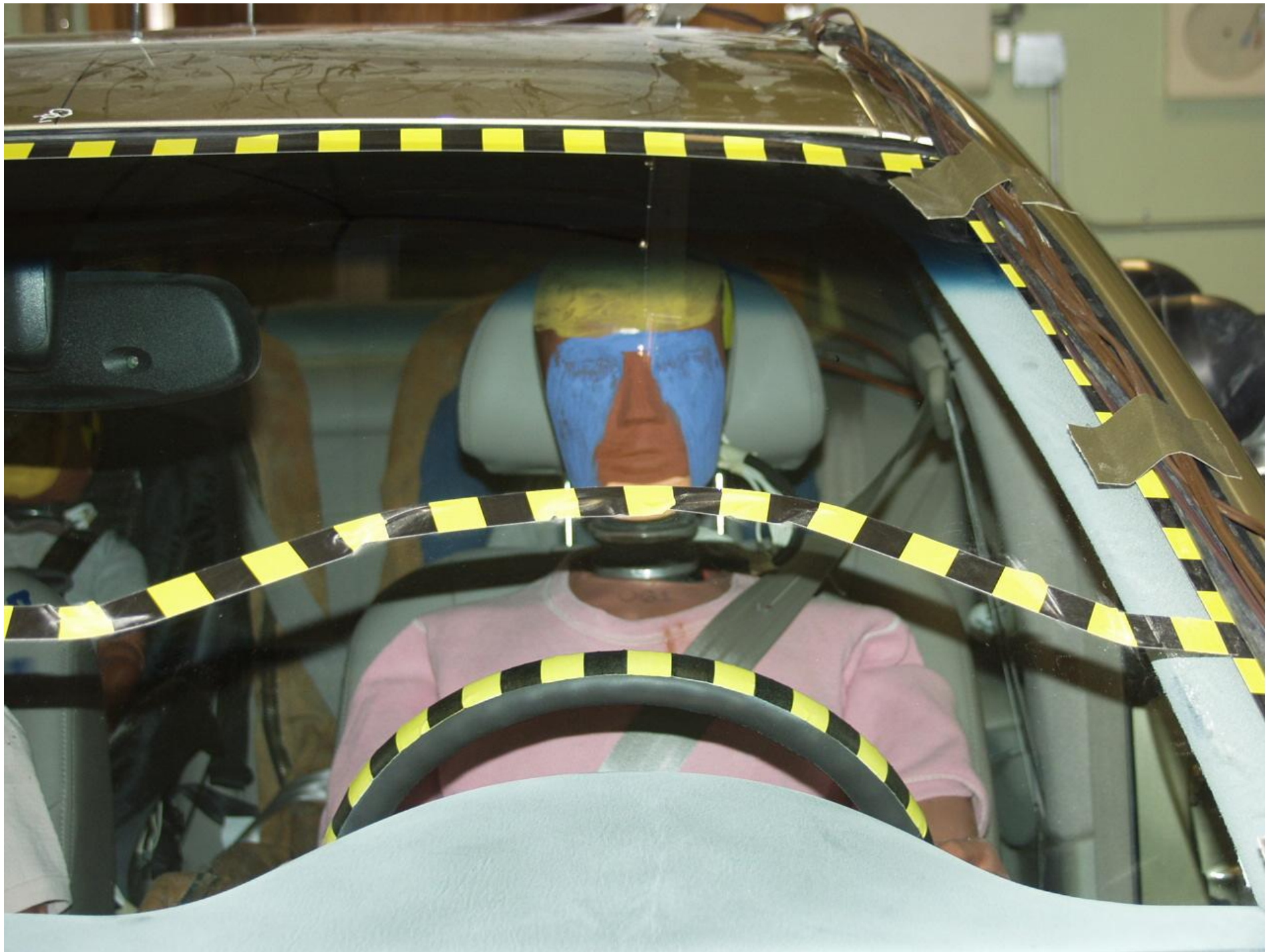
Figure A-30 PRE-TEST DRIVER HEAD LOCATION
