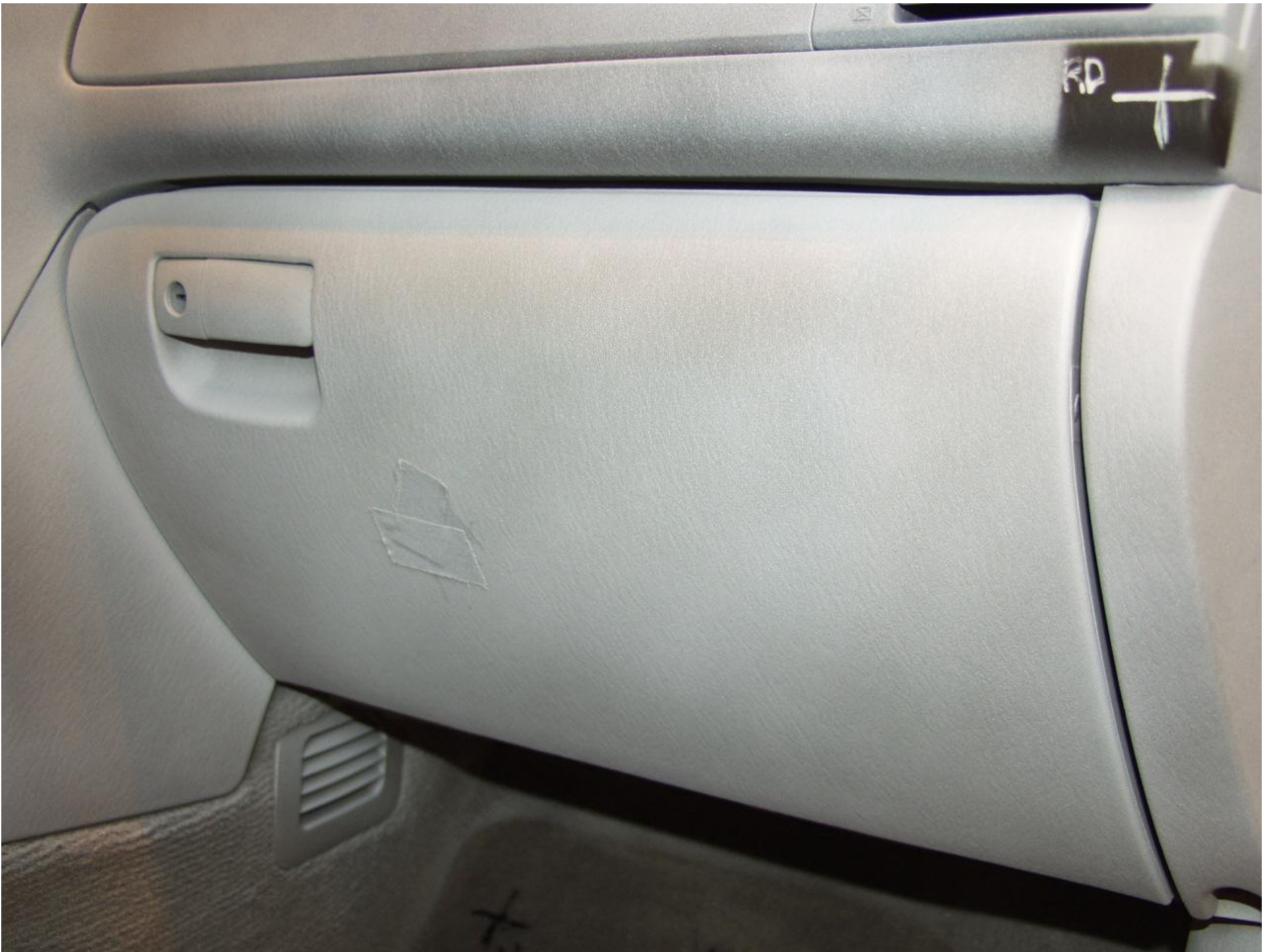
Figure A-52 PRE-TEST PASSENGER KNEE BOLSTER VIEW
