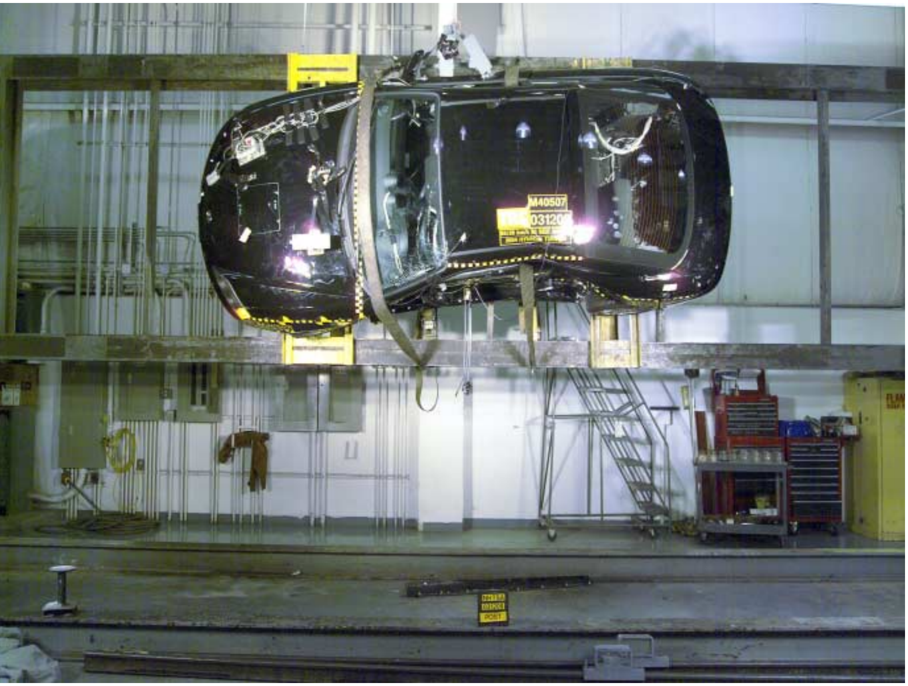
Figure A-44 FMVSS 301 Rollover View at 90°
