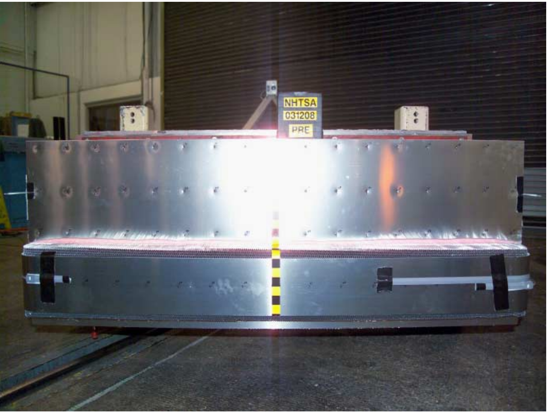
Figure A-17 Pre-Test View of MDB Showing Contact Switches in Place
