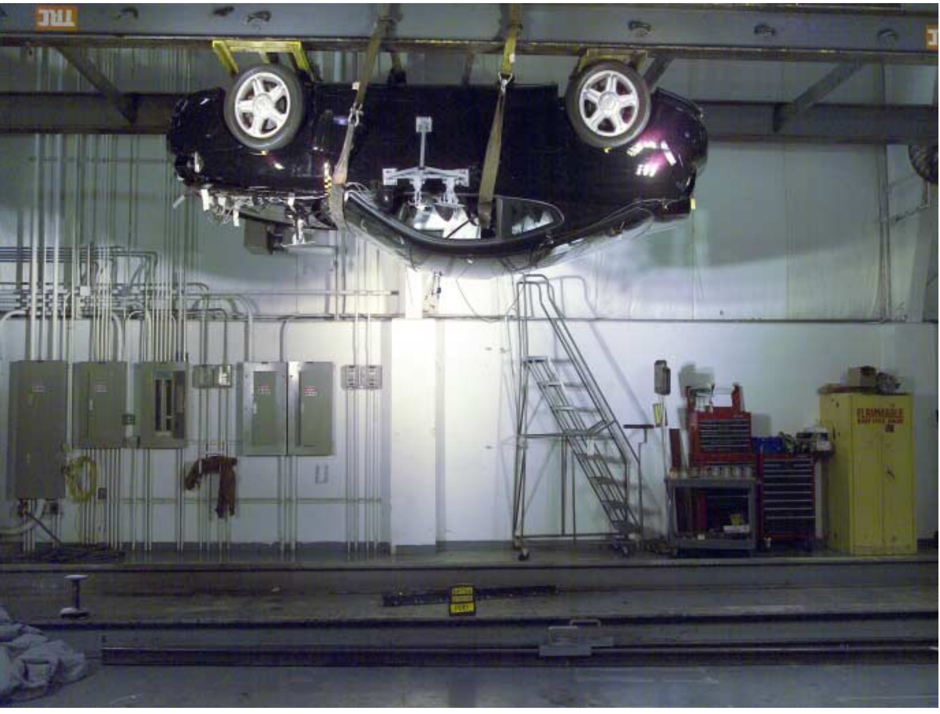
Figure A-45 FMVSS 301 Rollover View at 180°
