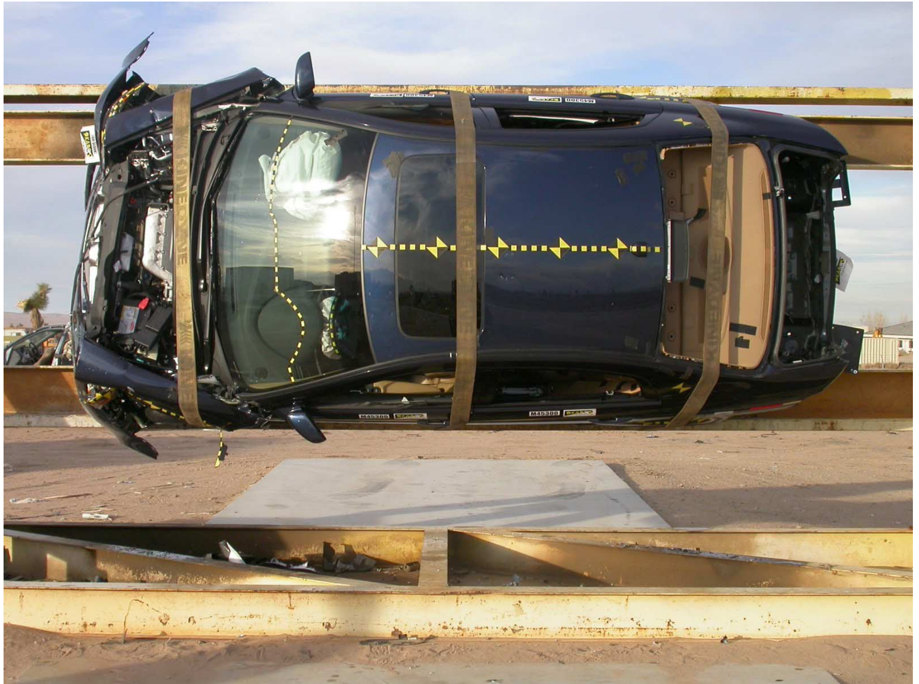
Figure A-59: Vehicle on Rollover Device
