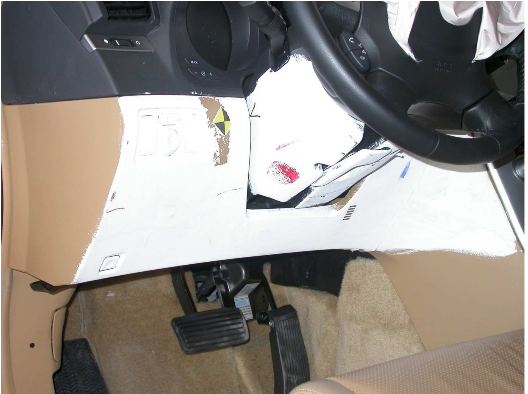
Figure A-39: Post-Test Driver Side Knee Bolster
