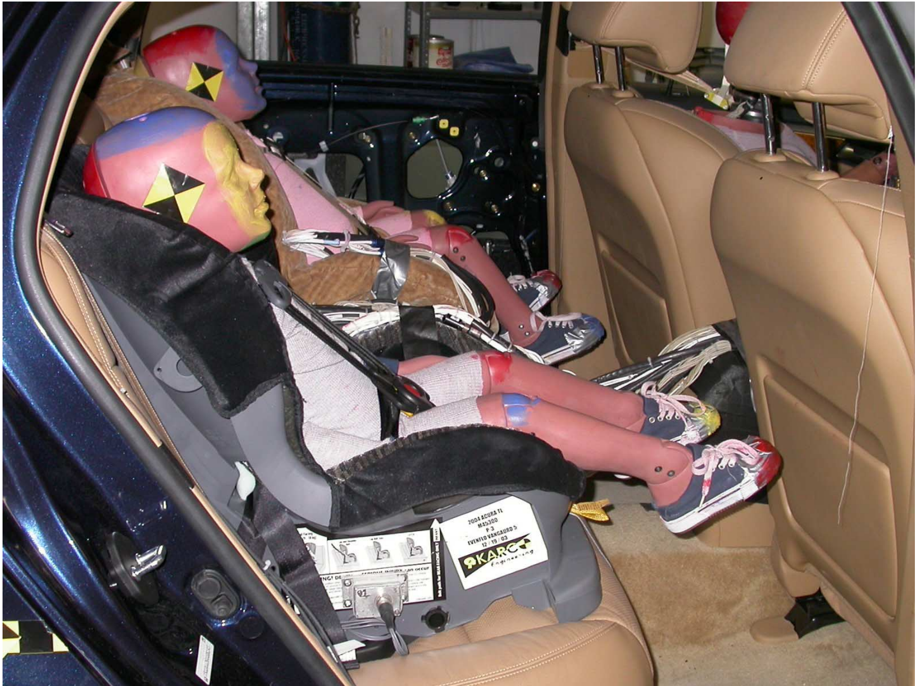
Figure F2-14: Pre-Test Position 3 Right Side View
