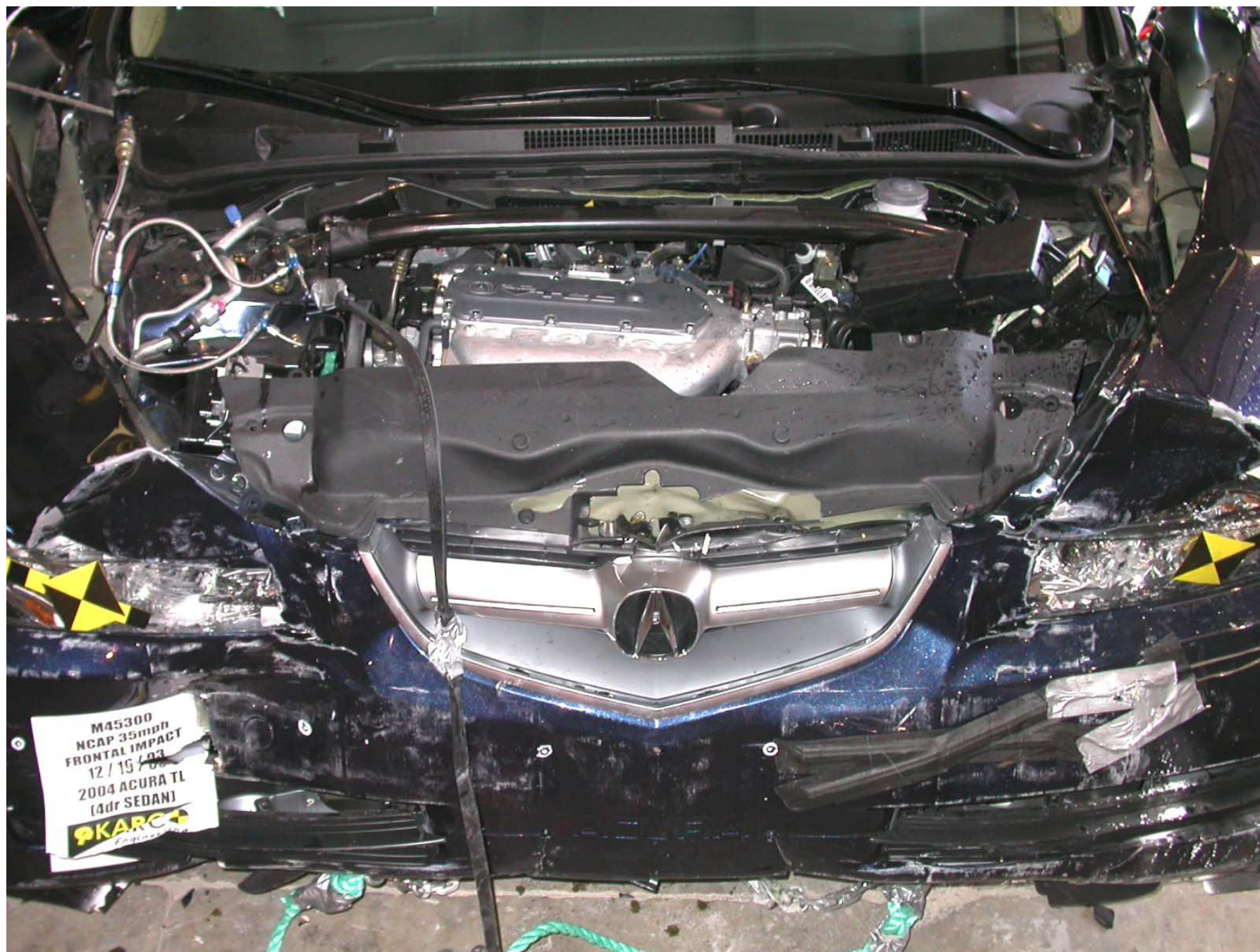
Figure A-21: Post-Test Engine Compartment (Vehicle Moved)
