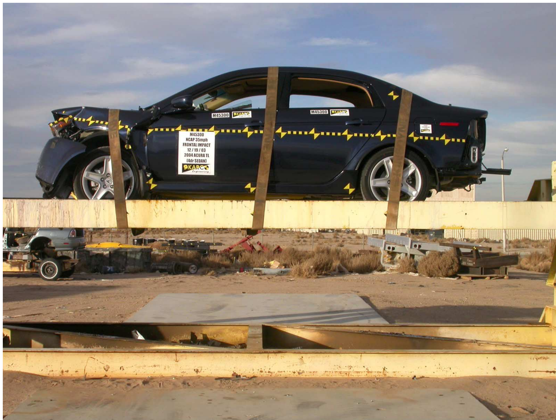
Figure A-58: Vehicle on Rollover Device
