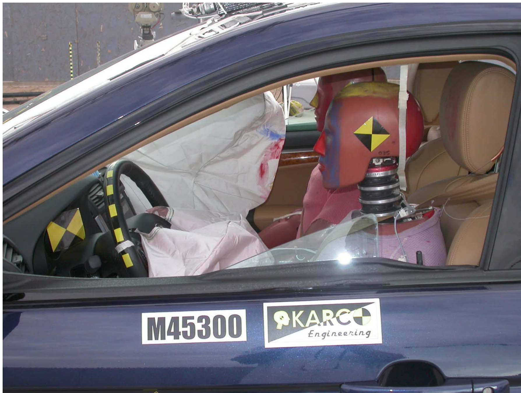
Figure A-33: Post-Test Driver Dummy Front Through Window
