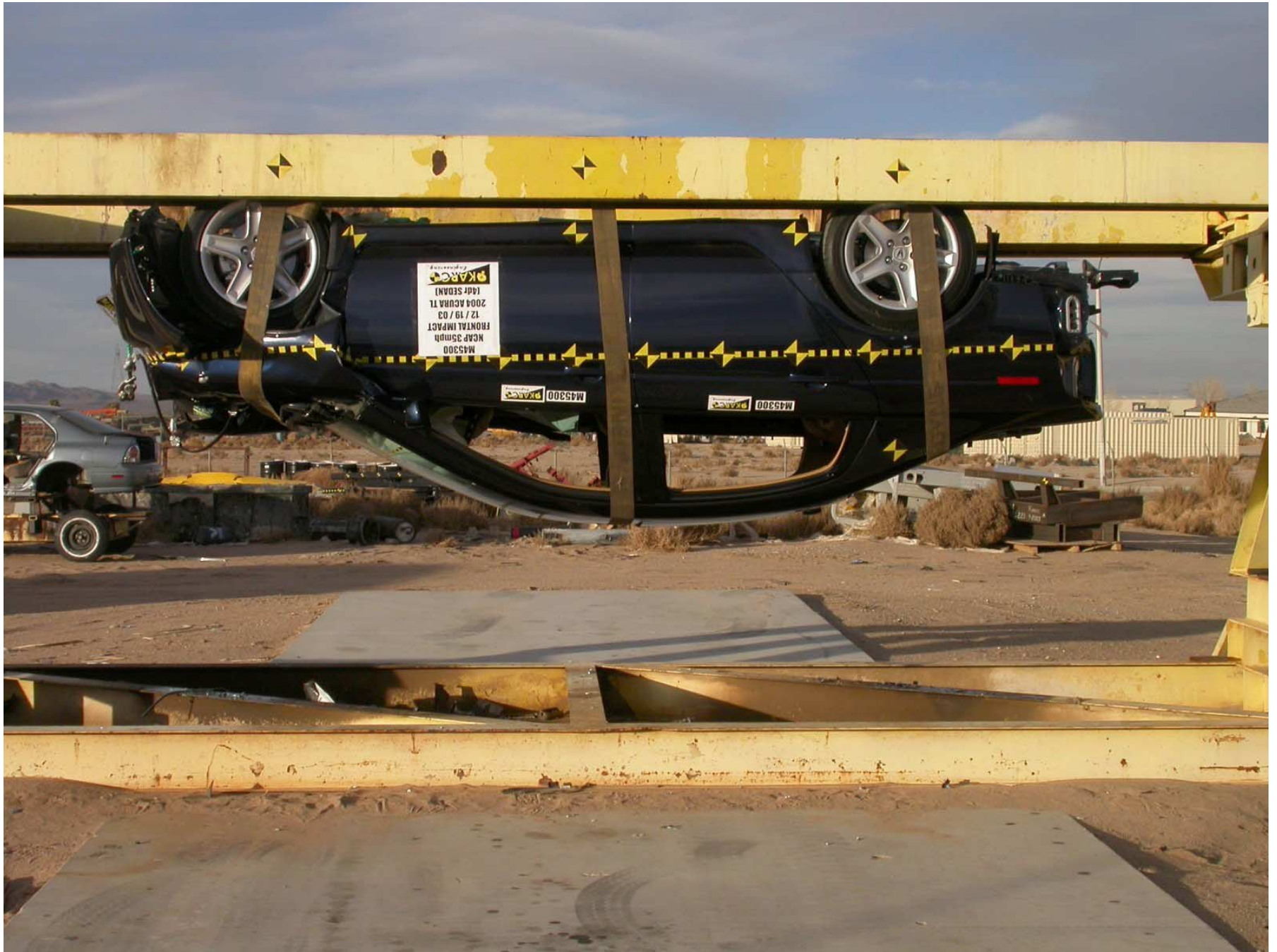
Figure A-60: Vehicle on Rollover Device
