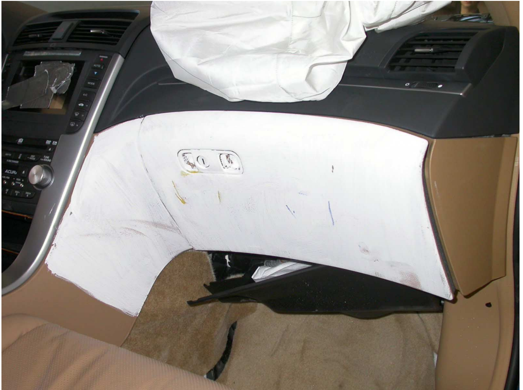
Figure A-53: Post-Test Passenger Side Knee Bolster
