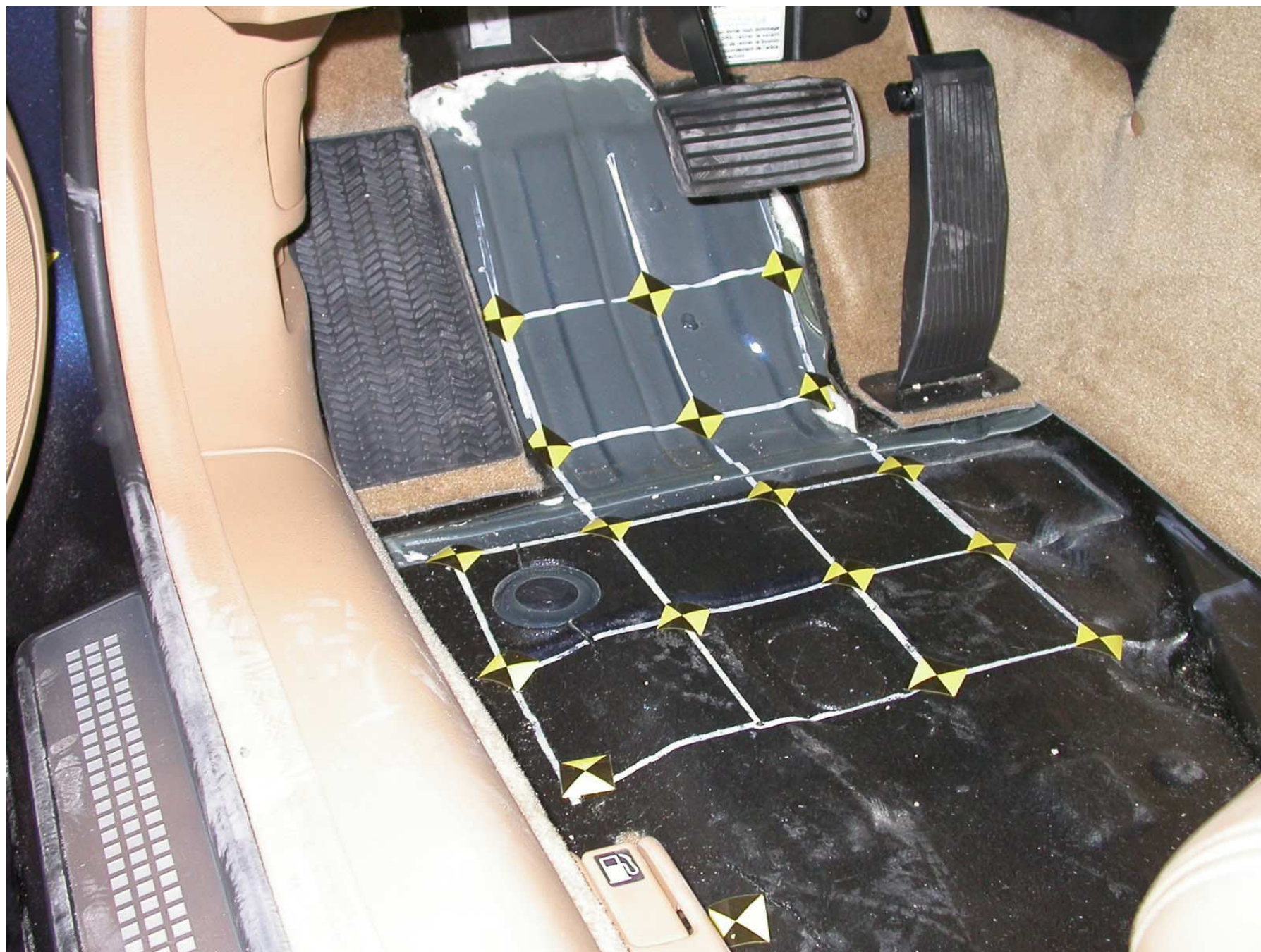
Figure A-40: Pre-Test Driver Side Floor Pan
