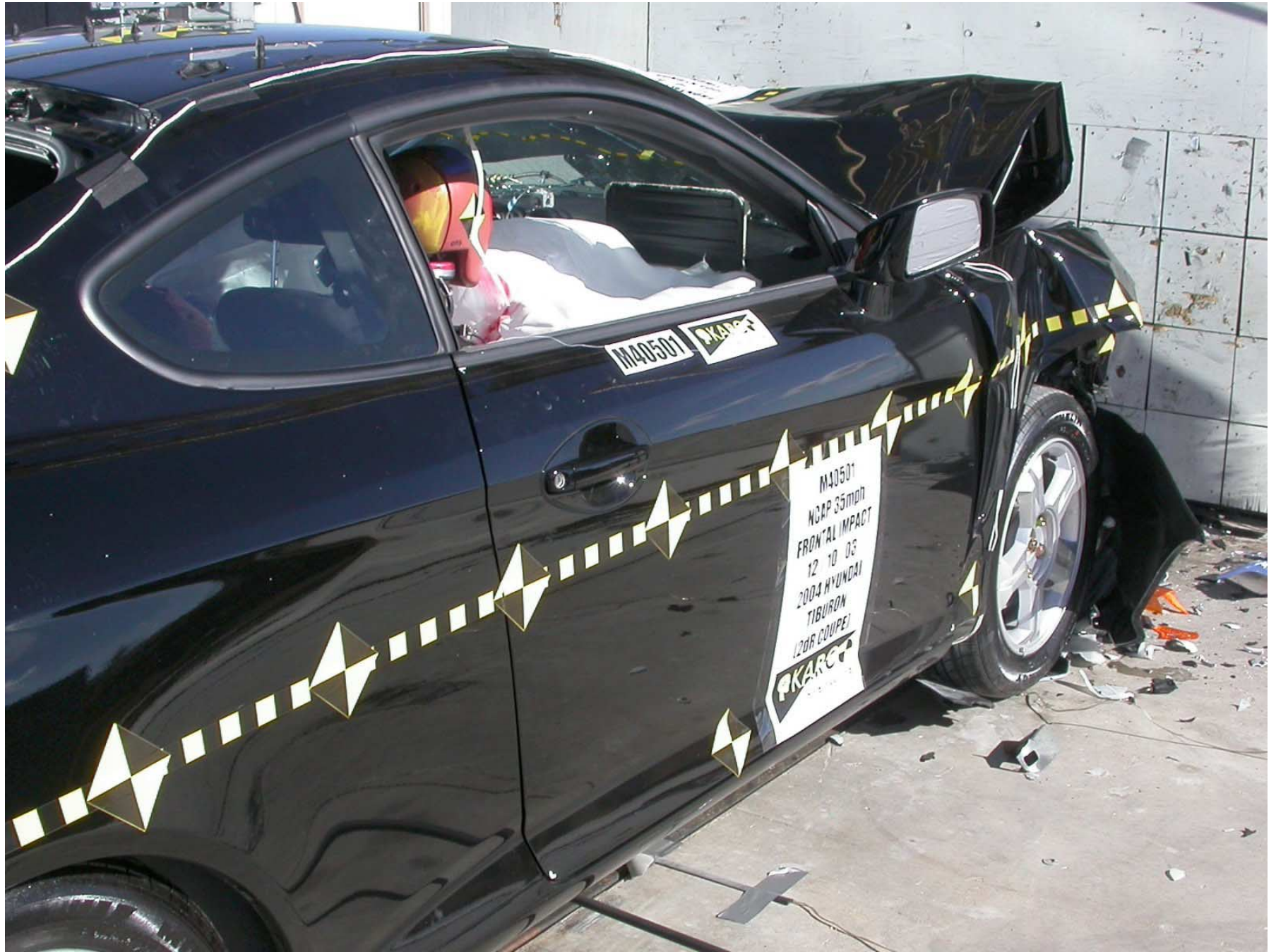
Figure A-17: Right Rear 3/4 View of Doors After Impact
