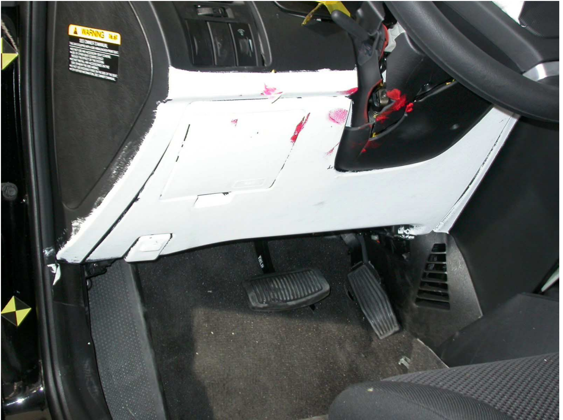
Figure A-39: Post-Test Driver Side Knee Bolster
