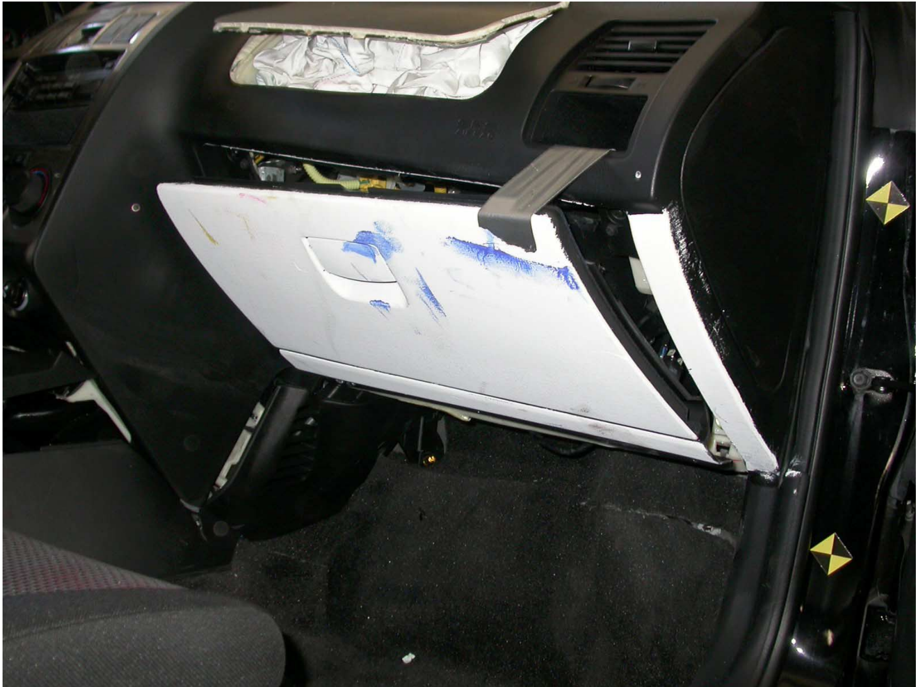
Figure A-53: Post-Test Passenger Side Knee Bolster
