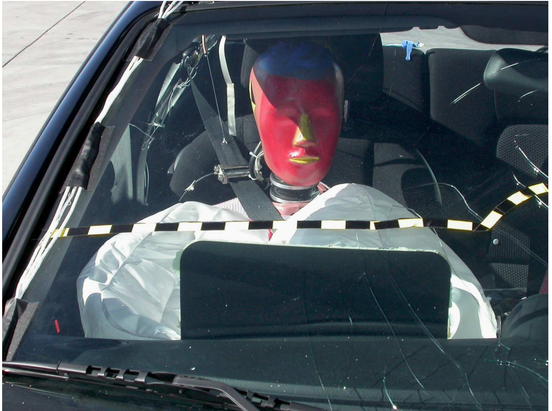
Figure A-45: Post-Test Passenger Dummy Front View (Head Position)
