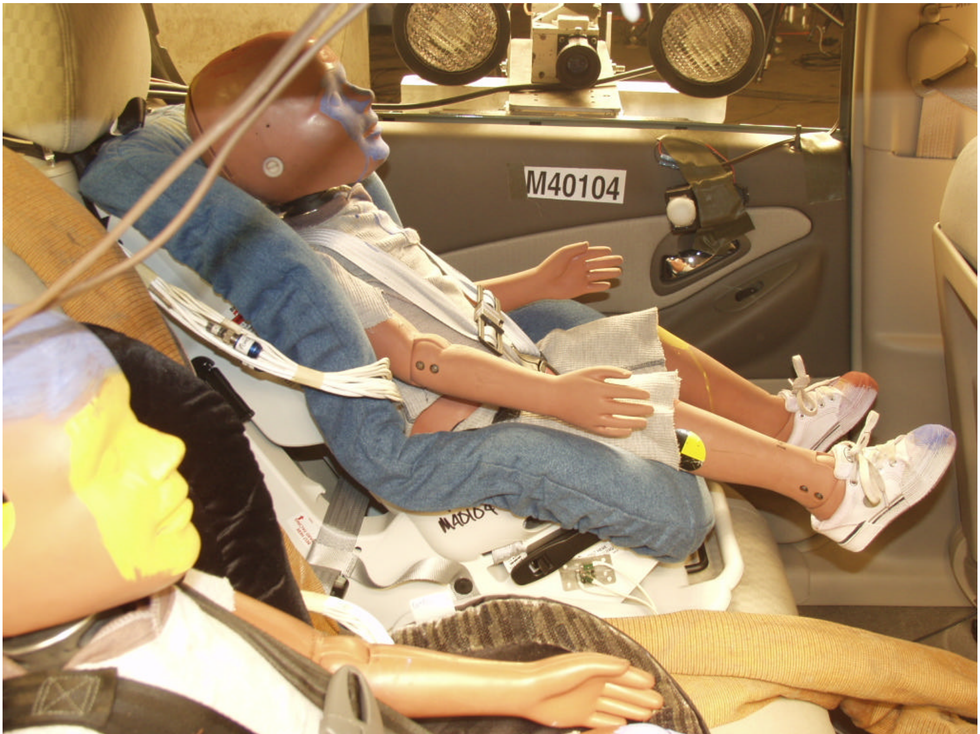
Figure 3-26 POST-TEST POSITION 4 RIGHT SIDE VIEW
