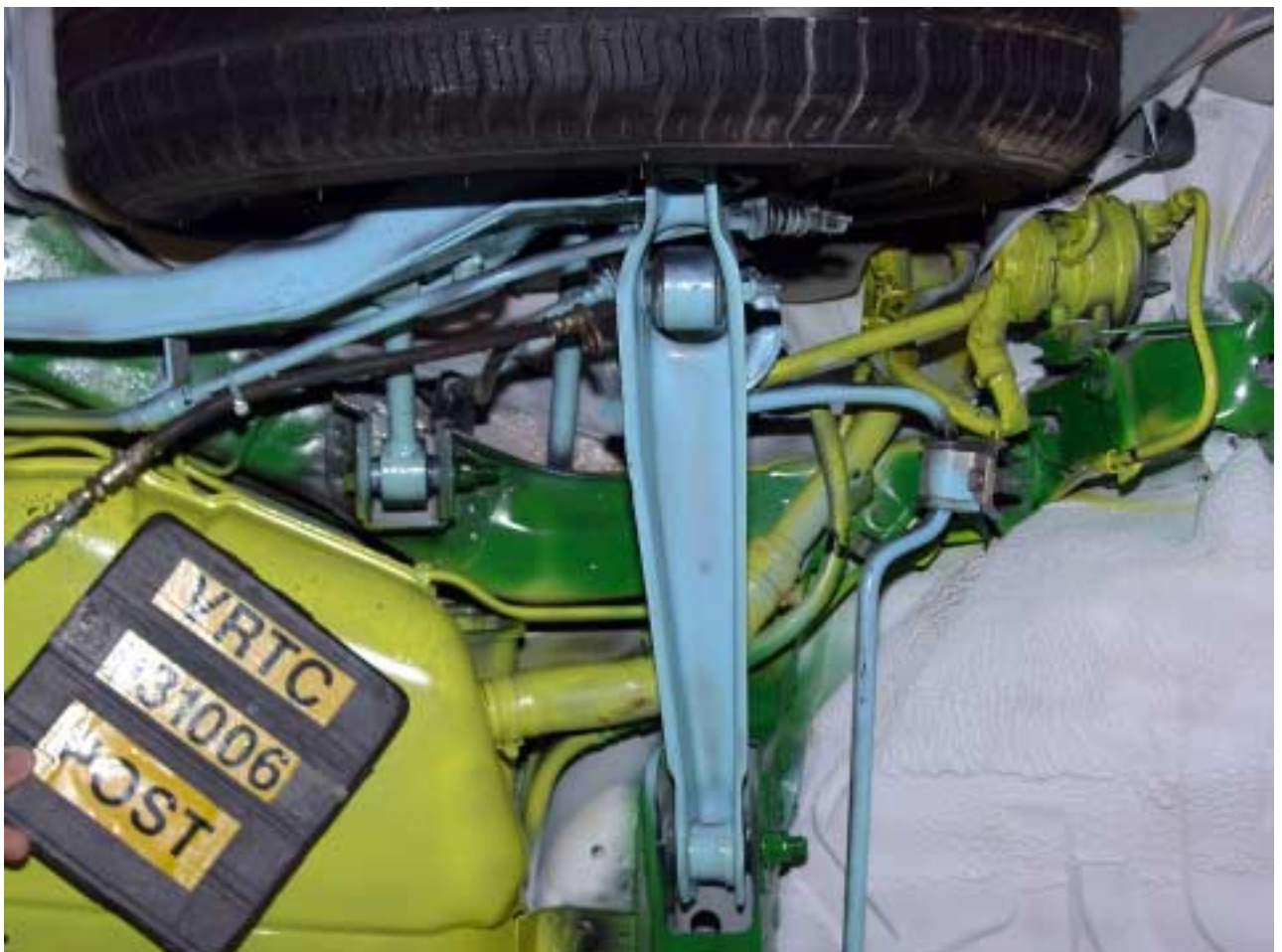
Figure A-34 Post-Test Fuel Filler Neck View
