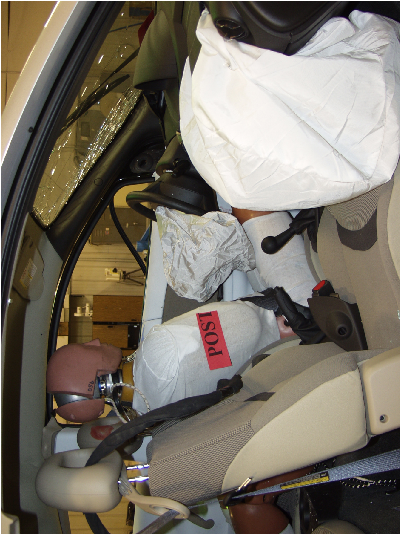
Figure A-18: POST-TEST RIGHT OCCUPANT COMPARTMENT VIEW OF FRONT SID (SID H3 SKIN FELL OFF DURING IMPACT)
