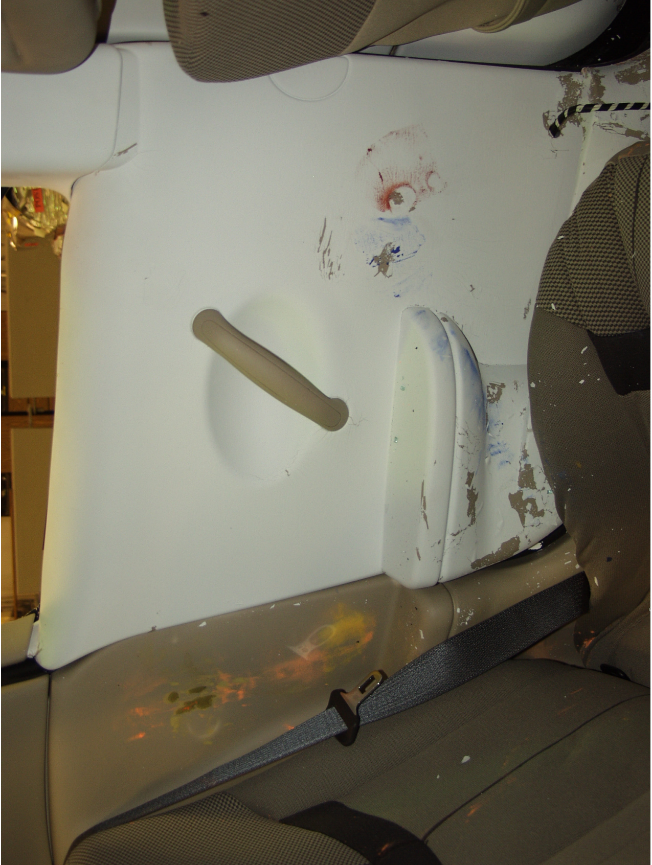
Figure A-30: POST-TEST INTERIOR OF REAR DOOR SHOWING SID H3 IMPACT LOCATIONS 2
