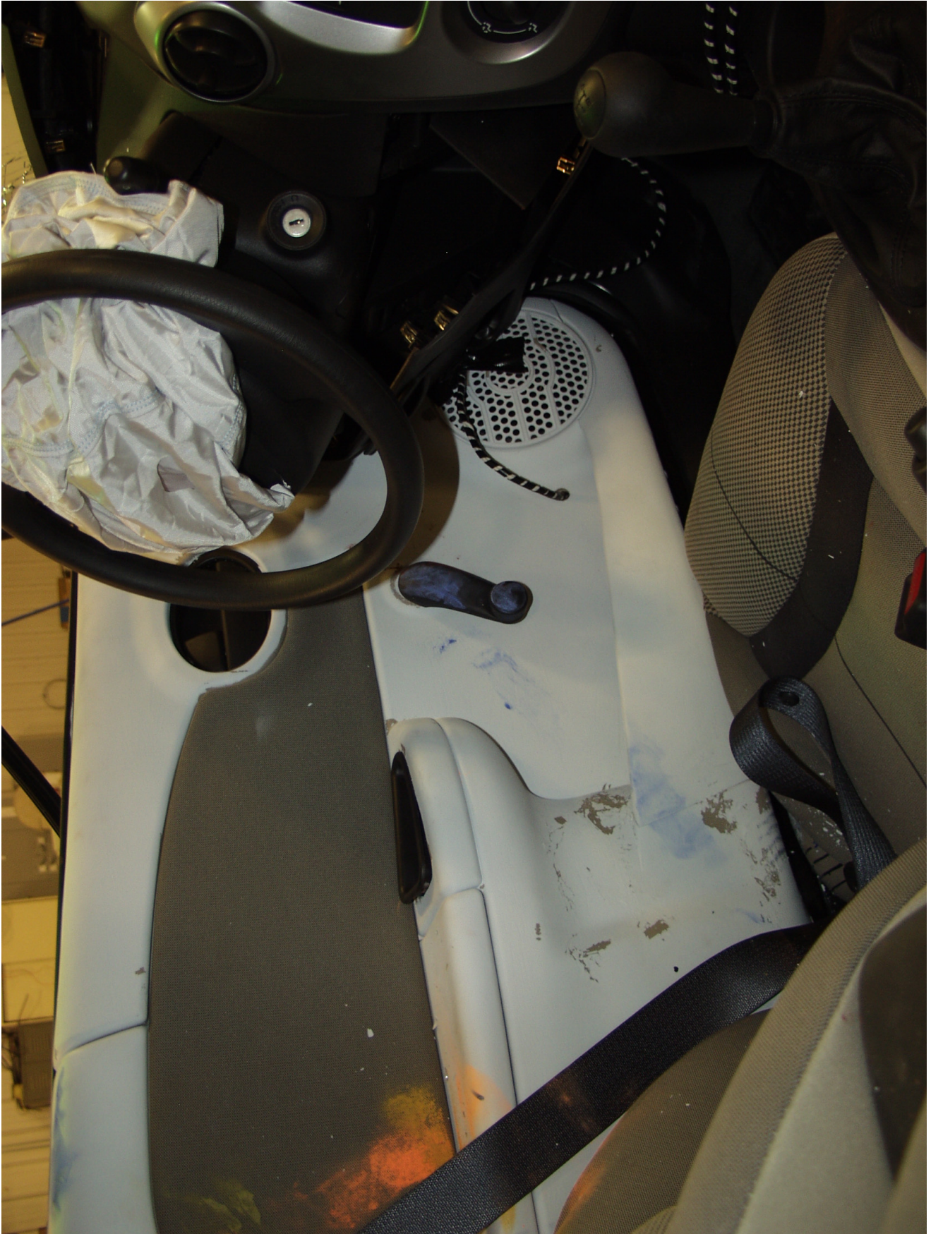
Figure A-26: POST-TEST INTERIOR OF FRONT DOOR SHOWING SID H3 IMPACT LOCATIONS
