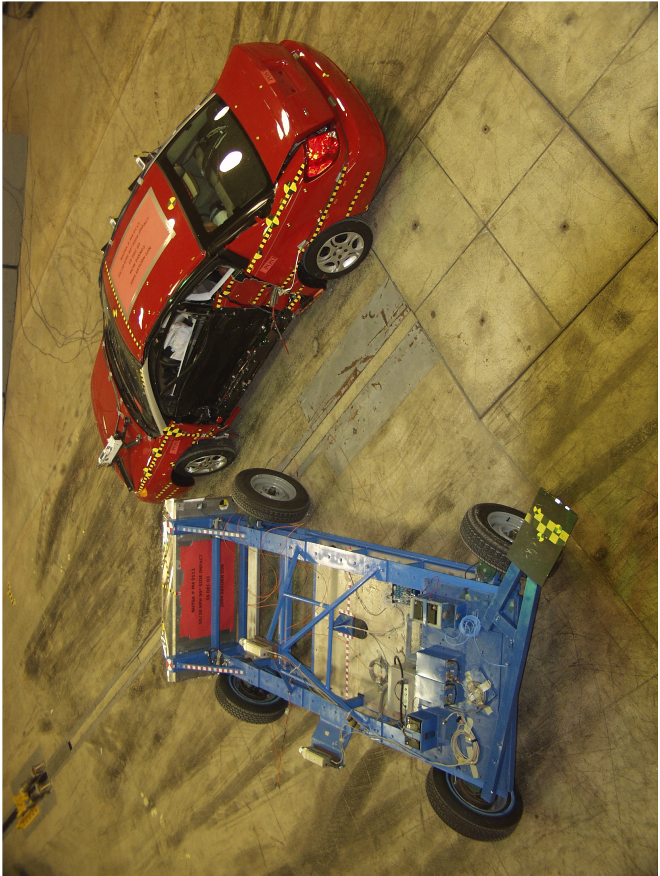
Figure A-36: POST-TEST OVERHEAD VIEW OF MDB (TRUNK OPENED POST TEST TO ACCESS DATA)
