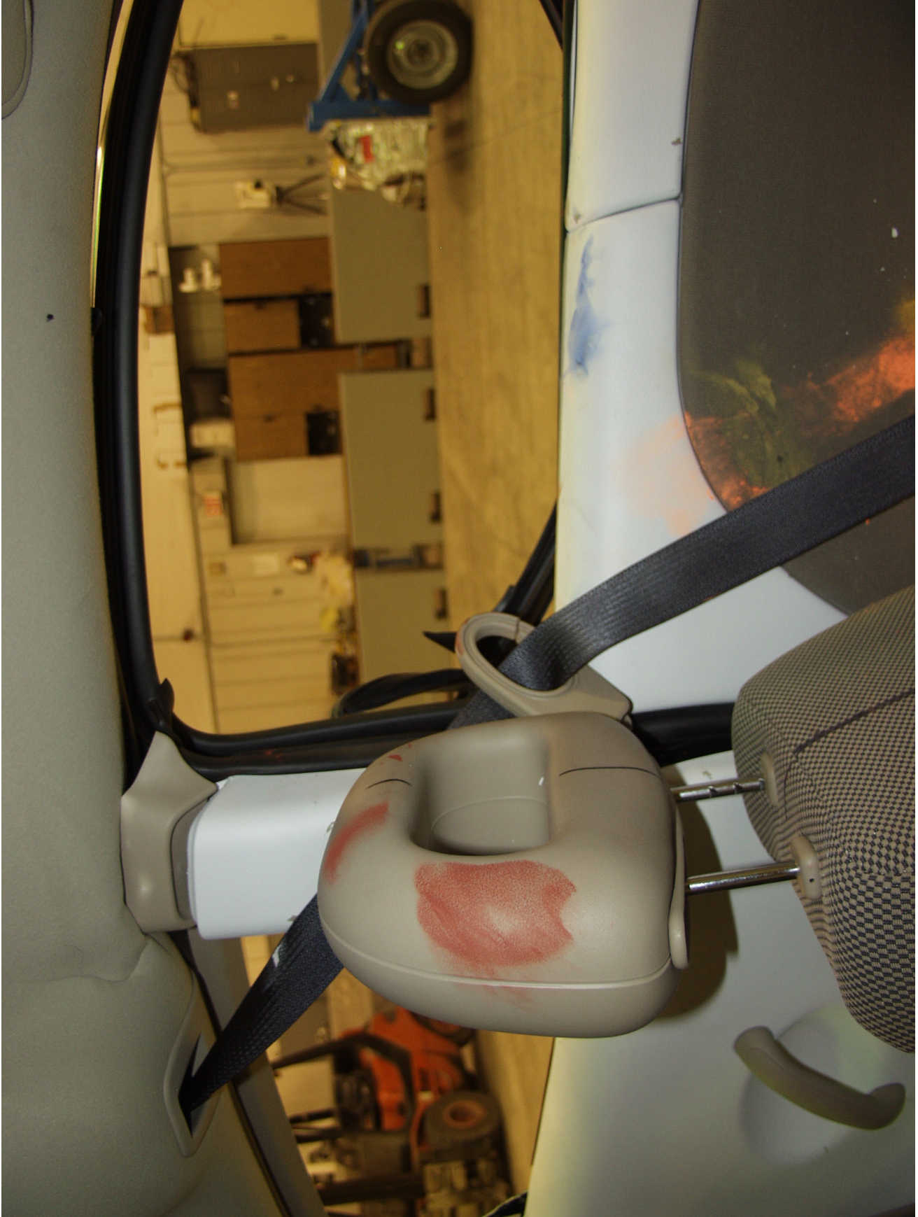
Figure A-27: POST-TEST INTERIOR OF FRONT DOOR SHOWING SID H3 IMPACT LOCATIONS 2
