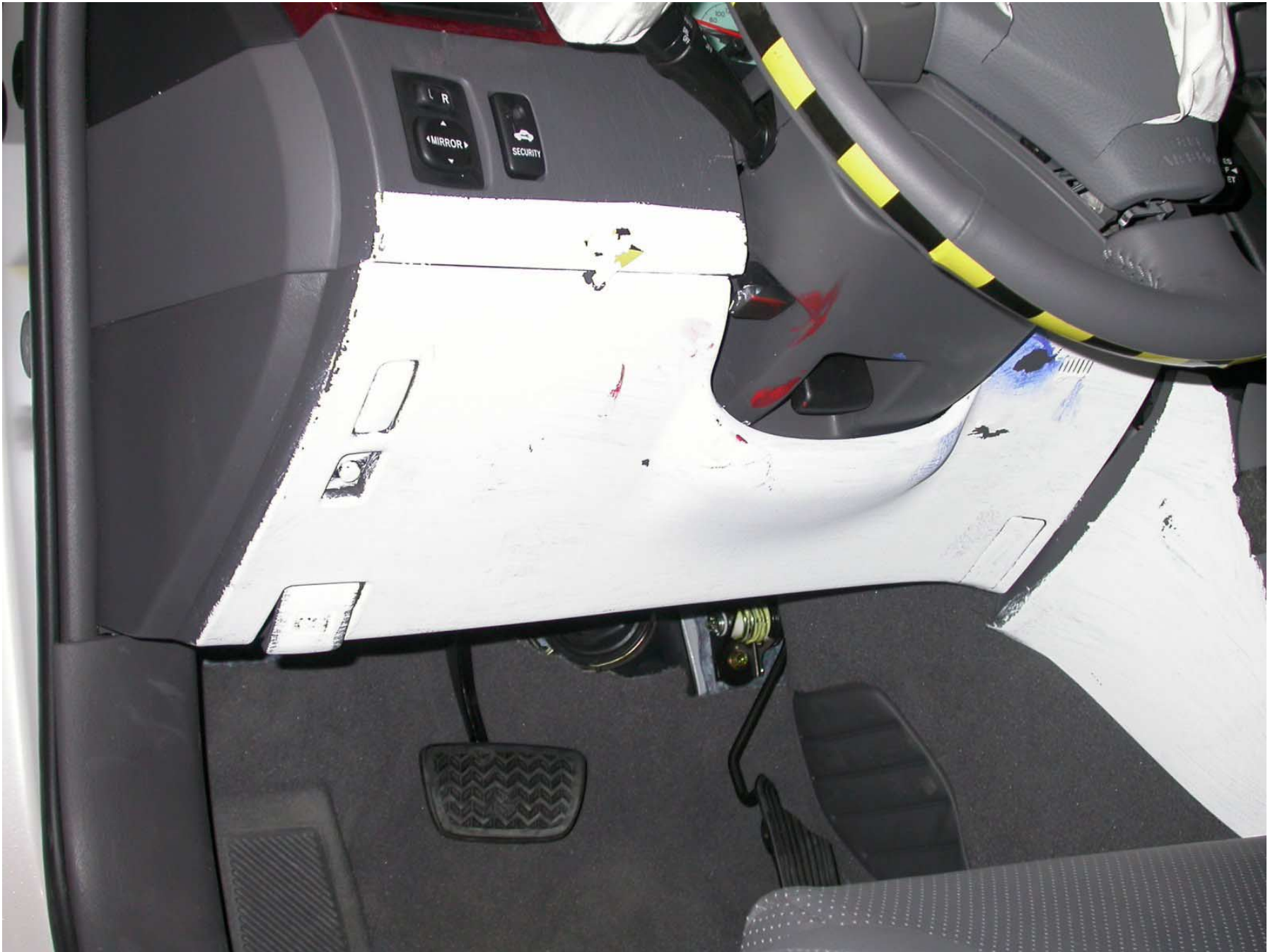
Figure A-39: Post-Test Driver Side Knee Bolster
