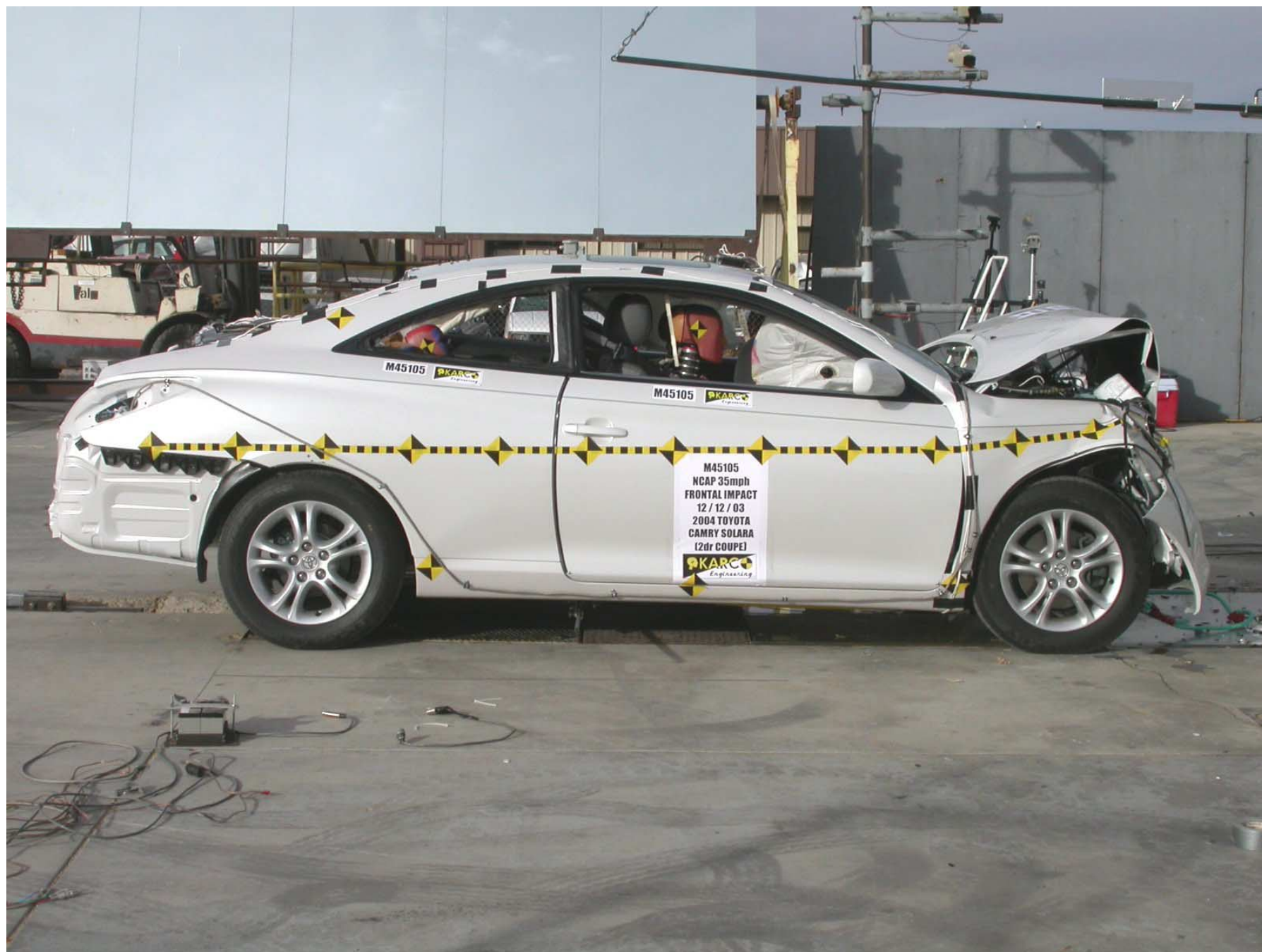
Figure A-11: Post-Test Right Side View
