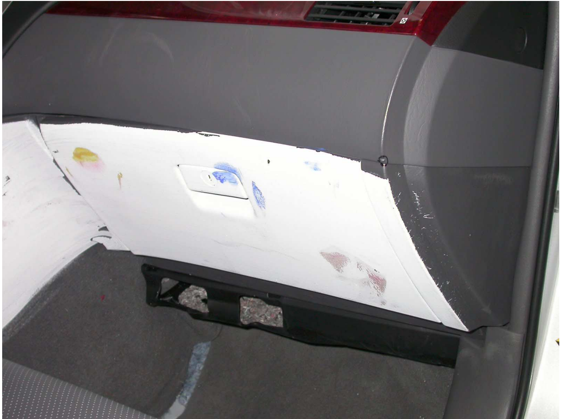
Figure A-53: Post-Test Passenger Side Knee Bolster
