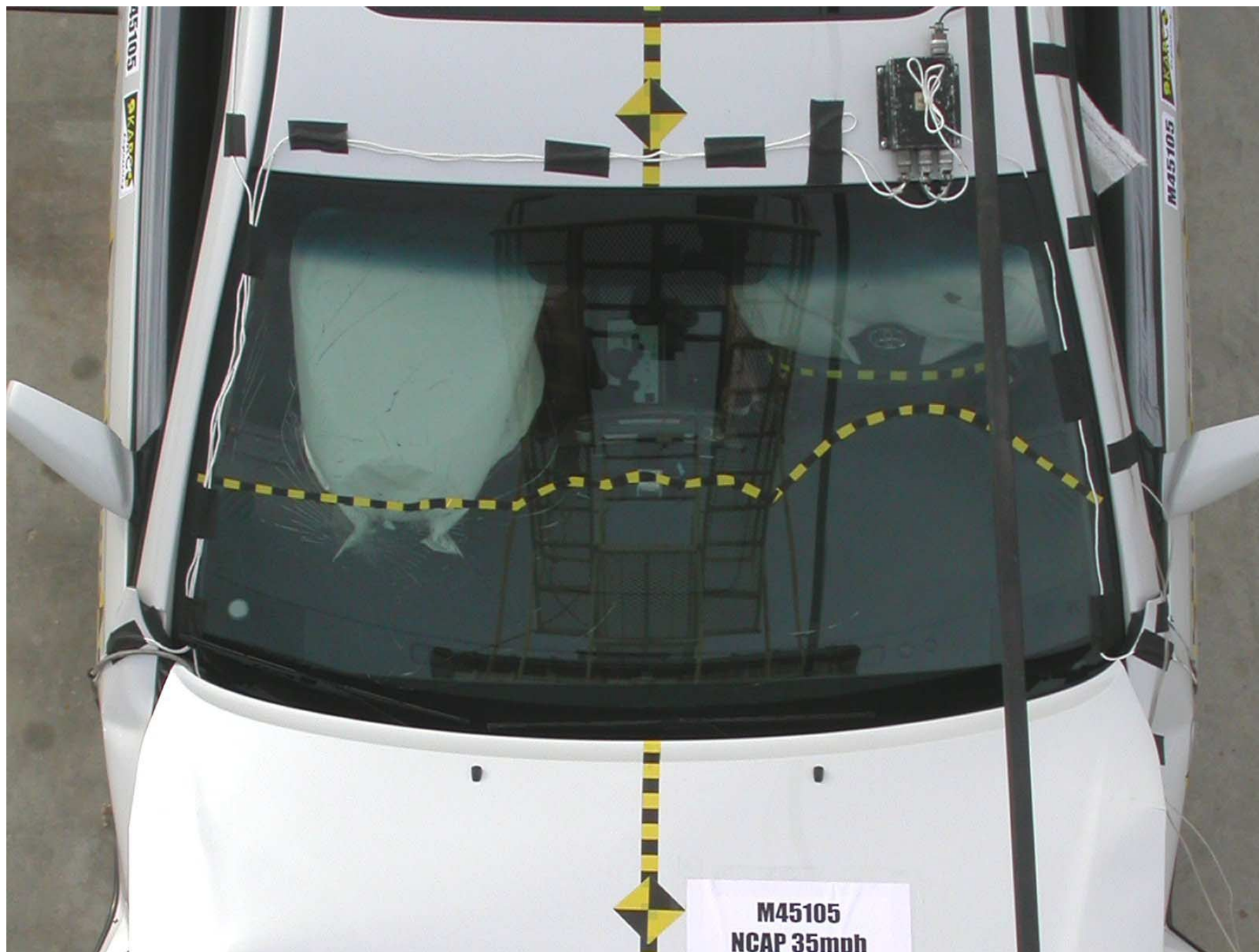
Figure A-19: Post-Test Windshield View
