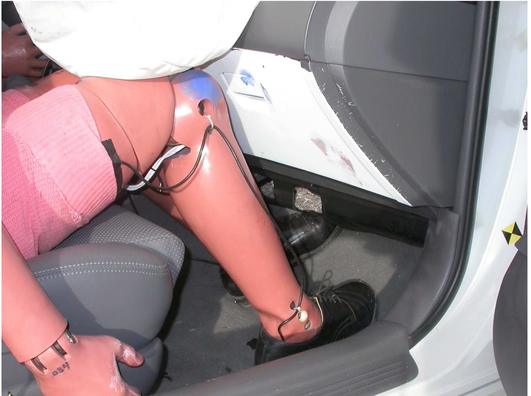
Figure A-51: Post-Test Passenger Dummy Feet
