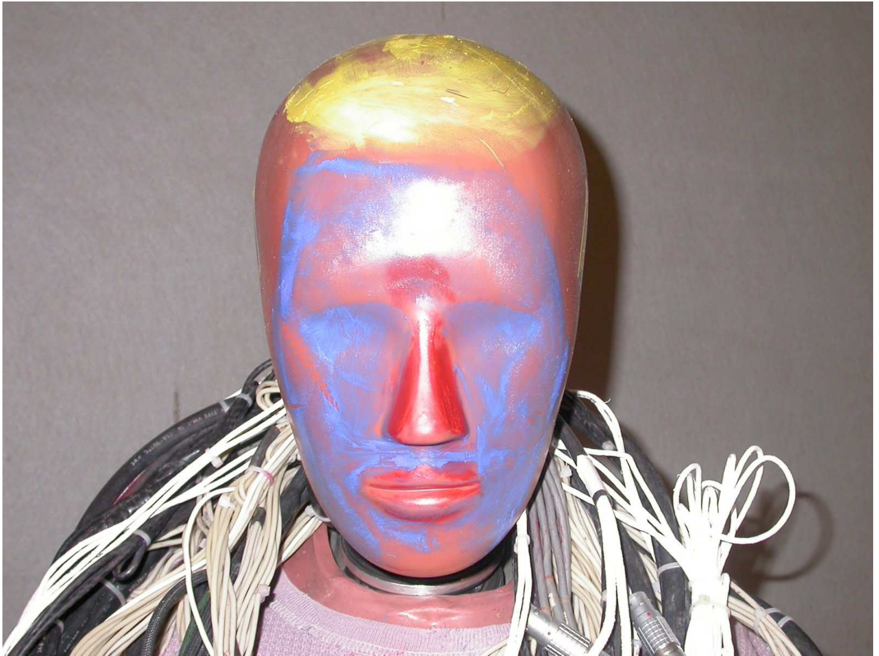
Figure A-42: Post-Test Driver Dummy Head
