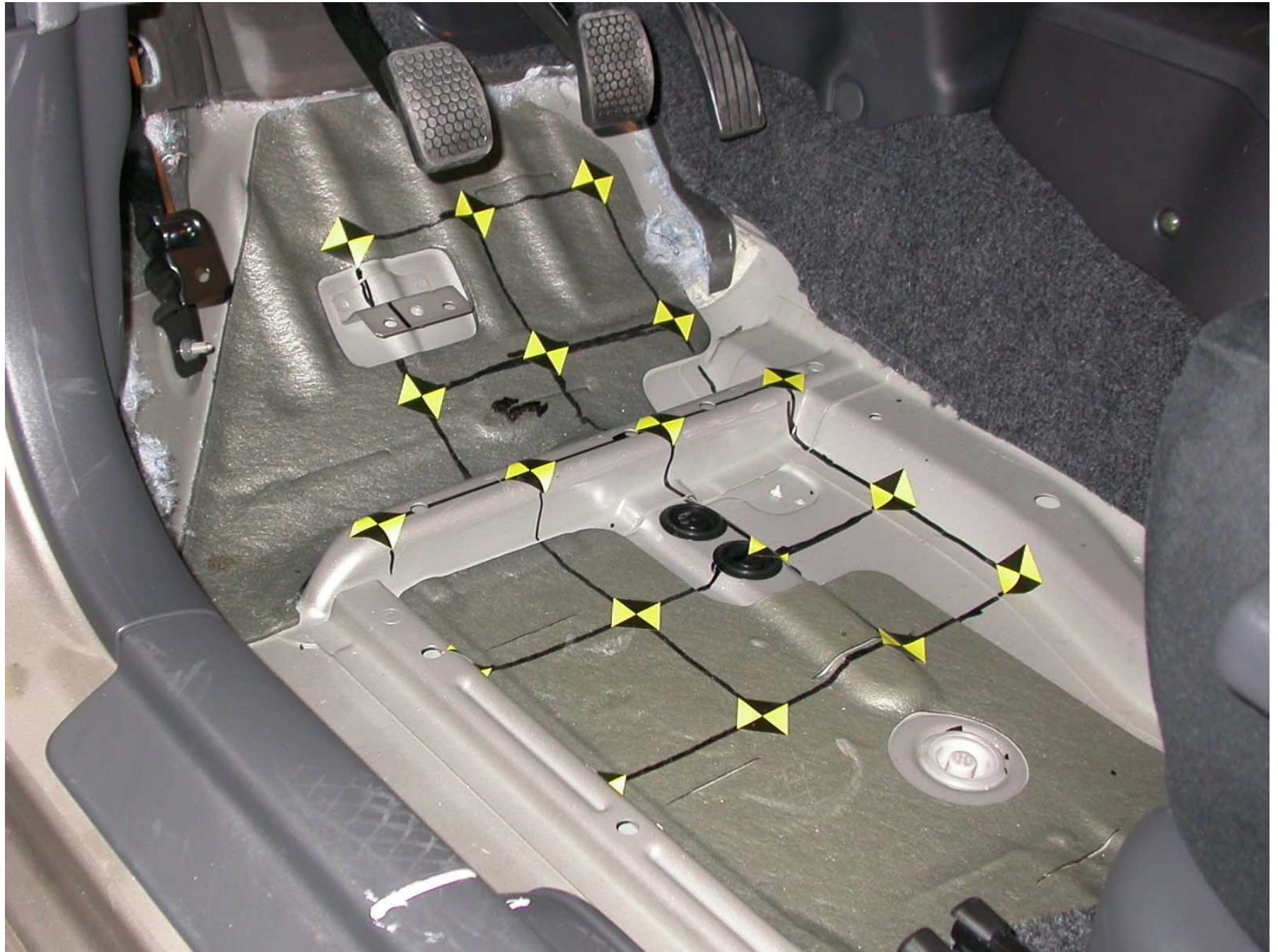
Figure A-40: Pre-Test Driver Side Floor Pan
