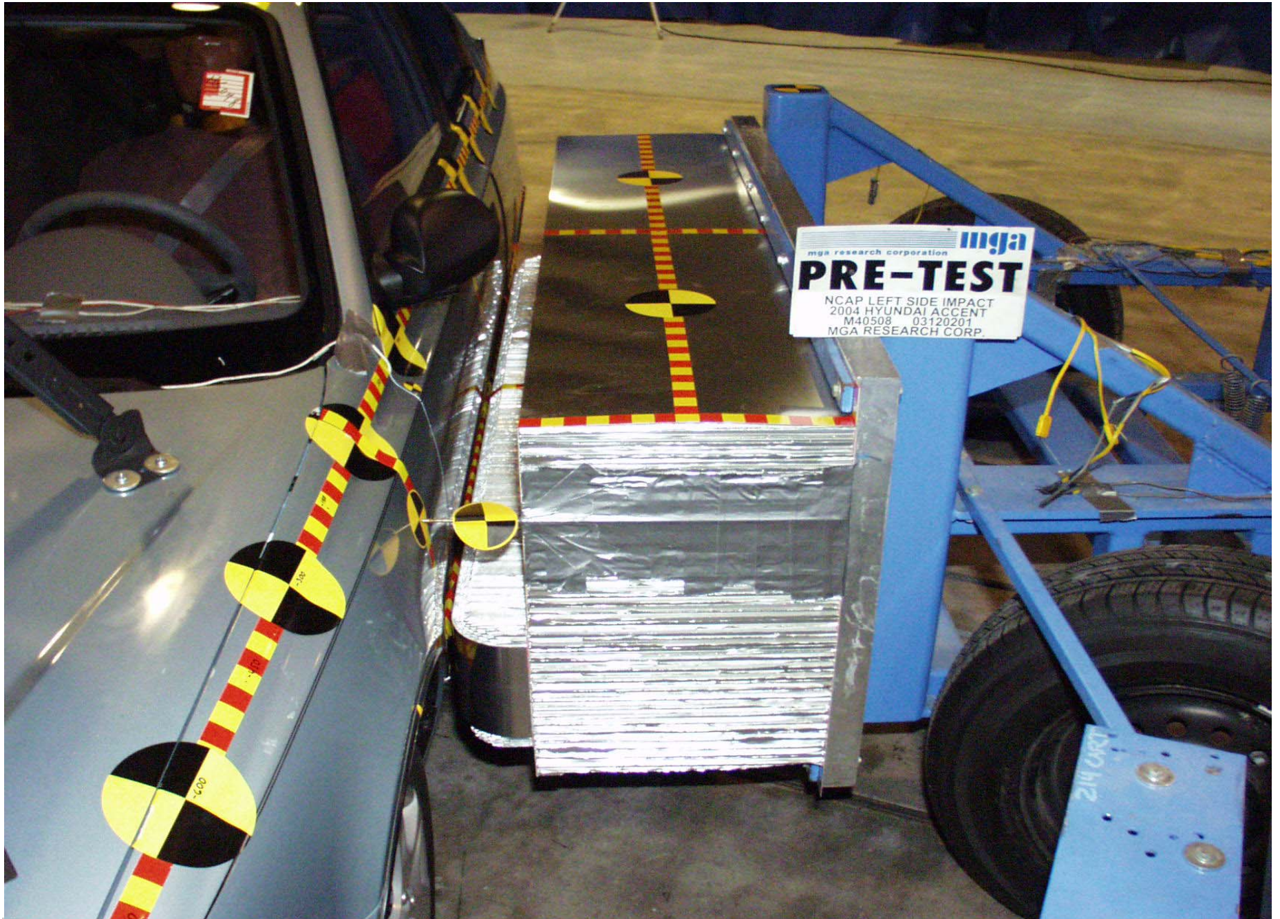
Pre-Test MDB Positioned Against Vehicle (left side)
