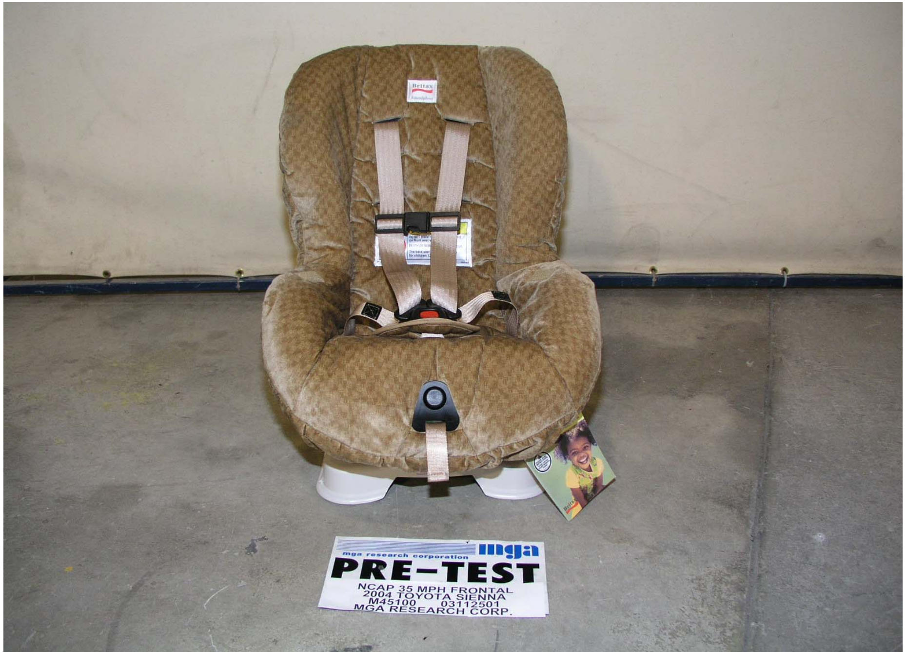
Pre-Test Front View of Position 4 CRS
