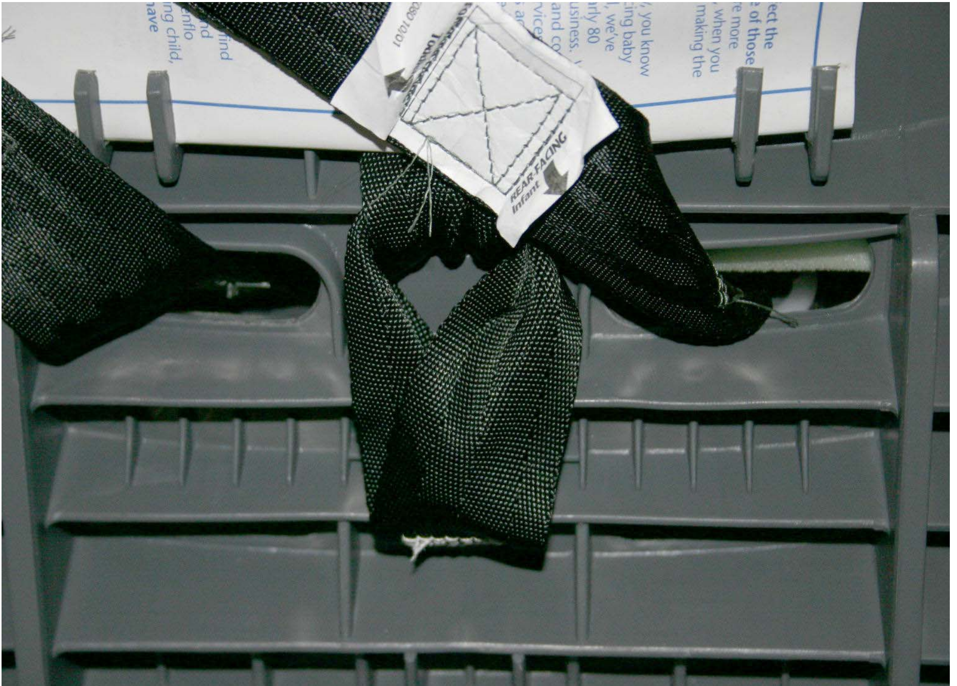
Post-Test Stress Marks on Position 3 CRS
