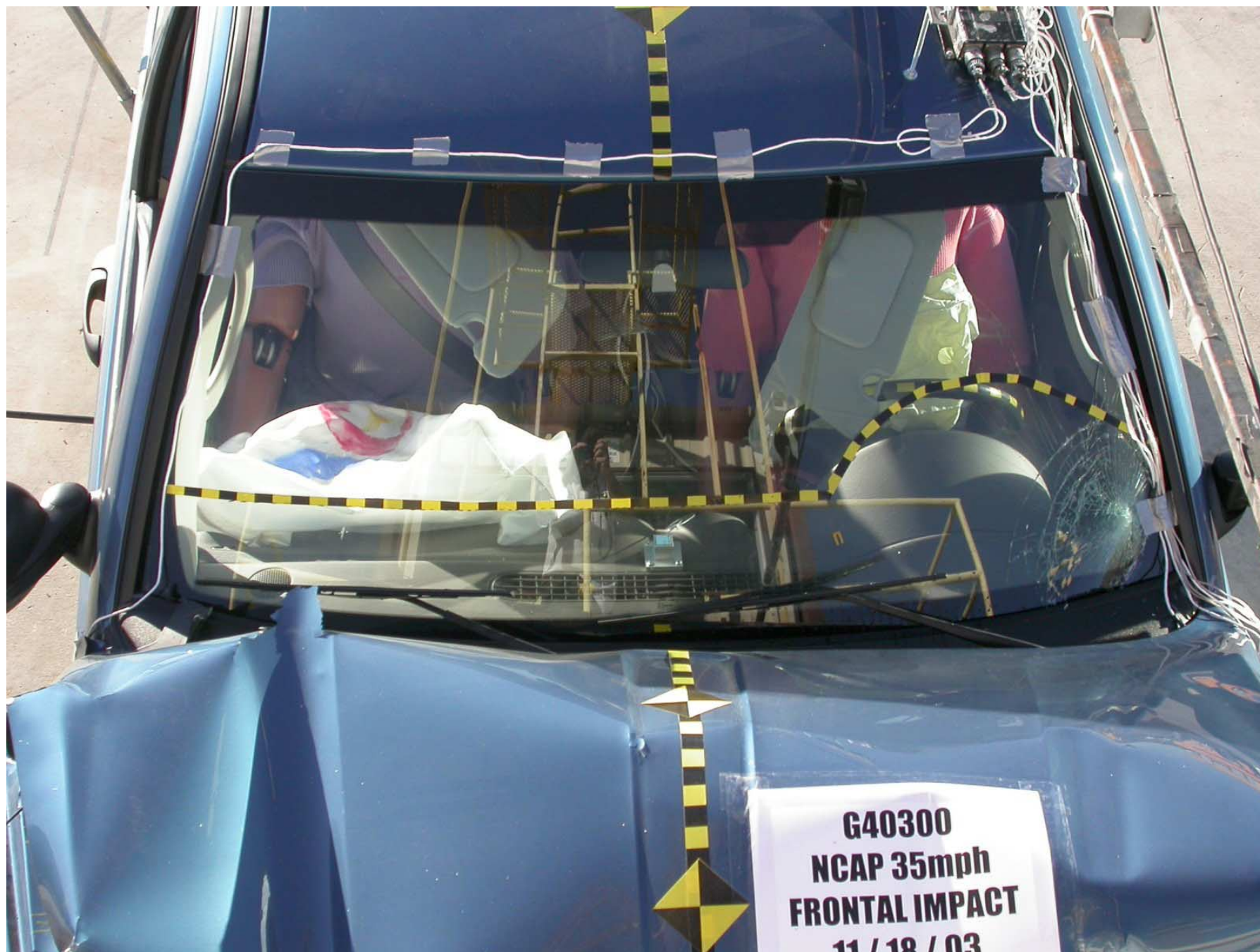
Figure A-19: Post-Test Windshield View (Correct NHTSA # is M40300)
