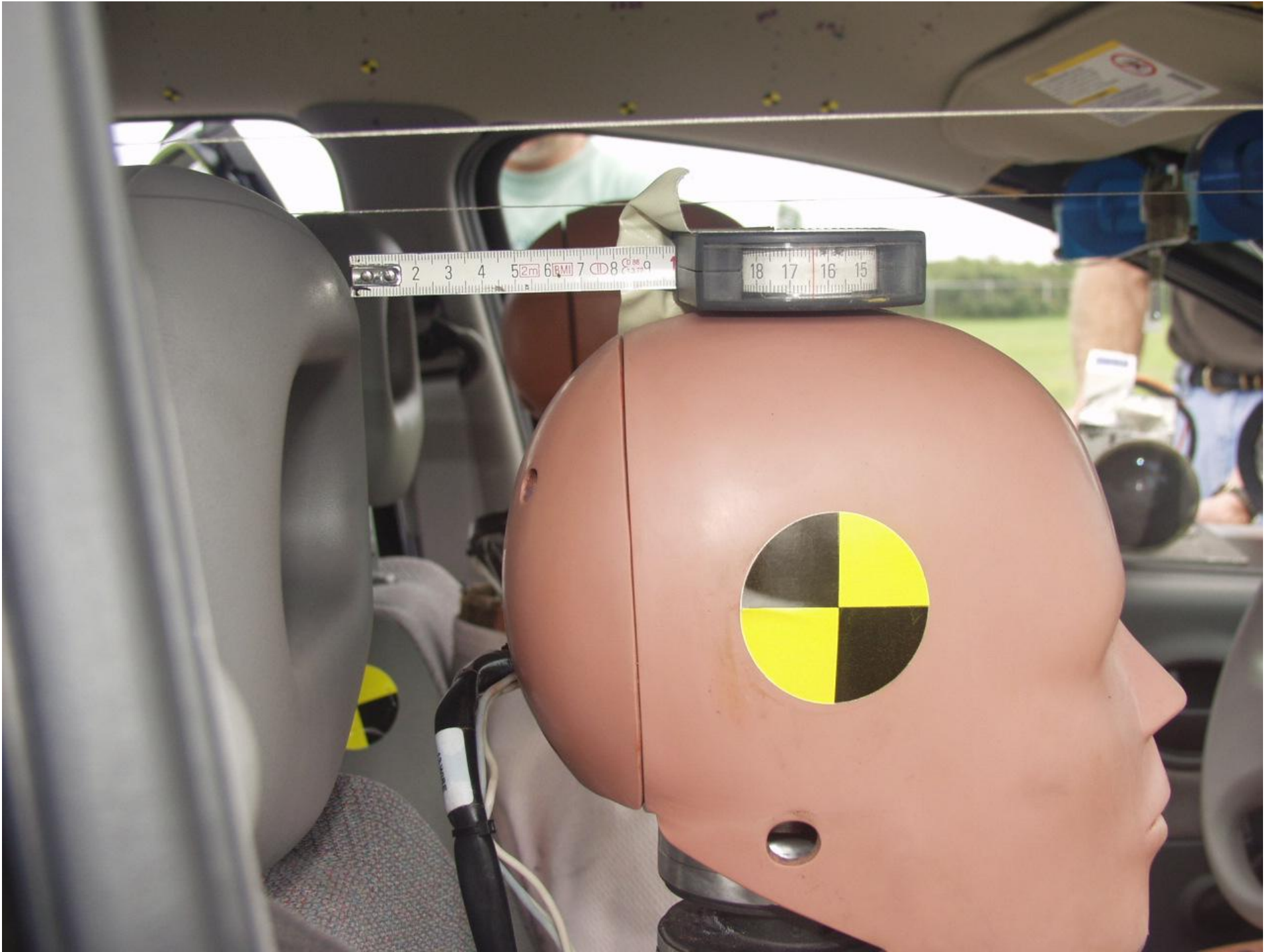
Figure A-4 PRE-TEST PASSENGER BACKSET VIEW
