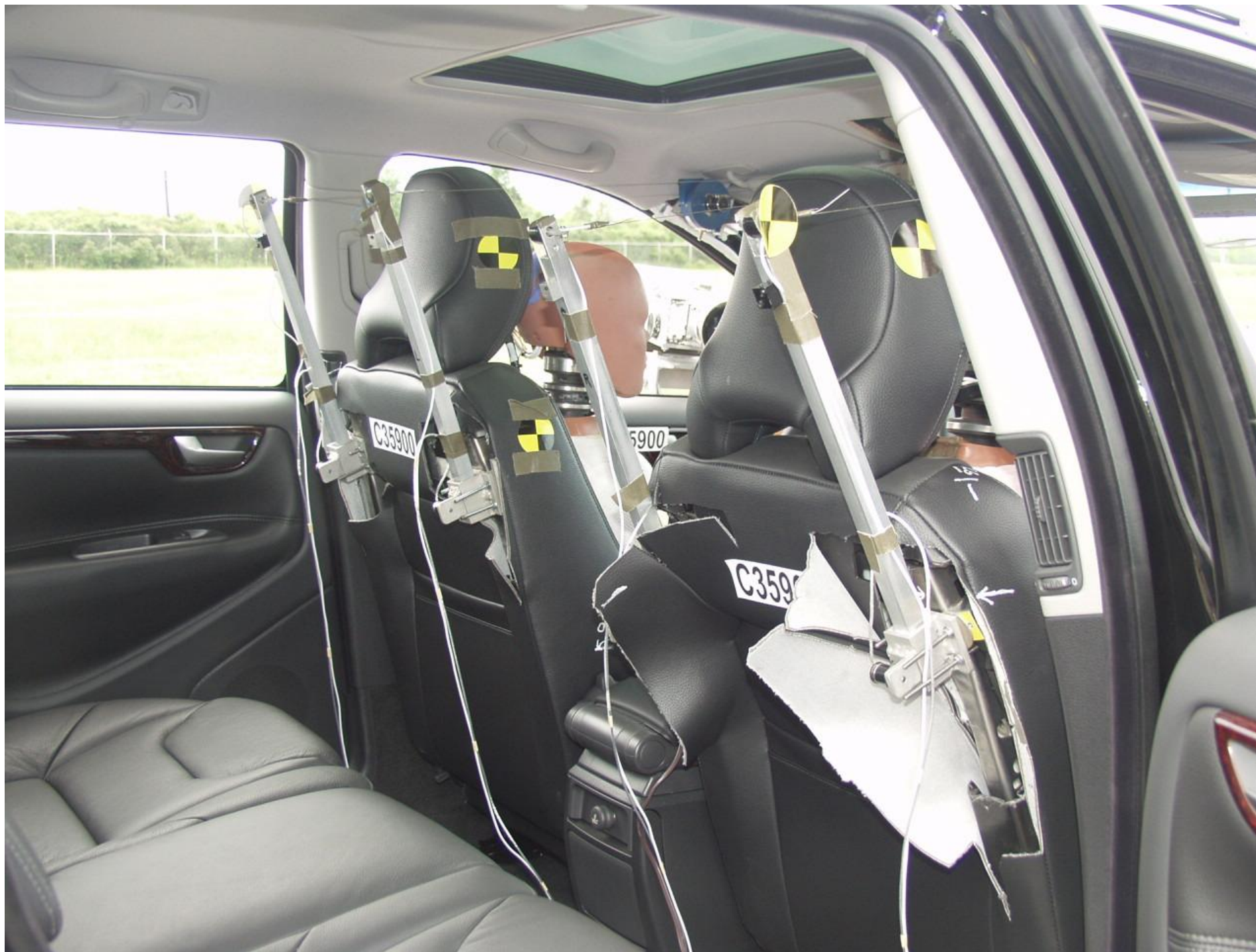
Figure A-7 PRE-TEST PASSENGER SEAT VIEW
