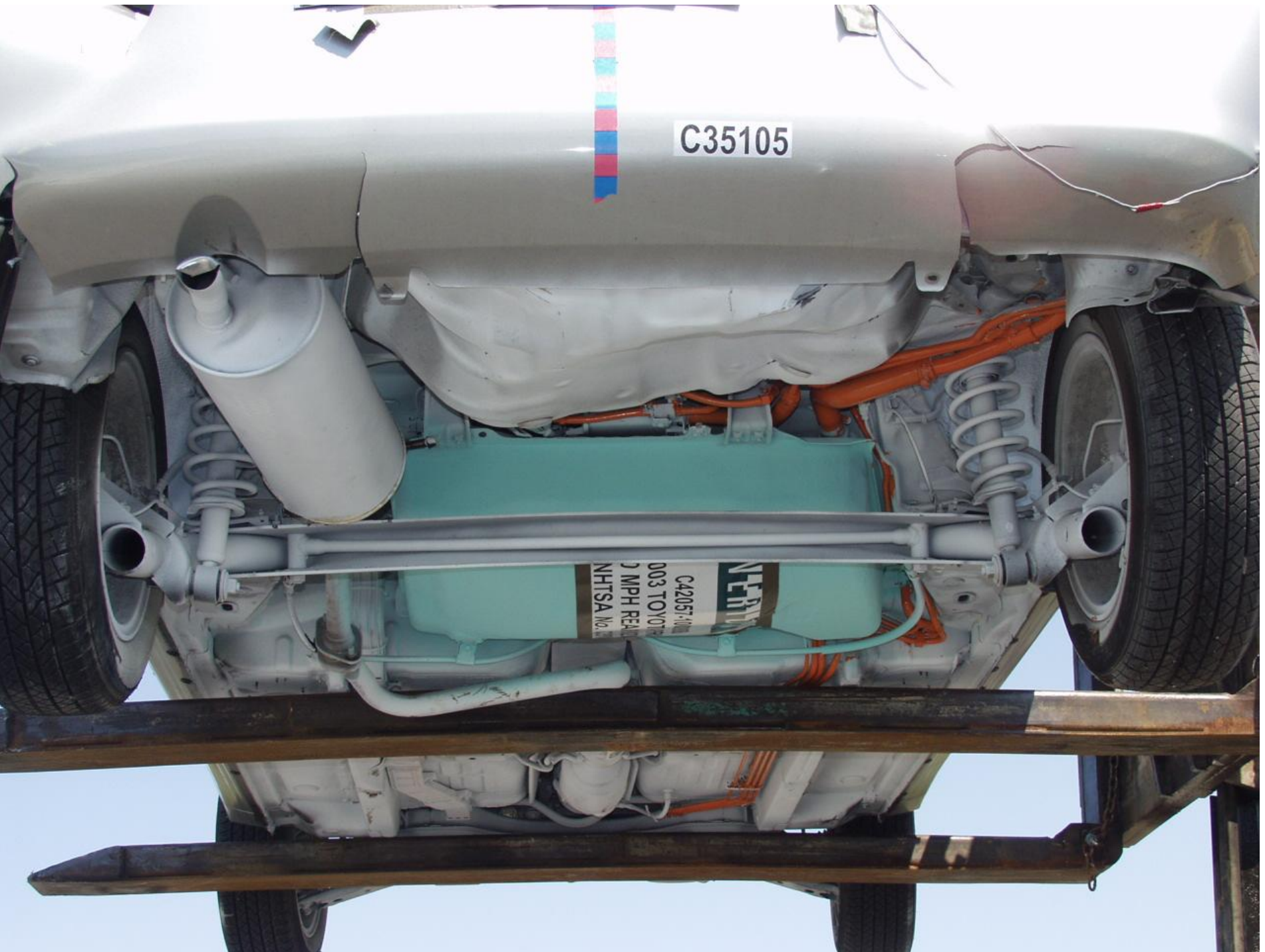
Figure A-16 POST-TEST REAR UNDERBODY VIEW
