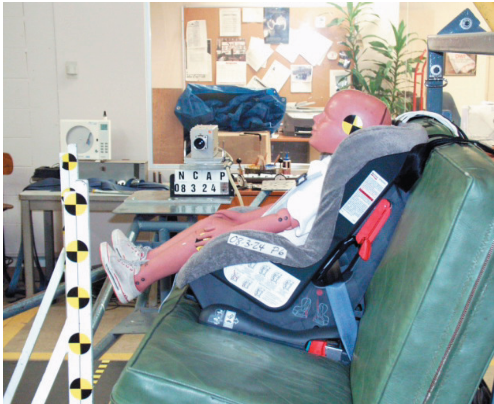
Pre Test Left Side View - Test 08-3-24
