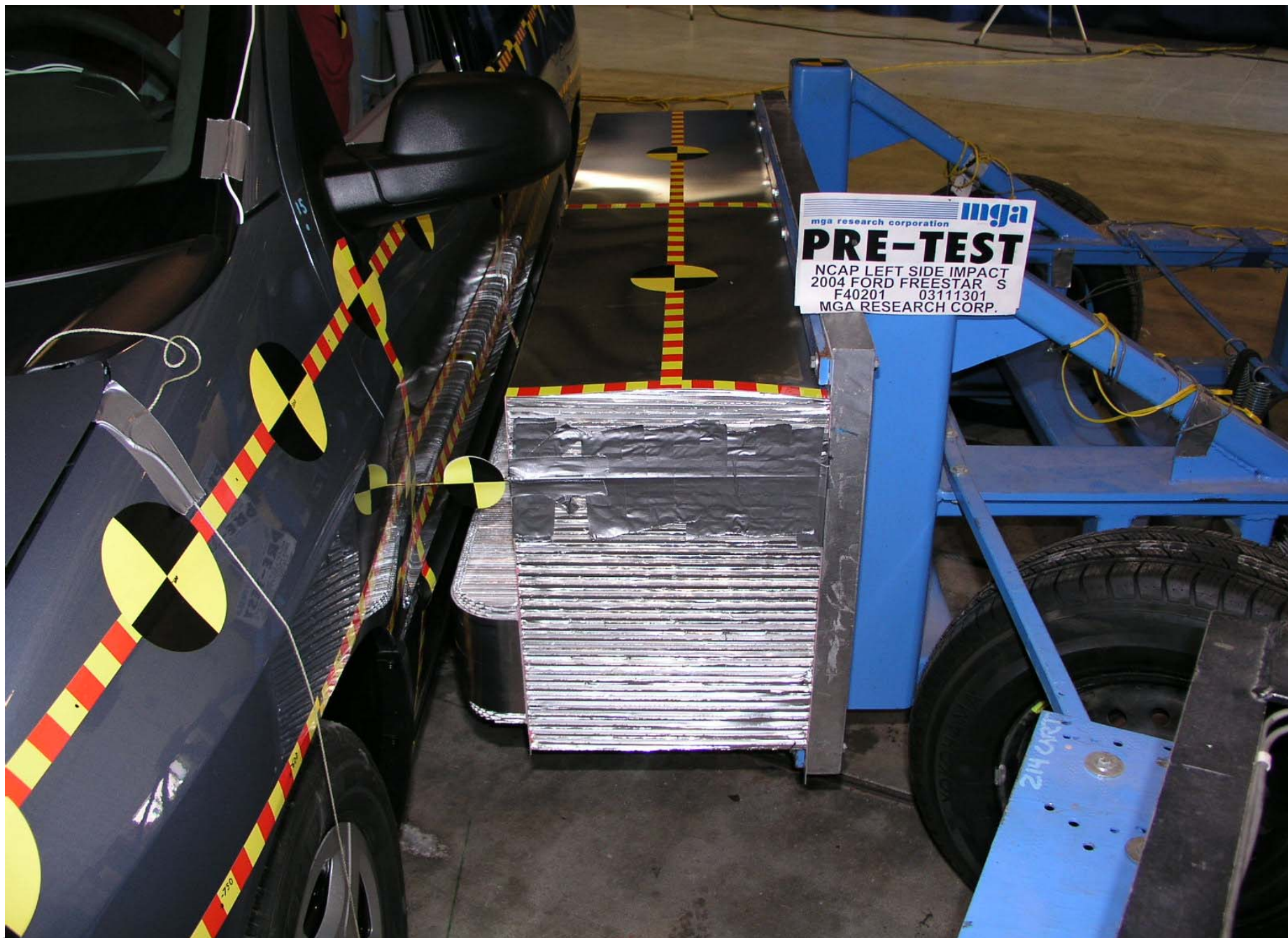
Pre-Test MDB Positioned Against Vehicle (left side)
