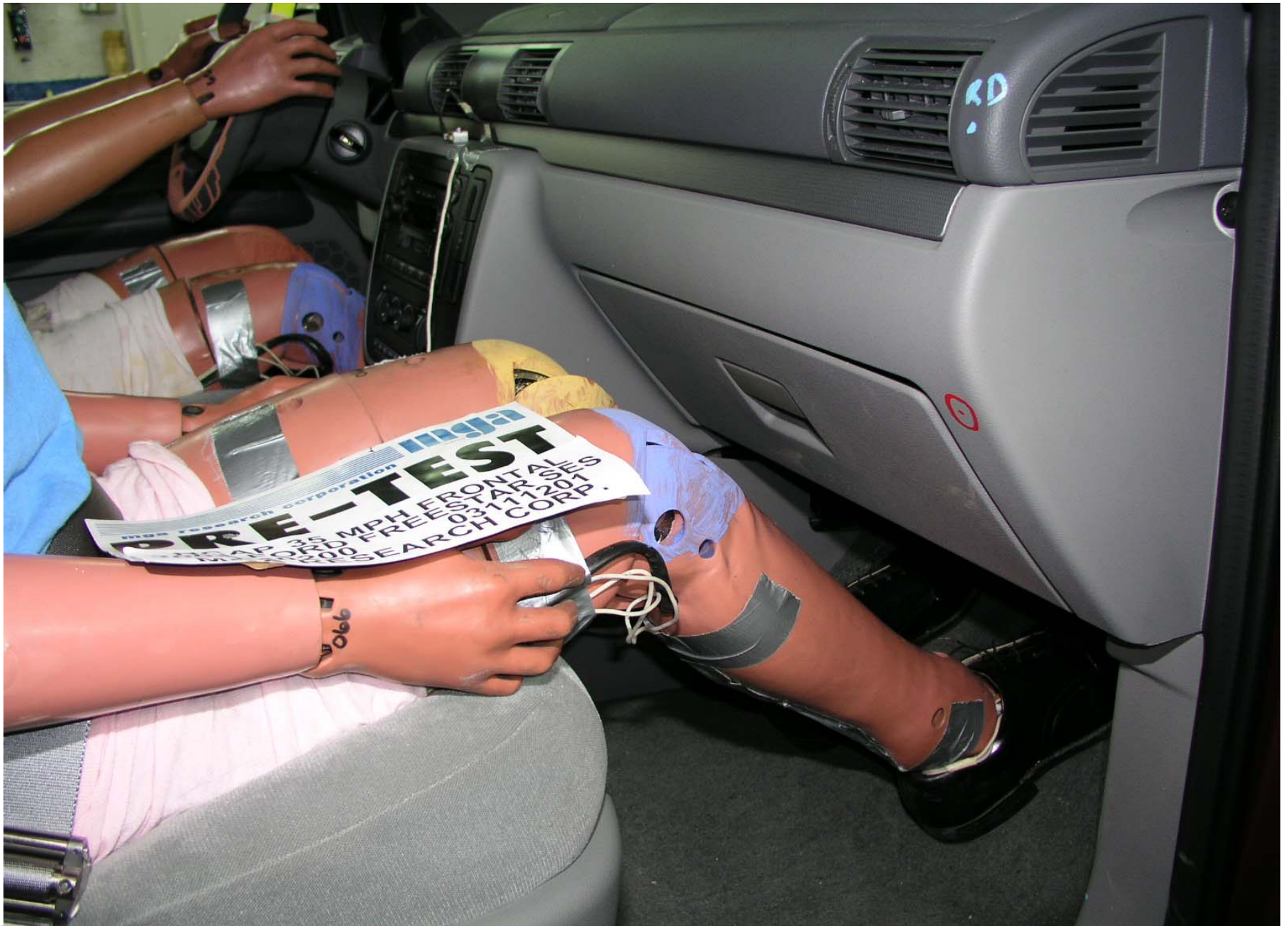
Pre-Test Passenger Side Knee Bolster View
