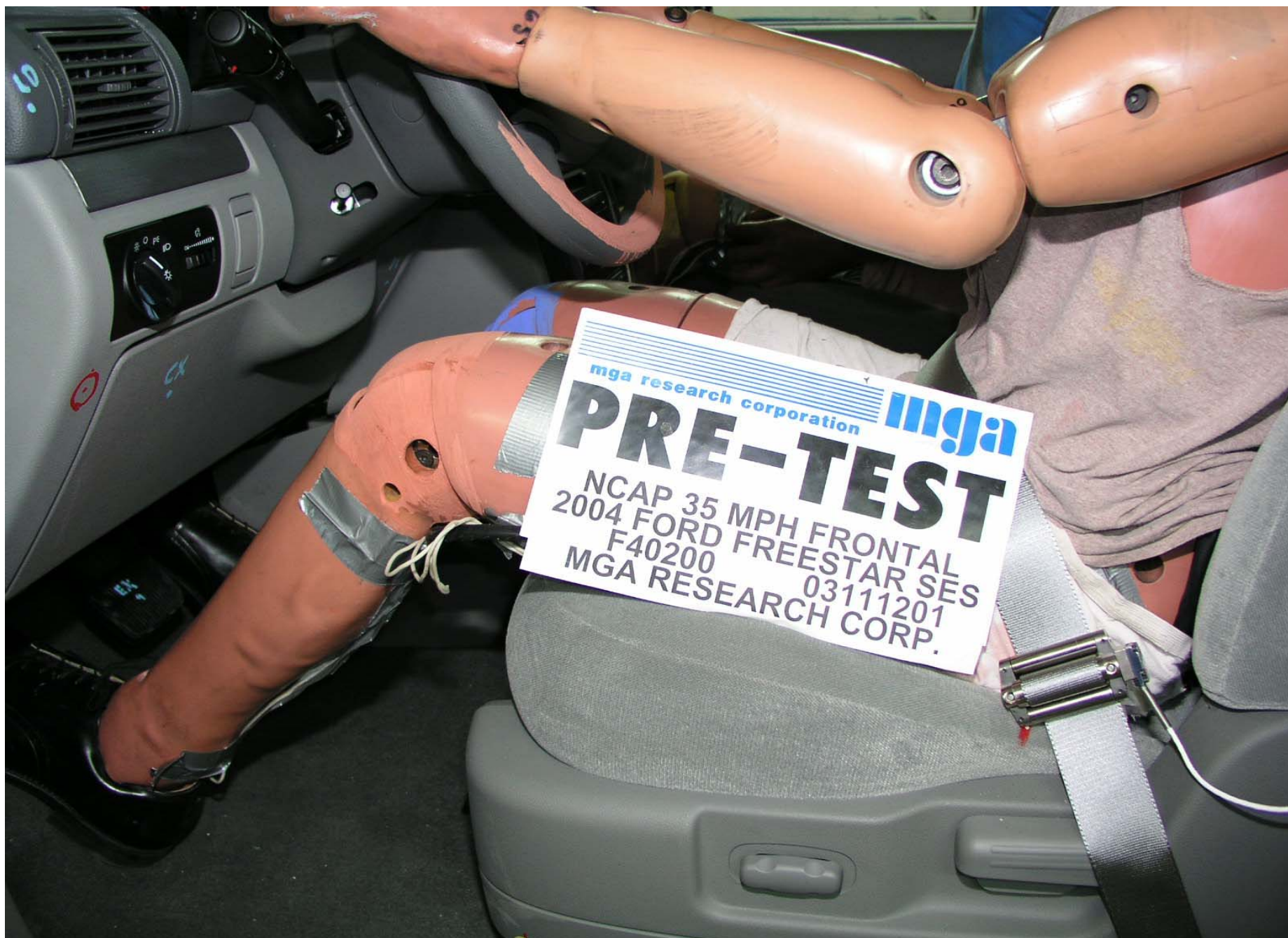
Pre-Test Driver Side Knee Bolster View
