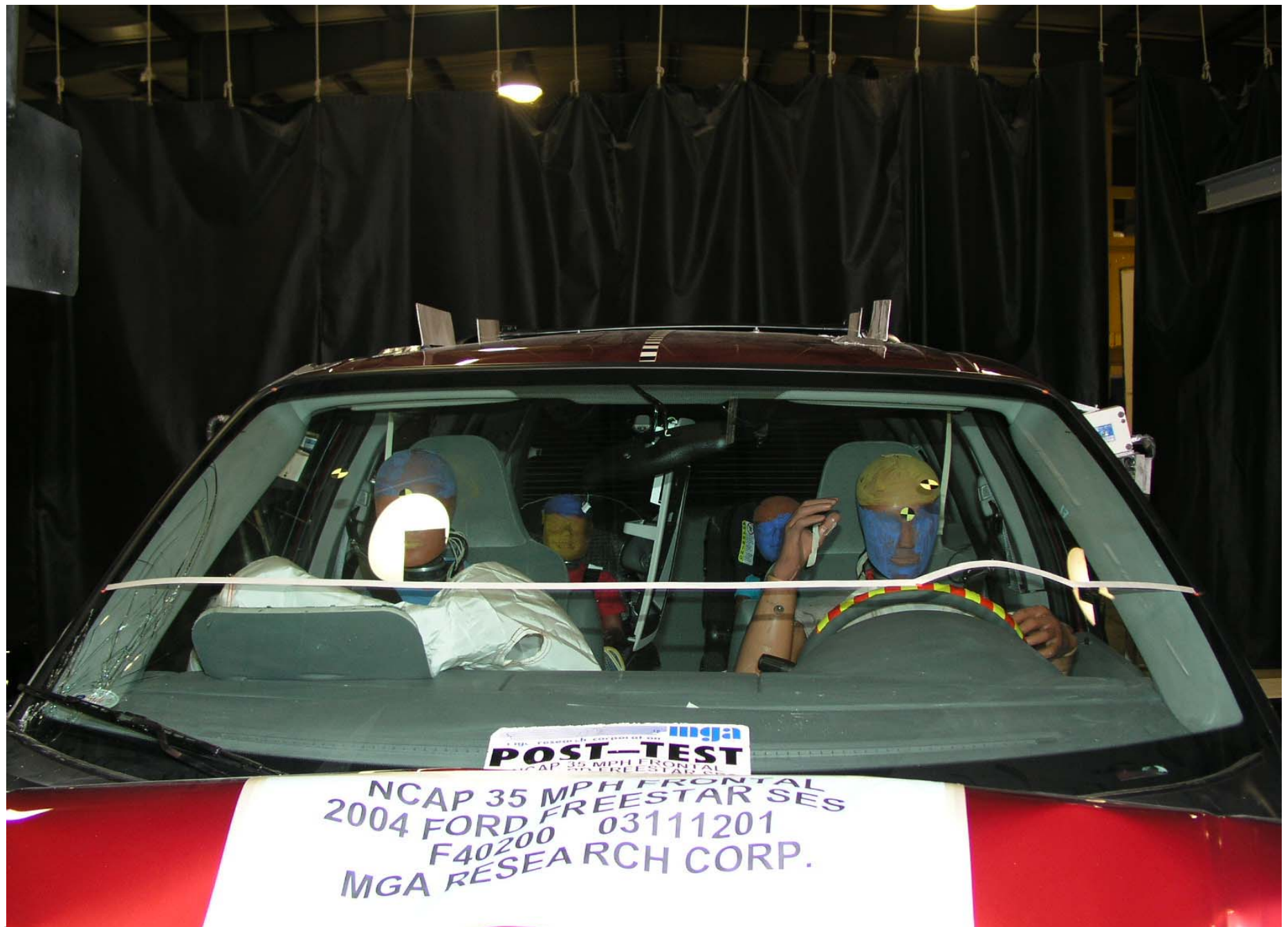
Post-Test Windshield View
