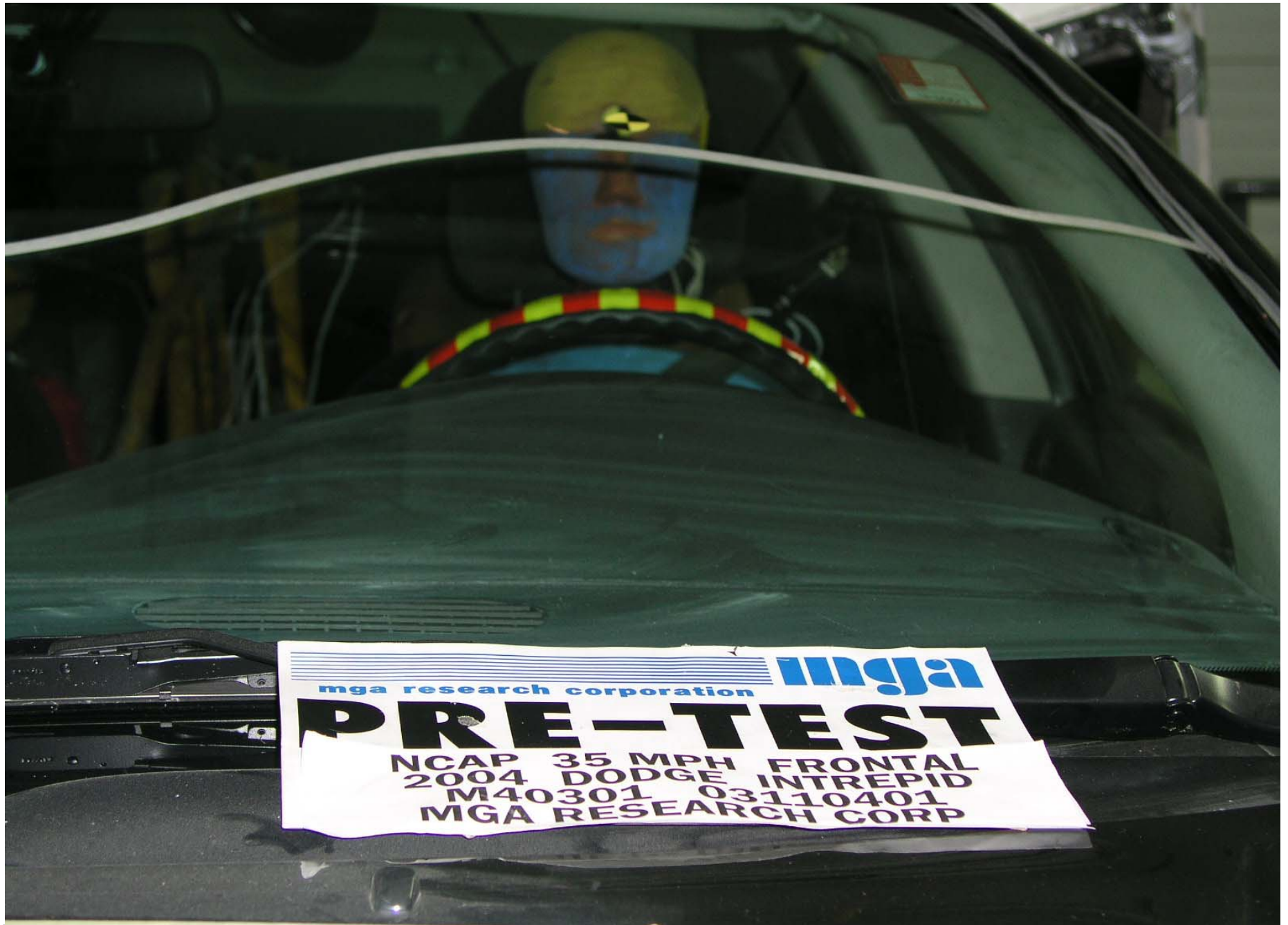
Pre-Test Driver Dummy Front View (head position)
