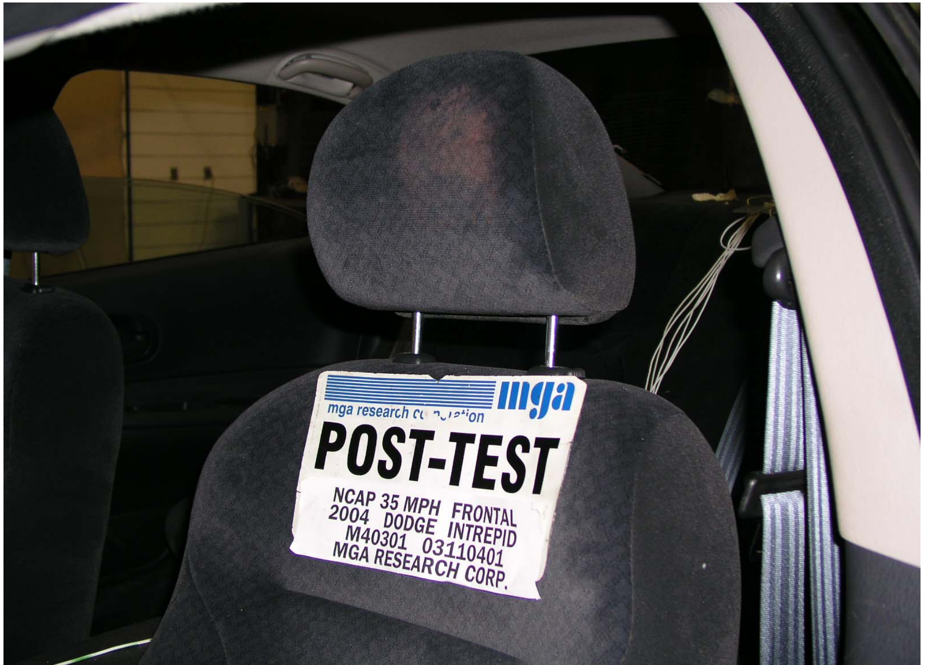
Post-Test Driver Dummy Head Contact
