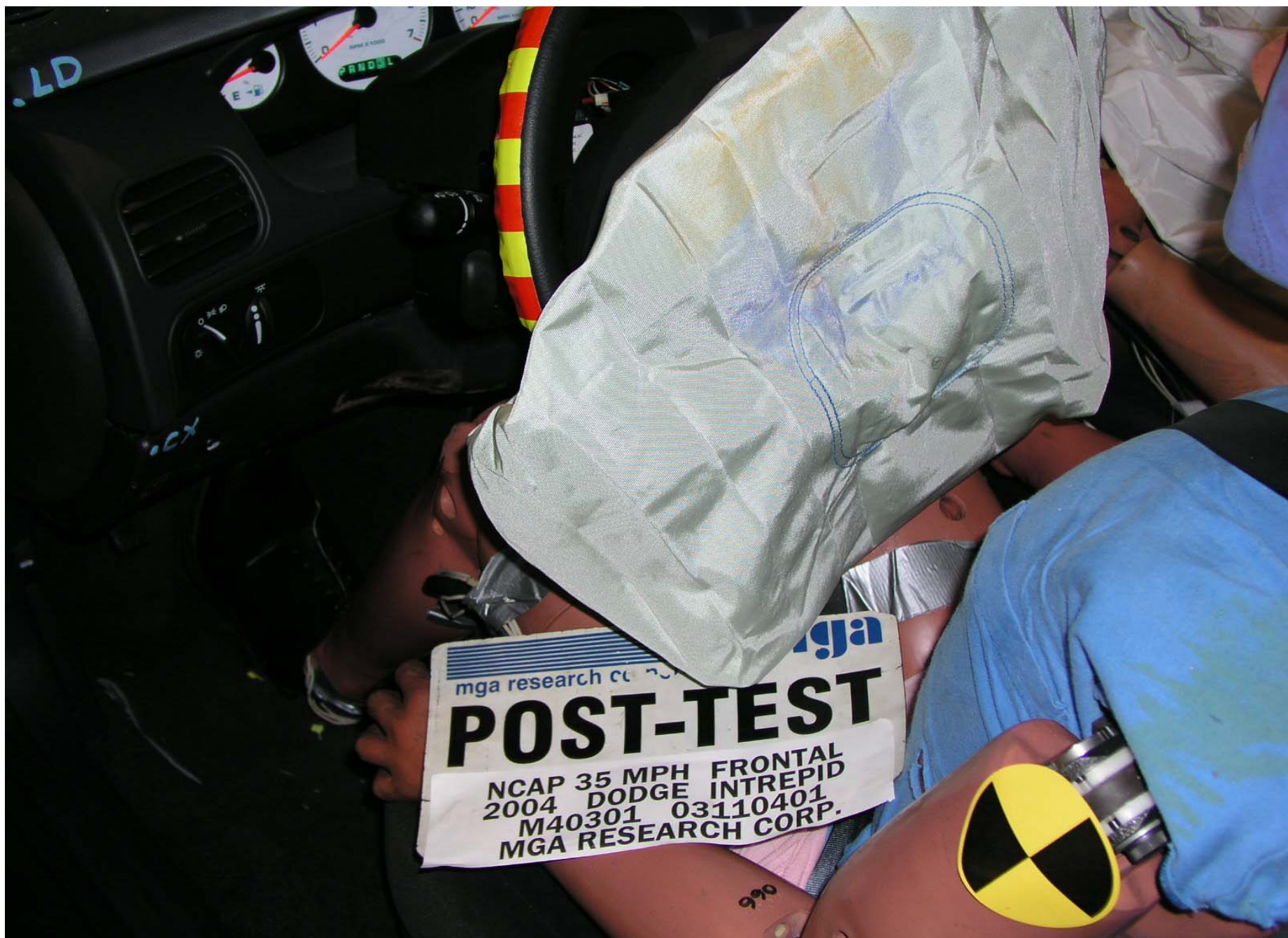
Post-Test Driver Dummy Airbag Contact
