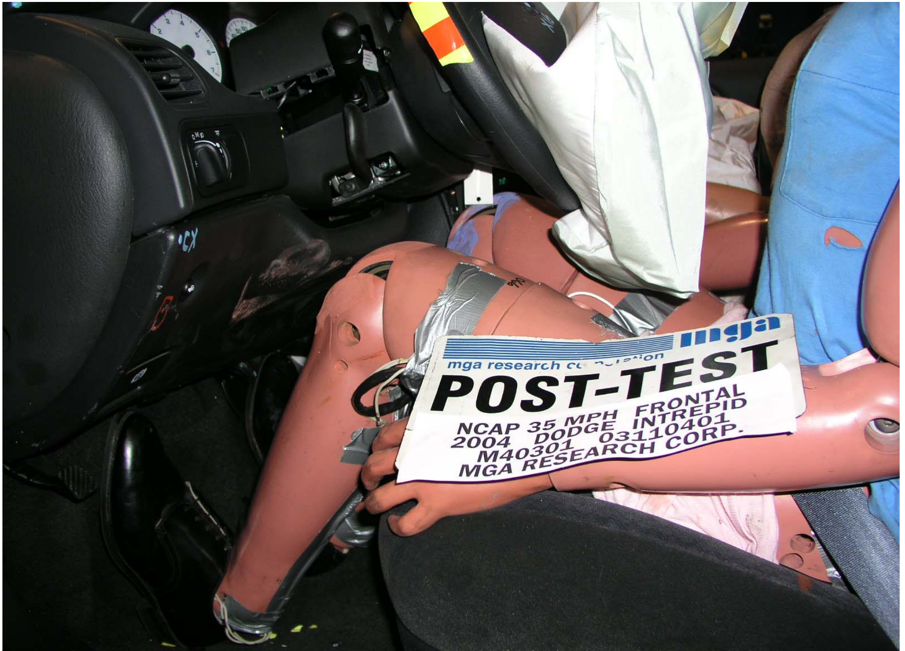
Post-Test Driver Side Knee Bolster View
