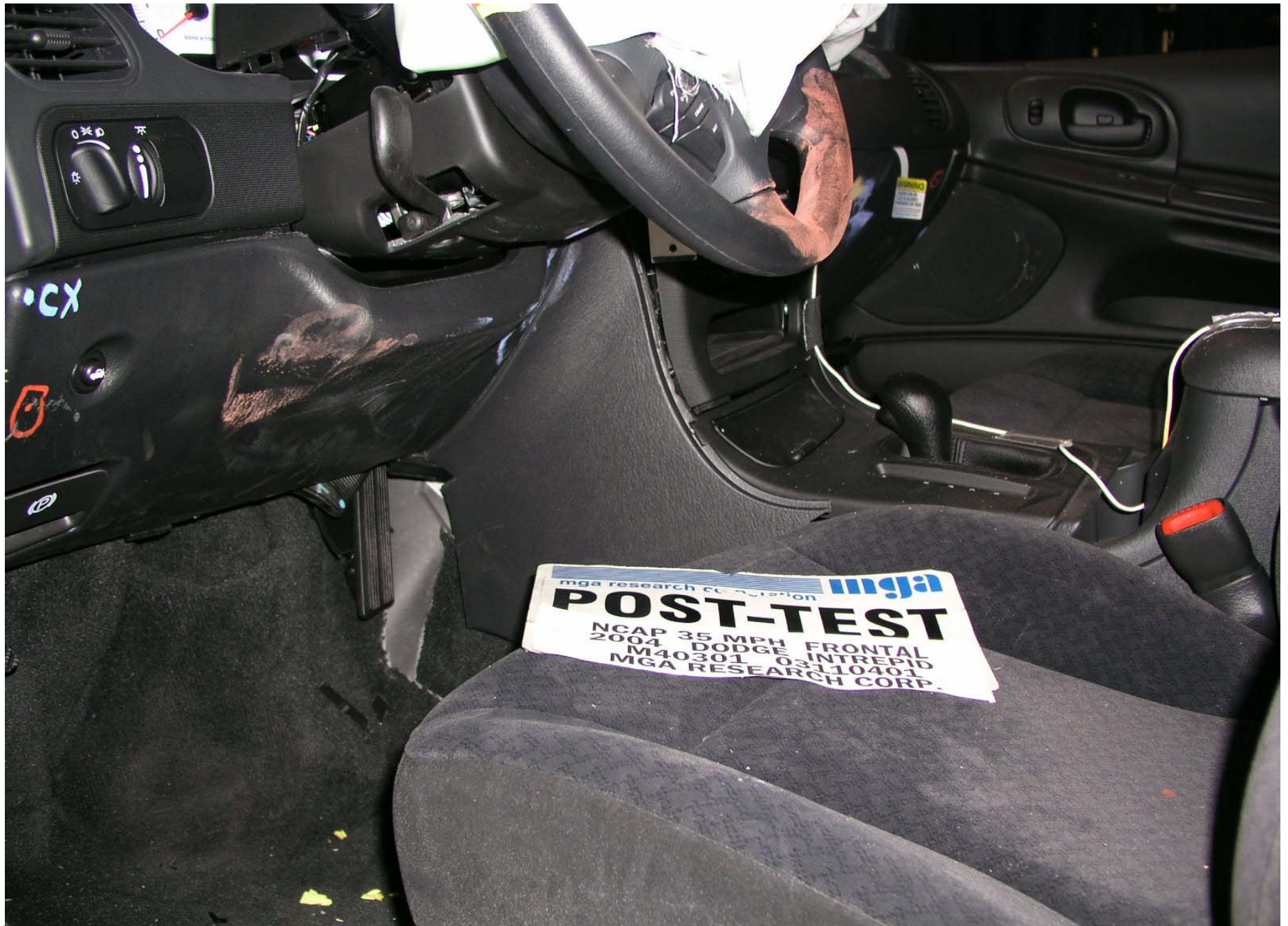
Post-Test Driver Dummy Knee Contact
