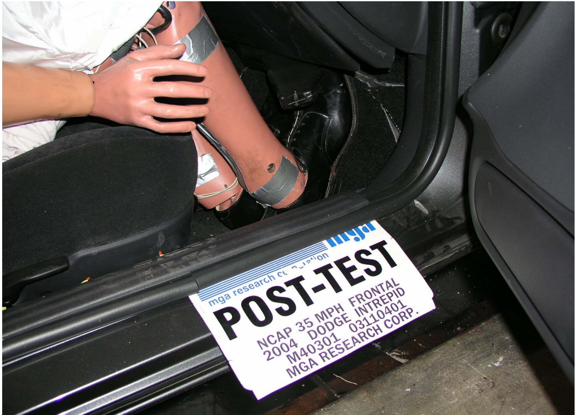
Post-Test Passenger Dummy Feet Position
