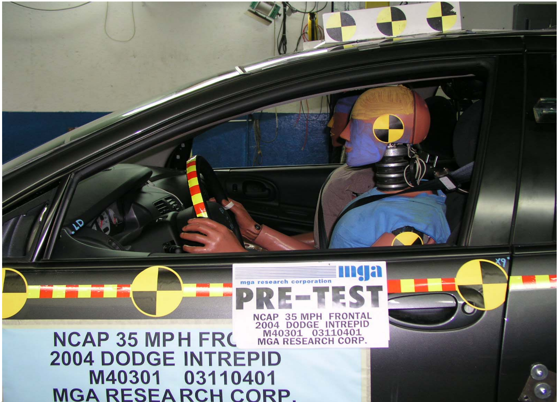
Pre-Test Driver Dummy Position Left Side View
