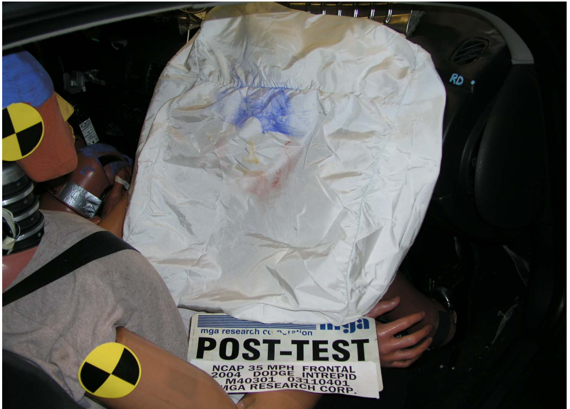
Post-Test Passenger Dummy Airbag Contact
