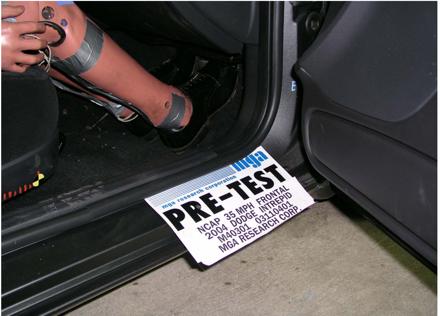
Pre-Test Passenger Dummy Feet Position
