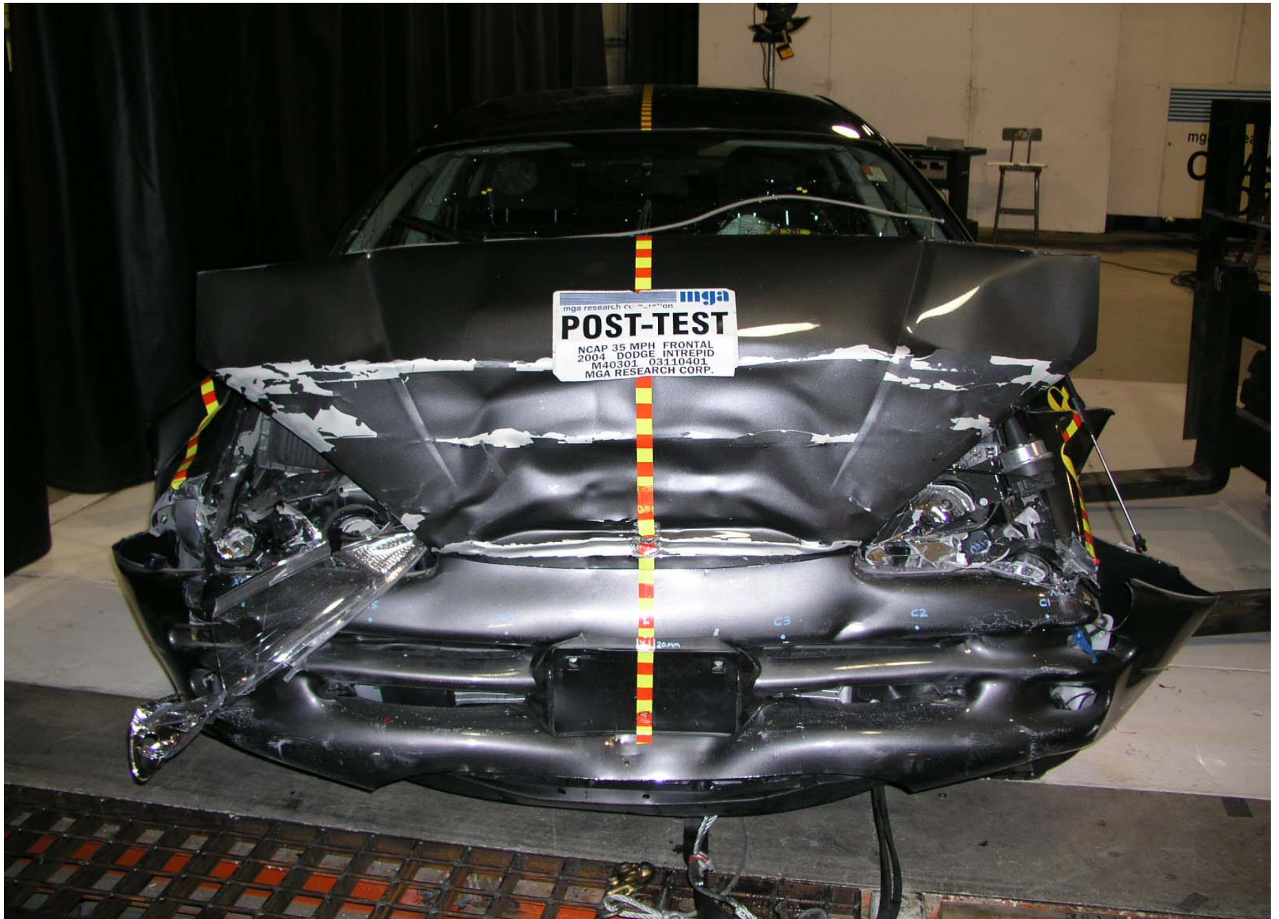
Post-Test Front View of Test Vehicle
