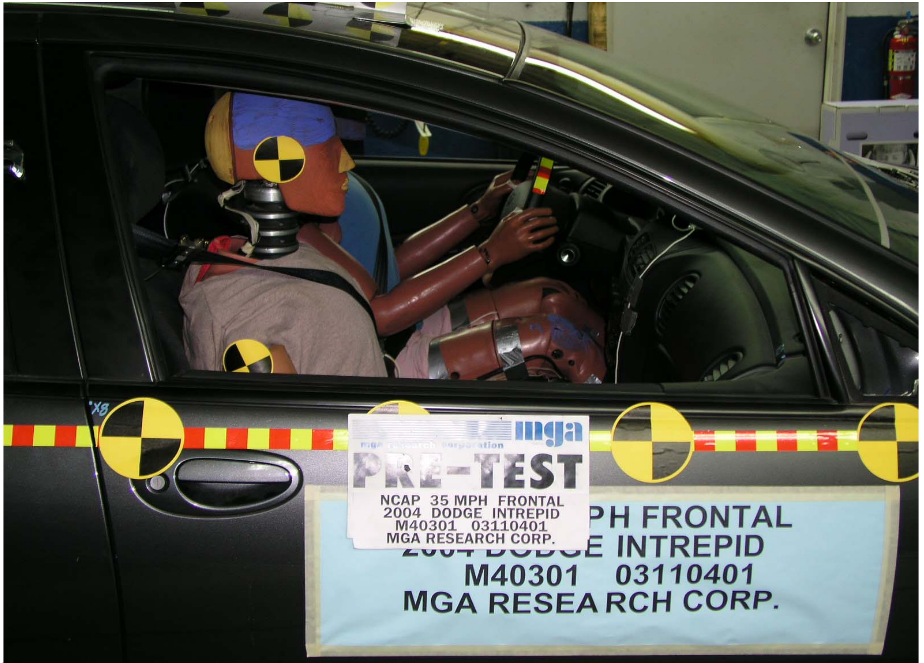
Pre-Test Passenger Dummy Position Right Side View
