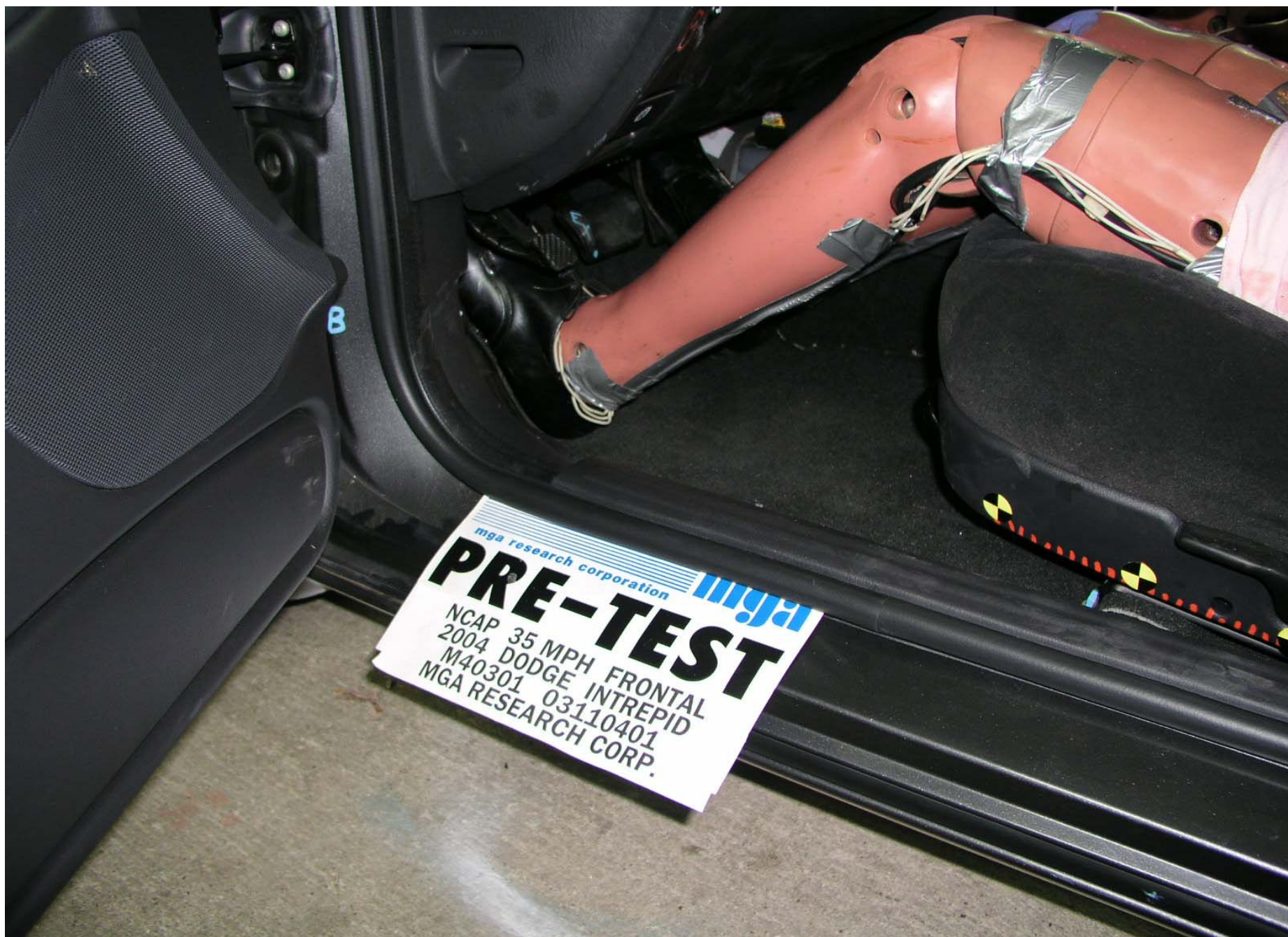
Pre-Test Driver Dummy Feet Position
