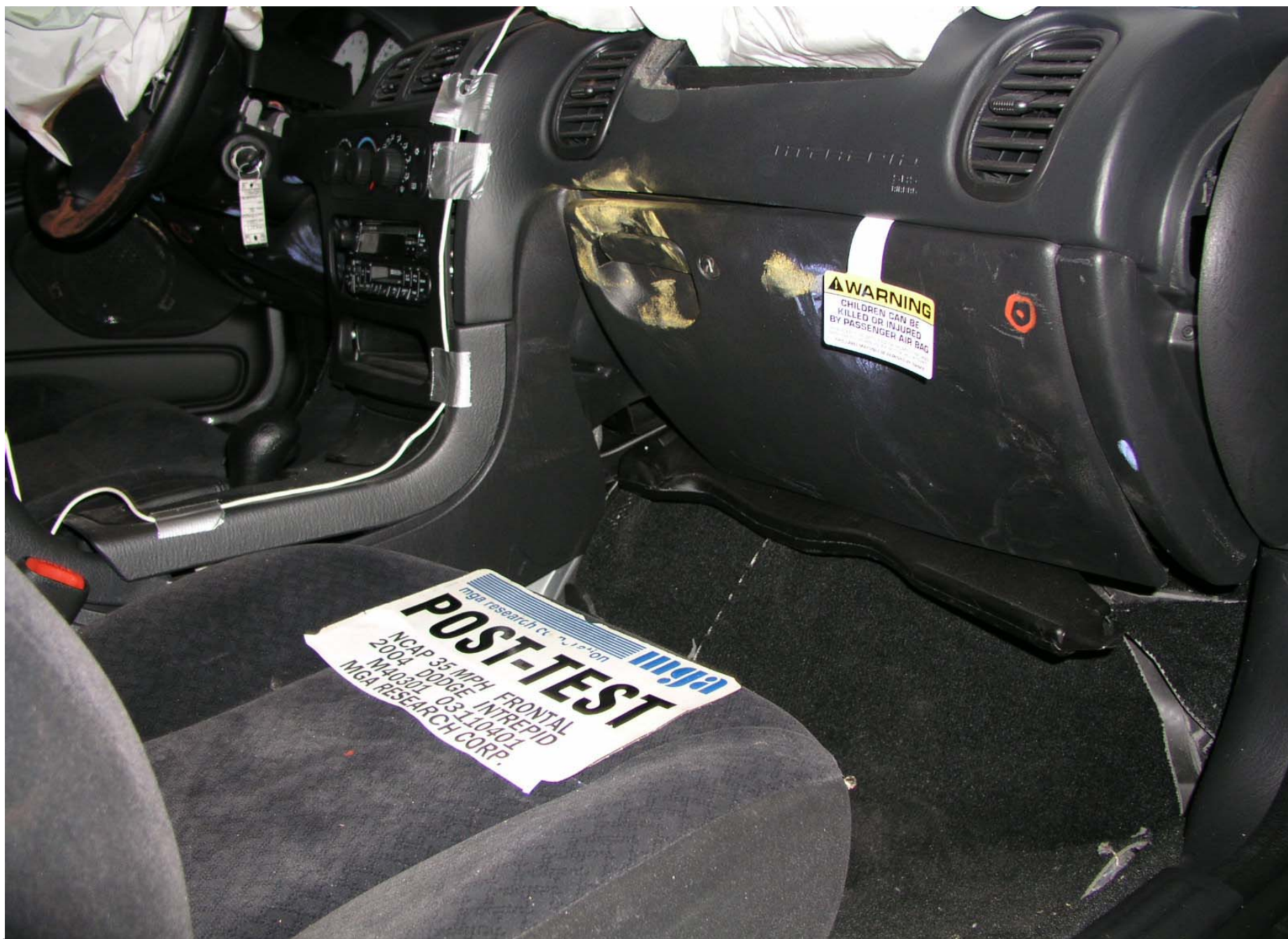
Post-Test Passenger Dummy Knee Contact
