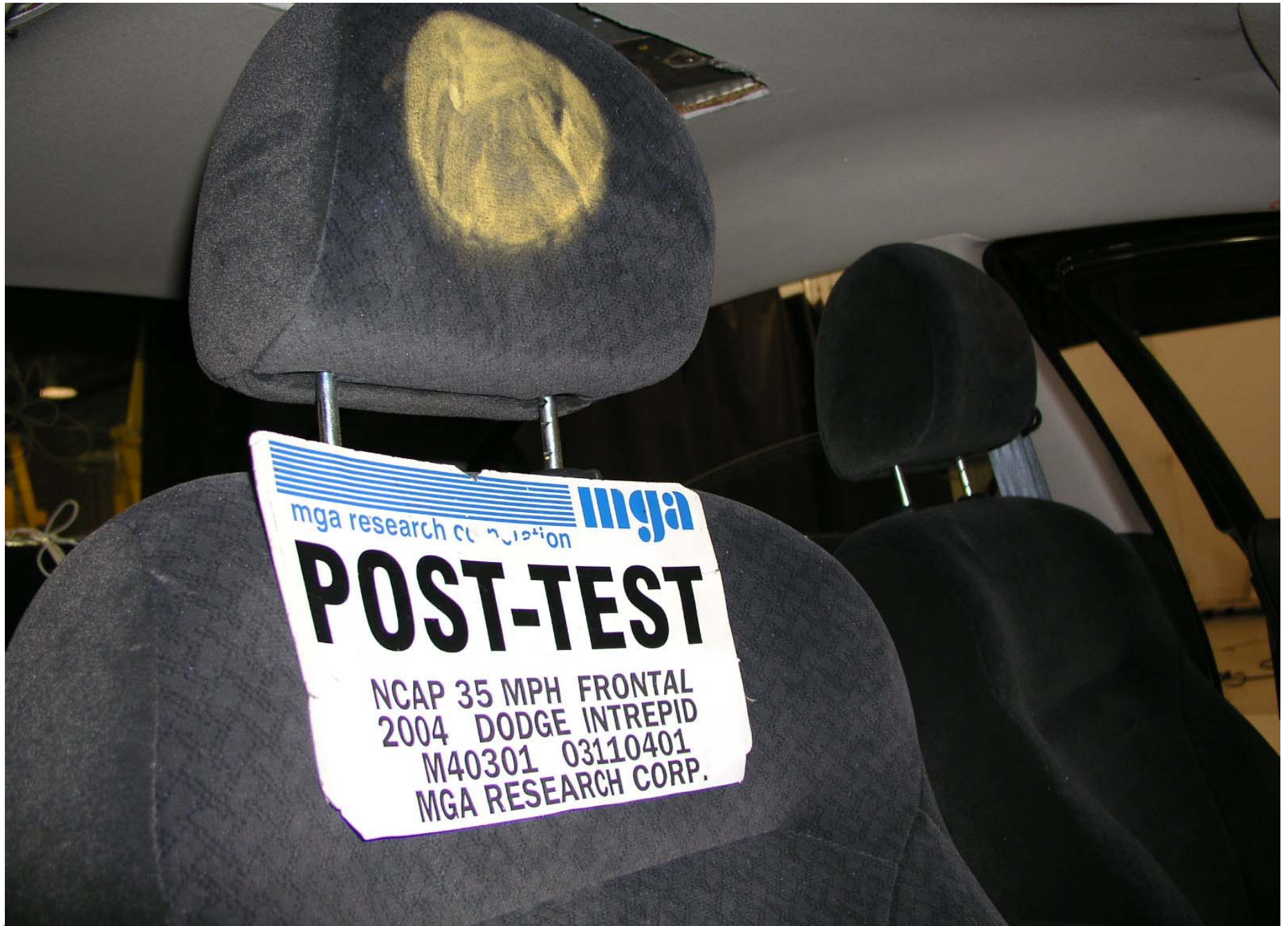
Post-Test Passenger Dummy Head Contact
