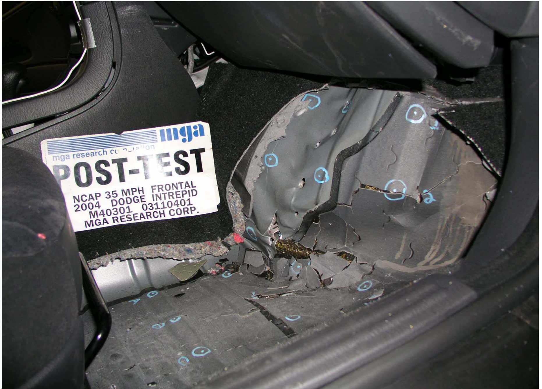
Post-Test Passenger Side Floor Pan View
