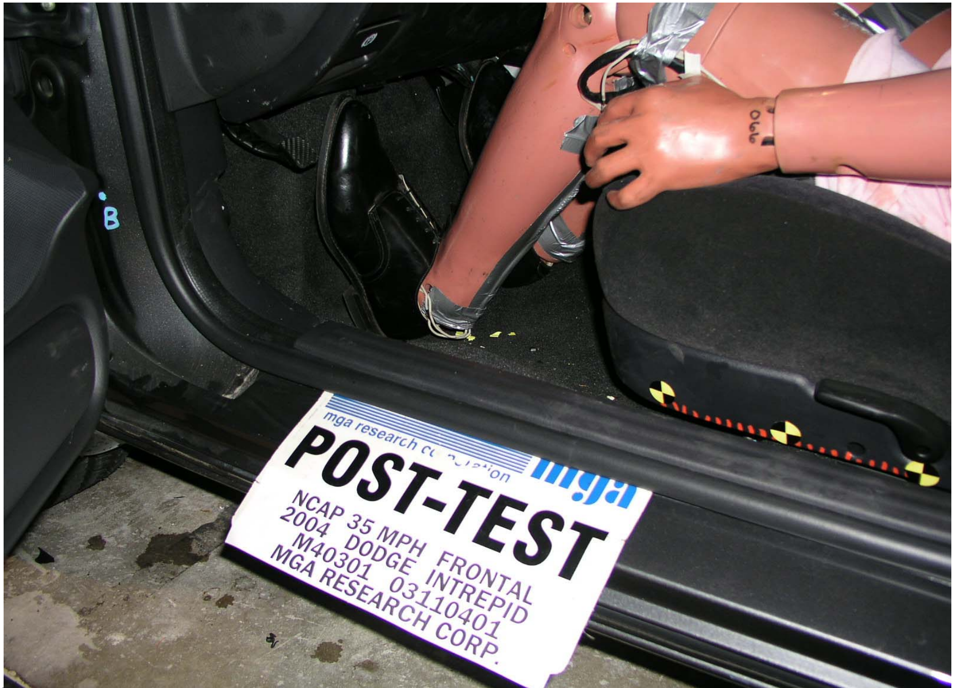
Post-Test Driver Dummy Feet Position
