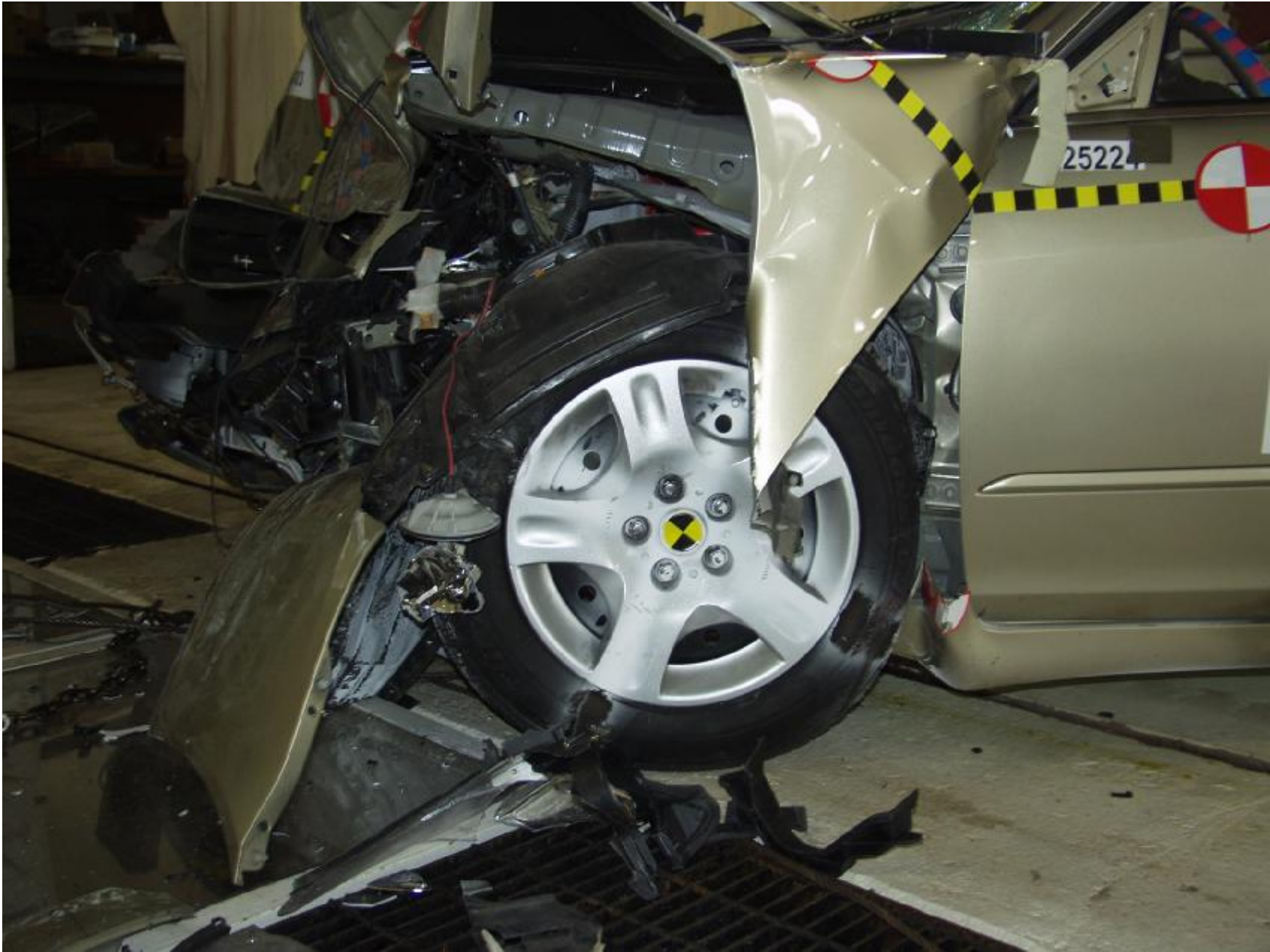
Figure A-66 : POST-TEST WHEEL/TIRE DEFORMATION
