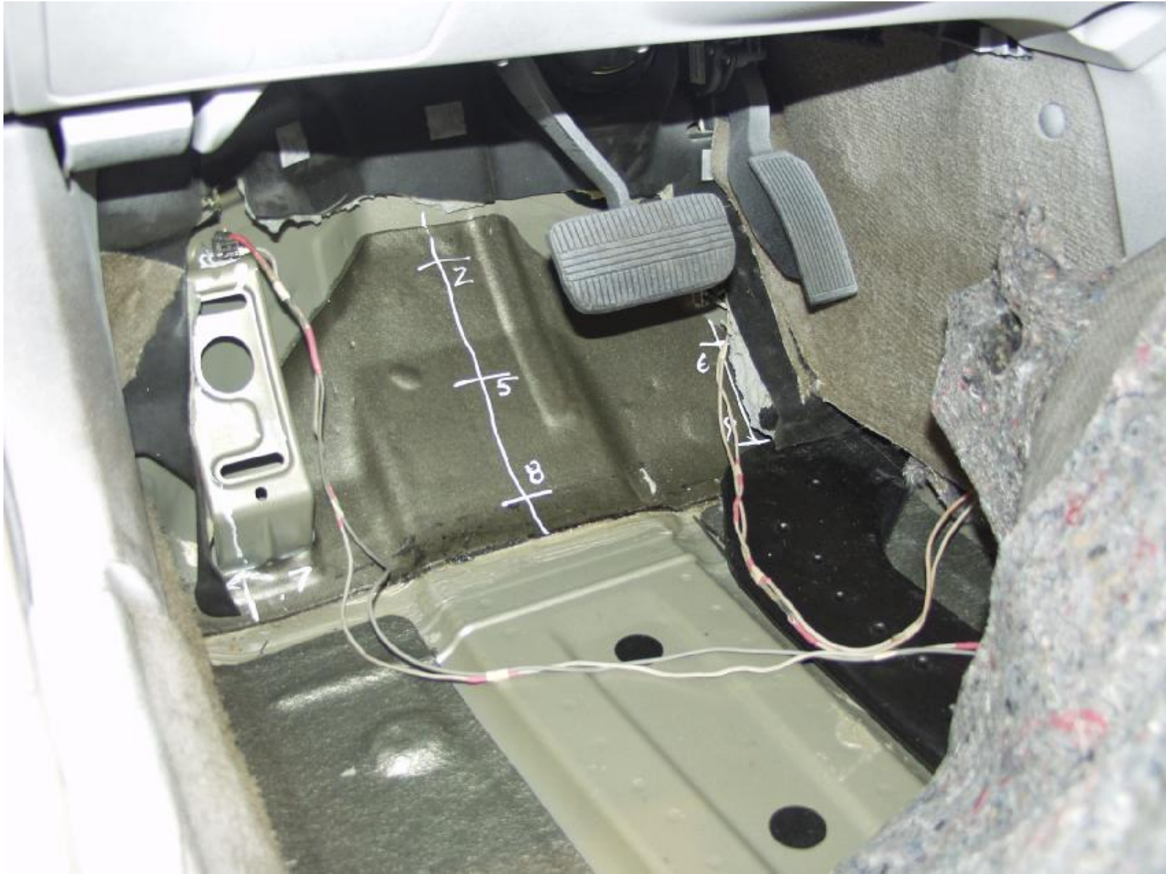
Figure A-54 : PRE-TEST DRIVER TOE-PAN
