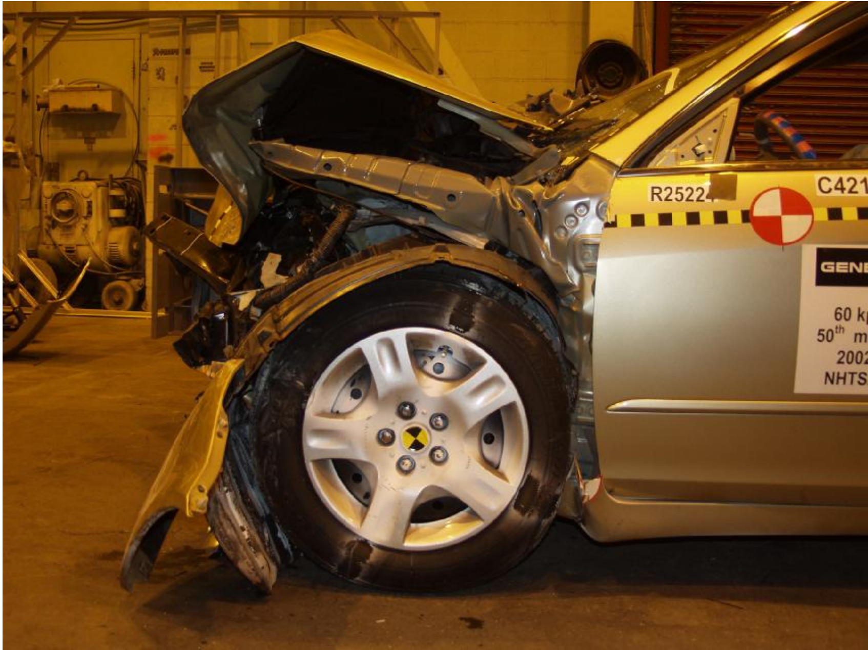
Figure A-67 : POST-TEST WHEEL TO A-PILLAR
