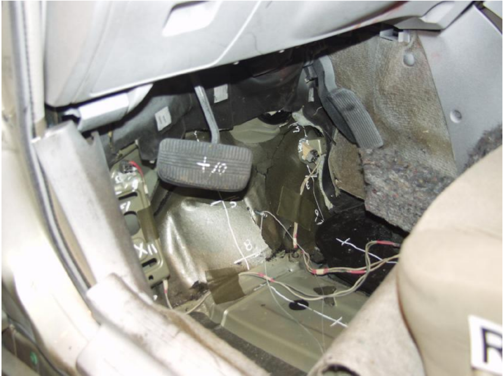
Figure A-55 : POST-TEST DRIVER TOR-PAN
