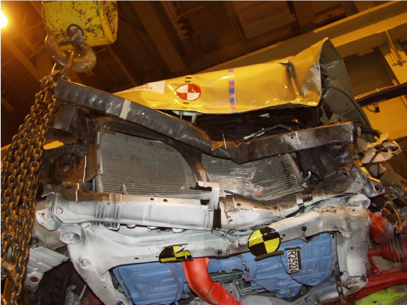
Figure A-65 : POST-TEST BUMPER TO RAIL ATTACHMENTS
