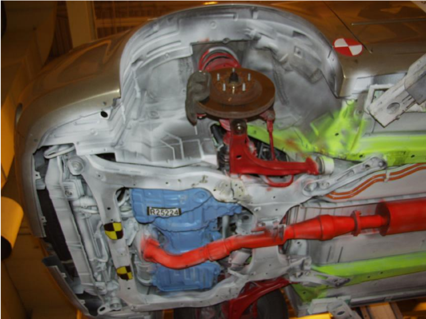
Figure A-72 : PRE-TEST UNDERBODY FRONT STRUCTURE
