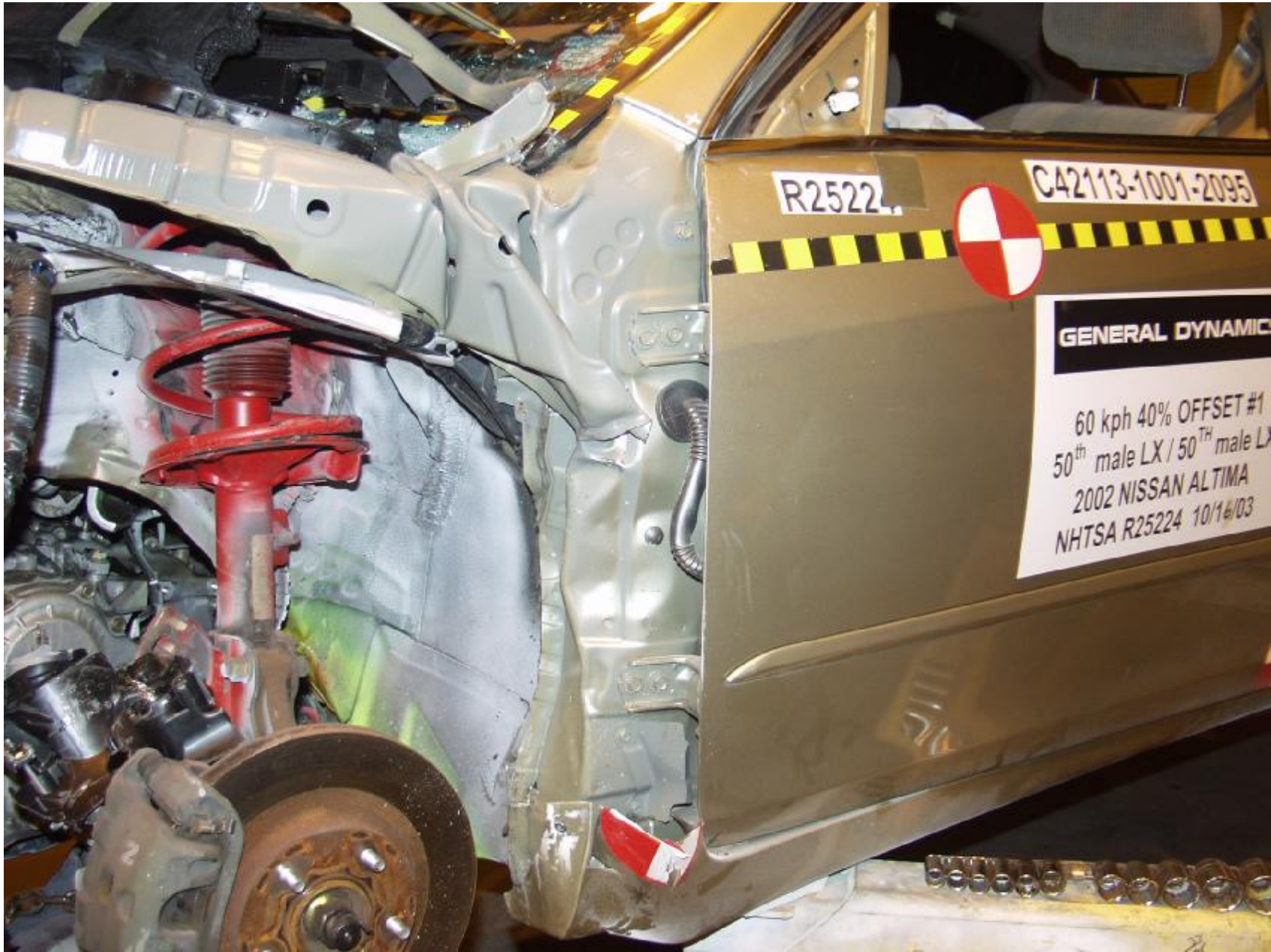
Figure A-58 : POST-TEST OF DRIVER SIDE A-PILLAR
