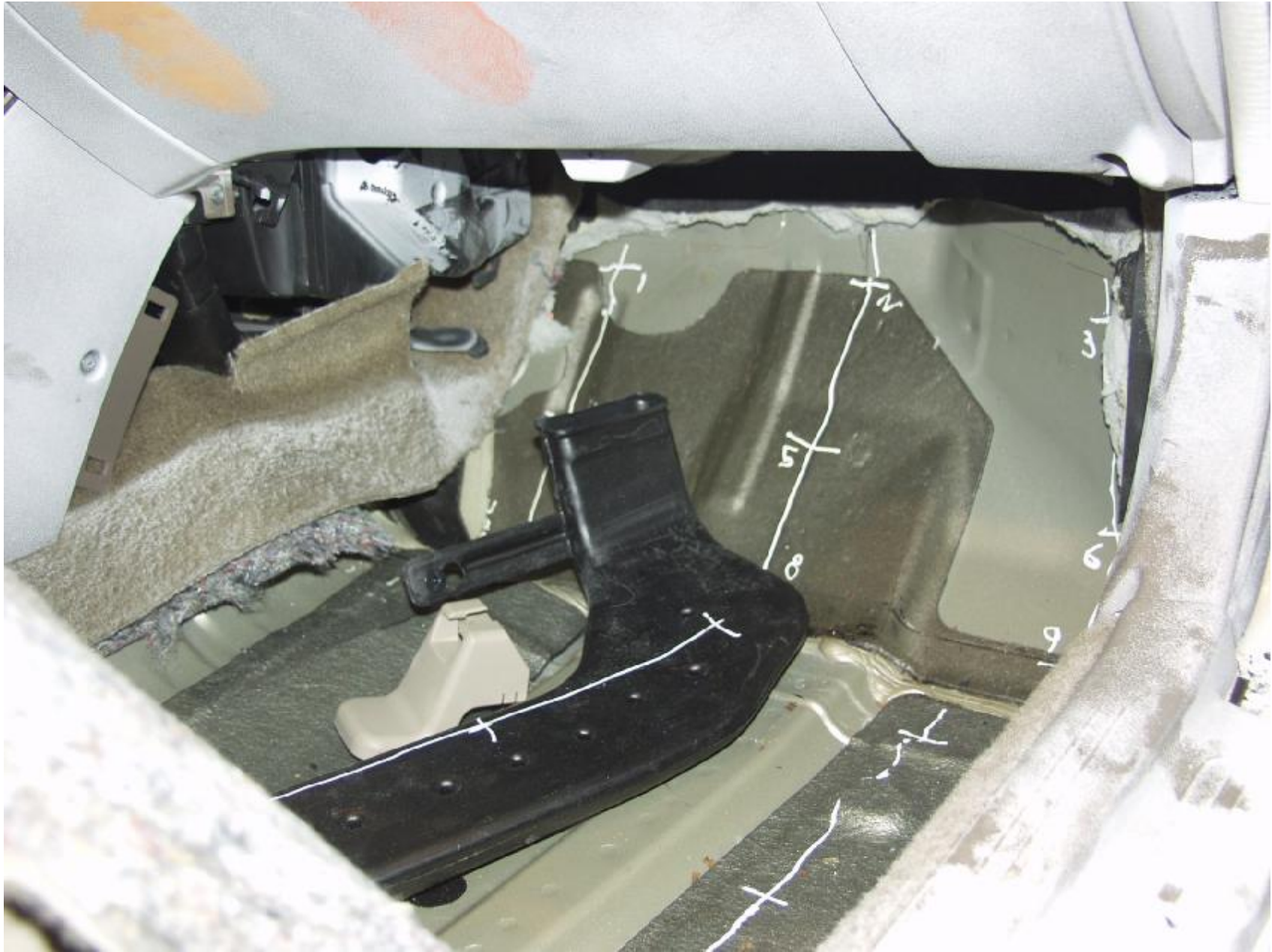
Figure A-57 : POST-TEST PASSENGER TOE-PAN
