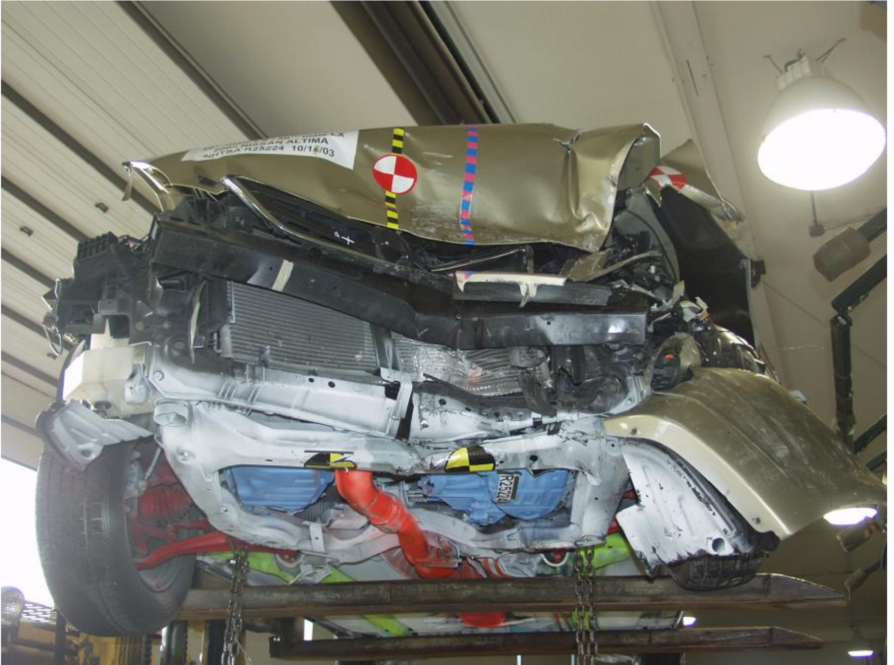
Figure A-16: POST-TEST FRONT UNDERBODY VIEW
