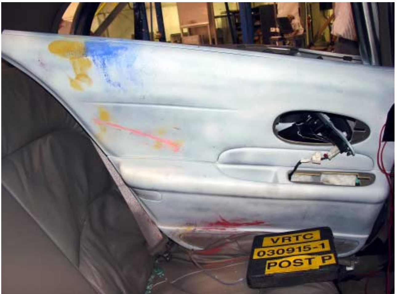
Figure A-38 Post-Test Interior of Rear Panel Showing SID-IIs Impact Locations
