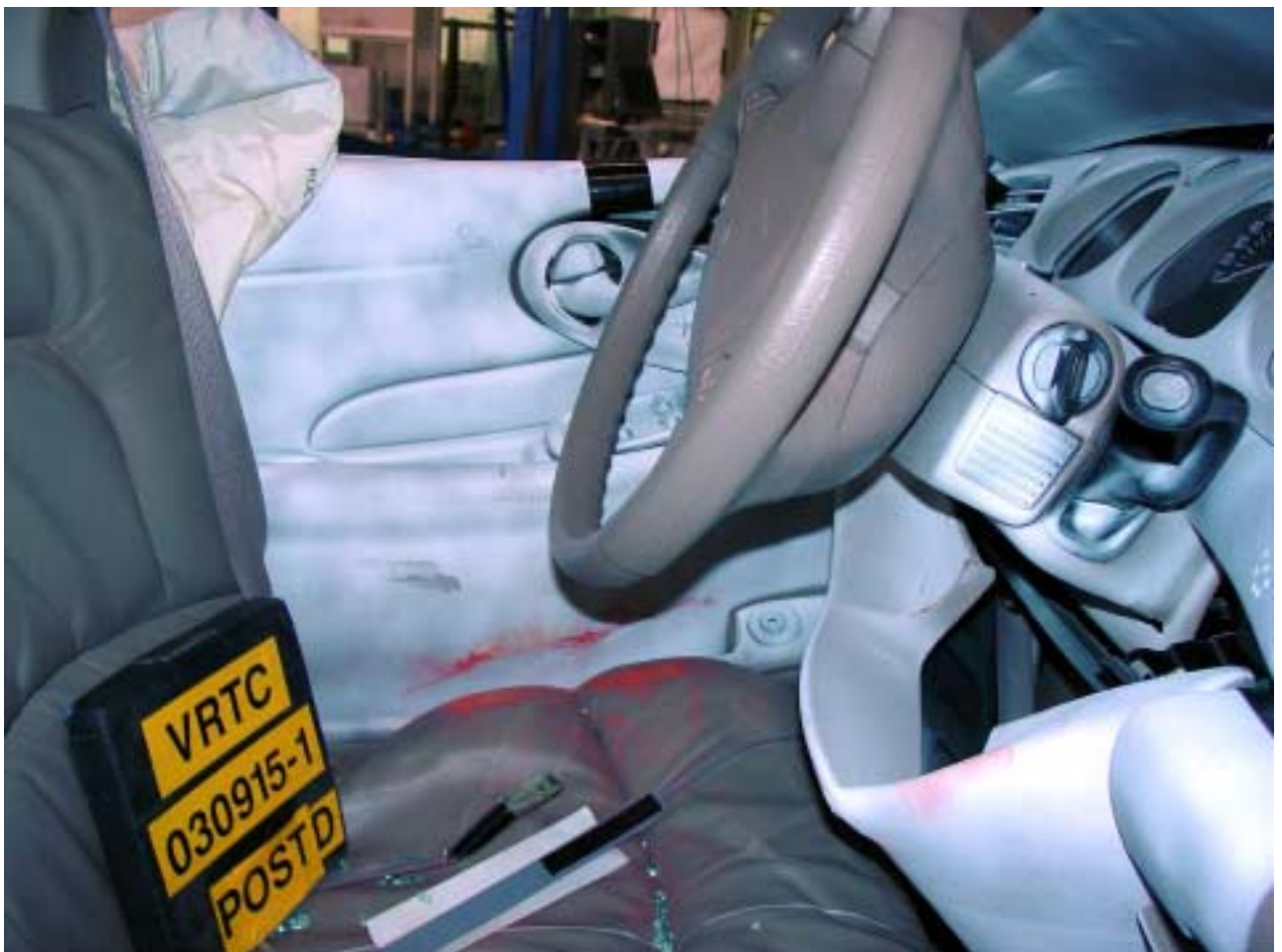
Figure A-33 Post-Test Interior of Front Door Showing SID-IIs Impact Locations
