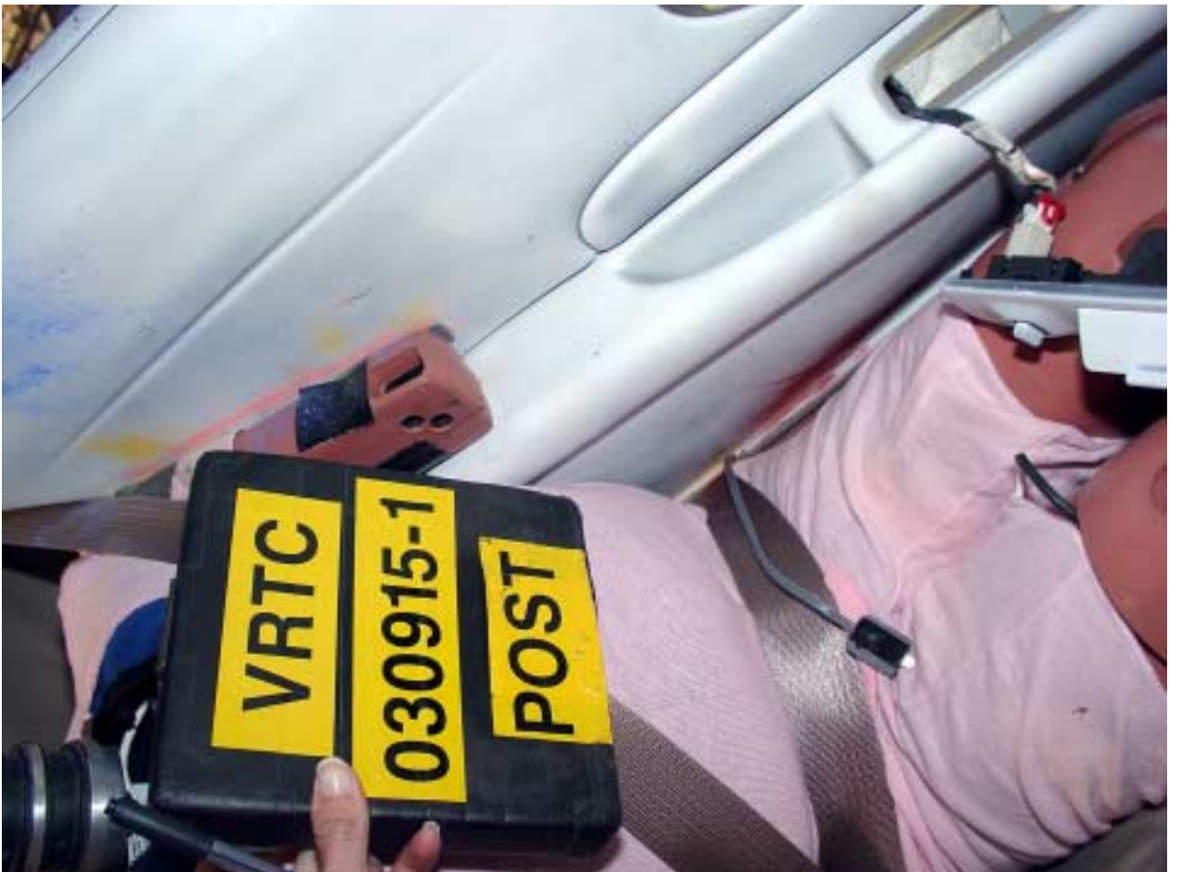
Figure A-31 Post-Test Left View of Rear SID-IIs and Door Clearance
