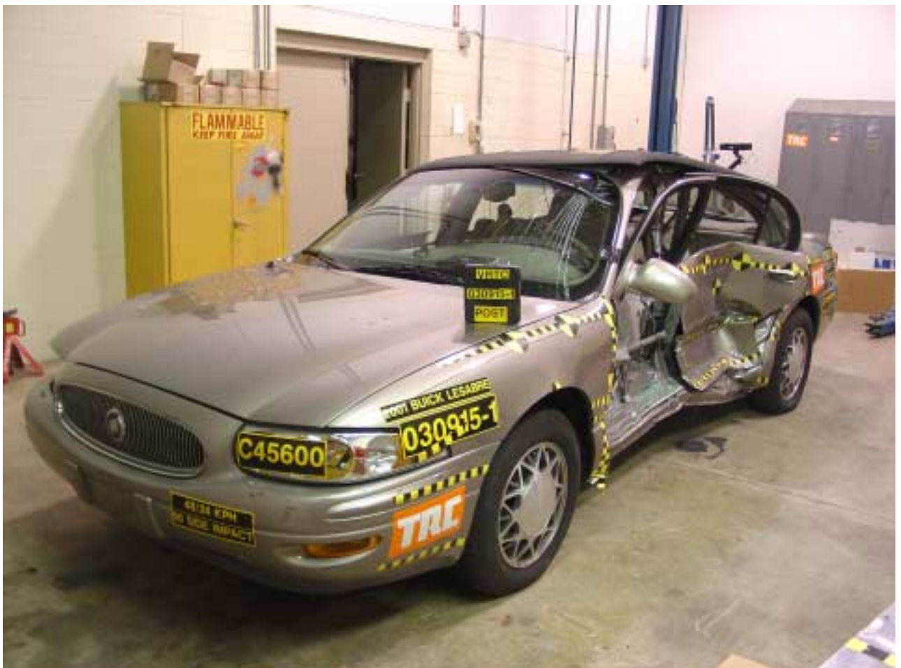
Figure A-49 Post-Test Vehicle Door Deformation Rear Angled View
