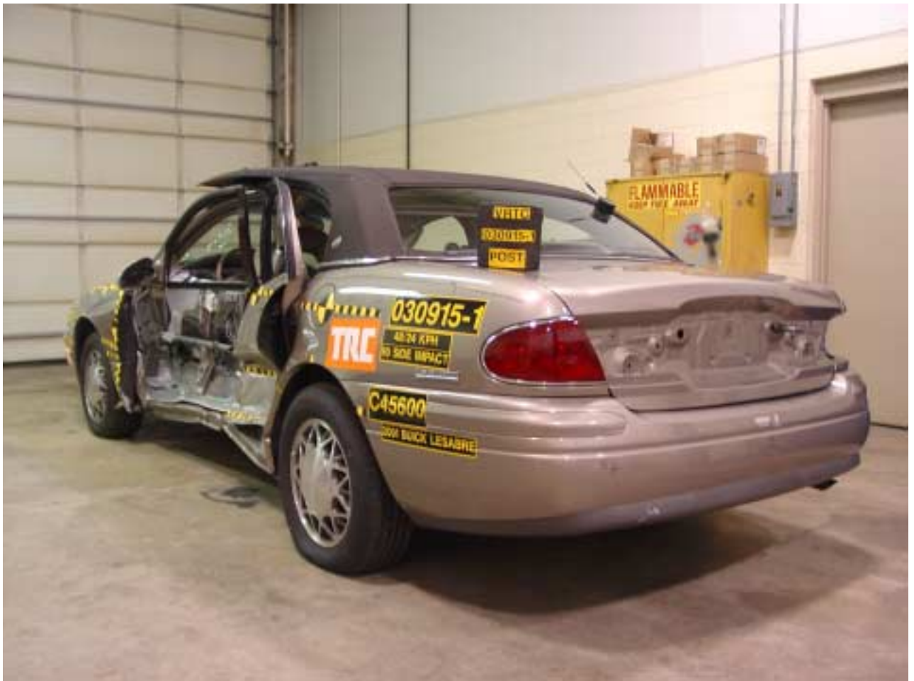
Figure A-48 Post-Test Vehicle Door Deformation Front Angled View
