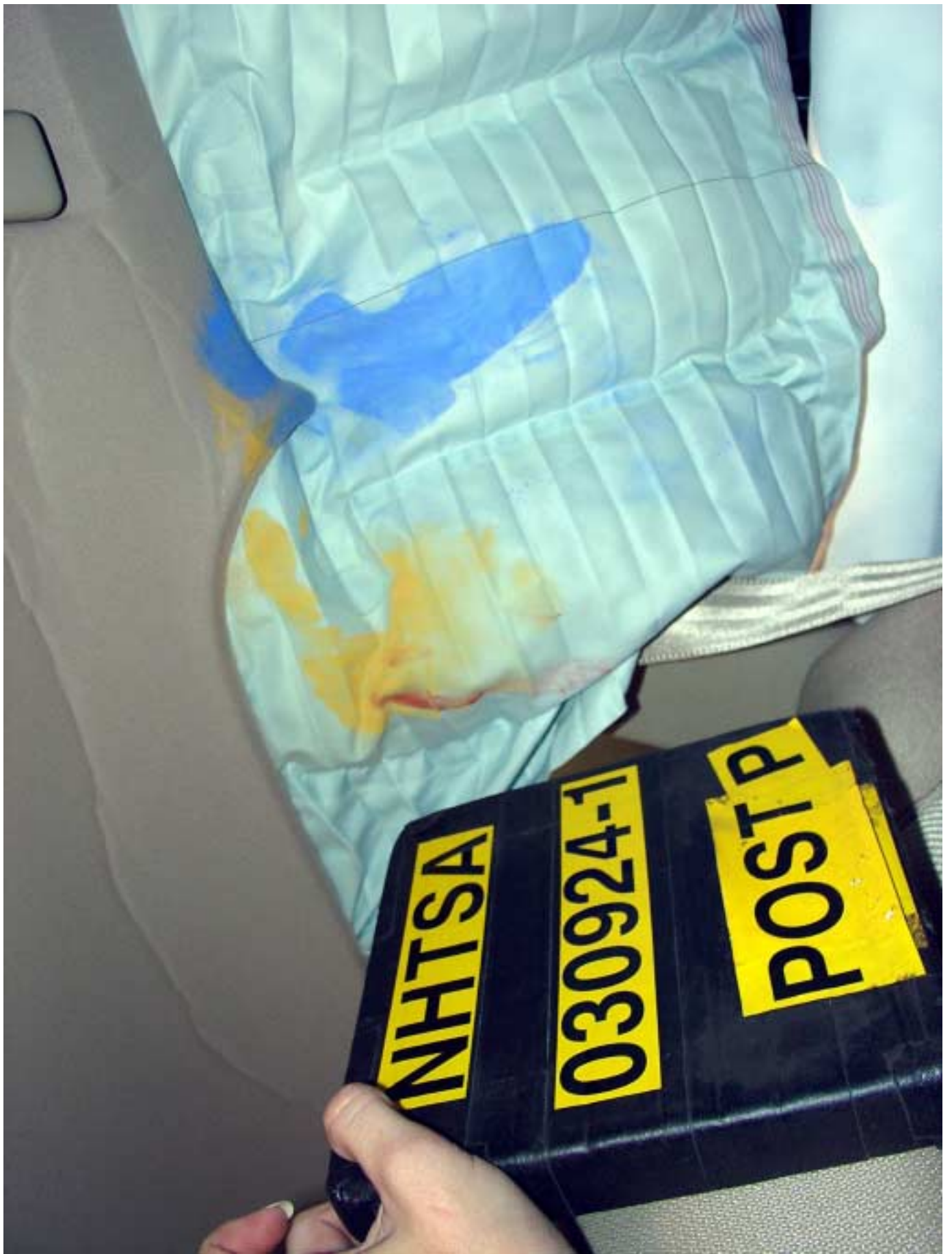
Figure A-41 Post-Test Rear SID HIII Contact View
