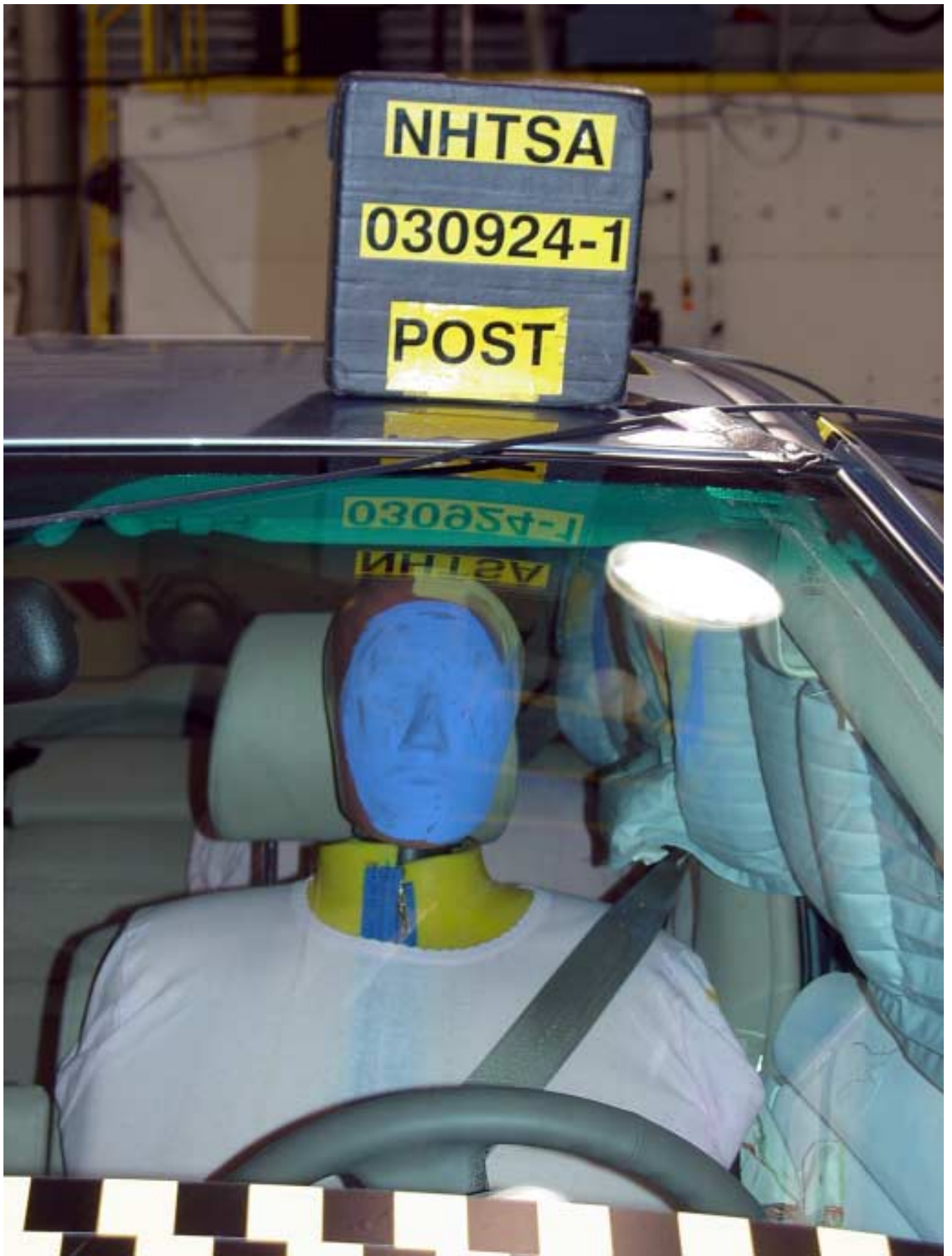
Figure A-30 Post-Test Front View of Front SID HIII and Door Clearance
