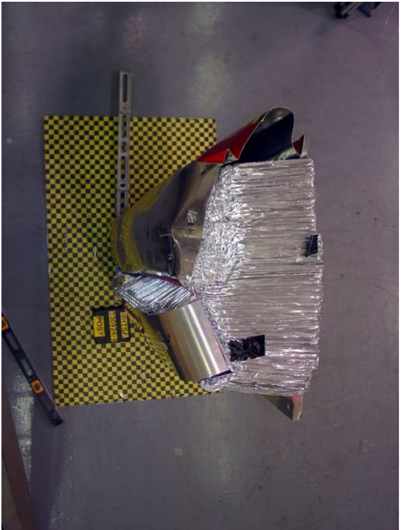
Figure A-14 Post-Test Left Side View of Impactor Face
