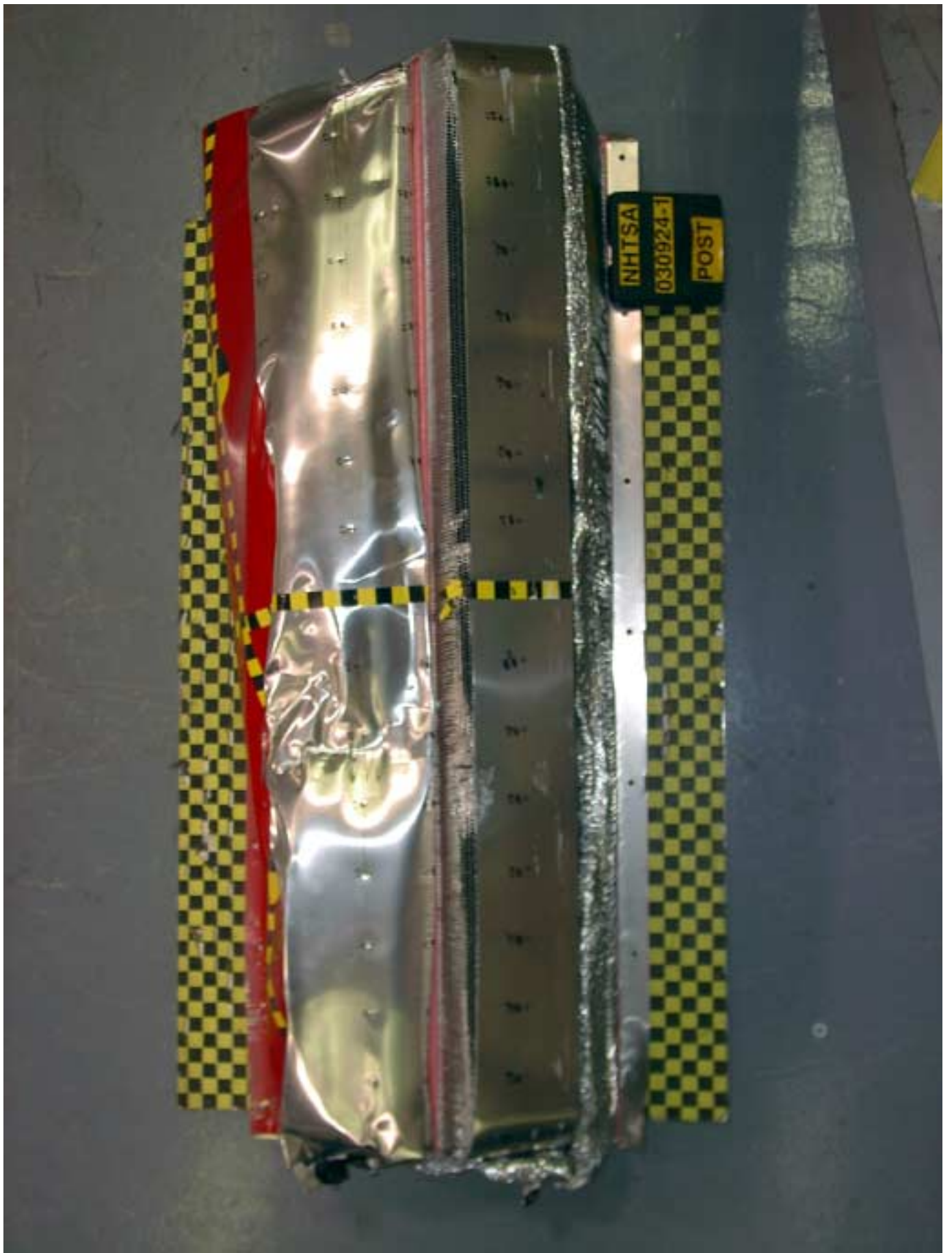
Figure A-12 Post-Test Frontal View of Impactor Face
