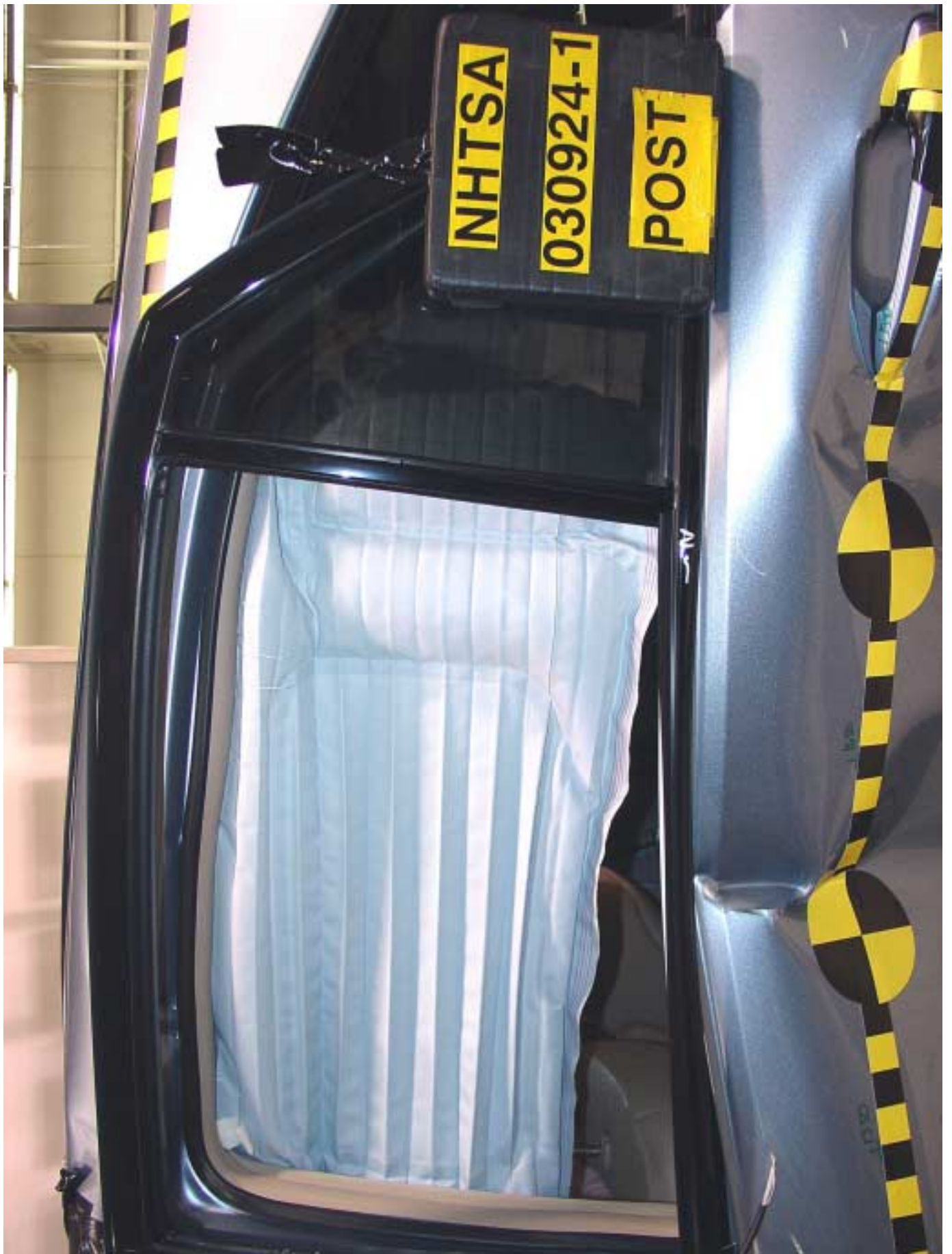
Figure A-32 Post-Test Left View of Rear SID HIII
