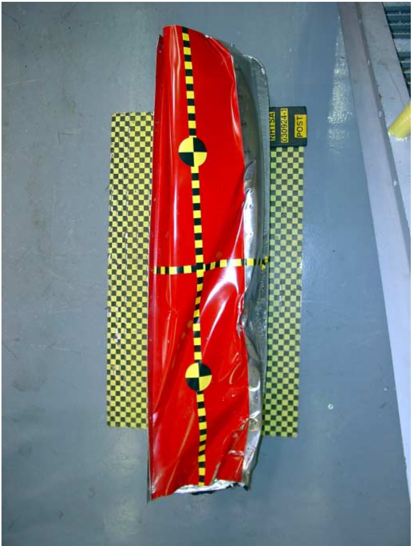
Figure A-18 Post-Test Top View of Impactor Face
