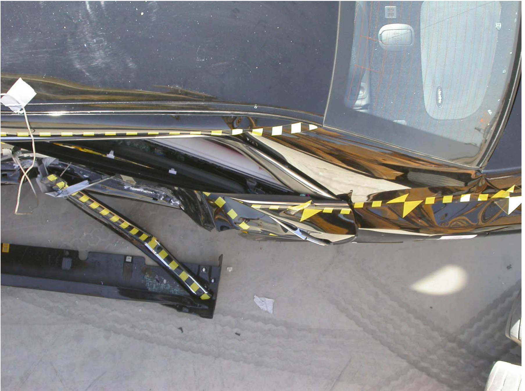
Figure A-42: Passenger Dummy Clearance, Post-Test
