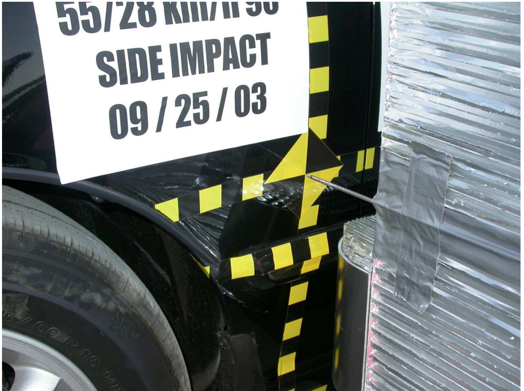
Figure A-19: Impact Point Target Set-up, Pre-Test
