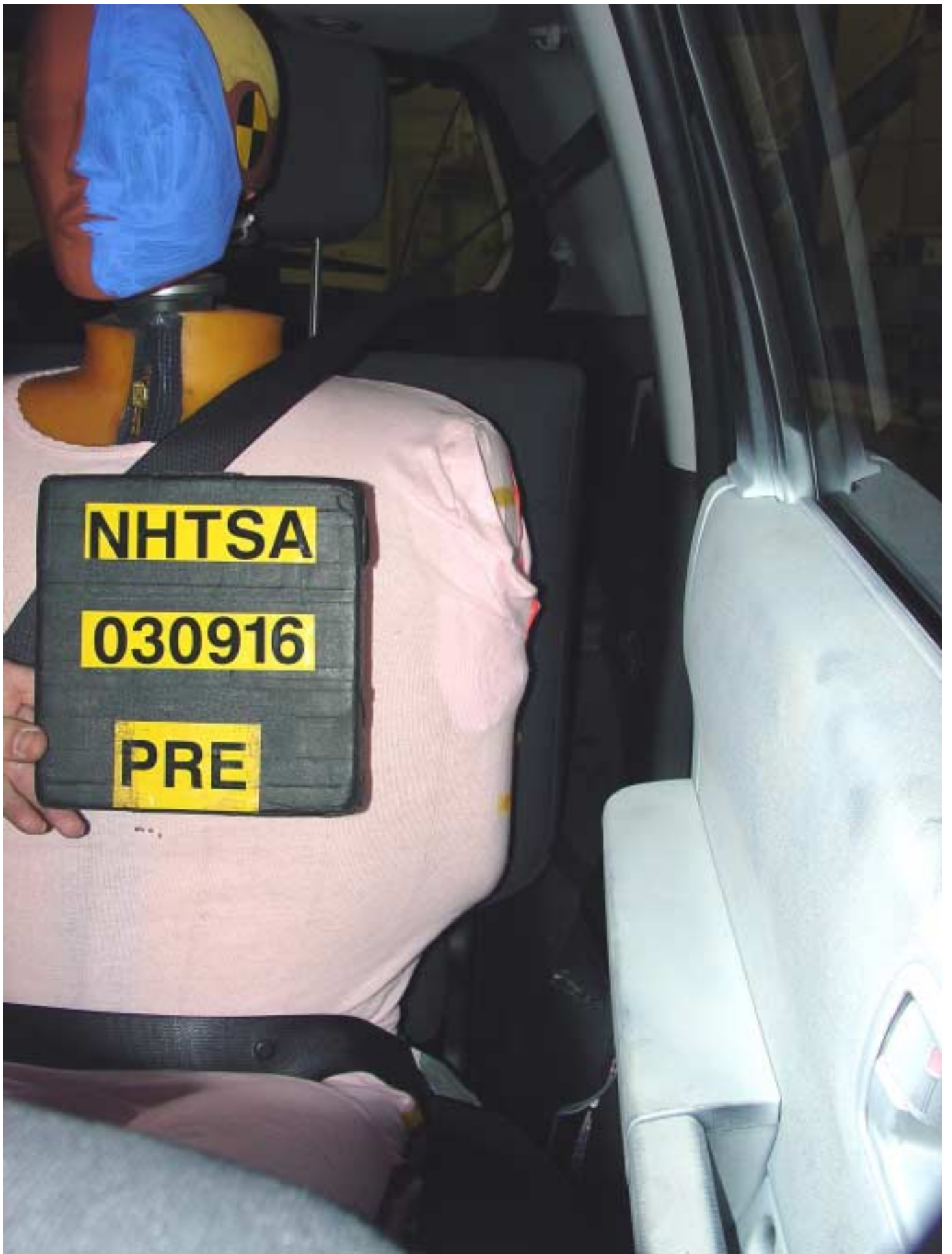
Figure A-32 Pre-Test Left View of Rear SID HIII and Door Clearance
