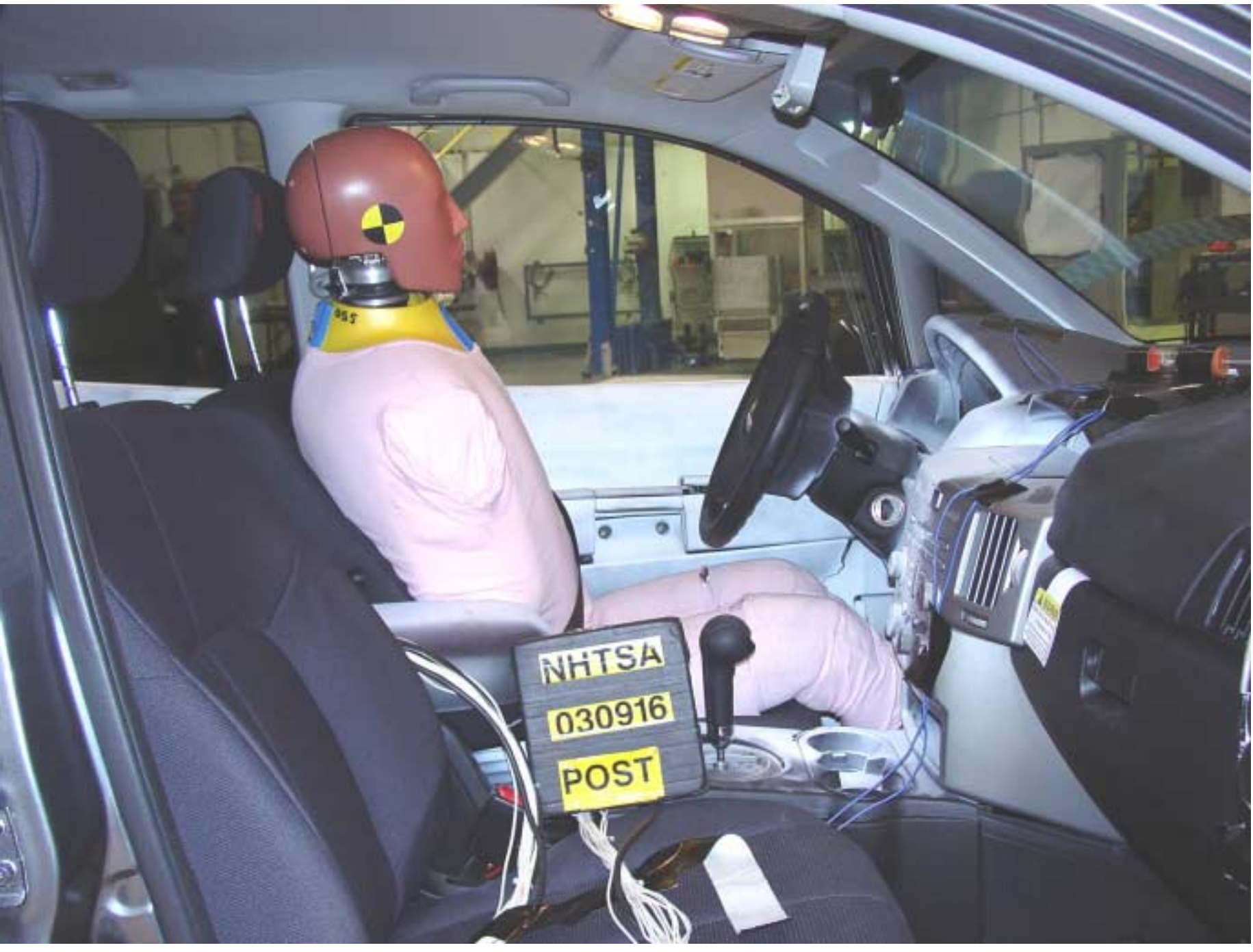
Figure A-21 Post-Test Right Occupant Compartment View of Front SID HIII
