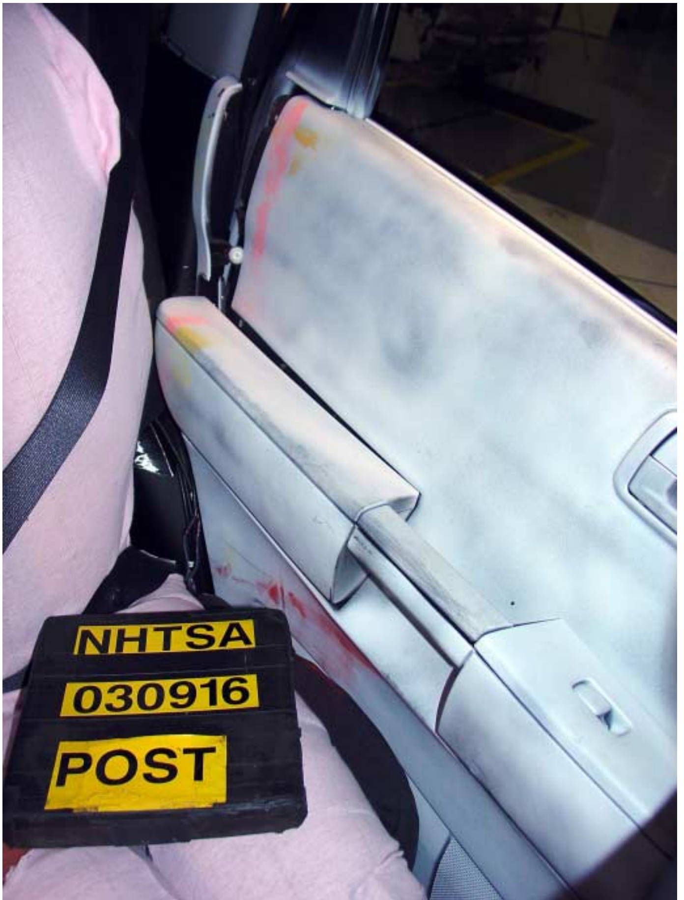
Figure A-33 Post-Test Left View of Rear SID HIII and Door Clearance
