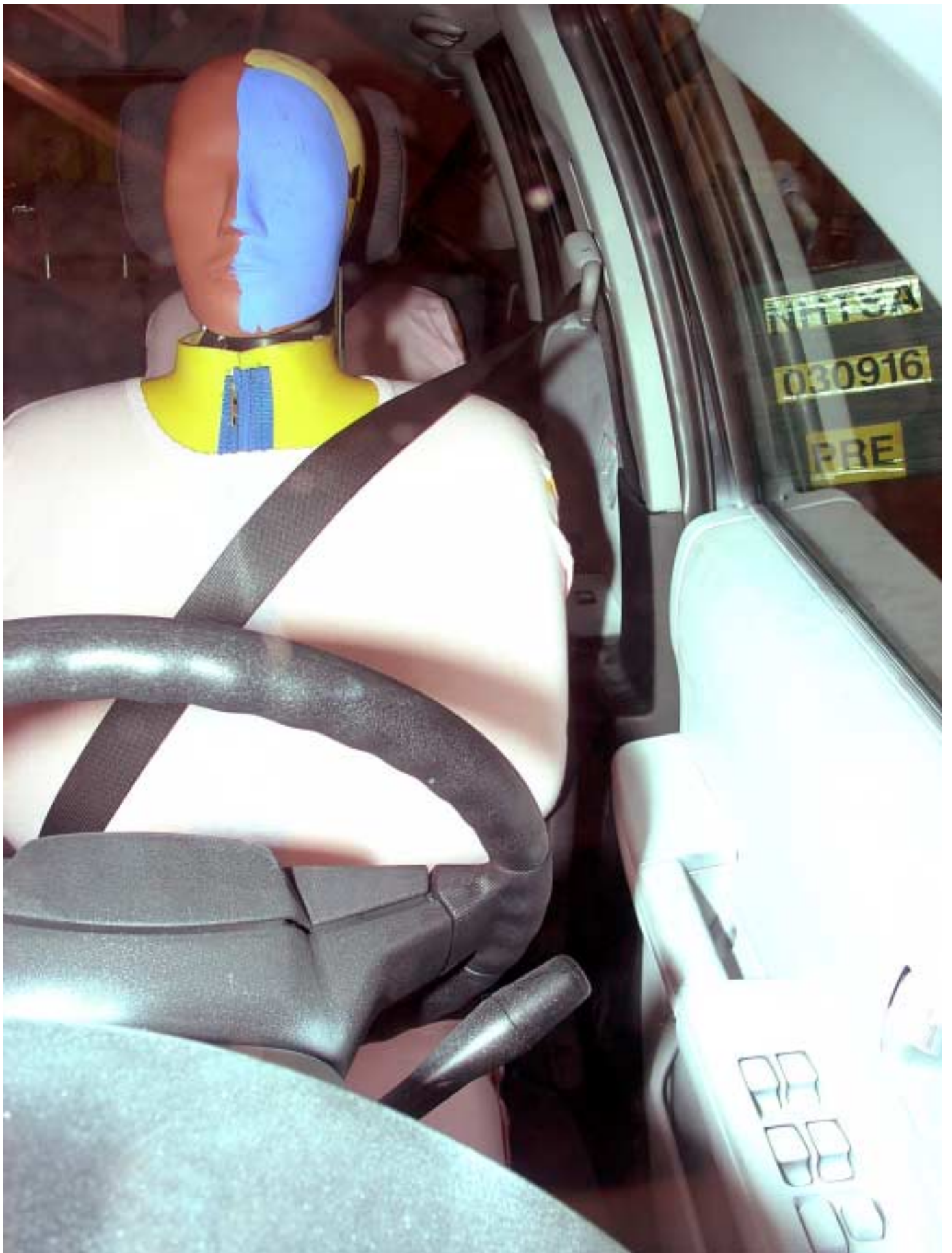
Figure A-27 Pre-Test Left View of Front SID III and Door Clearance
