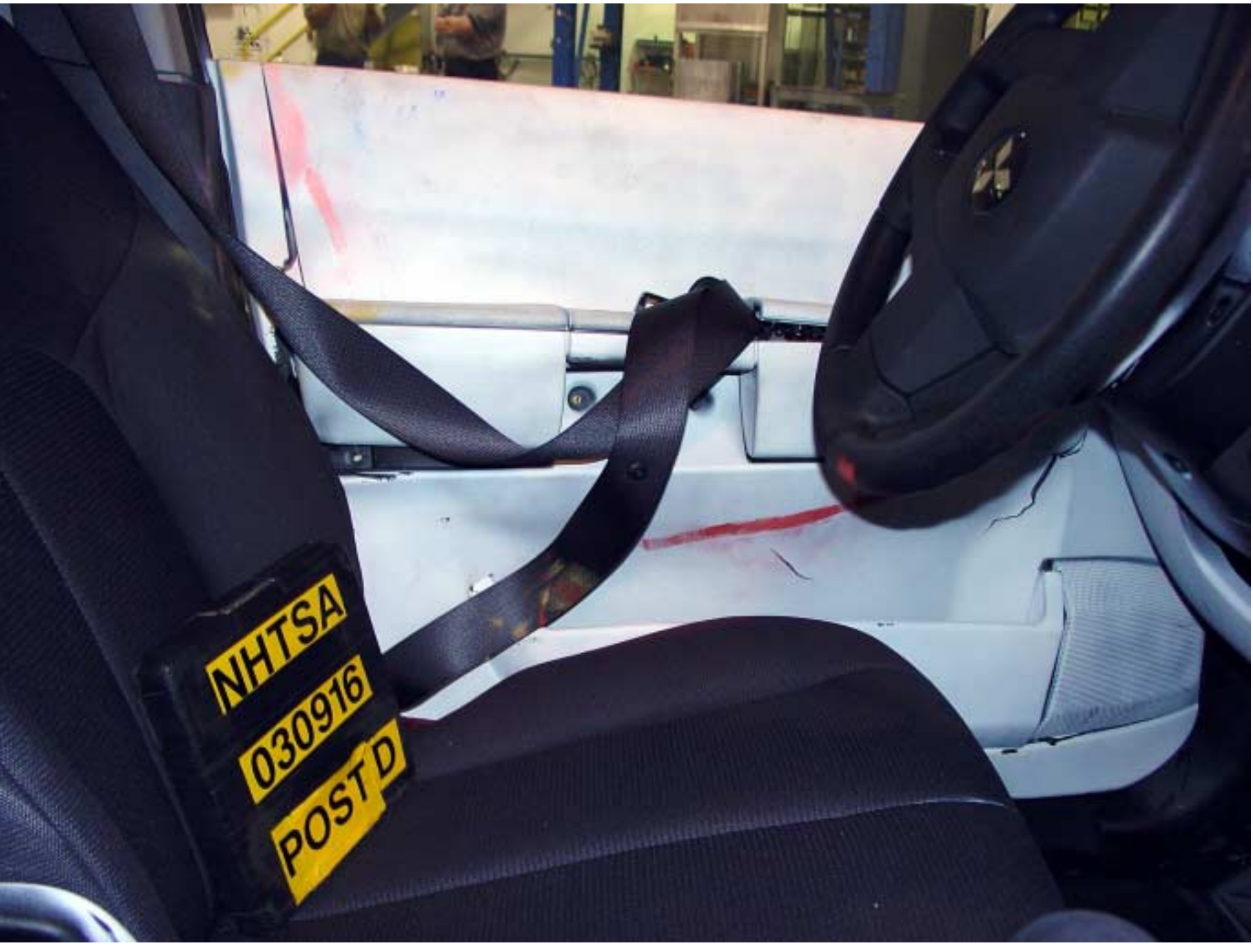
Figure A-35 Post-Test Interior of Front Door Showing SID HIII Impact Locations
