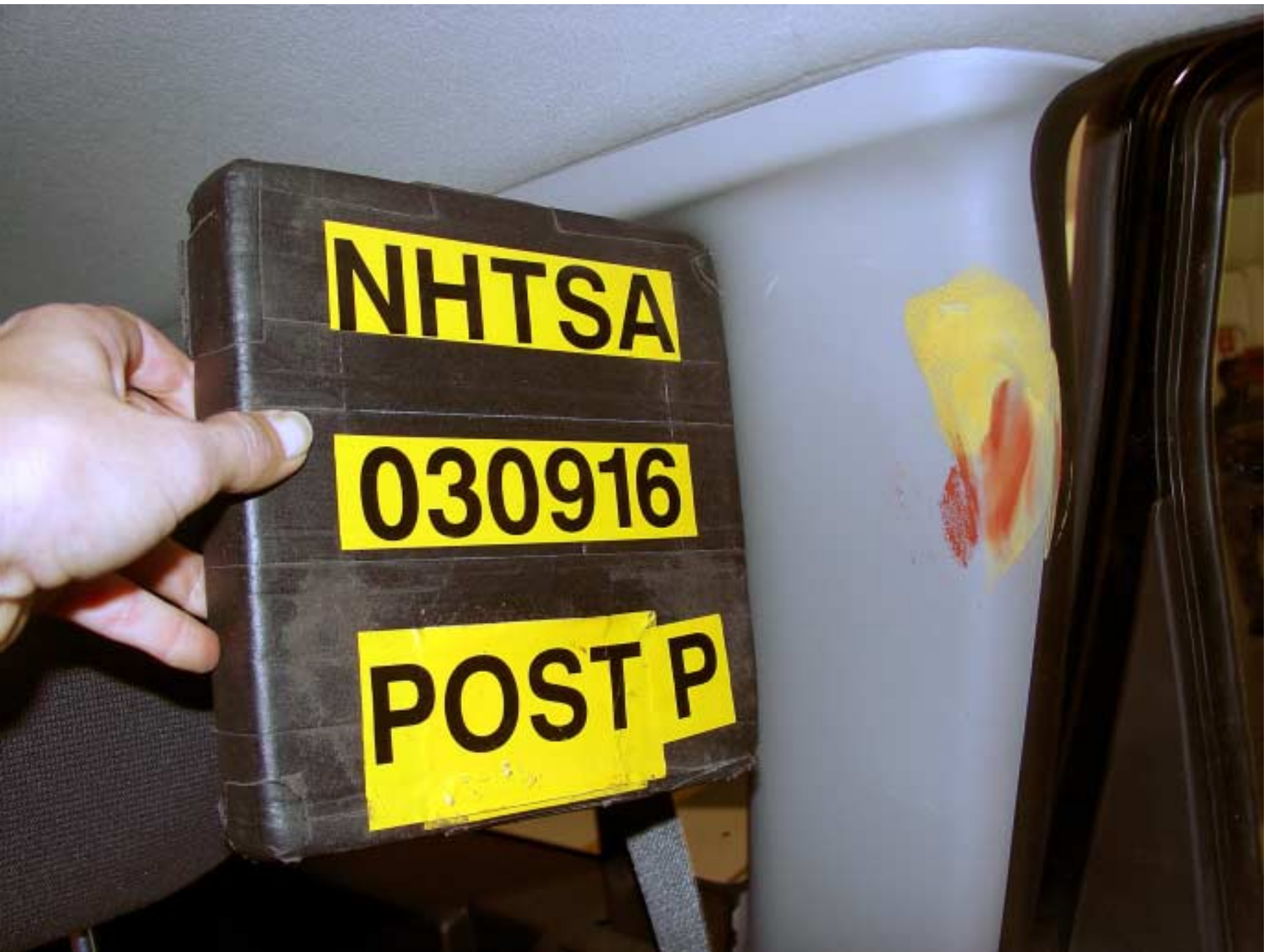
Figure A-40 Post-Test Rear SID HMI Contact View A-43
