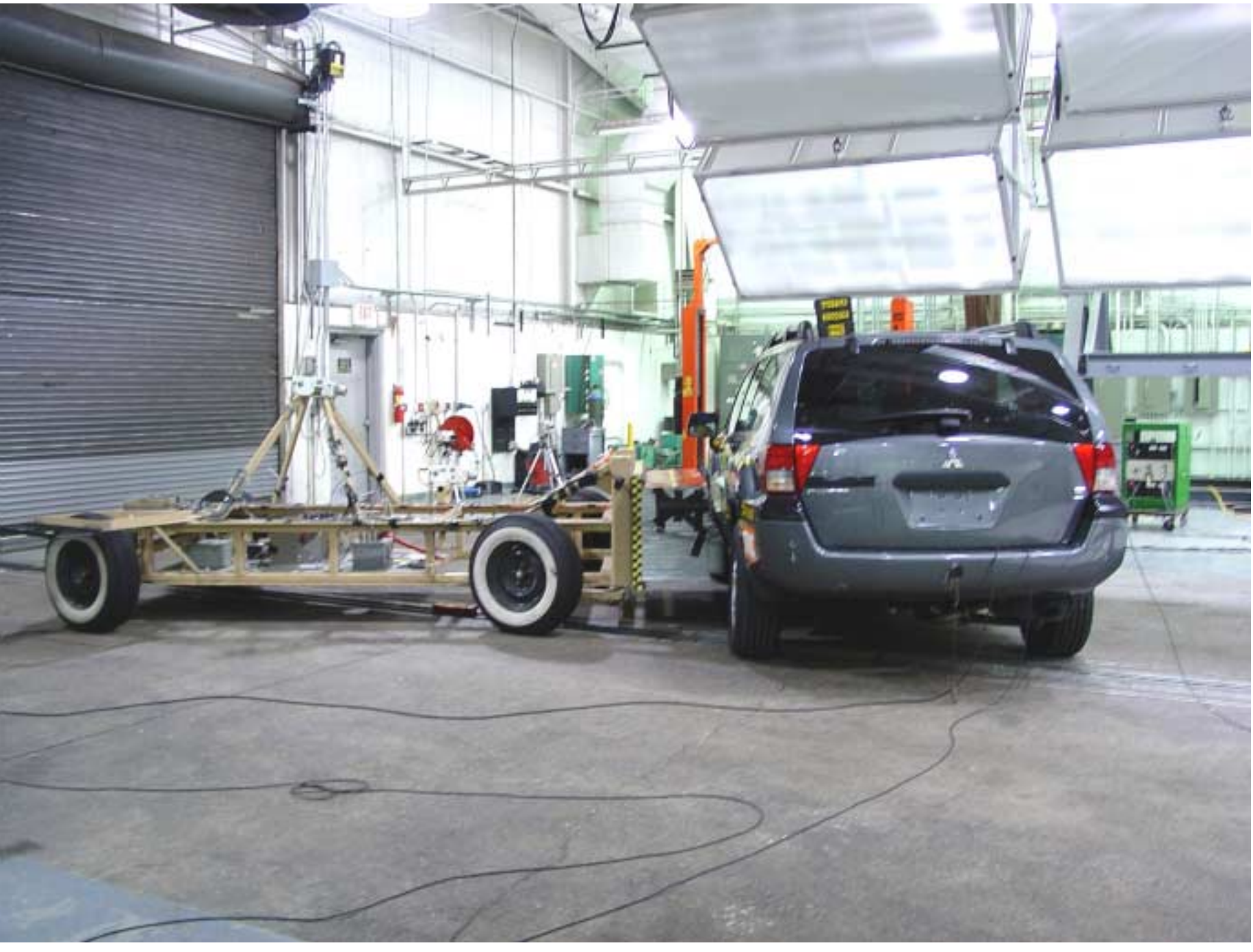
Figure A-44 Pre-Test Right Side View of MDB With Impactor Face in Position
