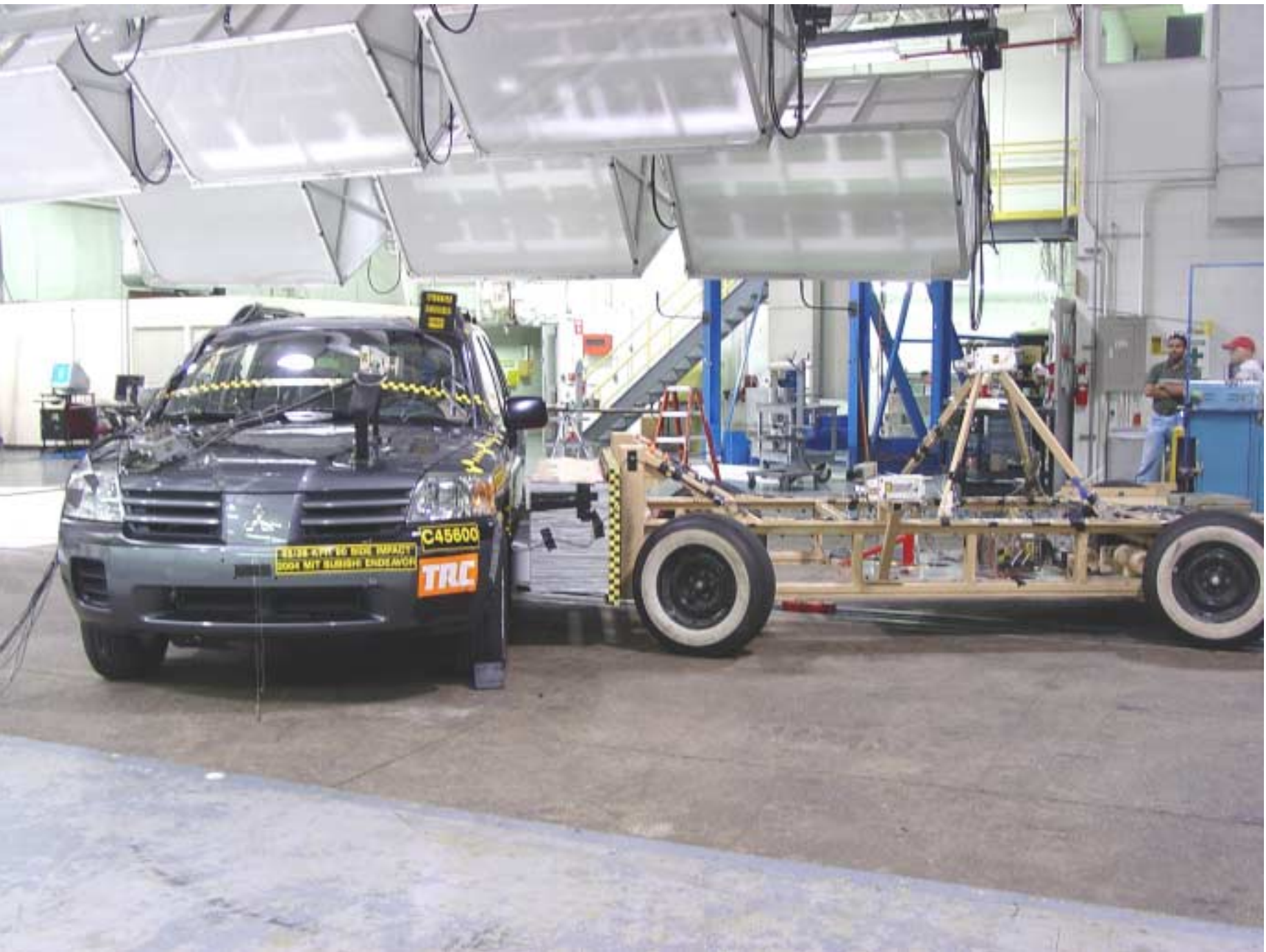
Figure A-41 Pre-Test Left Side View of MDB With Impactor Face in Position
