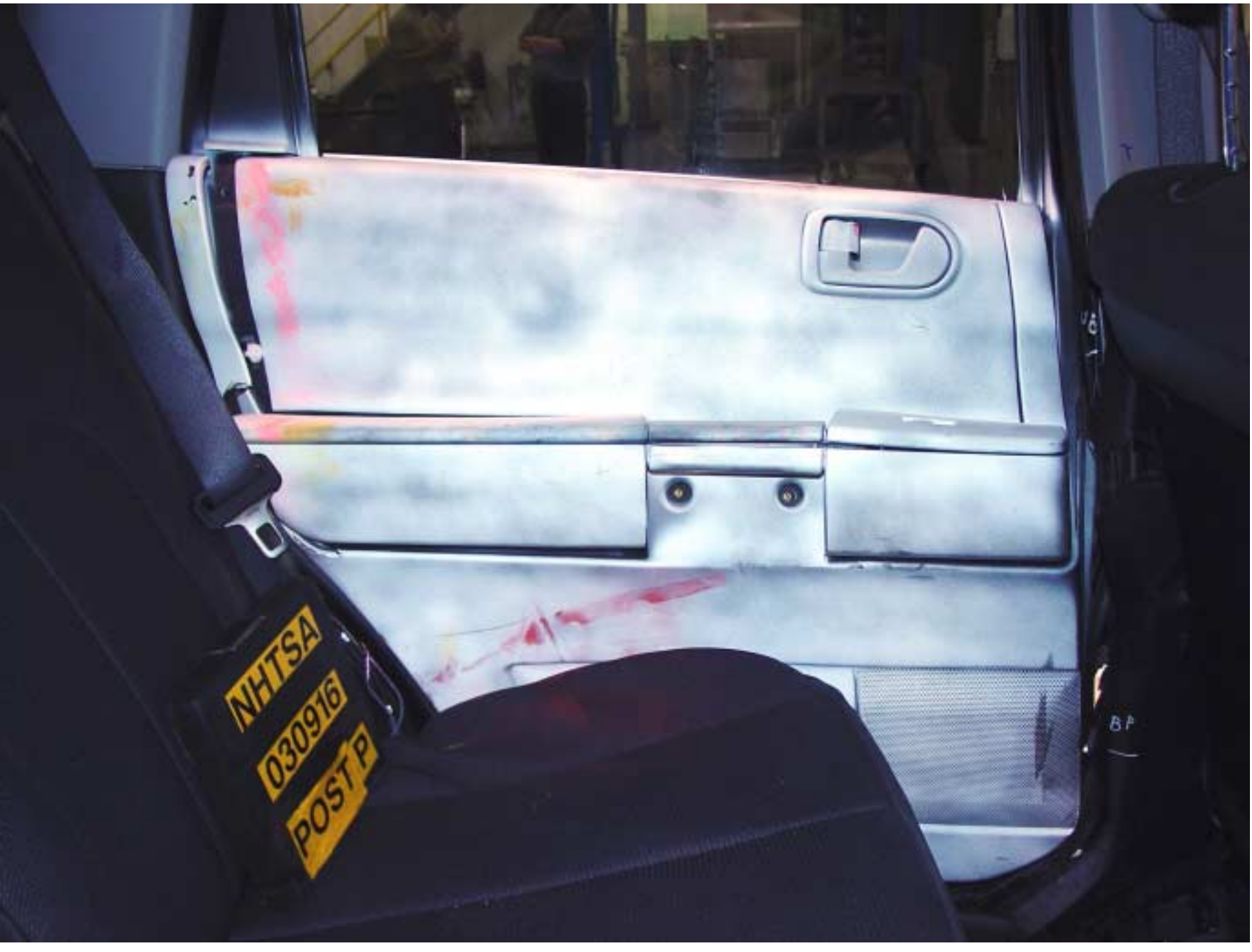
Figure A-39 Post-Test Interior of Rear Panel Showing SID HMMI Impact Locations
